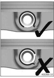
Position the piston pin retainer.
