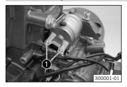
Remove screws ①. Take off the starter motor.
