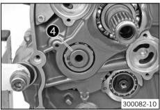
Remove the lock ring 4 and the stop disk.
