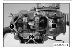
Put on the cylinder head gasket.
