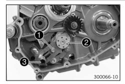
Push sliding plate • away from the shift drum locating •. Remove shift shaft • with the washer.
