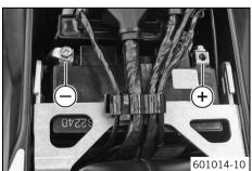
Measure the voltage between the specified points.
