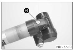
Remove screw 6. Drain the oil.
