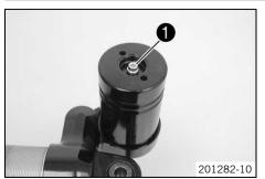
Screw in screw • by approx. 2 rotations but do not tighten.
