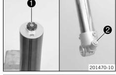
Clamp the fork leg in the area of the lower triple clamp.
