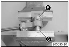
Place special tool **⑤** underneath and press out the heim joint with special tool **⑥**.
