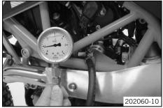
Position the banjo bolt with the connector and sealing rings. Mount and tighten the banjo bolt.
