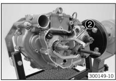
Pull of the timing chain sprocket with the special tool ②.
