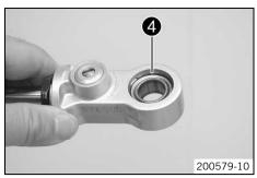
Remove lock rings 4 on both sides.
