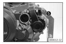
Put on the water pump cover **6**. Mount and tighten screws.
