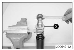
Clamp the special tool in the vise. Loosen screw cover 3.
