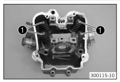
Take shims ① out of the valve spring retainers and lay them to one side according to their normal built-in position.
