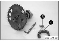
Disconnect the autodecompression spring. Loosen the screw 3 and remove it together with the autodecompression spring and the autodecompression weight 4.
