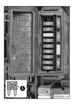
Remove the defective fuse.
