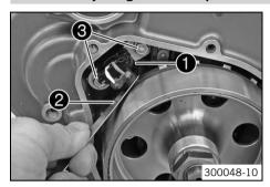
Adjust the distance between the crankshaft position sensor • and the conductive element of the rotor using the special tool •.
