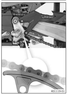
Pull on the upper section of the chain with the specified weight .
