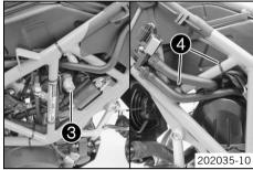
Plug in connector 3 of the lambda sensor. Position the cable and secure it with cable binder 4.
