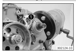
Remove the spacer • of the countershaft.
