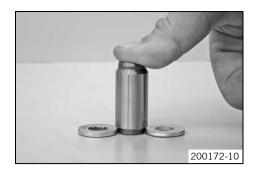
Place two compensating disks or similar aids next to the piston of the timing chain tensioner. This should ensure that when pushed down, the piston does not fully withdraw.
