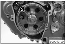
Use the special tool to hold the rotor tight.
