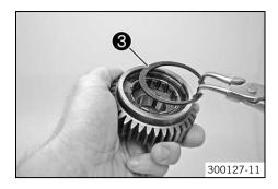
Insert the lock ring 3 into the groove with suitable pliers and check that it is seated correctly.
