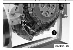
Remove the spacer 1 and spring 2 of the shift shaft.
