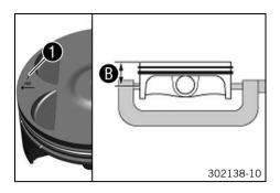
Measure the piston at the piston skirt, at right angles to the piston pin, at a distance 9.
