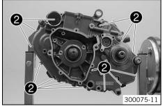
Put on the left engine case half. If necessary, tap lightly with a rubber mallet and turn the transmission shafts.
