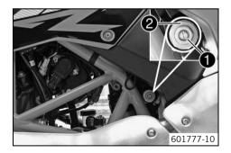
Turn adjusting screw • clockwise with a screwdriver up to the last perceptible click.
