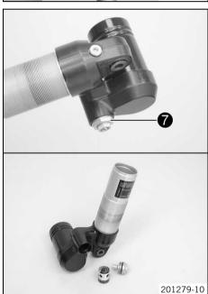
Remove compression adjuster 7. Remove the spring, sleeve, and piston.
