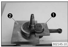
Fix the crankshaft with special tools • and • in the vise.
