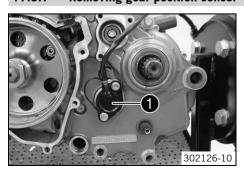
Remove screws. Remove the gear position sensor ①.
