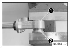
Place special tool 1 underneath and press in the heim joint as far as the center using special tool 2.
