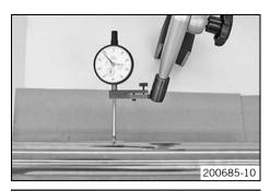
Measure the run-out of the inner tube.
