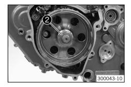
Mount the tab washer and the nut ②. Tighten nut.
