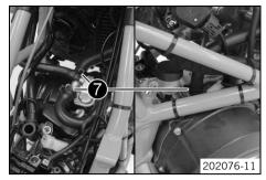
Position the hoses of the engine breather, the SLS and the oil return line. Mount the spring band clamp • using the special tool.
