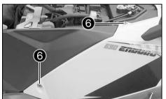
Mount and tighten screws 6.
