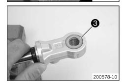
Remove seal rings 3 on both sides.
