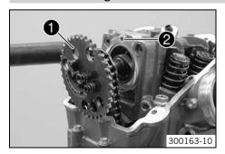
Lay the timing chain over the camshaft. Push the timing chain into the bearing seats. The middle drill hole of the camshaft • and the drill hole of the cylinder head • must be aligned.
