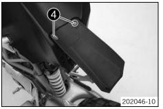
Position the splash protector. Mount and tighten screws 4.
