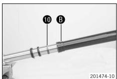
Warm up the outer tube in area of the lower sliding bushings.
