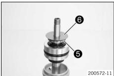
Remove compression shim stack 6 with supporting plate 6.
