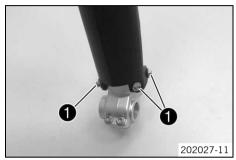
Slide on the fork protector from above and position it. Mount and tighten screws ①.
