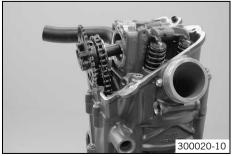
Pull the camshaft out of the bearing seats. Take the timing chain off the camshaft gear. Remove the camshaft.
