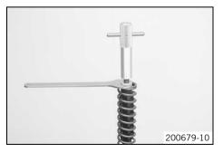
Pull the spring down. Mount the special tool on the hexagonal part.
