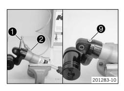
When the pressure gauge reaches the specified value, turn the Damper control lever 4 to Pressure.
