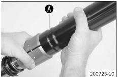
Heat up the outer tube in area of the lower sliding bushings.
