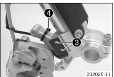
Position the wheel speed sensor. Mount and tighten screws 3.
