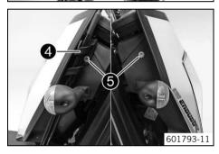
Position brake line guide 4. Mount and tighten screws 5.
