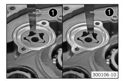
Use a feeler gauge 1 to measure the play between the external rotor and the engine case as well as between the external rotor and the internal rotor.
