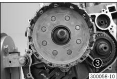
Install the clutch cage 3.
