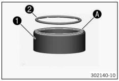
Grease spacer ● in area ● and O-ring ● before mounting.
