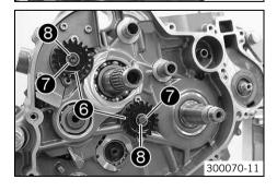
Mount the oil pump gears 6, washers 7 and lock washers 8.
