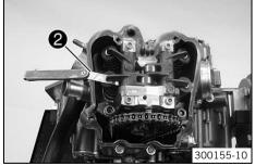
Check the valve clearance on all valves between the valve and the rocker arm using the special tool ②.
