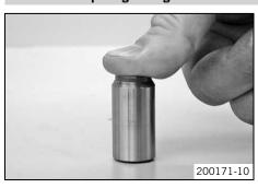
Fully compress the timing chain tensioner.
