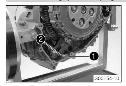
Install the spacer • and spring • of the shift shaft.
