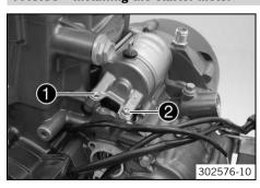
Grease O-ring. Mount the starter motor.
