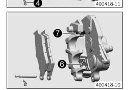
Check that leaf spring 6 in the brake caliper and sliding plate 7 in the brake caliper support are seated correctly.
