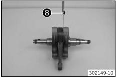
Position the special tool • with the heel at the bottom.
