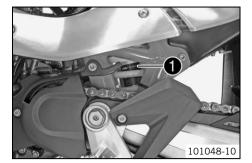
The shock absorber part number **1** is on the left of the shock absorber.
