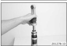
Remove the piston rod. Drain the remaining oil.
