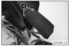
Position the splash protector. Mount and tighten screws 4. Guideline
