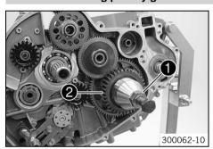
Plug the special tool into the crankshaft.
