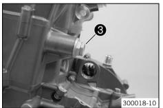
Remove screw 3 and use the special tool to push the timing chain tensioner toward the timing chain.
