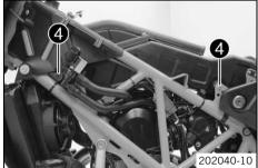
Mount and tighten screws 4.
