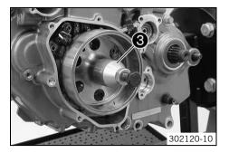
Install the special tool ② on the rotor. Hold it tight using the special tool and pull
