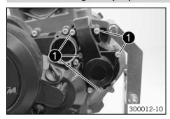
Remove screws ●. Take off the water pump cover.
