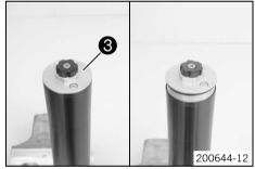
Release the fork leg and clamp it with the axle clamp.
