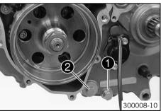
Mount the oil drain plug • with the magnet and a new seal ring and tighten it.
