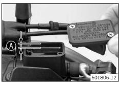
Adjust the brake fluid level to level **(A)**. Guideline
