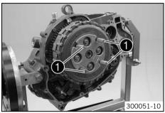
Clamp the antihopping clutch with special tool ①.
