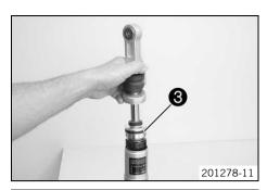
Grease O-ring 3 of the seal ring retainer.
