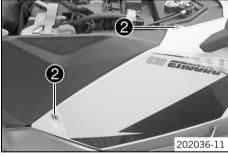
Mount and tighten screws ②.
