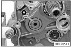
Install the shim 3 and lock ring of the countershaft.
