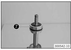
Remove seal ring retainer 7.
