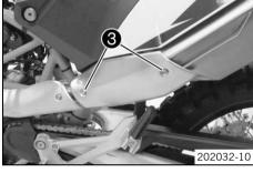
Remove nuts 4 of the manifold.
