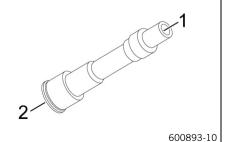
Measure the resistance between the specified points. Measuring point 1 – Measuring point 2
