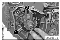
Position the timing chain securing guide ①.
