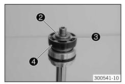
Remove supporting plate 2 and rebound shim stack 3 together with piston 4.
