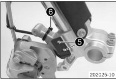
Loosen screws of the triple clamp on both sides. Remove the fork legs from the bottom.
