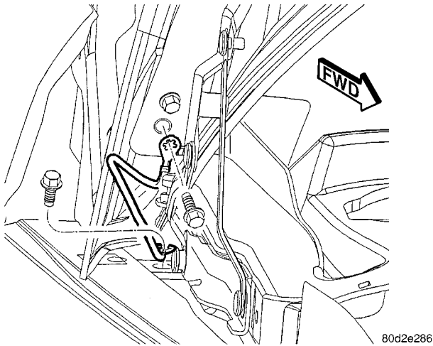
Fig. 12 HOOD HINGE GROUND STRAP
