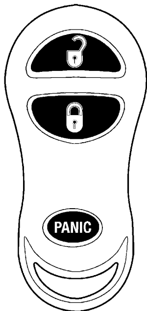
Fig. 3 Remote Keyless Entry (Key Fob) Transmitter
