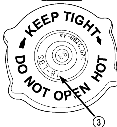
Fig. 15 Cooling System Pressure Cap
