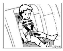
To release the child from the seat belts, separate the shoulder belts then press the buckle release button.
