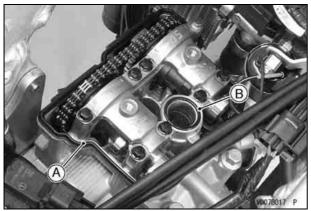
A. Head Cover Gasket B. Spark Plug Hole Gasket • Remove the two caps from the magneto cover.
