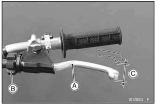
A. Clutch Lever B. Adjuster C. 8 ~ 13 mm (0.3 ~ 0.5 in.) If the clutch lever free play cannot be adjusted at the clutch lever, make the adjustment further down the cable as follows.
