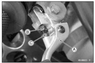
A. Brake Lever B. Adjuster C. Locknut
