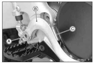
A. Brake Pedal Bolt B. Brake Pedal C. Return Spring
