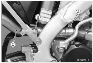
A. Muffler Clamp Bolt B. Muffler Mounting Bolt C. Muffler Body
