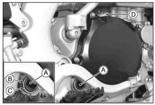
A. Oil Level Gauge B. High Level Line C. Low Level Line D. Oil Filler Plug
