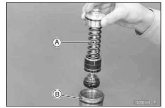
A. Left Front Fork Base Valve Assembly B. Left Front Fork Cylinder Unit
