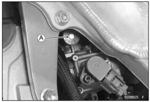
A. Idle Adjusting Screw/Choke Knob
