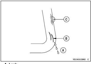
A. Leak B. Cracks
