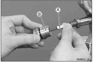
A. Push Rod B. Left Front Fork Adjuster Assembly
