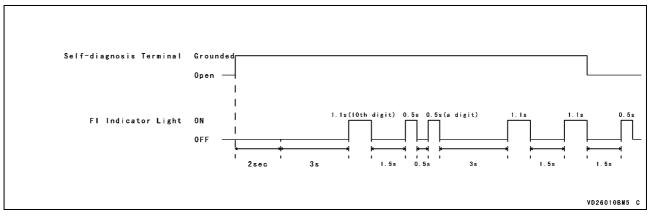
• If the problem is with the following parts, the ECU cannot memorize these problems, the FI indicator light doesn't go on, and no service codes can be displayed.
