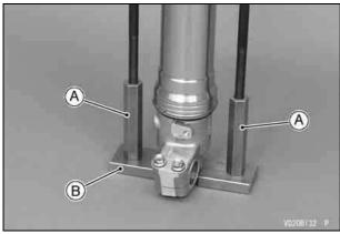
A. Extension Rod (Special Tool: 57001-1753) B. Base (Special Tool: 57001-1753)
