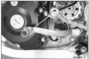
Apply an aerosol cable lubricant with a pressure lubricator on all cables:
