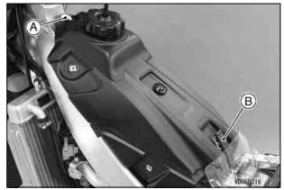
A. Fuel Tank Mounting Bolt B. Band
