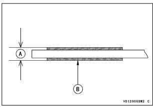
A. Thickness B. Friction Plate
