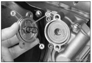
A. Spring B. O-ring C. Oil Filter Cover
