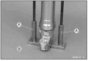
A. Extension Rod (Special Tool: 57001-1753) B. Base (Special Tool: 57001-1753)
