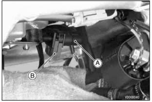
A. Fuel Hose Joint B. Joint Lock
