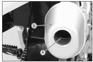
A. Muffler Pipe End B. Baffle
