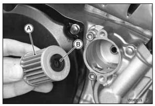
A. Oil Filter Element B. Grommet
