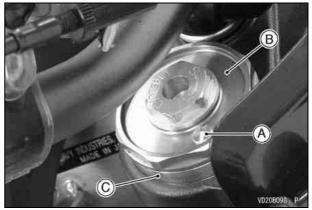
A. Screw B. Front Fork Top Plug C. Front Fork (Right Side)
