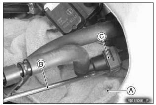
A. Cloth B. Thin Blade Screwdriver C. Joint Lock
