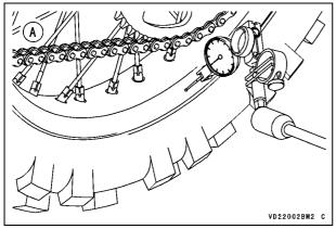
A. Axial Rim Runout Measurement
