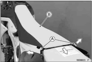
A. Side Covers B. Seat Remove the wing bolt, and take out the air cleaner element.
