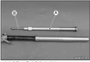
A. Left Front Fork Cylinder Unit B. Piston Rod
