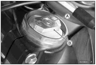
A. Compression Damping Adjuster B. Left Front Fork Base Valve Assembly
