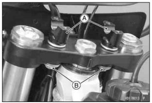
A. Handlebar Holders B. Handlebar Holder Nuts
