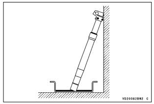
• Install the fork spring with the smaller end facing upward.
