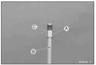
A. Piston Rod Nut B. Piston Rod C. 13 mm (0.51 in.) or more • Install the spring collar.
