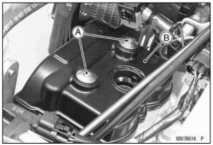
A. Cylinder Head Cover Bolts and Washers B. Cylinder Head Cover
