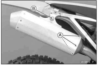
A. Muffler Cover Bolts B. Muffler Mounting Bolt • Remove the muffler cover with the plastic mallet.
