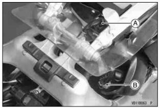
A. Intake Air Temperature Sensor Connector B. Upstream Injector Connector
