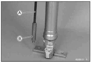
A. Compression Shaft B. Extension Rod (Special Tool: 57001-1753) • Screw the extension rod (special tool: 57001 -1753) into the base (special tool: 57001-1753).
