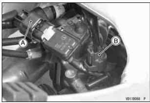
A. Intake Air Pressure Sensor Connector B. Downstream Injector Connector • Free the main harness from the clamps.
