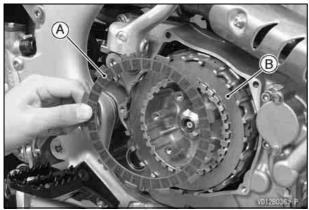
A. Friction Plate B. Steel Plate
