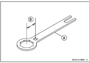
A. Top Plug Wrench (Special Tool: 57001-1645) B. Distance • Install the front brake caliper to the fork leg, and tighten the front caliper mounting bolts to the specified torque.
