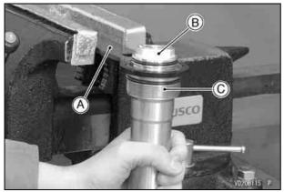
A. Top Plug Wrench (Special Tool: 57001-1645) B. Left Front Fork Base Valve Assembly C. Left Front Fork Cylinder Unit
