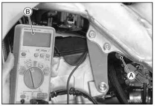
A. Idle Adjusting Screw/Choke Knob B. Tester
