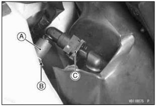
A. Fuel Hose Joint B. Yellow Paint C. Joint Lock
