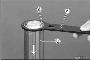
A. Top Plug Wrench (Special Tool: 57001-1645) B. Left Front Fork Cylinder Unit C. Left Front Fork Outer Tube • Place a drain pan under the front fork and drain fork oil.
