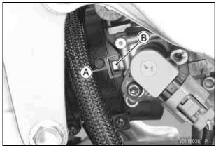
A. Groove B. Projection • Hold the main harness to the clamps.
