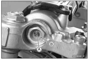
A. Rebound Damping Adjuster B. Left Front Fork Cylinder Valve
