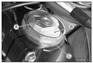
A. Screw B. Front Fork Top Plug C. Front Fork (Left Side)
