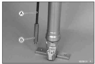
A. Compression Shaft B. Extension Rod (Special Tool: 57001-1753)
