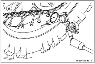
A. Radial Rim Runout Measurement
