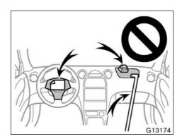
• Do not put objects or your pets on or in front of the dashboard or steering wheel pad that houses the front airbag system. They might restrict inflation or cause death or serious injury as they are projected rearward by the force of deploying airbags. Likewise, the driver and front passenger should not hold things in their arms or on their knees.
