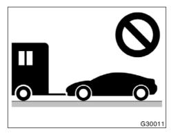
Your vehicle is not designed to be dinghy towed (with four wheels on the ground) behind a motorhome.
