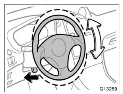
To change the steering wheel angle, hold the steering wheel, push the lock release lever, tilt the steering wheel to the desired angle and return the lever to its original position.
