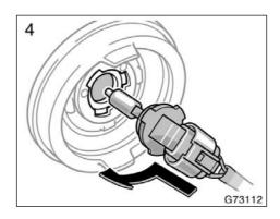
4. Insert the bulb base into the mounting hole by turning it clockwise.
