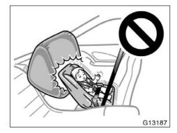
Never put a rear-facing child restraint system on the front passenger seat because the force of the rapid inflation of the front passenger airbag can cause death or serious injury to the child.
