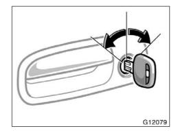
LOCKING AND UNLOCKING WITH KEY Insert the key into the keyhole and turn it
