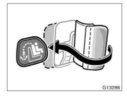
Slide the back-plate of the flap under the carpet to cover the anchor bracket when it is not in use.
