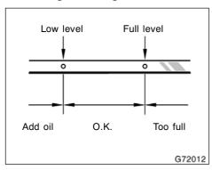
With the engine at operating temperature and turned off, check the oil level on the dipstick.
