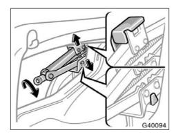
To store the jack, put the jack base on the fitting place. Turn the joint until the jack upper side fits securely with the protrusion of the carrier.
