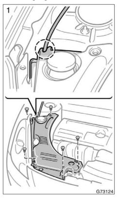
RIGHT SIDE PARKING LIGHT—Remove and install the clips as shown in the following illustrations.
