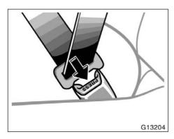
4. To remove the infant seat, press the buckle-release button and allow the belt to retract completely. The belt will move freely again and be ready to work for an adult or older child passenger.
