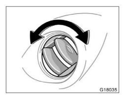
You can change air flow direction by turning the instrument panel vents.
