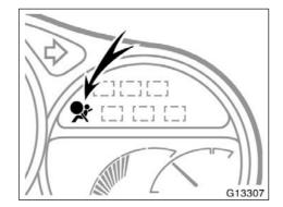
This indicator comes on when the ignition key is turned to the "ON" position. It goes off after about 6 seconds. This means the SRS side airbags are operating properly.
