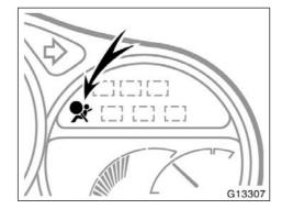
This indicator comes on when the ignition key is turned to the "ON" position. It goes off after about 6 seconds. This means the front seat belt pretensioners are operating properly.
