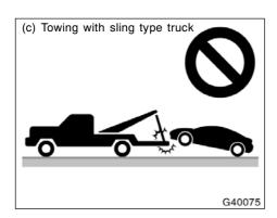
(c) Towing with sling type truck
