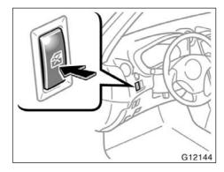
If you push in the window lock switch on the instrument panel, the passenger's window cannot be operated.
