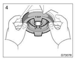
Install the rubber cover with the "TOP" mark upward, and snuggle on the boss. Insert the connector.
