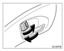
LOCKING AND UNLOCKING WITH INSIDE LOCK KNOB
