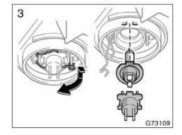
Release the bulb retaining spring and remove the bulb along with the socket. Install a new bulb into the socket and return the bulb retaining spring to its original position.
