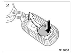
2. Remove the discharged transmitter batterv.
