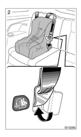
2. Fix the child restraint system with the seat belt.
