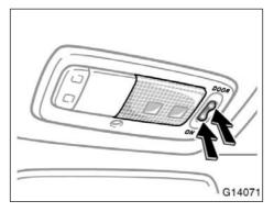
To turn the interior light on, push the "ON" or "DOOR" side switch. To turn the light off, push the switch lightly on the opposite side.
