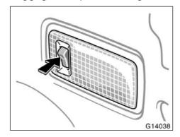
To turn the luggage compartment light on, open the back door and push the switch. Closing the back door will turn the light off.
