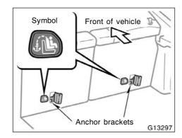
Use the anchor bracket on the rear of the seat back to attach the top strap.
