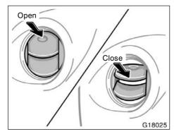
If air flow control is not satisfactory, check the instrument panel vents. The instrument panel vents may be opened or closed as shown.
