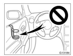
• Do not attach a cup holder or any other device or object on or around the door. When the side airbag inflates, the cup holder or any other device or object will be thrown with great force or the side airbag may not activate correctly, resulting in death or serious injury. Likewise, the driver and front passenger should not hold things in their arms or on their knees.
