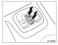
LOCKING AND UNLOCKING WITH POWER DOOR LOCK SWITCH
