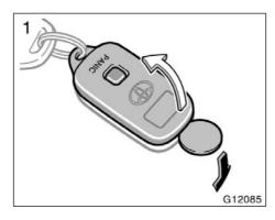
1. Using a coin or equivalent, open the transmitter case.
