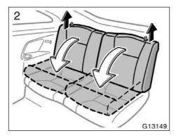
2. Pull the lock release button and fold down the seatback.
