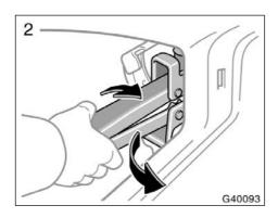
2. Twist the jack head clockwise and pull out the jack.
