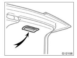
When closing the back door, use the inside handle for easier reach to the back door.
