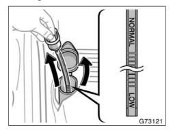
If any washer does not work, the washer tank may be empty. Check the washer fluid level on the level gauge. If the washer fluid level is below "LOW", add washer fluid.
