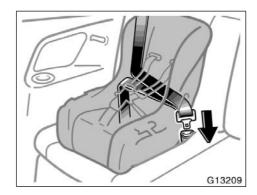
Run the lap and shoulder belt through or around the convertible seat following the instructions provided by its manufacturer and insert the tab into the buckle taking care not to twist the belt. Keep the lap portion of the belt tight.
