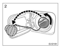
2. To remove the fuel tank cap, turn the cap slowly counterclockwise, then pause slightly before removing it. After removing the cap, hang the tether as shown in the illustration.
