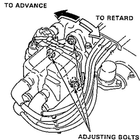
6. Tighten the adjusting bolts recheck the timing.
