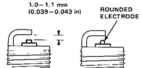
5. Adjust the gap with a suitable gapping tool.
