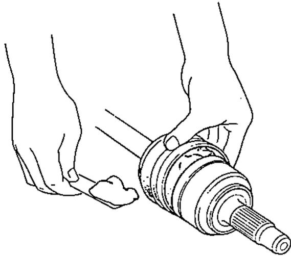
10. Adjust the length of the driveshafts to the figure below, then adjust the boots to halfway between full compression and extension.
