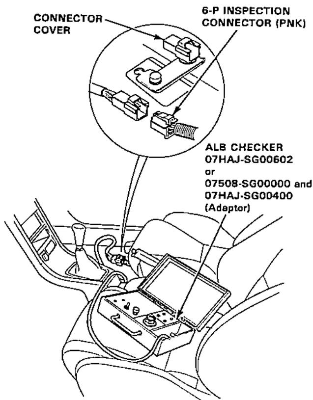
NOTE: The adaptor 07HAJ-SG00400 is not necessary when using of the checker 07HAJ-SG00602.
