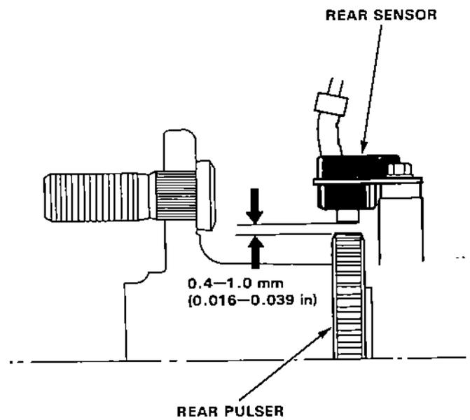
2. Measure air gap between the sensor and pulser all the way around while rotating the driveshaft by hand.
