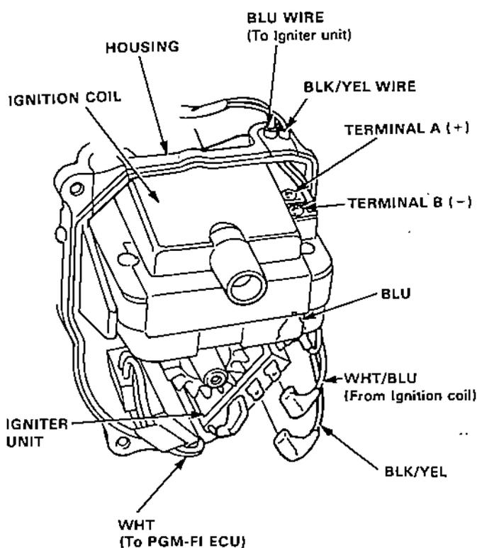
5. Disconnect the WHT/BLU wire from the Igniter unit. There should be battery voltage between the WHT/BLU (+) wire and body ground.
