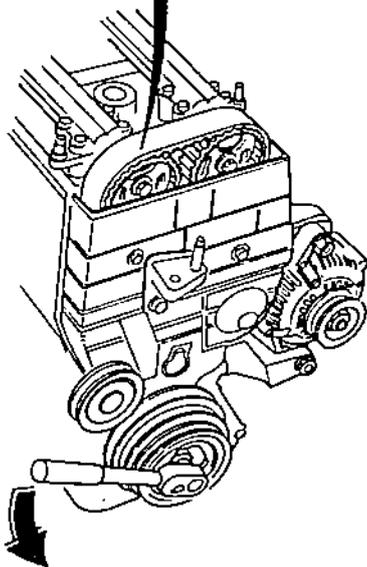
4. If the pulley bolt loosens while turning the crank, retorque it to 120 N·m(12.0 kg-m, 87 lb-ft).
