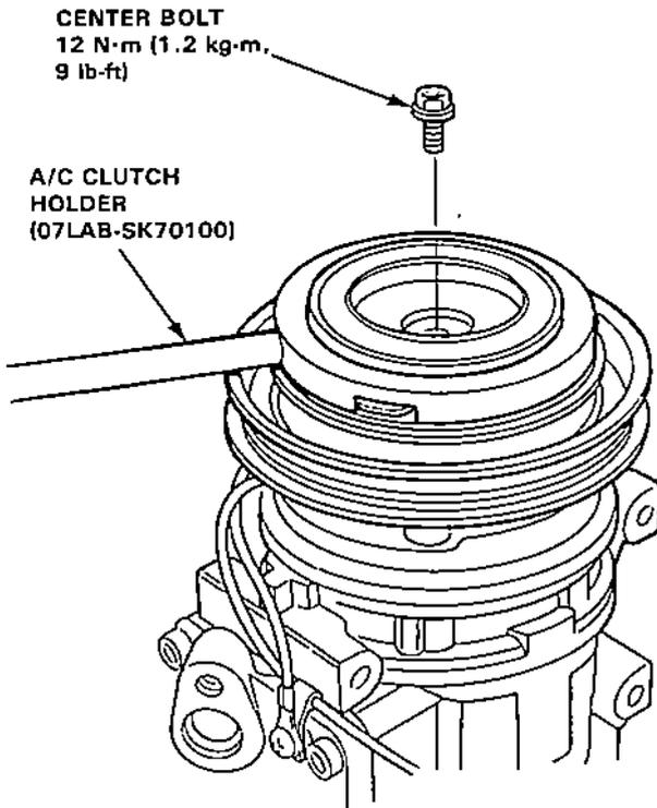
2. Remove the pressure plate and shim(s) taking care not to lose the shims.
