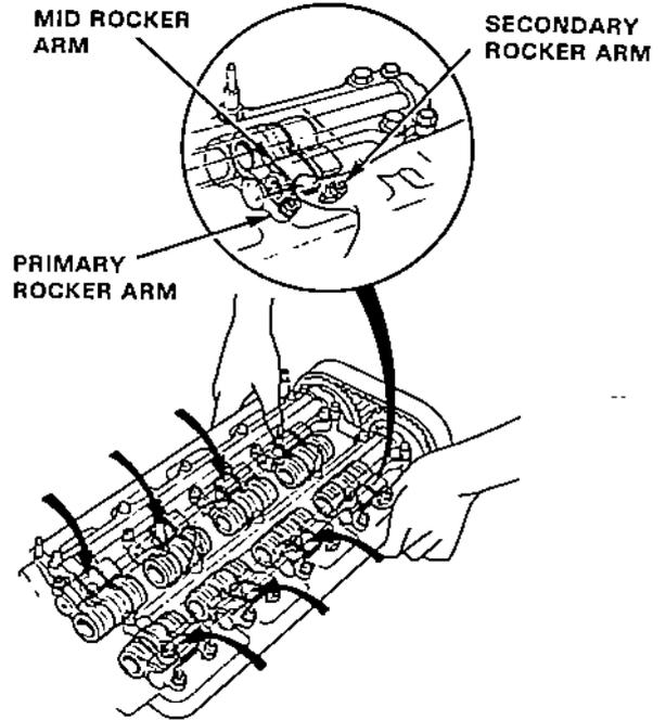
7. Check the mid rocker arm of each cylinder at TDC.
