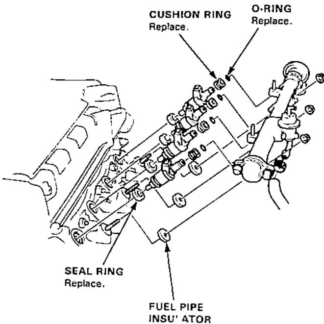
7. Slide new cushion rings onto the injectors.
