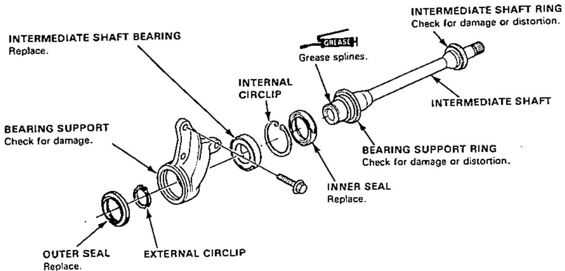
**CAUTION:** Be careful not to damage the rubber on the bearing support during installation.
