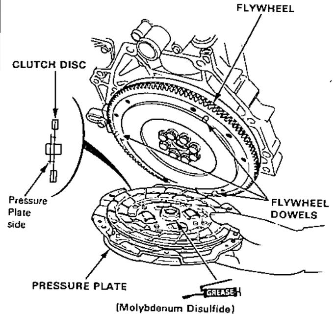
4. Install the attaching bolts finger tight.
