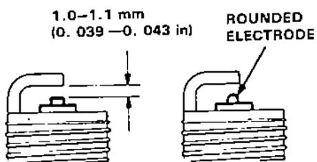
3. Adjust the gap with a suitable gapping tool.
