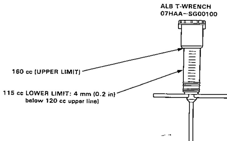
NOTE: The fluid enters the reservoir under pressure; wait 1 or 2 minutes for air bubbles to disappear and level to stabilize.
