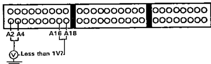
Repair open in wire between ECU and thermostat housing (G101) that had more than 1V.
