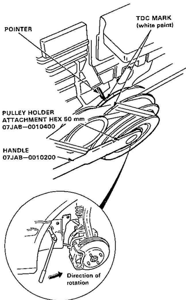
NOTE: If the pulley bolt loosens while turning the crank, retorque it to 120 N·m (12.0 kg-m, 87 lb-ft).
