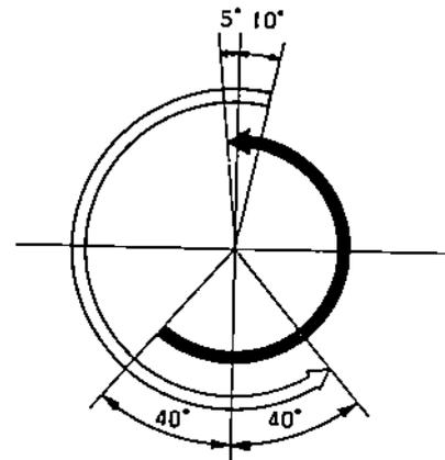
High-speed valve timing
