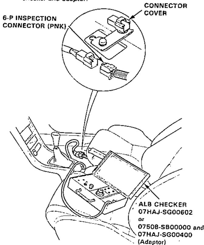
NOTE: The adaptor 07HAJ-SG00400 is not necessary when using of the checker 07HAJ-SG00602.
