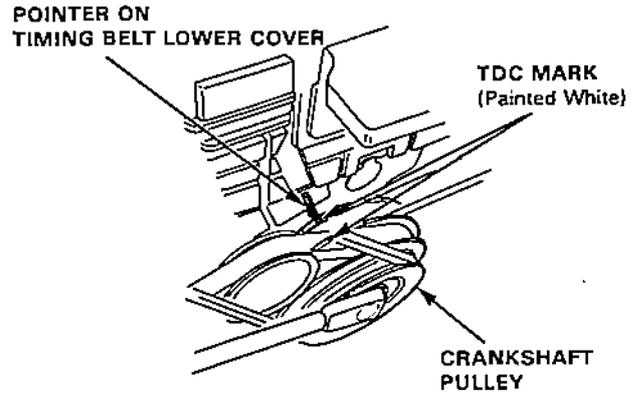
3. Adjust valve clearance on No. 1 cylinder.
