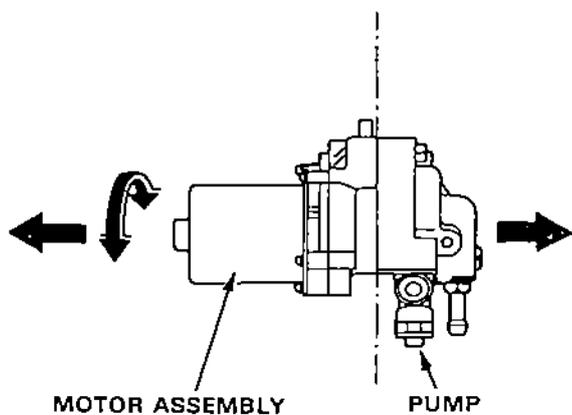
NOTE: About 10 cc(0.6cu-in)of brake fluid will flow out when the motor is removed from the pump.
