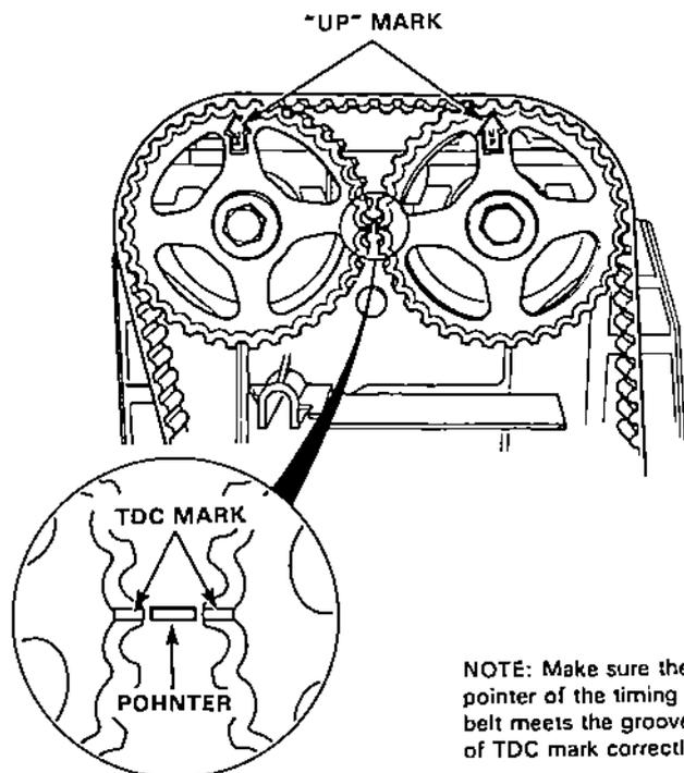
NOTE: Make sure the pointer of the timing belt meets the grooves of TDC mark correctly.
