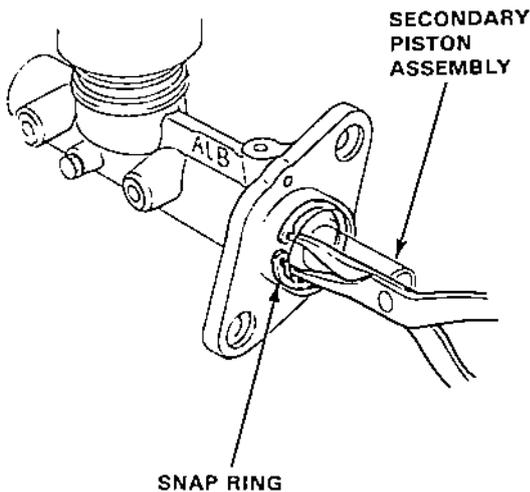
3. Remove the stop bolt while pushing in the secondary piston assembly.
