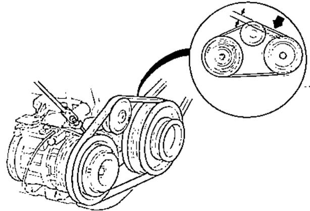
② When using ND tension gauge:
