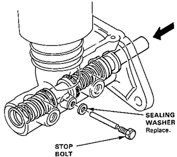
4. Remove the piston guide, secondary piston assembly and primary piston assembly.
