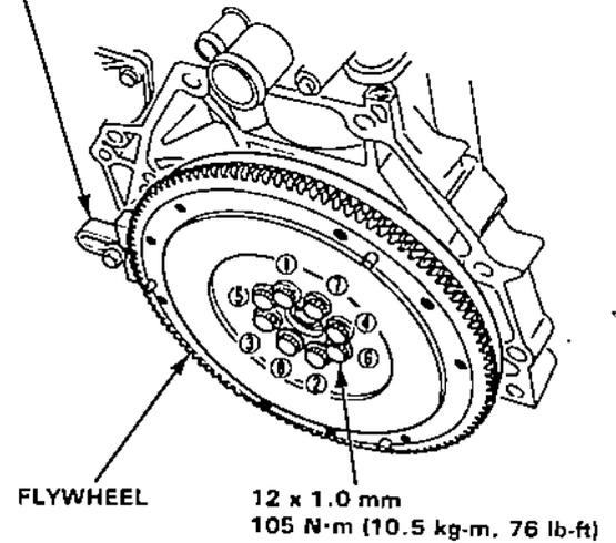
3. Install the clutch disc and pressure plate by aligning the flywheel dowels with dowel holes in the pressure plate.
