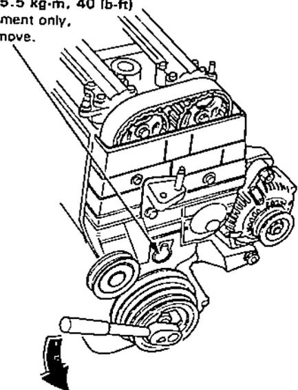
5. Rotate the crankshaft counterclockwise 3-teeth on the crankshaft pulley to create tension on the timing belt.
