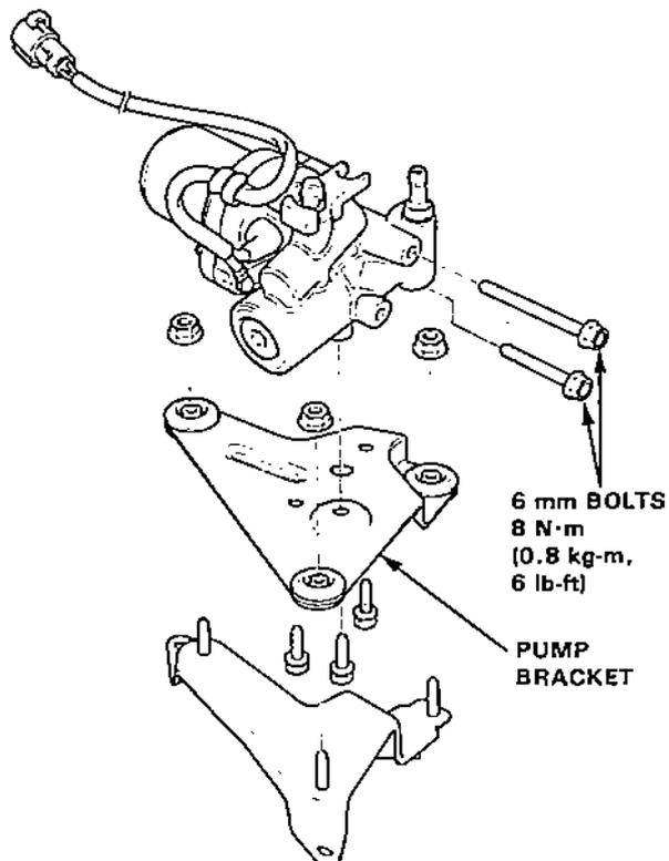
3. Separate the motor from the pump while rotating the pump right and left.
