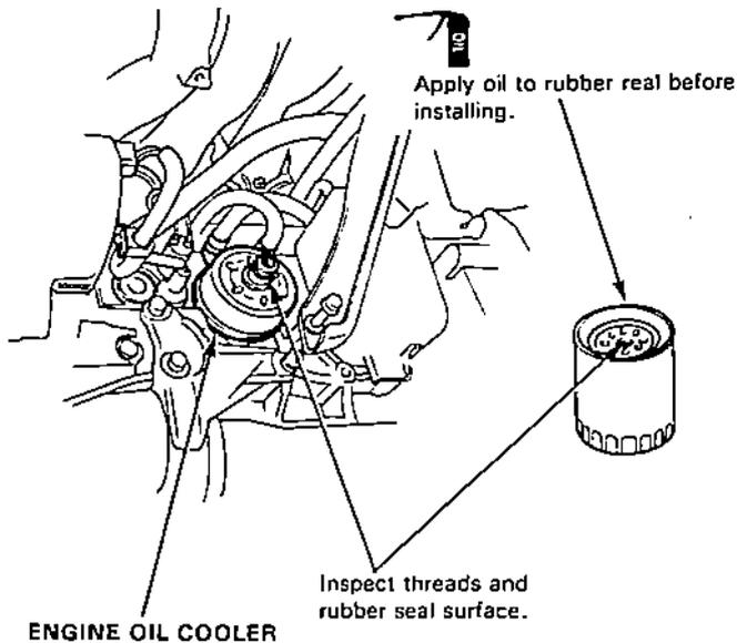
3. Install the oil filter by hand.
