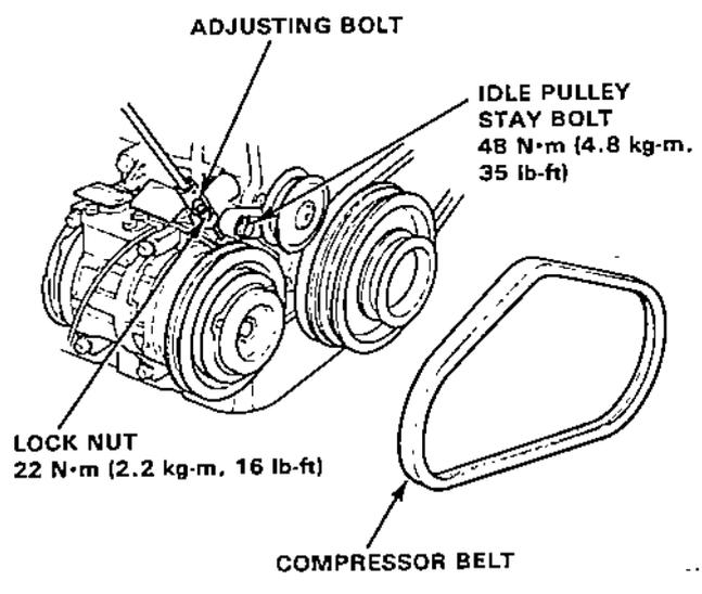
6. Remove the compressor mounting bolts (4) and compressor. Rest the compressor on the front beam.
