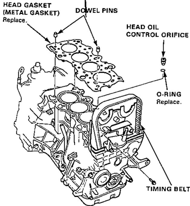
2. Tighten cylinder head bolts in two steps. In the first step tighten all bolts, in sequence, to about 30 N·m (3.0 kg-m, 22 lb-ft); in the final step tighten, in same sequence, to 85 N·m (8.5 kg-m, 61 lb-ft)
