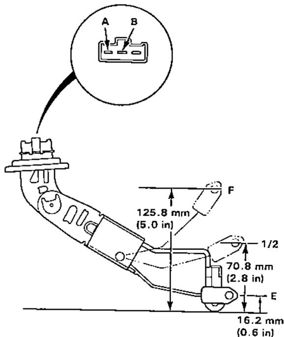
5. If unable to obtain the above readings, replace the fuel gauge sending unit.
