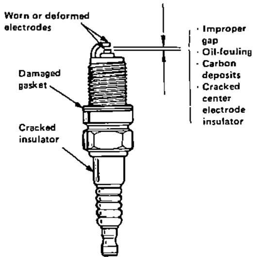
Burned or worn electrodes may be caused by:
