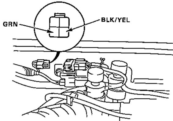
Is there battery voltage? **NO** → Repair in BLK/YEL wire between No. 14 fuse and 4P connector.
