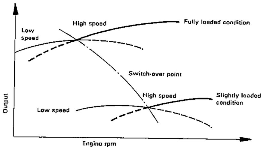
The above graph shows changes in the switch-over point in relation to engine rpm and load.
