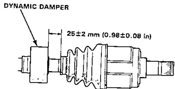
12. Install new boot bands on the boot and bend both sets of locking tabs.
