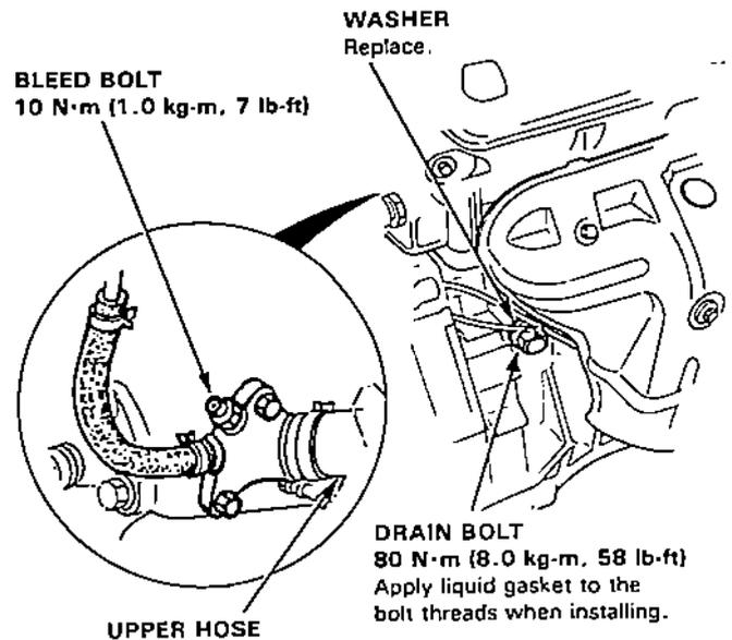
10. With the radiator cap off, start the engine and let it run until warmed up (fan goes on at least twice). Then, if necessary, add more coolant mix to bring the level back up to the bottom of the filler neck.
