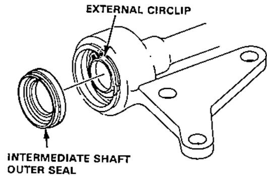
3. Remove the intermediate shaft.
