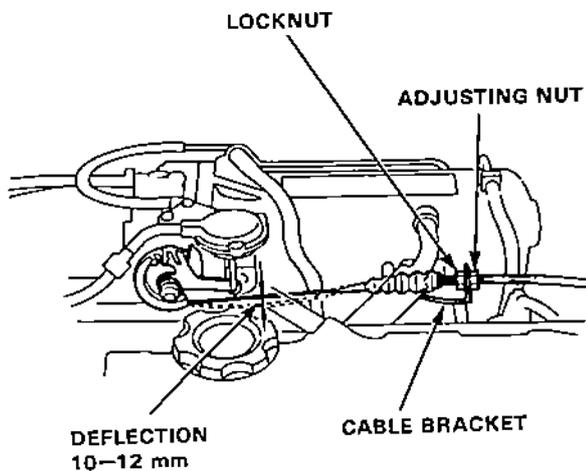
4. If deflection is not within specs, loosen the locknut and turn the adjusting nut until the deflection is as specified.
