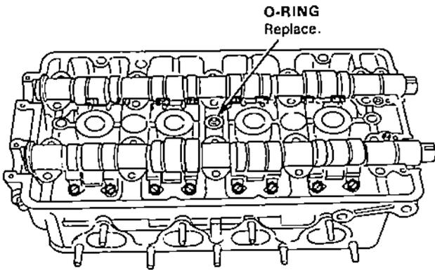
6. Apply liquid gasket to the head mating surfaces of the No.1 and No.5 camshaft holders, then install them, along with the No.2, 3 and 4.
