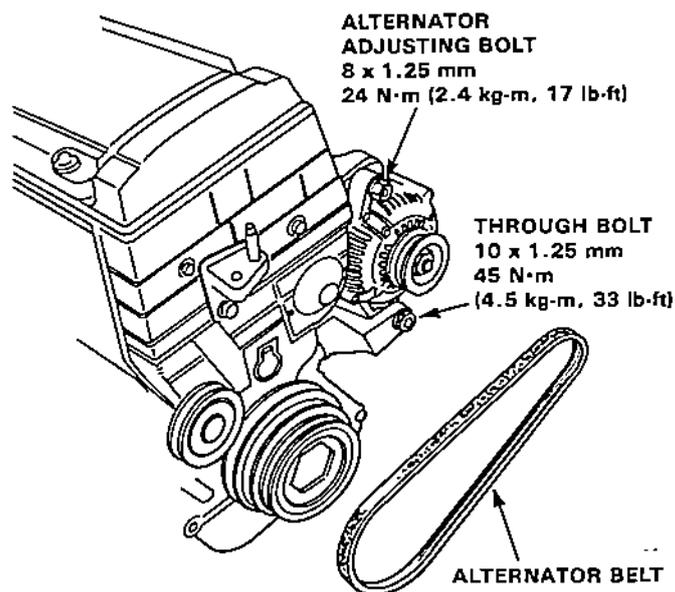
4. After installation, adjust the tension of each belt.
