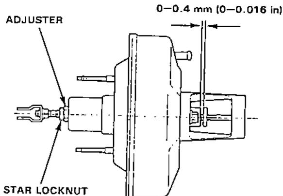
NOTE: If the clearance between the gauge body and adjusting nut is 0 mm, the pushrod-to-piston clearance is 0.4 mm. If the clearance between the gauge body and adjusting nut is 0.4 mm, the pushrod-to-piston clearance is 0 mm.
