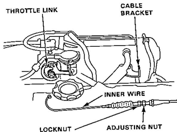
3. Hold the cable sheath, removing all slack from the cable.
