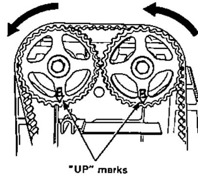
8. Rotate the crankshaft 180° counterclockwise to bring No.2 piston TDC. The "UP" mark should be on the intake side. Adjust valves on No.2 cylinder.
