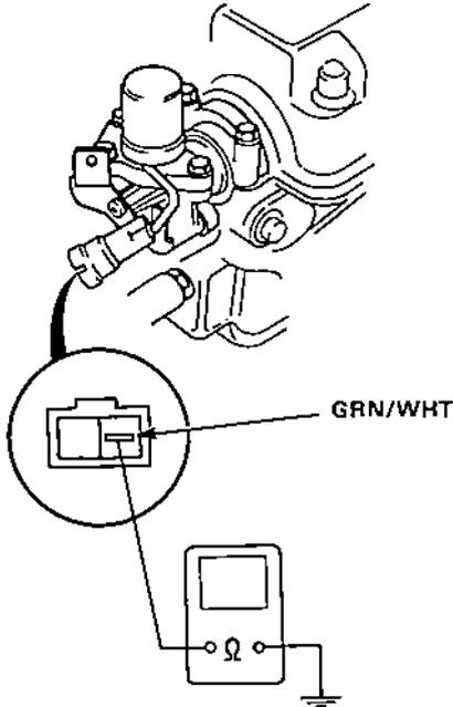
3. If the resistance is within specifications, remove the spool valve assembly from the cylinder head, and check the spool valve filter for clogging.
