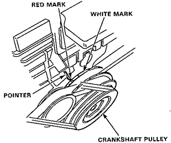
5. Adjust as necessary by loosening the distributor adjusting bolts, and turn the distributor housing counter clockwise to advance the timing, or clockwise to retard the timing.
