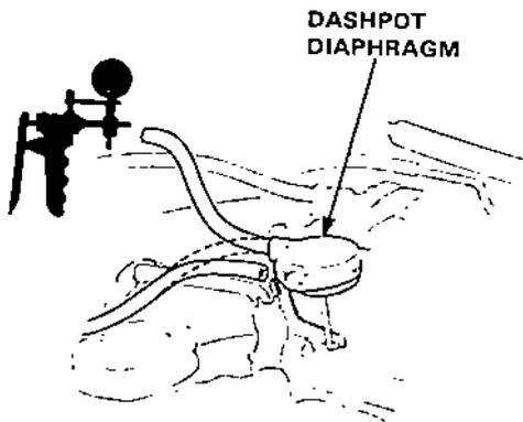
4. Apply the vacuum and check that the rod pulls in and vacuum holds.
