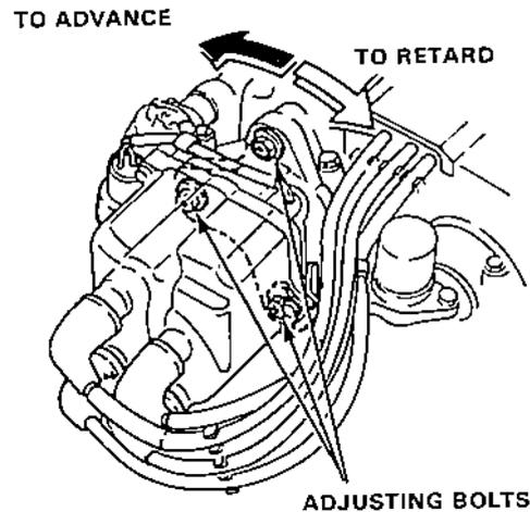
6. Tighten the adjusting bolts recheck the timing.
