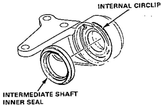
6. Press the intermediate shaft bearing out of the bearing support.
