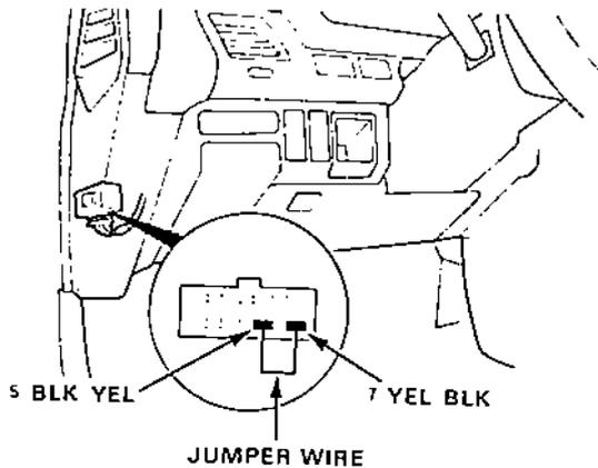
4. Check that battery voltage is available at the fuel pump connector when the ignition switch is turned ON (positive probe to the YEL/BLK wire, negative probe to the BLK wire).
