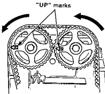
7. Rotate the crankshaft 180° counterclockwise to bring No. 4 piston to TDC. Both TDC grooves are once again visible. Adjust valves on No.4 cylinder.
