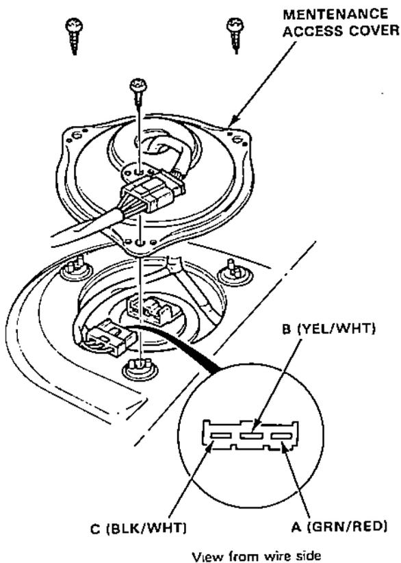
3. Connect the voltmeter positive probe to the B (YEL/WHT) terminal and the negative probe to the C (BLK/WHT) terminal. Then turn the ignition switch ON. There should be between 5 and 8 V.
