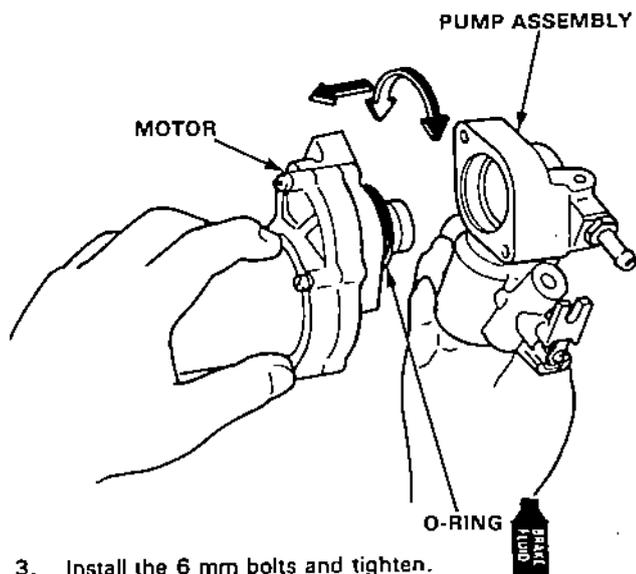
3. Install the 6 mm bolts and tighten.
