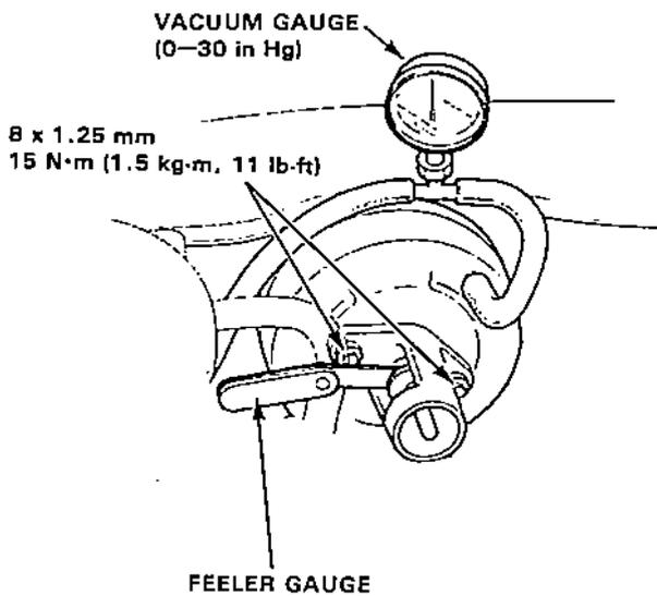
7. If clearance is incorrect, loosen the star locknut and turn the adjuster in or out to adjust. Hold the clevis while adjusting.
