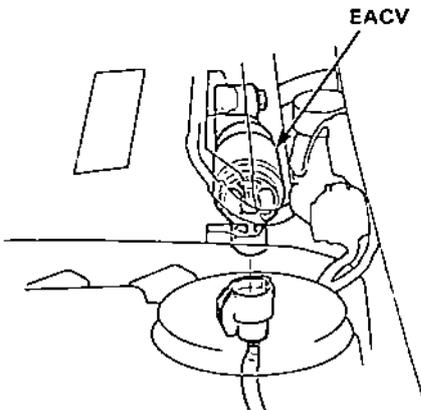
4. Check idling in no-load conditions in which the headlights, blower fan, rear defogger, cooling fan, and air conditioner are not operating.
