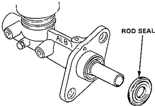
2. Push the secondary piston assembly, then remove the snap ring.
