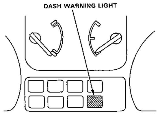
2. If you receive a customer's report that the dash warning light, sometimes comes on, check the system using the ALB checker to confirm whether there is any trouble in the system.
