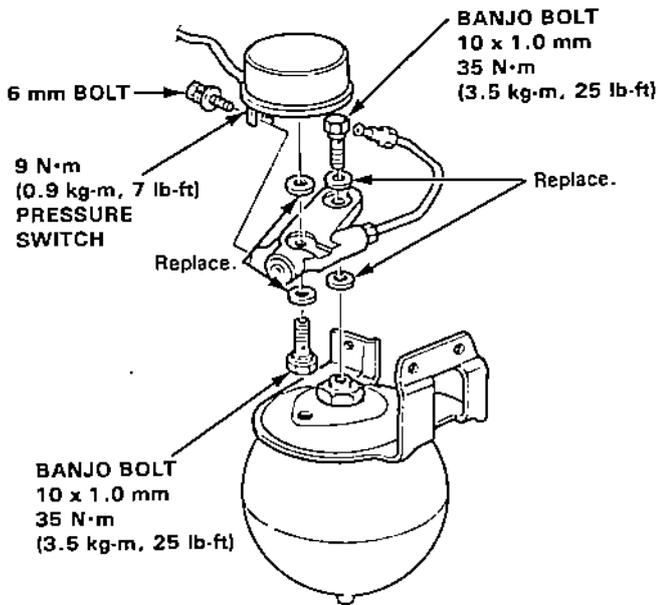
3. Remove the accumulator nut as shown.
