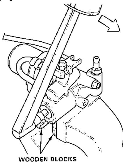
NOTE: Clamp the pump in a vise only as shown above.
