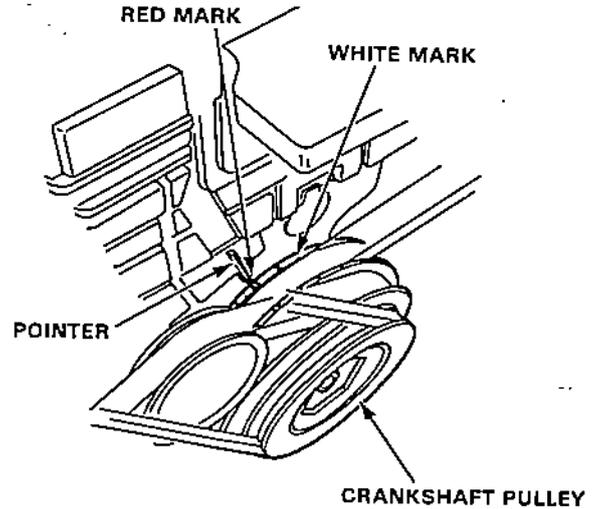
5. Adjust as necessary by loosening the distributor adjusting bolts, and turn the distributor housing counter clockwise to advance the timing, or clockwise to retard the timing.
