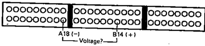
Does the voltage decrease when headlights and rear defogger are turned on?
