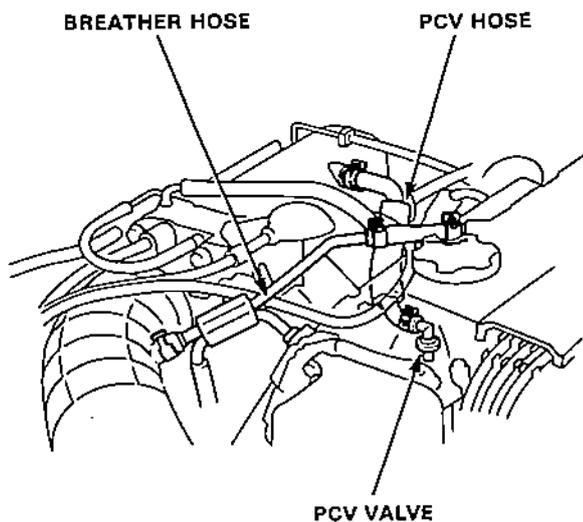
2. At idle, make sure there is a clicking sound from the PCV valve when the hose between PCV valve and intake manifold is lightly pinched with your fingers or pliers.
