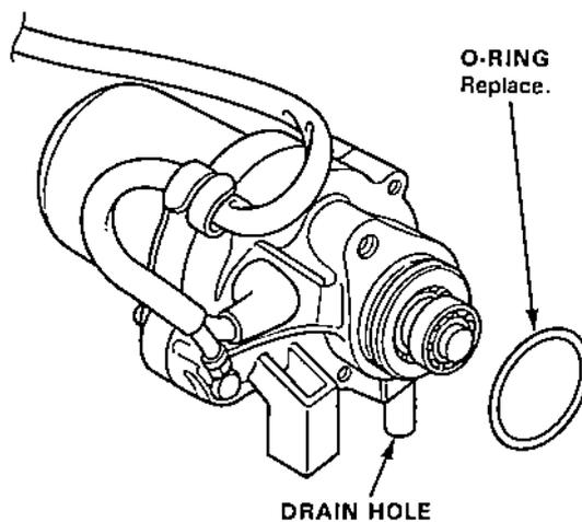
NOTE: Do not wash or dip the motor in brake fluid. Also be careful not to allow oil or water to enter the inside through the water drain hole.
