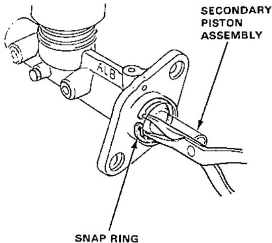
CAUTION: Avoid damaging the sliding surface of the secondary piston when installing the snap ring.
