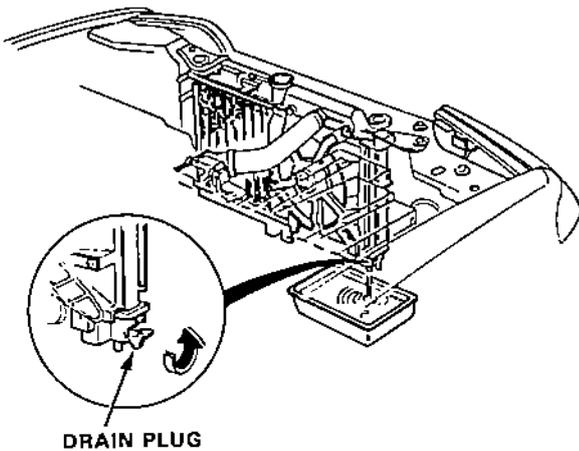
5. Apply liquid gasket to the drain bolt threads, then reinstall the bolt with a new washer and tighten it securely.
