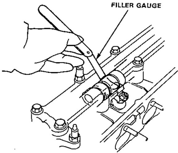
6. Rotate the crankshaft 180° counterclockwise (cam pulley turns 90°). The "UP" mark should be on the exhaust side. Adjust valve on No.3 cylinder.
