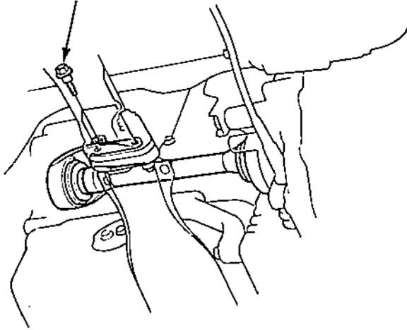
3. Lower the bearing support close to the steering gear-box and remove the intermediate shaft from the differential.
