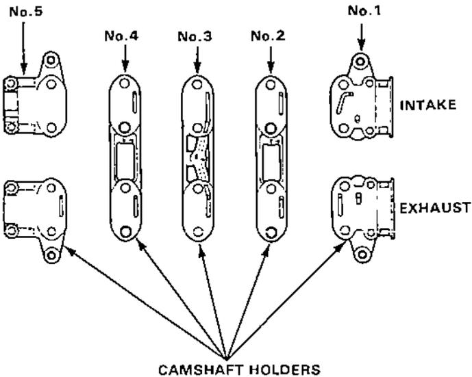
7. Set the camshaft folders and camshaft holder pipes, then tighten temporarily the bolts.
