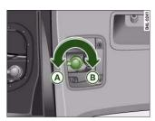
Fig. 287 Diagram: Bulb holder with a bayonet fastener
