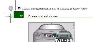
Fig. 46 Release catch on the boot lid
