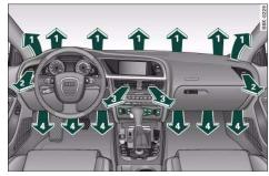
Fig. 110 Dashboard: Location of air outlets
