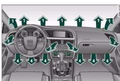
Fig. 119 Dashboard: Location of air outlets
