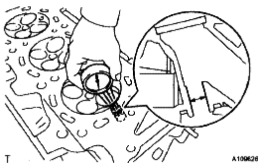
Fig. 392: Checking Bush Bore Diameter Of Cylinder Head Courtesy of TOYOTA MOTOR SALES, U.S.A., INC.
