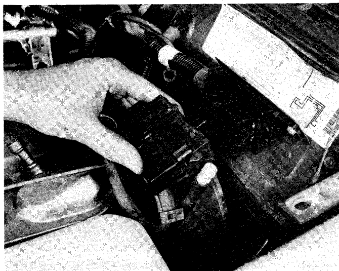
5.56 Remove the attaching screw and unplug the firewall electrical connector
