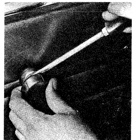
12.3 Pry off the crank handle
