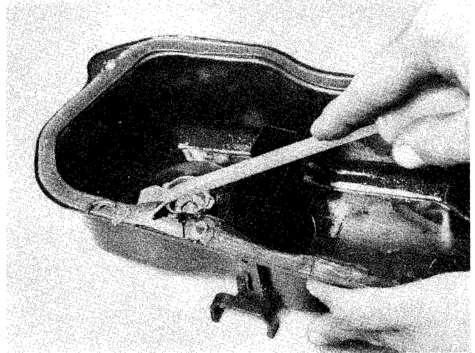
4.6 Remove the old sealant from the rocker arm cover flange and the cylinder head with a gasket scraper, then clean the mating surfaces with lacquer thinner or acetone
