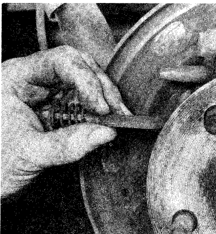
6.4j Remove the parking brake link
