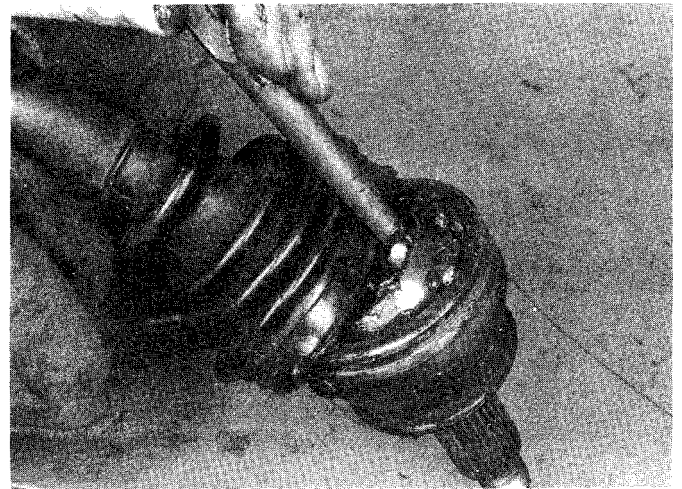
16.11b Dislodge the CV joint assembly with a brass punch and hammer (be careful not to let the joint fall!)
