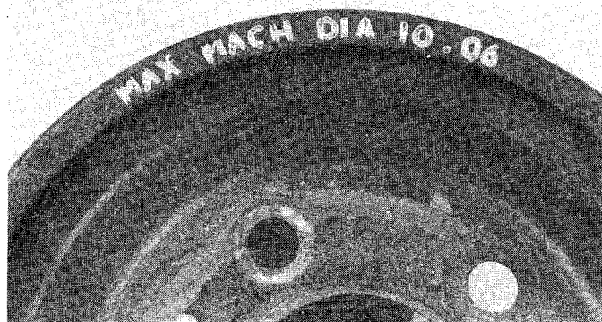
6.5 The maximum allowable drum diameter is cast into the drum
