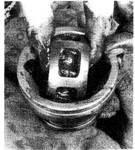
16.13 Tilt the inner race and cage 90-degrees, then align the windows in the cage with the lands and rotate the inner race up and out of the outer race
