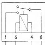
A relay is effectively an electromagnetic switch. To close the relay contacts and complete the circuit, an electromagnet in the relay is energised which causes the relay contacts to close, making the circuit complete.
