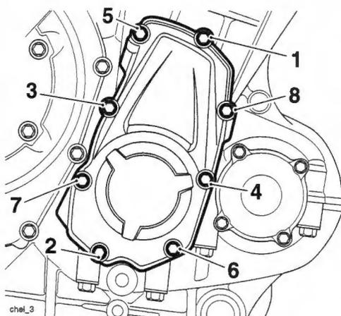
**Crankshaft Cover Tightening Sequence**
