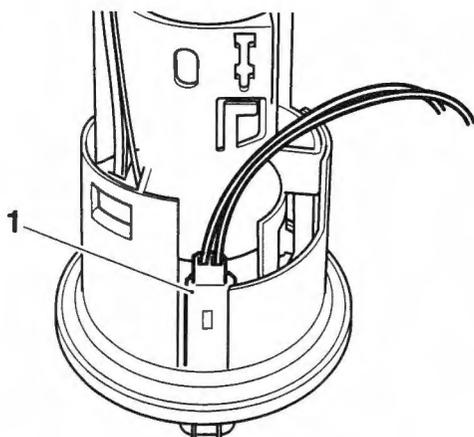
**1. Fuel level sensor electrical connector**
