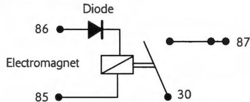
Make continuity checks across the electromagnet first, usually from pin 86 (positive) to pin 85 (negative). If a diode appears in the circuit use the diode check on the multimeter (Volts scale) in the direction of current flow. If there is no diode, use the resistance check facility. An open circuit or unusually high resistance value indicates a faulty relay.
