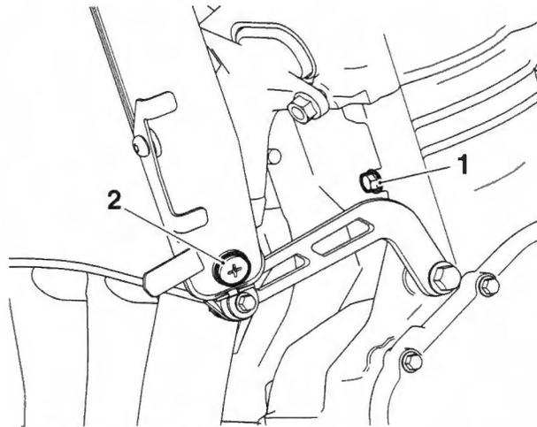
1. Crankcase coolant drain screw
