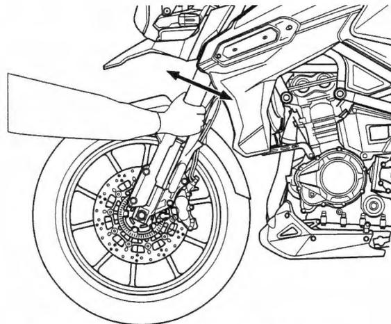
**Checking Headstock Bearing Adjustment**
