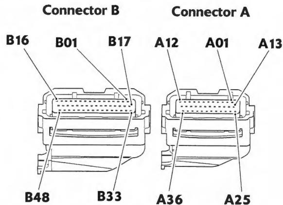
The above illustration shows the pin numbering system used in the engine management circuit diagram.
