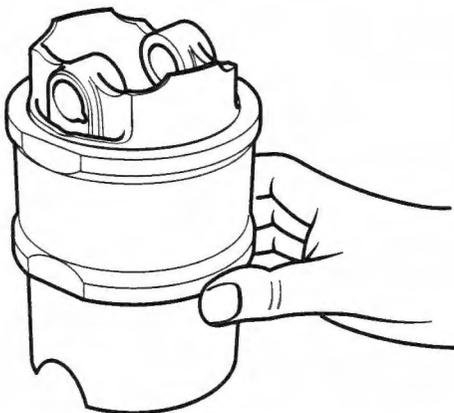
Aligning Piston Rings using the Piston
