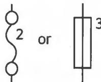
A fuse is a device which protects a circuit in the event of a fault. The fuse will 'blow' if a short circuit occurs, protecting that circuit from further damage. The number next to the fuse on the circuit diagram indicates the position of the fuse in the fusebox.
