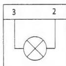
This symbol is used to show all types of light bulbs. The numbers in the box relate to the terminal numbers of the connector pins. An additional number outside the box will identify the component.
