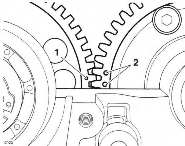
1. Balancer drive gear markings
