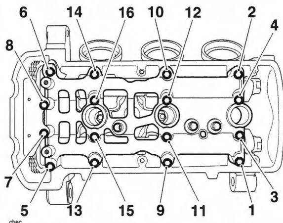
**Camshaft Ladder Bolt Release Sequence**
