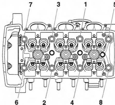
Cylinder Head Bolt Tightening Sequence
