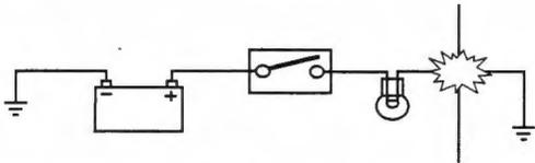
A 'short cut' in an electrical circuit - current by-passes the intended circuit, either to earth or to another, different circuit. Often caused by failure of the cable insulation due to chafing or trapping of the wire. There are two different types of short circuit - short to ground and short to Vbatt.
