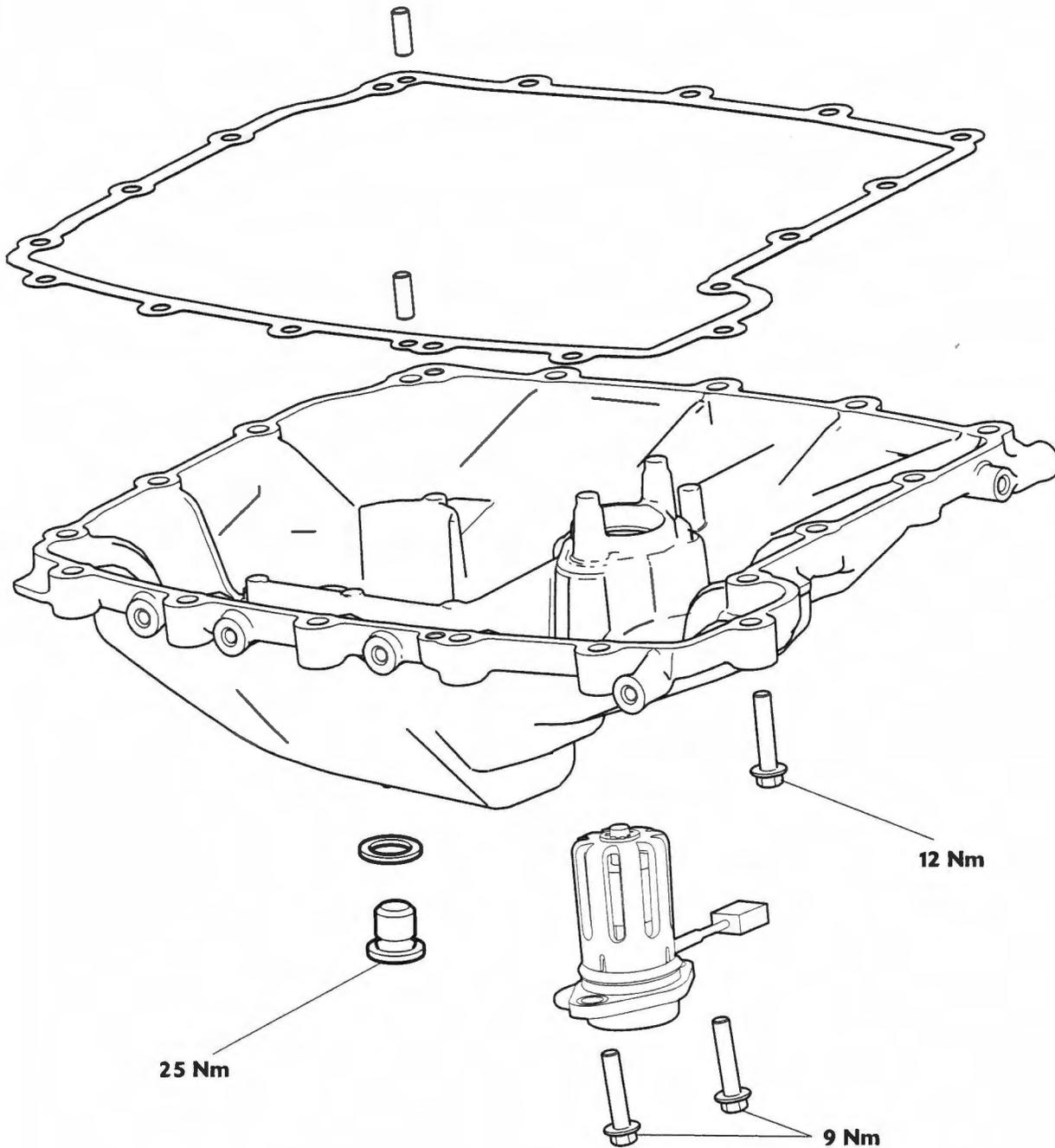
Exploded View - Lubrication System
