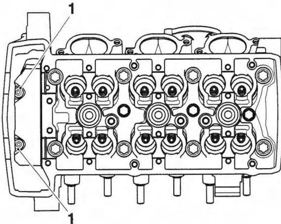
**1. Cylinder head to upper crankcase screws**
