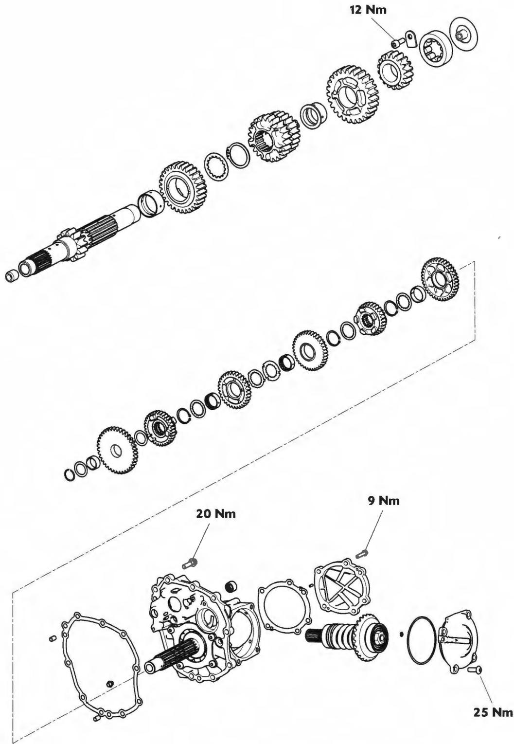
Exploded View - Flywheel, Sprag Clutch and Starter Gears
