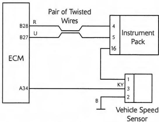
**Extract from the Circuit Diagram Showing CAN Connection Between ECMs**
