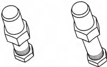
Alternator/Flywheel Rotor Puller T3880365
