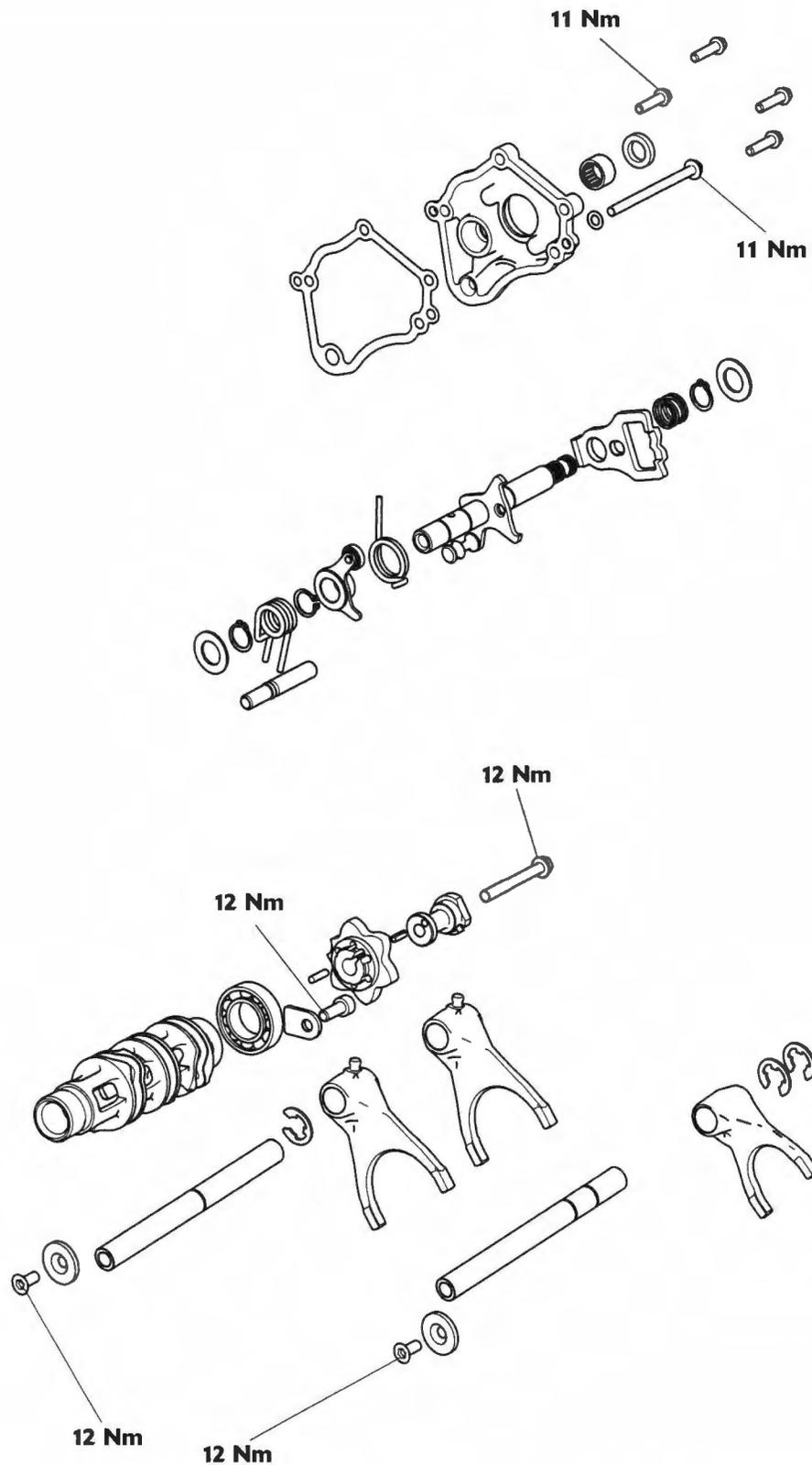
Exploded View - Gear Change Mechanism
