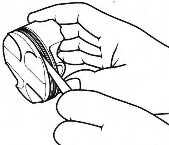
Piston Ring to Ring Groove Clearance Check
