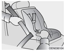
Remove as much slack from the belt as possible by pushing down on the child restraint system while feeding the shoulder belt back into the retractor.
