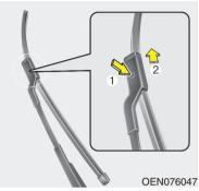
2. Press the button and slide the blade assembly upward.
