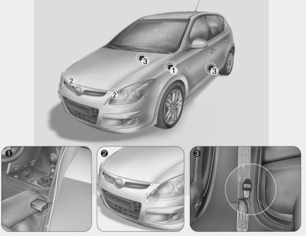
Air bag collision sensors (1) SRS control module (2) Front impact sensor OFD037023/OFD037021/OFD037022/OHD036030
