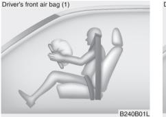
The front air bag modules are located both in the center of the steering wheel and in the front passenger's panel above the glove box. When the SRSCM detects a sufficiently severe impact to the front of the vehicle, it will automatically deploy the front air bags.
