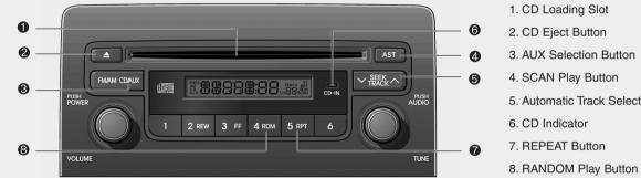
2. CD Eject Button 3. AUX Selection Button 4. SCAN Play Button 5. Automatic Track Selection Button 6. CD Indicator 7. REPEAT Button
