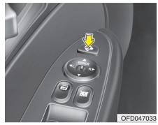
Electric type (if equipped) To fold the outside rearview mirror, depress the button.
