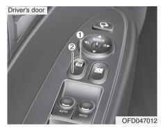
D050202AUN With central door lock switch Operate by depressing the central door lock switch.
