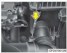
After the transaxle is warmed up sufficiently (fluid temperature 158~176°F (70~80°C), for example by 10 minutes usual driving, move the shift lever through all positions then place the selector lever in "N (Neutral) or P (Park)" position.
