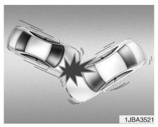
In an angular collision, the force of impact may direct the occupants in a direction where the air bags would not provide additional occupant protection, and thus the sensors may not deploy any air bags.
