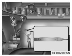
4. Pull the dipstick out, wipe it clean, and re-insert it fully.
