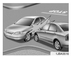
• Front air bags are not designed to inflate in side impact collisions, because frontal air bag deployment would not provide additional occupant protection.
