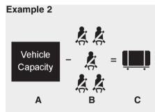
Description Total Item Vehicle Capacity 1400 lbs А Weight (635 kg) Subtract Occupant 750 lbs В Weight (340 kg) 150 lbs (68 kg) × 5 Available Cargo and 650 lbs С Luggage weight (295 kg)
