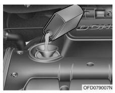
If it is near or at L, add enough oil to bring the level to F. **Do not overfill.**
