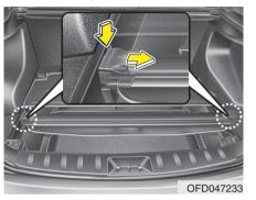
When not in use, place the cargo security screen on the lower portion of the cargo area.
