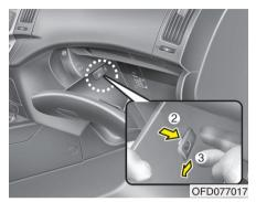
2. With the glove box open, remove the stoppers on both sides to allow the glove box hang freely on the hinges.
