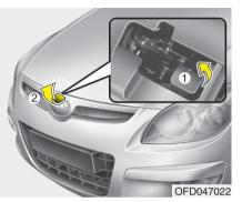
Go to the front of the vehicle, raise the hood slightly, pull the secondary latch (1) inside of the hood center and lift the hood (2).
