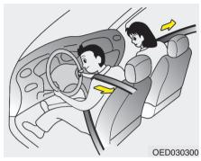
When the vehicle stops suddenly, or if the occupant tries to lean forward too quickly, the seat belt retractor will lock into position. In certain frontal collisions, the pre-tensioner will activate and pull the seat belt into tighter contact against the occupant's body.
