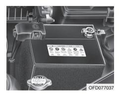
A WARNING - Radiator cap Do not remove the radiator cap when the engine and radiator are hot. Scalding hot coolant and steam may blow out under pressure causing serious injury.
