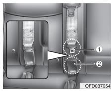
Insert the metal tab (1) into the open end of the anchor connector (2) until an audible "click" is heard, indicating the latch is locked. Make sure the belt is not twisted.
