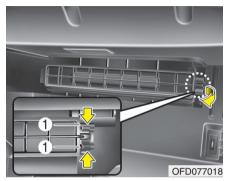
3. Remove the climate control air filter case pulling out the cover.
