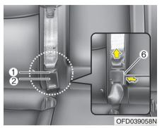
3. If necessary, disconnect the metal tab (1) from the anchor connector (2) by inserting a key or similar small rigid device into the release button (6) on the anchor connector (2) and allow the webbing to draw back automatically into the retractor.
