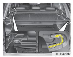
• To use the cargo security screen, pull the handle backward and insert the edges into the slots.
