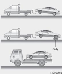
It is acceptable to tow the vehicle with the rear wheels on the ground (without dollies) and the front wheels off the ground. If any of the loaded wheels or suspension components are damaged or the vehicle is being towed with the front wheels on the ground, use a towing dolly under the front wheels.
