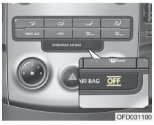
If the front passenger seat is occupied by a person that the system determines to be of adult size, and he/she sits properly (sitting upright with the seatback in an upright position, centered on the seat cushion with their seat belt on, legs comfortably extended and their feet on the floor), the "PASSENGER AIR BAG OFF" or "PASS AIR BAG OFF" indicator will be turned off and the front passenger's air bag will be able to inflate, if necessary, in frontal crashes.
