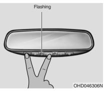
When programming the buttons for the first time, press and hold the left and center buttons (①, ①) simultaneously until the indicator light begins to flash after approximately 20 seconds. (This procedure erases the factory-set default codes. Do not perform this step to program additional hand-held transmitters.)
