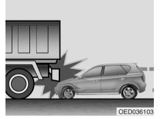
· Frontal Air Bags may not inflate in "under-ride" collisions where the collisions energy is absorbed above the vehicle's front bumper.
