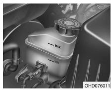
G080100AFD Checking the brake/clutch fluid level
