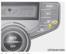
**Defrost-level (A, D)** Most of the air flow is directed to the windshield with a small amount of air directed to the side window defrosters.
