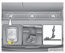
C030103AFD Securing a child restraint seat with tether anchor system Child restraint hook holders are located on the floor behind the rear seats.
