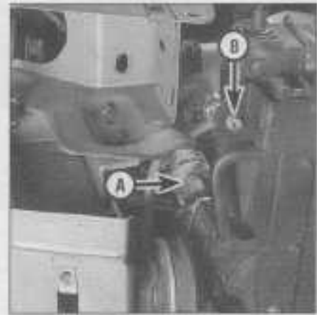
15.5 Using the appropriate quick-connect coupling tool, disconnect the air conditioner condenser lines (A) from the condenser and remove the mounting bolts (B)
