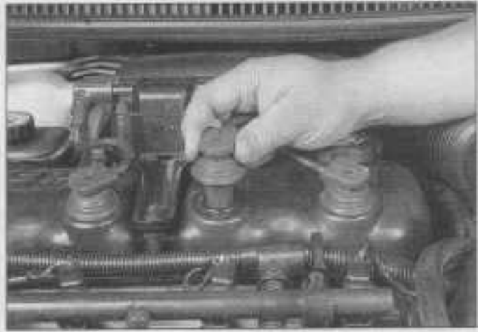
27.7b Use a twisting motion to free the boot and then pull it from the valve cover
