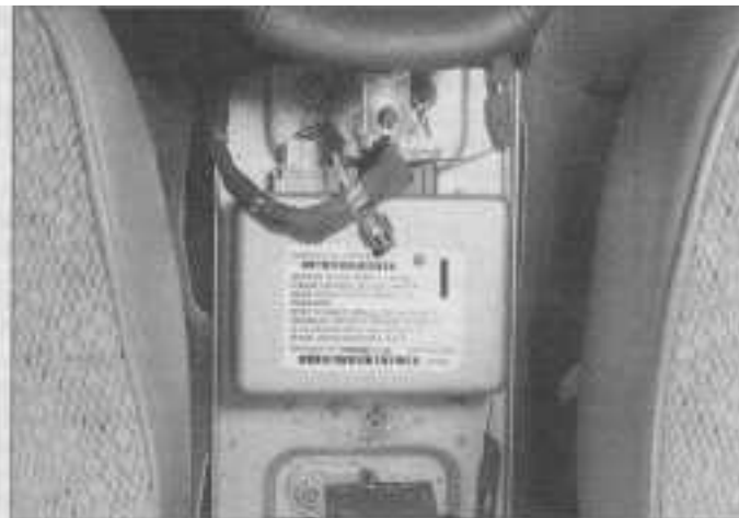
29.1c The Airbag Control Module is located under the center console and mounted to the floorpan
