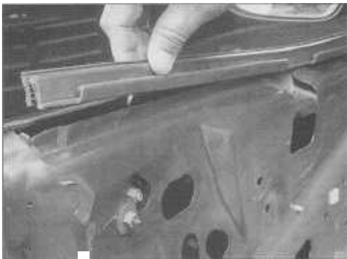
15.3 Remove the inner belt weatherstrip from the door window sill
