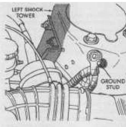
1.4b . . . then detach the cable and push the hole in the cable insulator over the stud
