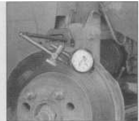
5.3 Use a dial indicator to check disc runout - if the reading exceeds the specified runout limit, the disc will have to be machined or replaced
