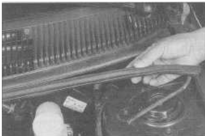
28.2 Carefully remove the hood rubber sealing strip from the edge of the cowl cover
