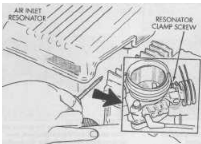
9.2 Four-cylinder engines - air inlet resonator clamp at the throttle body
