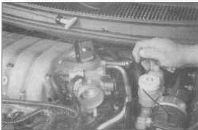
4.6 Remove the EGR tube
