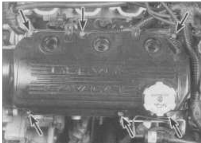
3.6 Valve cover mounting bolts (arrows)
