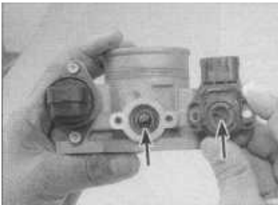
3.85 When installing the TPS onto the throttle body, make sure the socket tangs are on the proper side of the throttle valve shaft blade (arrows). When installed correctly, the TPS must be rotated slightly clockwise to align the screw holes
