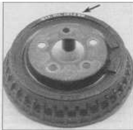
6.5 The maximum allowable diameter is stamped into the drum (arrow)
