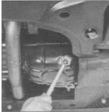
8.8 To avoid rounding off the corners, use the correct size box-end wrench or a socket to remove the engine oil drain plug
