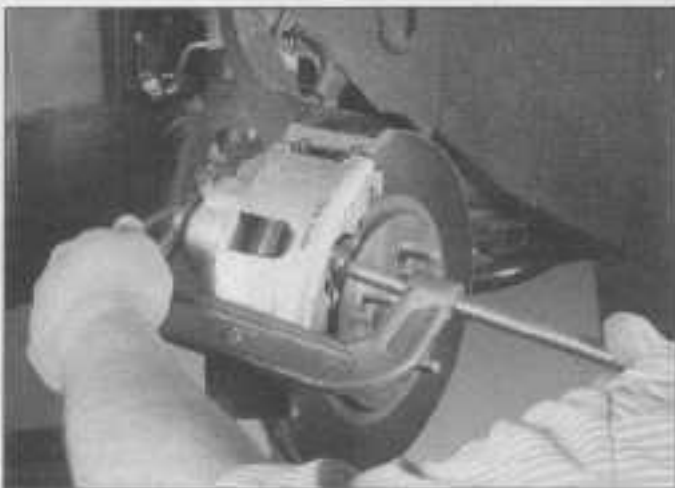
3.3 Use a C-clamp to press the caliper piston into its bore
