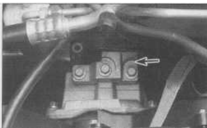
17.9d Right-side engine mount (arrow)
