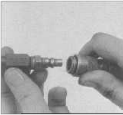
11.4 This is what the air hose adapter that threads into the spark plug hole looks like - they're usually available from auto parts stores
