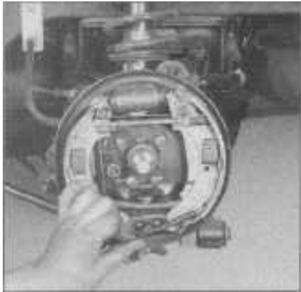
6.4b Remove the lower return spring - note that the shorter spring end is towards the trailing brake shoe
