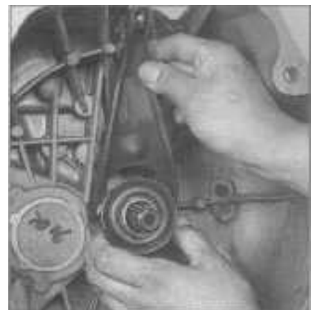
5.4 Removing the release bearing and lever
