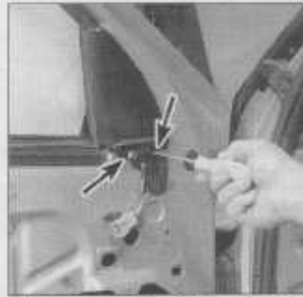
27.4a Remove the exterior mirror bezel mounting screws (arrows) ...
