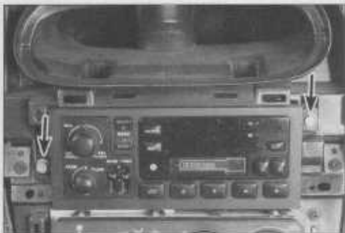
17.3 Radio mounting screws (arrows)
