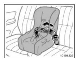
While pressing the convertible seat firmly against the seat cushion and seatback, tighten the lap belt by pulling its free end to hold the convertible seat securely.
