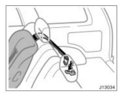
If your child restraint system requires the use of a top strap, latch the hook onto the anchor bracket and tighten the top strap.
