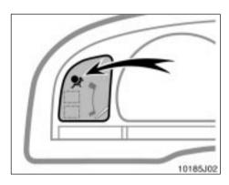
This indicator comes on when the ignition key is turned to the "ACC" or "ON" position. It goes off after about 6 seconds. This means the SRS airbags are operating properly.
