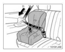
Fully extend the shoulder belt to put it in the lock mode. When the belt is then retracted slightly, it cannot be extended.
