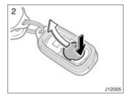
2. Remove the discharged transmitter battery.
