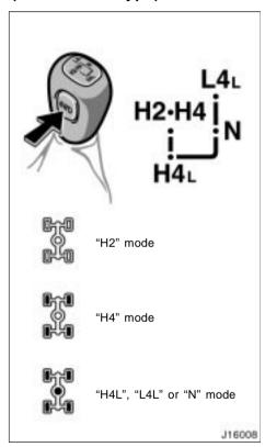
Use the front drive control lever and "4WD" button to select the transfer and center differential modes.
