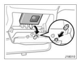
Remove spacers from the box. Place the largest spacer on the pin that would be below transmitter button when the cover is closed. Close the cover.
