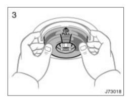
3. Install the rubber cover with the "TOP" mark upward, and snuggle on the boss. Insert the connector.
