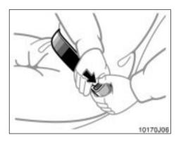
To release the belt, press the buckle-release button.
