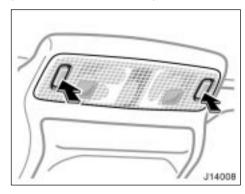
To turn on the personal light, push the switch. To turn the lights off, push the switch once again.
