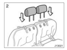
Store the head restraints in the head restraint retaining holes in the bottom cushion.
