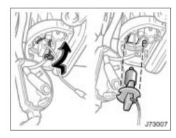
3. Release the bulb retaining spring and remove the bulb. Install a new bulb and the bulb retaining spring.
