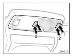
To turn on the personal light, push the switch on 1 side. To turn the light off, push the switch on 2 side.
