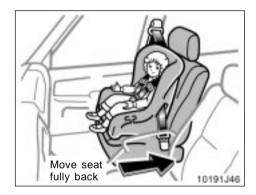
A forward-facing child restraint system should be allowed to be put on the front seat only when it is unavoidable. Always move the seat as far back as possible, because the force of a deploying airbag could cause death or serious injury to the child.
