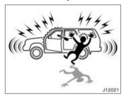
To deter the vehicle theft, the system is designed to give an alarm if any of the side doors, back door or hood is forcibly unlocked or opened or the battery terminal is disconnected and then reconnected when the vehicle is locked.
