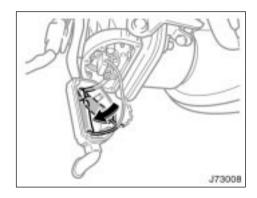
4. Connect the cord and put the soft casing into the cover.
