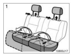
1. Swing the bottom cushion up by pulling the lock release strap, and remove the head restraint.
