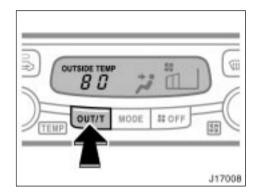
The thermometer indicates the outside air temperature when you push the "OUT/T" button.
