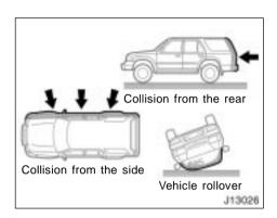
The SRS airbags are not designed to inflate if the vehicle is involved in a side or rear collision, if it rolls over, or if it is involved in a low-speed frontal collision.
