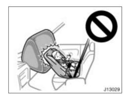
Never put a rear-facing child restraint system in the front seat because the force of the rapid inflation of the passenger airbag can cause death or serious injury to the child.
