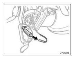
2. Lift up the soft casing and disconnect the cords.
