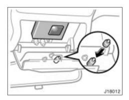
If the spacer does not contact with your garage door opener transmitter:
