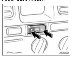
The back window can be operated with the inner switch on the center console or outer switch on the back door.
