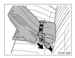
Run the center lap belt through or around the infant seat following the instructions provided by its manufacturer and insert the tab into the buckle taking care not to twist the lap belt.
