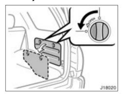
To open the box, turn the two knobs.
