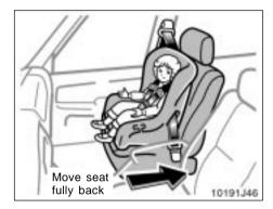
• A forward-facing child restraint system should be allowed to be put on the front seat only when it is unavoidable. Always move the seat as far back as possible, because the force of a deploying airbag could cause death or serious injury to the child. For instructions concerning the installation of a child restraint system, see "Child restraint" in this section.
