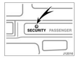
The system is automatically set when the key is removed from the ignition switch. The indicator light will start flashing every 2 seconds to show the system is set.
