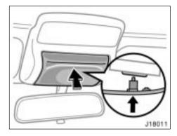
When the garage door opener transmitter is properly installed, you can operate the transmitter by pushing the cover.
