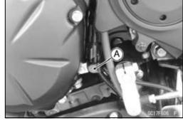
Disconnect the oxygen sensor lead connector and connect the measuring adapter [A] between these connectors.
