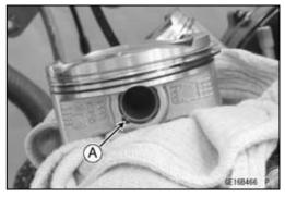
Remove the piston pins with the piston pin puller [A].
