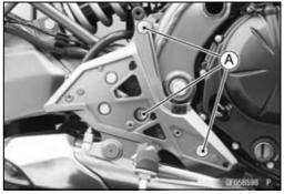
Remove: Clutch Cover Bolts [A]
