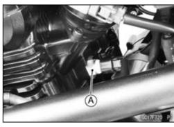
Subthrottle Sensor [A] Main Throttle Sensor [B] Subthrottle Valve Actuator [C]
