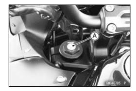
OThe spring preload can be left soft for average riding. But it should be adjusted harder for high speed riding or riding with a passenger. If the spring action feels too soft or too stiff, adjust it in accordance with the following table.
