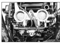
Air Switching Valve [A] Stick Coils #1, #2 [B]
