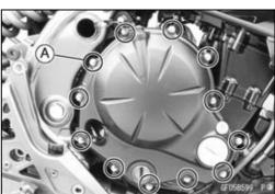
Turn the release lever [A] toward the rear as shown, and remove the clutch cover [B].
