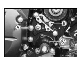
• Remove the shift shaft assembly [A].
