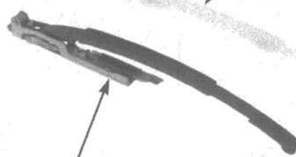
CAM CHAIN TENSIONER
