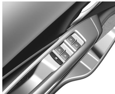
Pulse el interruptor
