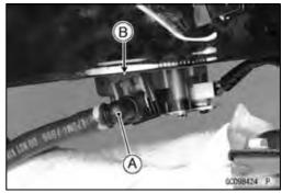
Push and pull [A] the hose joint [B] back and forth more than two times, and make sure it is locked and does not come off.
