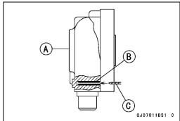
Drill the housing from the outside to the pin end [A] using a 3.0 ~ 3.5 mm (0.12 ~ 0.14 in.) drill bit [B].
