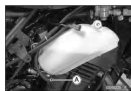
• Fill the radiator up to the filler neck [A] with coolant.
