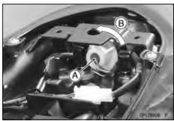
Push the bulb [A] in the socket, turn it counterclockwise
