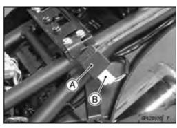
Connect one 12 V battery and turn signal lights as indicated in the figure, and count how may times the lights flash for one minute.
