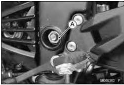
• Pull out the pivot shaft [A] and remove the swingarm [B].
