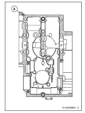
Apply molybdenum disulfide oil solution to the seating surface [A] and threads [B] of the M8 bolts.
