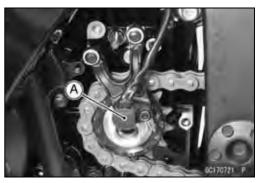
Water Temperature Sensor [A] Vehicle-down Sensor [B]
