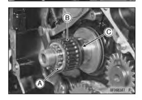
• Install the clutch housing, spacer, clutch hub, washer and clutch hub nut.
