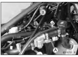
Inlet Air Temperature Sensor [A]
