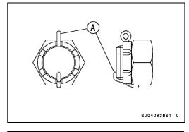
• Install the speedometer cable so that the drive notch [A] of it fits into the projection [B] of the speedometer pinion in the housing.
