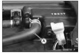
Connect a vacuum gauge (special tool) and hoses [A] to the fittings on the throttle body.
