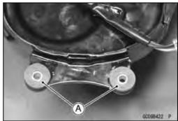
• Pull the joint lock [A] as shown in the figure.
