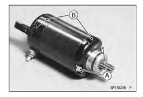
Remove the terminal locknut [A], washer and insulators, and then remove the brushes and terminal bolt [B] with the brush plate [C] from the end cover.
