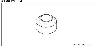
Valve Seat Cutter, 32° -  $\phi$ 25: 57001-1118
