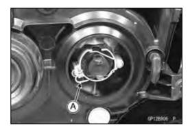
• Fit the dust cover [A] onto the bulb [B] firmly as shown in the figure.
