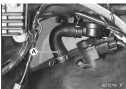
ODo not disconnect the air switching valve connector [A].
