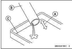
Hold the fork tube upright, pour in the type and amount of fork oil specified.
