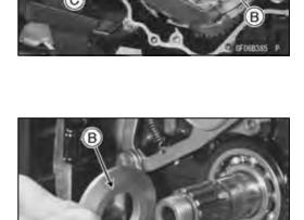
• Install the bushing [A] and needle bearing [B].
