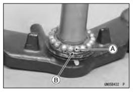
Apply grease to the upper ball bearings (19) [A] and outer race [B], and install the ball bearings onto the outer race.
