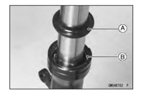
Use the fork outer tube weight [A] to separate the inner tube from the outer tube. Holding the inner tube by hand in a vertical position, pull down the outer tube several times to pull out the inner tube.
