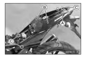
Remove the projections [A] from the holes [B], and pull out the center seat cover [C] forward.
