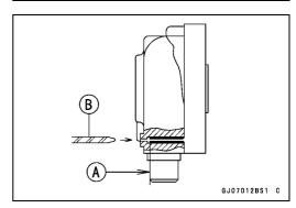
Using a 3 mm (0.12 in.) rod [A], tap out the pin [B], and then pull out the speedometer cable bushing and speedometer pinion.
