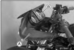
Remove: Bolts [A] Meter Unit [B]
