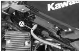
Open the fuel tank cap [A] to lower the pressure in the tank.
