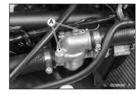
Move the thermostat cover [A] outwards and remove the thermostat [B].
