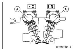
Using the thickness gauge [A], measure the valve clearance between the cam and the valve lifter.
