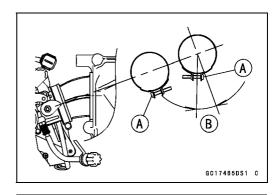
OInsert the duct portion [A] into the grommet [B]. OTighten:
