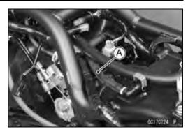
OTo maintain the correct fuel/air mixture (F/A), there must be no inlet air leaks in the DFI system. Be sure to install the oil filler plug [A] after filling the engine oil.
