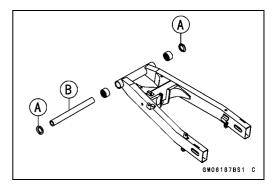
• Remove the needle bearings.
