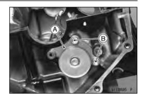
• Install the pin, spring, washer and, tighten the shift drum positioning bolt to the upper crankcase.
