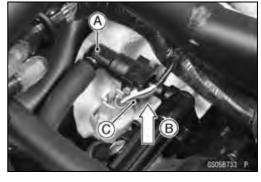
Push and pull [A] the fuel hose joint [B] back and forth more than two times, and make sure it is locked and does not come off.
