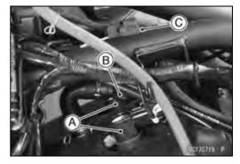
Subthrottle Valve Actuator [A]
