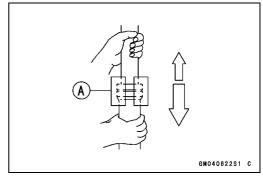
• Remove the inner guide bushing from the inner tube.
