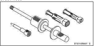
Steering Stem Bearing Driver Adapter,  $\phi$ 34.5: 57001-1074
