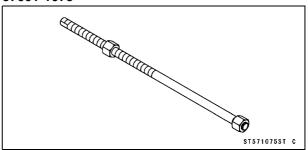
Head Pipe Outer Race Driver,  $\phi$ 51.5: 57001-1076
