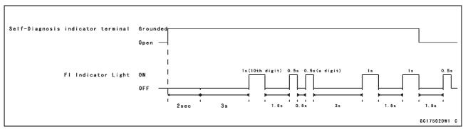
Olf the problem is with the following parts, the ECU cannot memorize these problems, the FI indicator light doesn't go on, and no service codes can be displayed.
