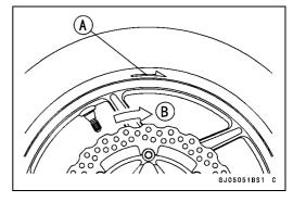
Position the tire on the rim so that the air valve [A] align with the tire balance mark [B] (the chalk mark made during removal, or the yellow paint mark on a new tire).
