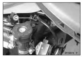
• Set the hand tester to the  $\times$  1  $\Omega$  range, and check the continuity as shown in the figure.
