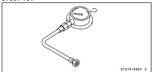
Oil Pressure Gauge Adapter, M18 x 1.5: 57001-1278
