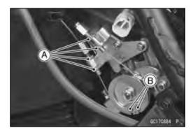
Remove: Bolts [A] Idle Adjusting Cable [B] (from Bracket)
