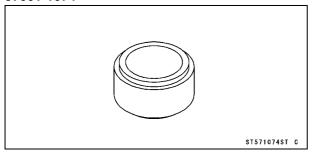
**Head Pipe Outer Race Press Shaft:** 57001-1075
