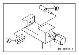
Turn the pin holder until the riveting pin touches the link pin.
