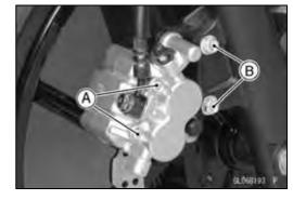
Remove: Pad Pins Brake Pads [A]
