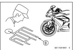
Even when the DFI system is operating normally, the FI indicator light [A] may light up under strong electrical interference. No remedy needed. Turn the ignition switch OFF to stop the indicator light.
