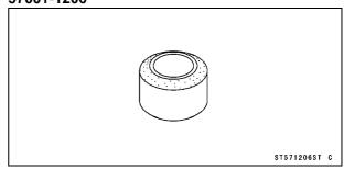
Valve Seat Cutter, 67.5° -  $\phi$ 22: 57001-1207
