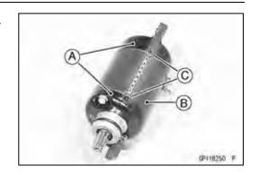
Replace the O-rings on the through bolts with new ones and tighten them.
