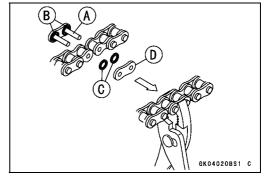
Set the plate holder (A) [A] and plate holder (B) [B] on the body.
