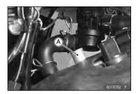
★ If the reading is out of the standard (with plug: DC 0.7 V or more, without plug: DC 0.2 V or less), remove the ECU and check the wiring for continuity between main harness connectors.
