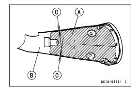
Insert the claw [A] into the cover clamp [B] and tighten the clamp screw [C] as shown in the figure.
