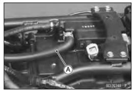
• Separate the hose [A] from the air suction valve cover.
