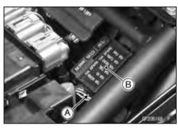
Pull the fuses [A] straight out of the fuse box with needle nose pliers.
