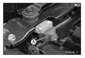
Pull out the main fuse [A] from the starter relay with a needle nose pliers.
