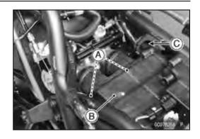
After removing the air cleaner housing, stuff pieces of lintfree, clean cloth into the throttle body assy.
