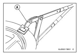
Step on the side of the tire opposite the valve stem and start prying the tire off the rim near the air valve with tire irons [A].
