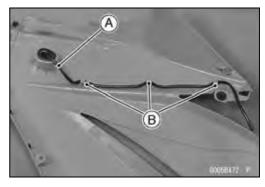
OFit [A] the front portion of the lower fairing in the rear portion of the upper fairing.
