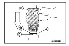
Apply molybdenum disulfide grease to the oil seal lips, and install the washer and the oil seal [A] into the outer tube.
