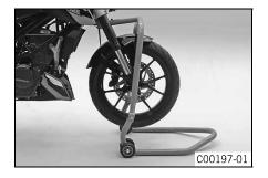
Move the handlebar to the straight-ahead position. Attach the lifting gear to the steering stem.
