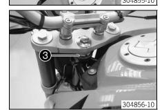
Tighten nut 9 with the special tool until there is no play in the steering head bearing.
