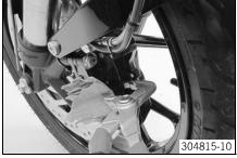
Press the brake piston back to its basic position and make sure that no brake fluid overflows from the brake fluid reservoir.
