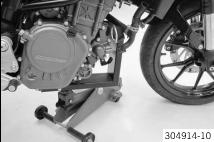
Position the floor jack under the engine and fix it using the special tool.
