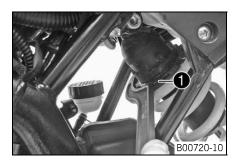
Turn adjusting ring • to adjust the spring preload.
