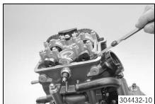
Check the valve clearance at all valves between the camshaft and cam lever.
