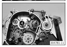
Mount timing chain sprocket 4.
