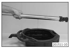
Unclamp the inner tube. Drain the oil.
