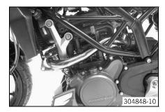
Remove the exhaust manifold toward the front.
