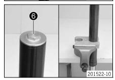
Mount screw cap 6 onto the piston rod.
