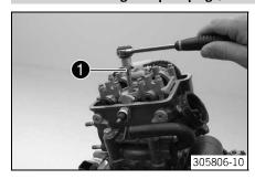
Mount and tighten the spark plug using special tool ①.
