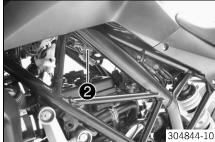
Remove the cable binder, expose the connector ② of the lambda probe, and detach
