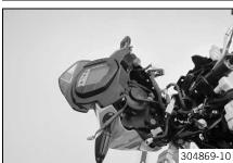
Remove the combination instrument.
