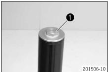
Loosen the screw cap 1.
