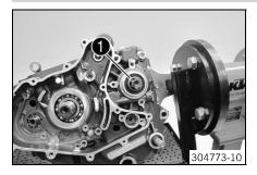
Remove the spacer • of the countershaft.
