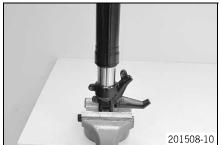
Release the fork leg and clamp it with the fork stub.
