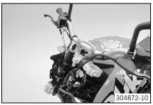
Remove the upper triple clamp with the handlebar and set aside.
