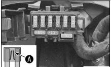
Remove the defective fuse.
