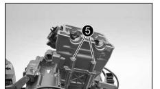
Mount and tighten screws 6.
