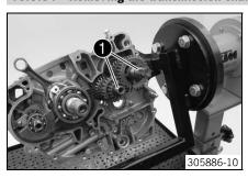
Pull both transmission shafts ● out of the bearing seats together.
