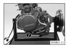
Mount and tighten oil drain plug ② with the O-ring.
