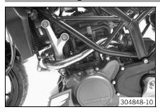
Position the exhaust manifold.
