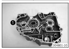
Warm the engine case section in an oven.
