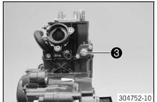
Mount and tighten screw 3 with the O-ring.
