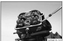
Check the valve clearance at all valves between the camshaft and cam lever.
