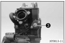
Mount and tighten screw 3 with the O-ring.
