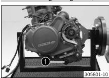
Remove oil drain plug • with the O-ring.
