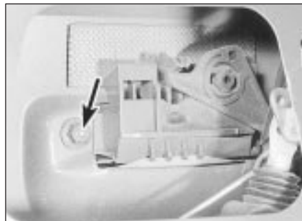
14.7a Exterior door handle securing nut (arrowed) - early model
