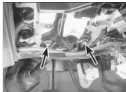
17.11 Lower steering column securing nuts (arrowed) - models from 1993
