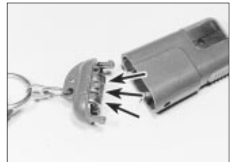
20.35 Rear cover removed from remote transmitter to expose batteries (arrowed)
