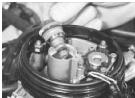
15.3b . . . then lift off the cap and withdraw the injector
