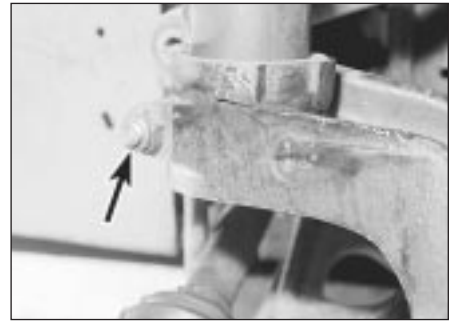
2.12 Hub carrier-to-suspension strut clamp nut (arrowed)
