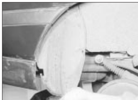
7.2 Removing a rear wheel arch liner
