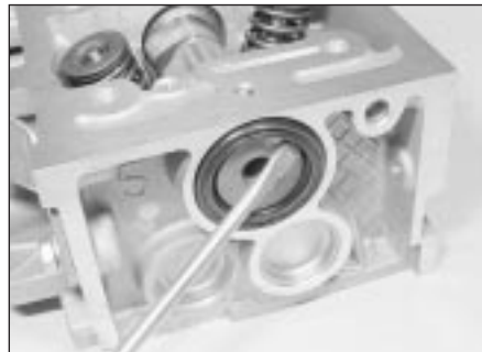
10.9a . . . prise out the oil seal . . .
