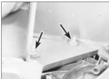
6.3 Front bumper front securing nuts (arrowed)
