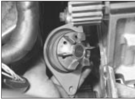
7.6a Withdraw the coolant pump . . .
