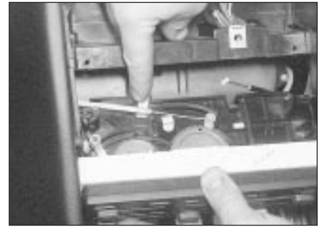
9.24 Disconnect the control cables from the heater control unit - models from 1993
