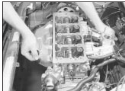
11.33 . . . then lower the cylinder head into position . . .
