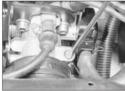
10.10 Adjusting the idle speed screw on the Bosch L3.1 injection system
