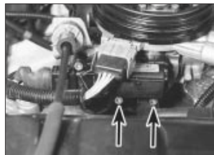
15.11 Idle control stepper motor retaining screws (arrowed)
