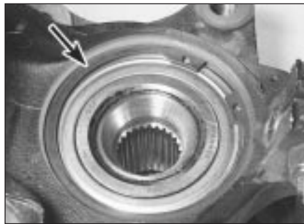
3.3 Front hub bearing retaining circlip (arrowed)
