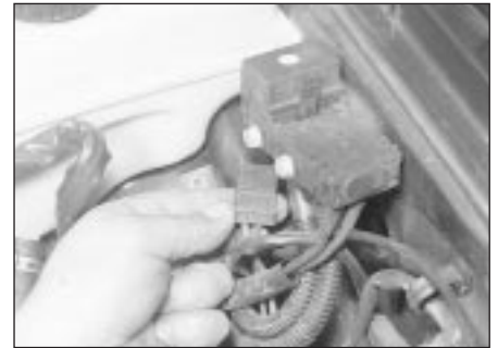
11.7c . . . and disconnect the plug from the terminal block - models from 1993
