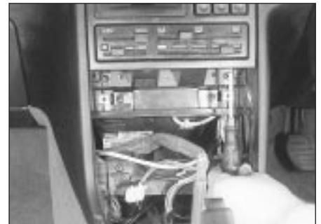
30.38b ... and the two screws from underneath
