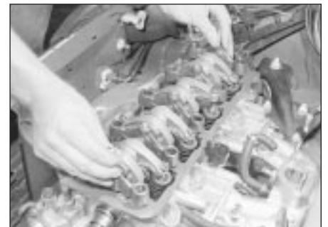
11.34 . . . and refit the rocker arm assembly
