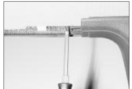
27.2 Removing an upper B-pillar trim panel top securing screw
