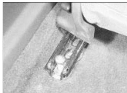
26.3 Front seat rear securing bolt partially removed
