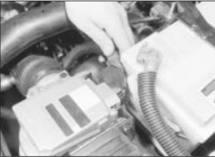
2.1 Disconnecting the airflow meter multi-plug (Bosch L3.1-Jetronic)
