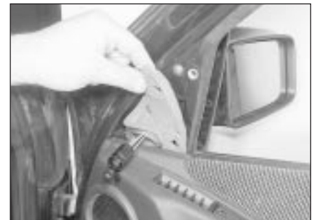
22.5a Prise off the sealing strip . . .
