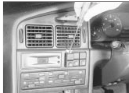
4.14 Prising out a fascia-mounted switch - models from 1993
