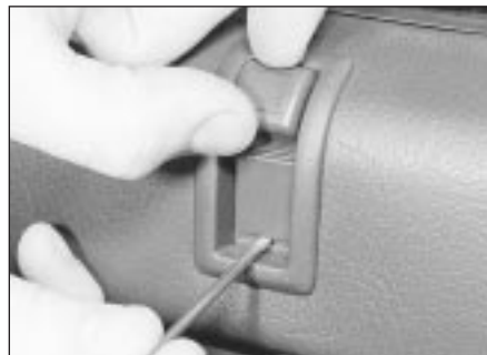
13.5 Depress the retaining tab and slide off the lock operating button
