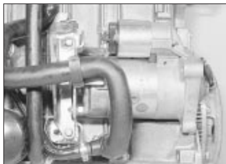
10.3 Starter support bracket bolts (arrowed) on an early model
