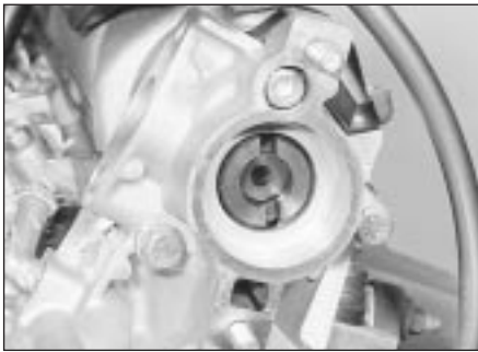
4.10 Off-set drive slots on the camshaft
