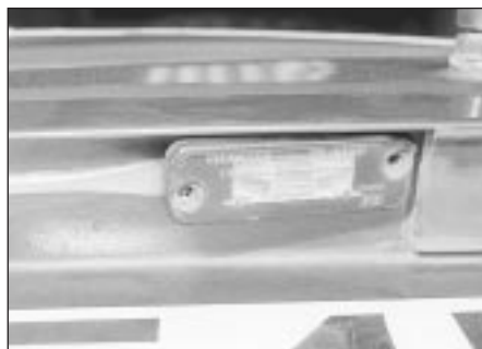
5.42 Prise out the number plate light unit ...
