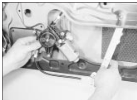
15.16 Removing the front door window regulator assembly
