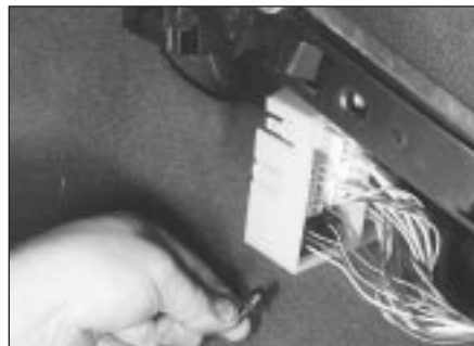
30.48 Release the connector block from the bracket on the driver's side of the facia
