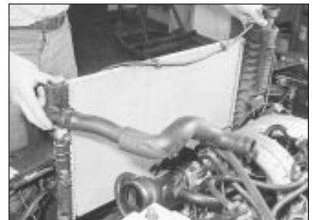
3.11 Lifting out the radiator
