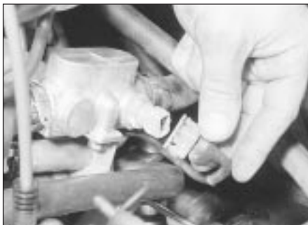
14.48 Disconnecting the injection thermistor wiring
