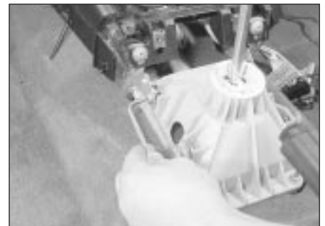
30.67 Unscrew the centre fascia lower securing bolts
