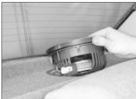
21.13 Removing the rear loudspeaker - Saloon models
