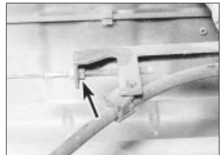
17.7 Handbrake cable adjuster (arrowed)
