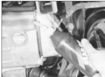
26.4 Topping-up the transmission oil level
