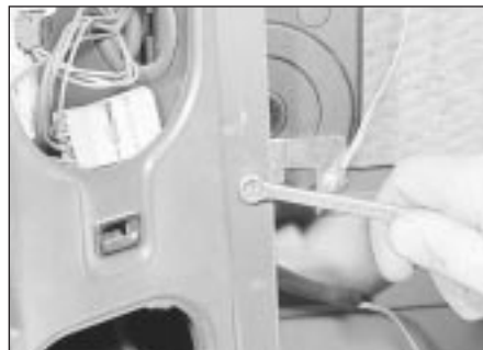
22.18b Unscrew the aerial motor securing bolt . . .
