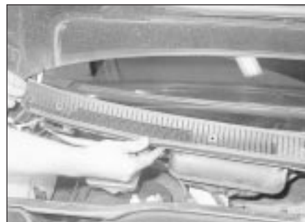
25.11 Removing the scuttle grille panel
