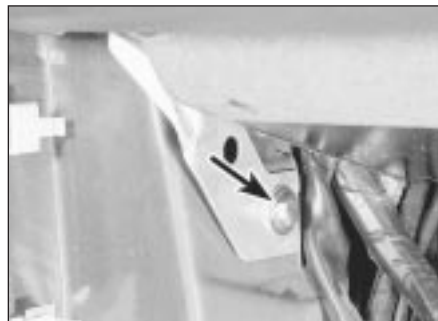
30.21 Lower facia mounting bracket-to-footwell bolt (arrowed)
