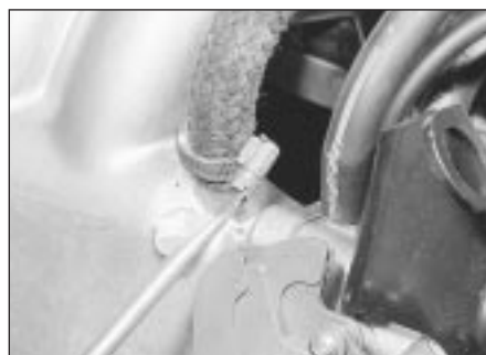
18.3 Disconnecting the brake servo vacuum hose
