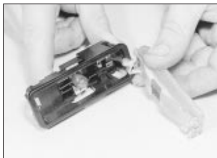
6.2b Prise off the lens for access to the bulb
