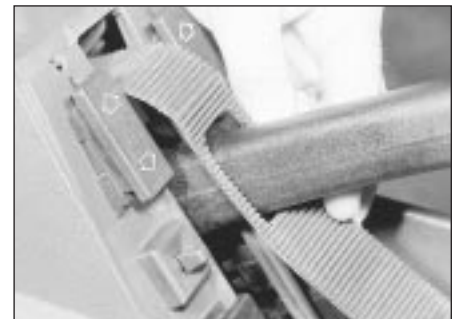
29.9 Removing the handbrake lever dust cover - models up to 1992
