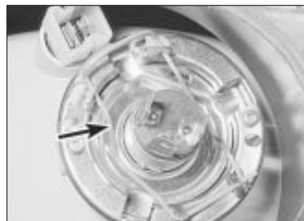
5.4a Release the spring clip (arrowed) . . .
