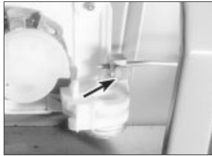
17.4 Unscrew the lock operating rod pinch-bolt (arrowed)
