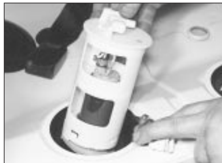
9.12a . . . then lift out the fuel pump . . .
