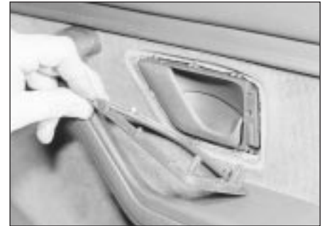
13.2 Removing the door interior handle surround
