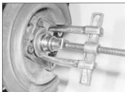
10.6b Removing the inner bearing race . . .
