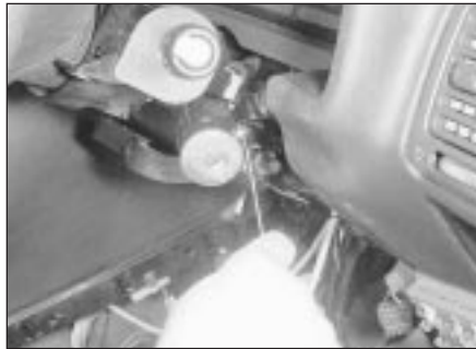
18.5 Unscrewing the lock securing screw
