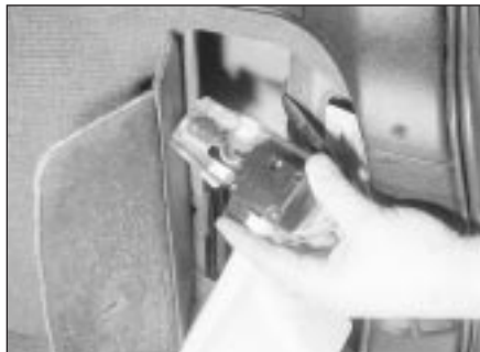
20.24b Removing the fuel filler flap lock motor - Estate model
