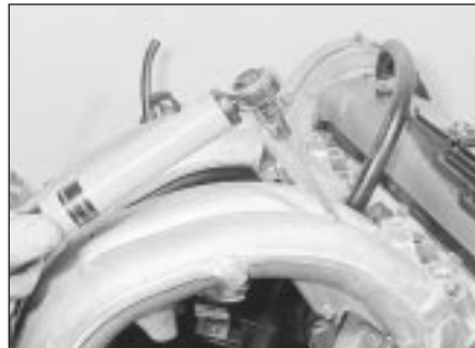
18.12d Tightening the manifold securing bolts
