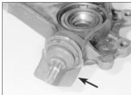
7.2 Tap the dust shield (arrowed) from the balljoint
