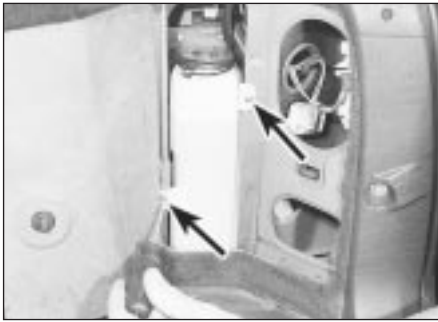
19.8a Remove the two securing screws (arrowed) . . .
