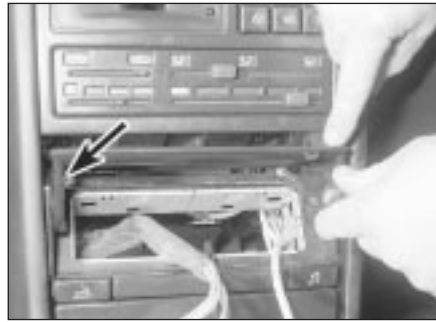
30.36a Remove screws from top of radio/cassette player/oddmeters housing ...
