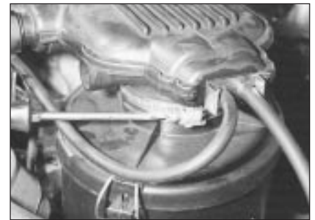
2.2a . . . slacken the retaining clips . . .
