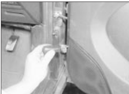
13.3 Removing a loudspeaker cover panel securing screw
