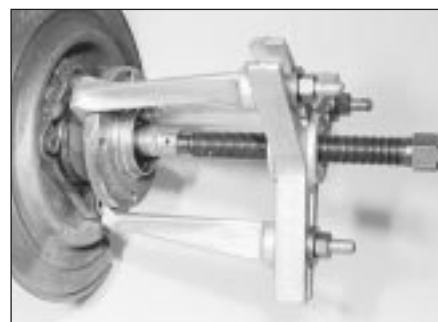
10.6a Using a puller to draw the rear hub assembly from the stub axle
