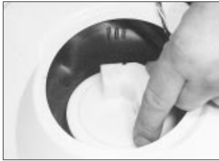
10.1 Removing the fuel gauge sender unit
