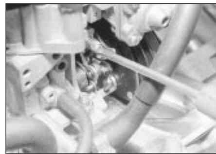
10.4b Idle speed adjustment screw
