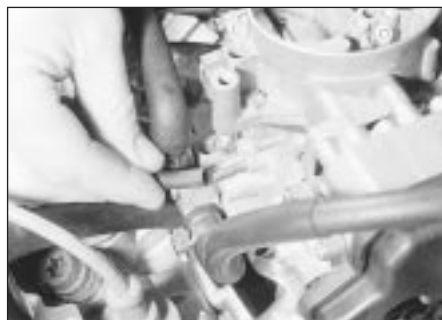
12.4 Disconnecting the distributor vacuum pipe
