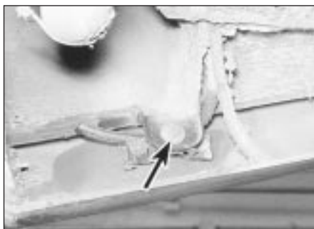
7.12 Rear bumper side securing bolt (arrowed) - Estate model
