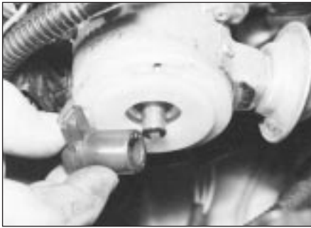
22.9 The rotor arm is a push fit on the distributor shaft
