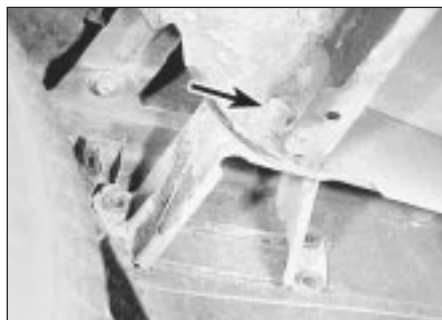
6.4 Front bumper side securing bolt (arrowed)
