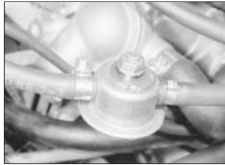
14.40 Fuel pump damper showing fuel hose connections
