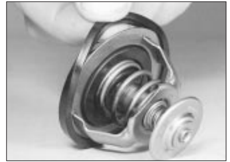
4.5 Removing the sealing ring from the thermostat flange
