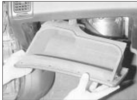
28.14 . . . and withdraw the glovebox - models from 1993
