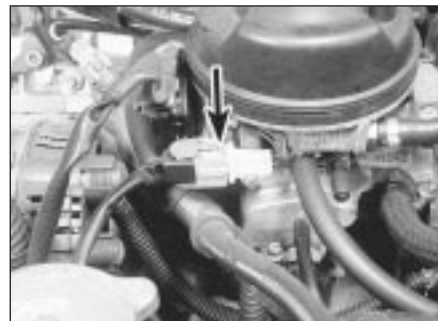
16.3 Injector wiring connector (arrowed)
