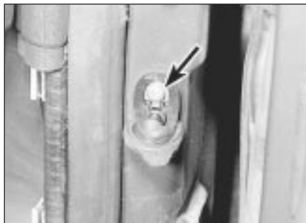
4.29 Rubber gaiter pulled back to expose courtesy light securing screw (arrowed)
