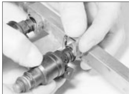
14.29 Removing an injector from the fuel rail
