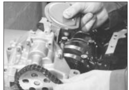
14.3 Removing the oil pump
