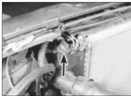
20.4c Radiator bleed screw (arrowed)
