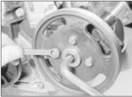
22.3 Counterhold the pump spindle and slacken the pulley bolts
