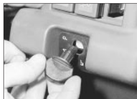
9.5 Prise off the headlight adjuster switch knob
