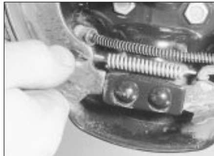
6.8 Ease the shoes out of the lower pivot point, and disconnect the lower return spring - Bendix rear brakes
