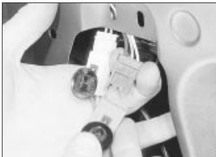
22.3 Disconnecting the door mirror wiring connectors
