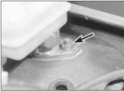
13.5 Master cylinder securing nut (arrowed)
