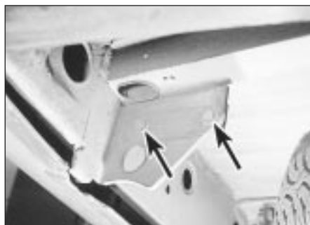
7.13 Rear bumper side securing bolts (arrowed) - Estate model
