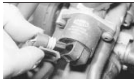
C Check the idle speed stepper motor wiring plug for security.
