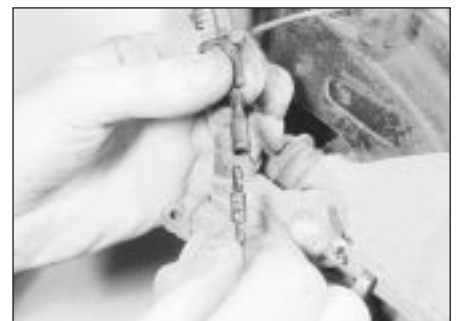
4.2 Disconnecting the pad wear sensor wiring connector
