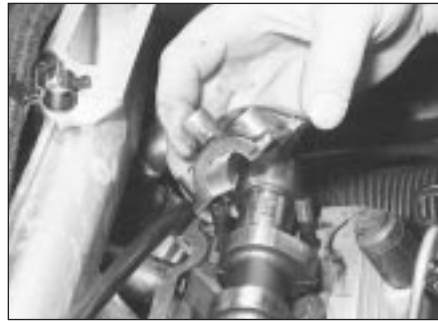
10.32 . . . and remove the camshaft bearing caps . . .
