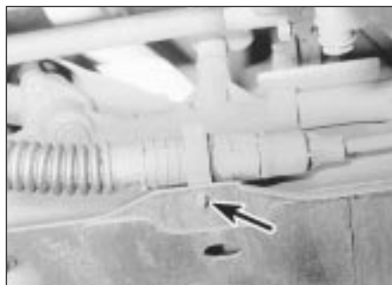
9.5 Release the clip (arrowed) securing the clutch cable to the subframe
