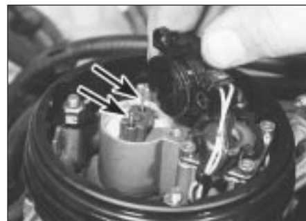
15.3c On refitting, ensure cap terminals are aligned with injector pins (arrowed)
