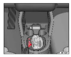
Fig. 138 Central console: selector lever for automatic gearbox / direct shift gearbox DSG
