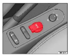
Fig. 117 Socket, centre console, front
