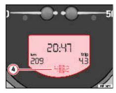
Fig. 37 Detail of the instrument cluster: screen with Tiptronic gear indicator
