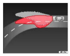
Fig. 76 Cornering lighting using directional headlights
