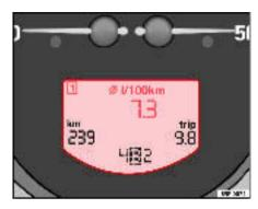
Fig. 40 Digital instrument panel display: average fuel consumption indicator
