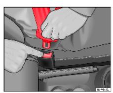
Fig. 16 Removing latch plate from buckle
