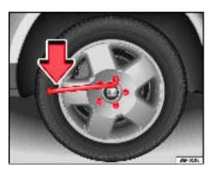
Fig. 175 Changing the wheel: loosen the wheel helts
