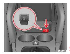
Fig. 118 Auxiliary audio connection
