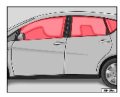
Fig. 25 Deployed curtain airbags
