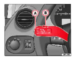
Fig. 145 Turn signal and main beam headlight lever switch and rocker switch for the cruise control
