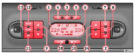
Fig. 131 On the dash panel: 2C Climatronic controls
