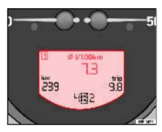
Fig. 42 Digital instrument panel display: average fuel consumption indicator.
