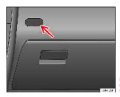
Fig. 27 Warning lamp for deactivated passenger airbag in centre console
