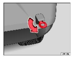
Fig. 205 Fitting the towing eye to the rear of the vehicle
