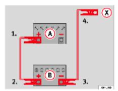
Fig. 203 How to connect the jump leads
