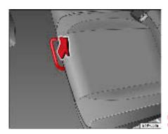
Fig. 96 For unlocking the rear seat
