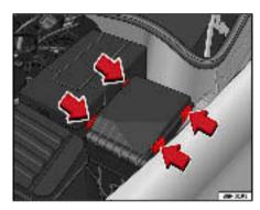
Fig. 181 Fuse box cover in engine compartment
