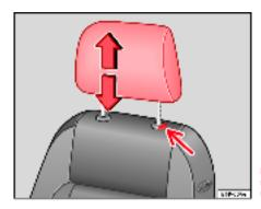
Fig. 93 Adjusting and removing the head restraints
