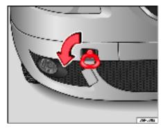
Fig. 204 The front right section of the vehicle: Fitting the front towing eve
