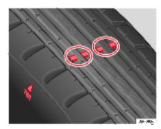
Fig. 171 Tyre tread wear indicators
