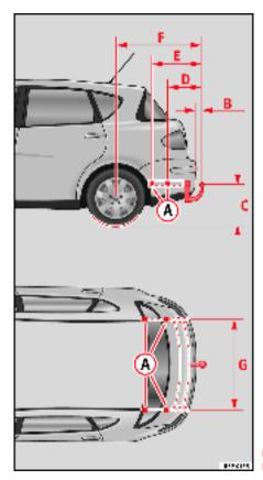
Fig. 158 Attachment points for towing bracket
