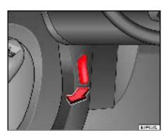
Fig. 160 Detail of footwell area on driver's side: lever for unlocking the bonnet.
