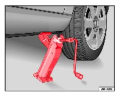
Fig. 177 Fitting the jack
