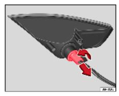
Fig. 195 Rear light after removal from bumper
