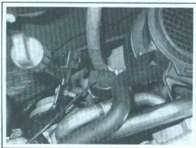
4.38 Pry out the locking clip securing the filler tube cap
