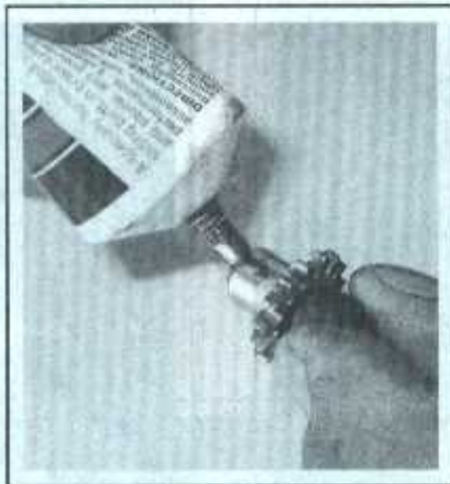
10.4m Lubricate the outer wall of the star-wheel adjuster in the adjuster assembly with high-temperature brake grease
