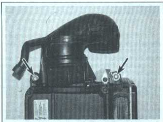
9.27 Air filter housing mounting bolt locations - 2003 and later four cylinder engine (housing removed for clarity)
