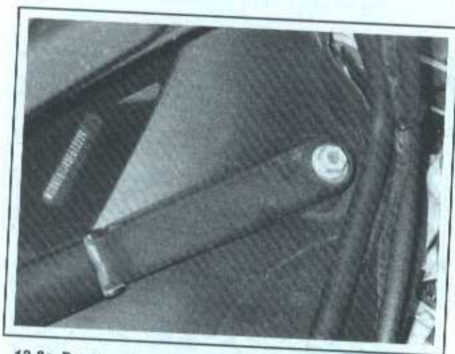
12.2a Remove the nut from the driver's side wiper arm . . .
