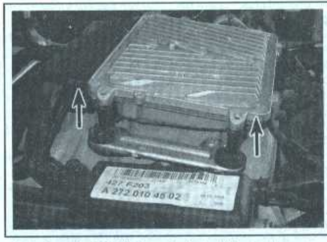
14.9 Grasp the PCM firmly and pull straight up to disengage the PCM locator pins (2006 and later V6 models)
