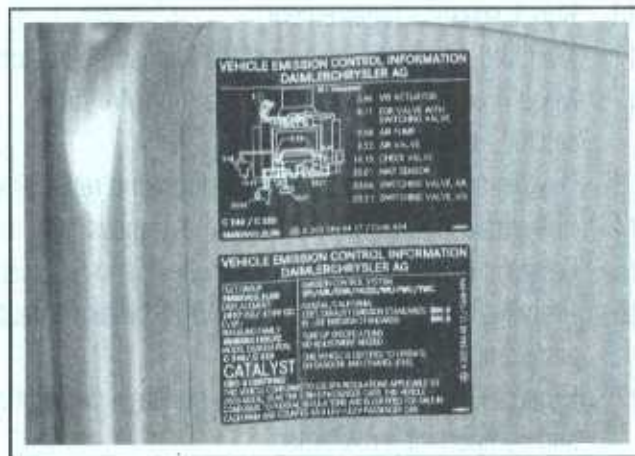
1.7 The Vehicle Emission Control Information (VECI) label, which is located on the underside of the hood, includes a vacuum hose routing diagram for your engine and information about the emission devices installed on your vehicle
