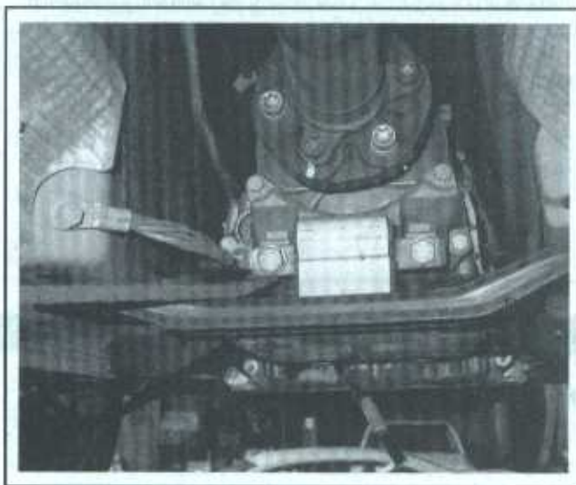
6.2 To check the transmission mount, insert a large screwdriver between the extension housing and the crossmember and try to lever the transmission up
