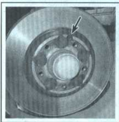
5.9 A disc retaining screw holds the disc to the hub flange
