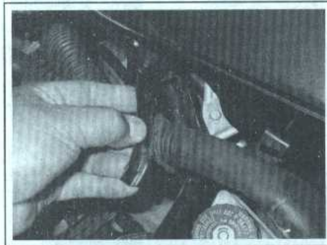
12.4c . . . slip the drain hose retainer out . . .
