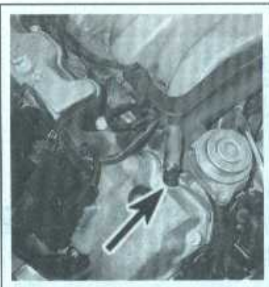
3.4a The fuel rails on all models are equipped with a Schrader valve test port like this one. To access the valve, simply unscrew the cap (2005 and earlier V6 engine shown)
