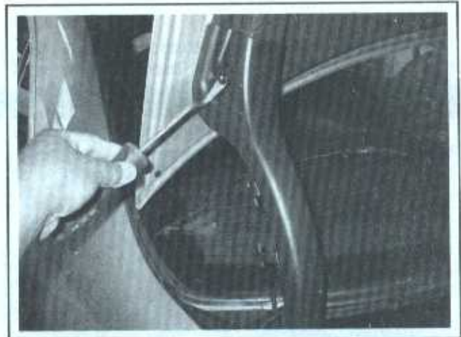
19.1b . . . pull out the center post on the pushpins and remove the hinge trim pieces
