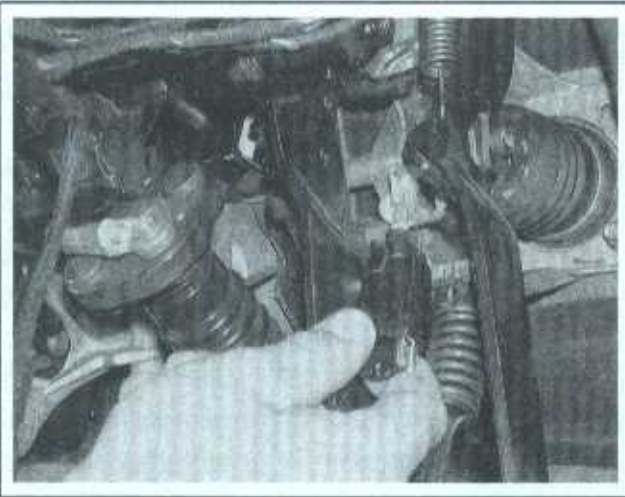
12.4 Press the small release tab and rotate the switch to remove it
