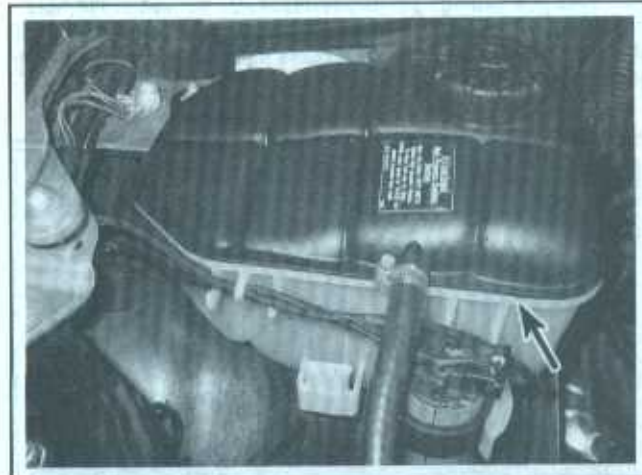
4.9 When the engine is cold, the coolant level should reach the black part of the expansion tank
