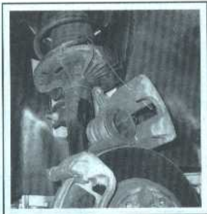
3.6d Lift the caliper up and secure it with a piece of wire; do not allow the caliper to hang by the flexible brake hose
