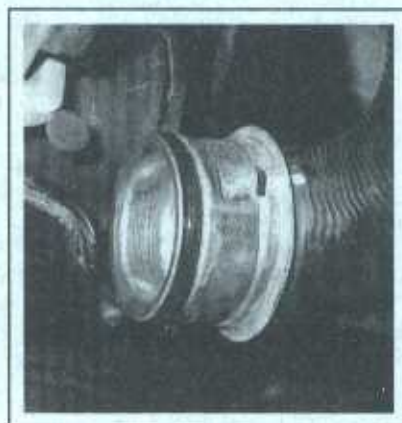
5.11c . . . then disconnect the hoses and remove the O-rings
