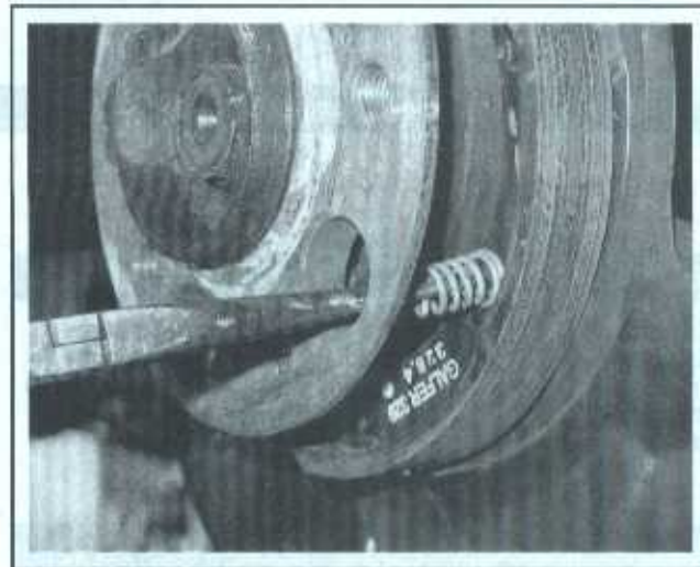
10.4d Release the lower shoe hold-down spring by grasping the center of the spring firmly with needle-nose pliers while pushing it in and turning it
