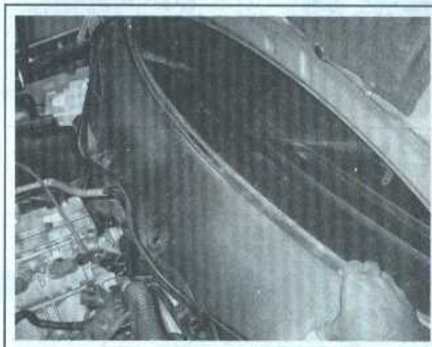
12.7b . . . and lift the water protector out
