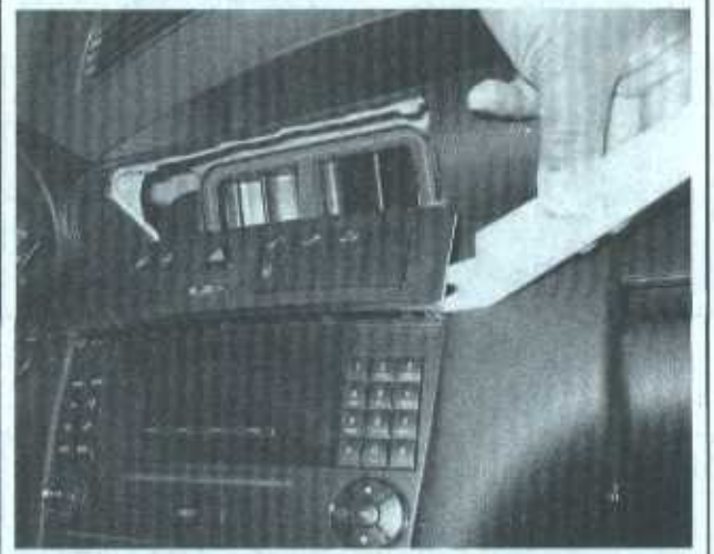
24.17b . . . then carefully pry the panel out
