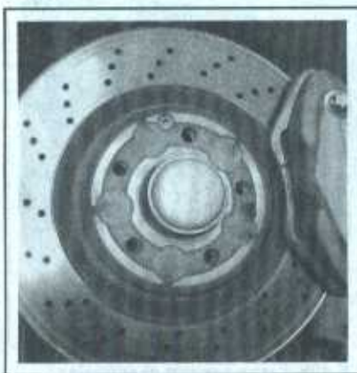
5.5 Cross-drilled discs have holes for added cooling that can get plugged with brake dust
