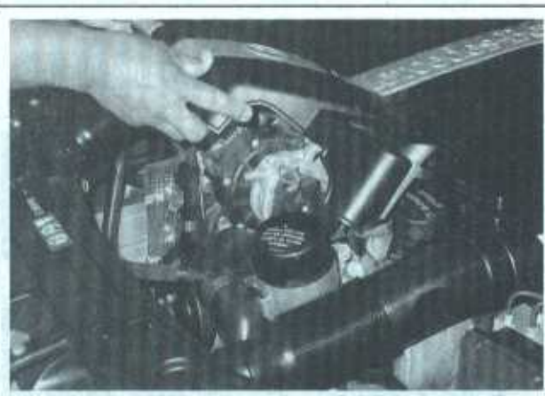
9.8 Pull up the front edge of the cover to disengage the front retaining clips and locator pin, then pull the cover forward to disengage the two rear retaining clips at the back of the cover (2001 through 2005 V6 models)
