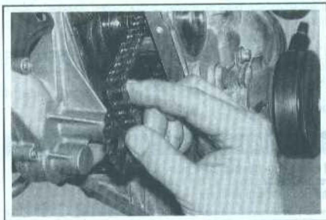
14.3 Push against the oil pump chain tensioner and slip the chain from the pump sprocket
