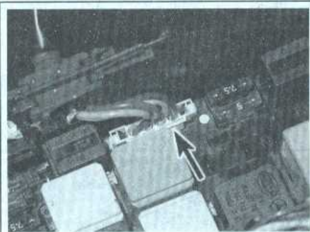
12.3 Unplug the wiper motor wiring connector and free its grommet from the fuse box
