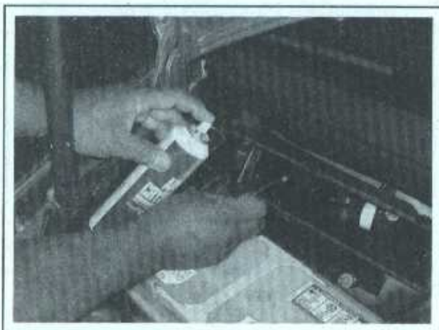
11.26 With the cabin air filter removed and the blower set to its highest setting, spray the disinfectant into the opening
