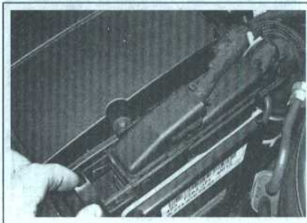
9.24a Flip up the lock and disconnect the electrical connectors from the PCM
