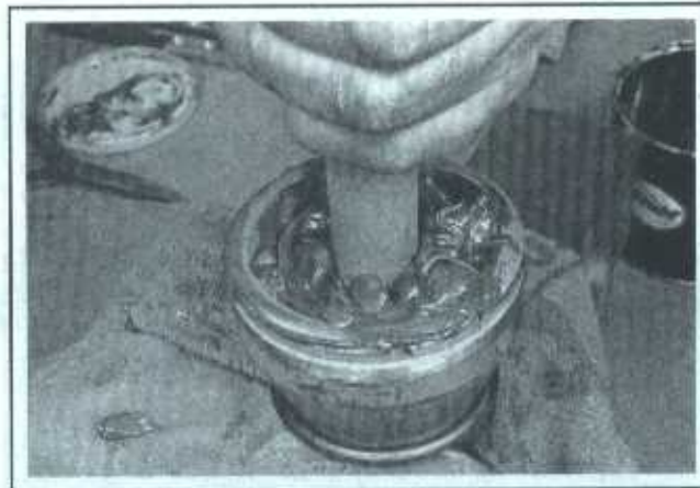
13.43d Apply CV joint grease through the splined hole, then insert a wooden dowel (slightly smaller in diameter than the hole) into the hole and push down - the dowel will force the grease into the joint. Repeat this until the joint is packed
