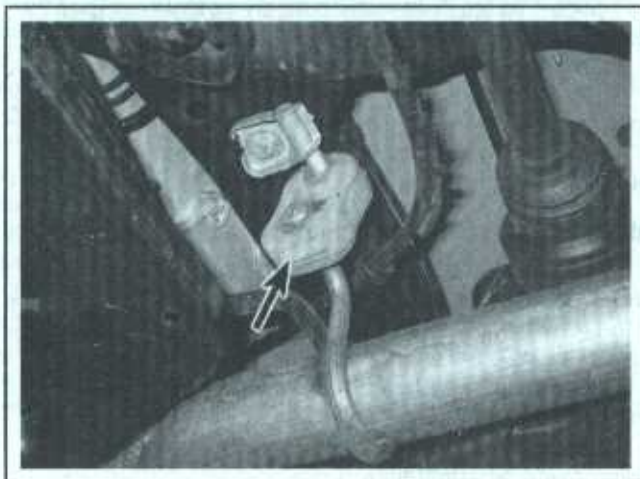
16.1a A typical rubber exhaust hanger for suspending the exhaust system
