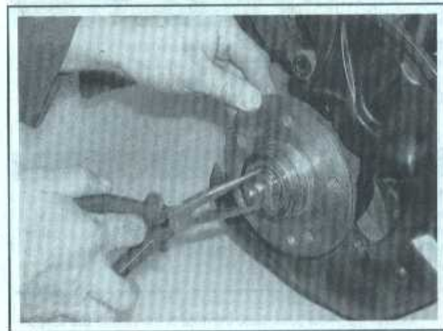
7.14 Rotate the hub forward while tightening the clamping hub nut. Repeat this a few times
