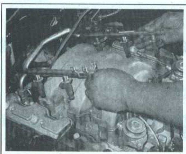
13.10 Remove the fuel rail and injectors as a single assembly
