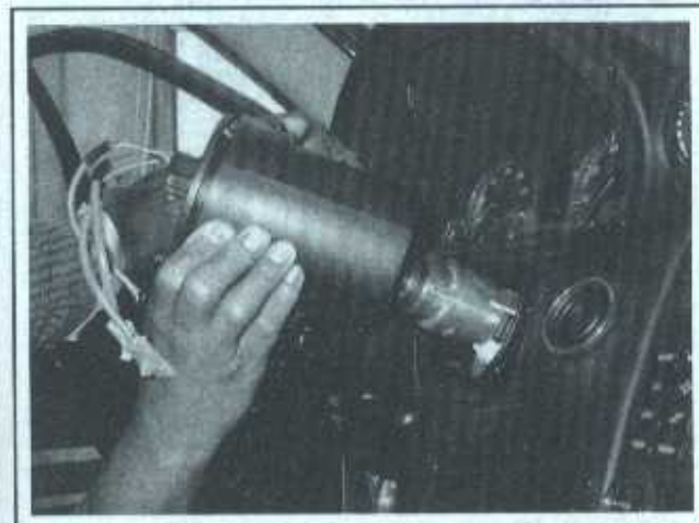
16.8b Pull the module from the steering column
