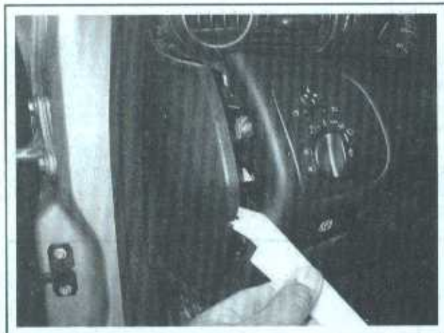
3.1e If there's a finger slot in the instrument panel cover, pull it off; if not, use a trim tool to pry it off . . .
