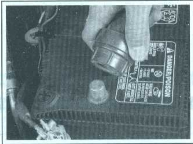
9.7b Regardless of the type of tool used to clean the battery posts, a clean, shiny surface should be the result
