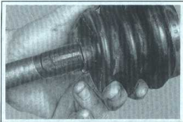
13.13 Wrap the driveshaft splines with electrical tape to prevent damaging the boot as it's slid onto the shaft
