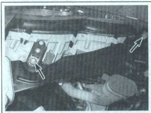
13.2a Remove the headlight housing upper mounting bolts . . .
