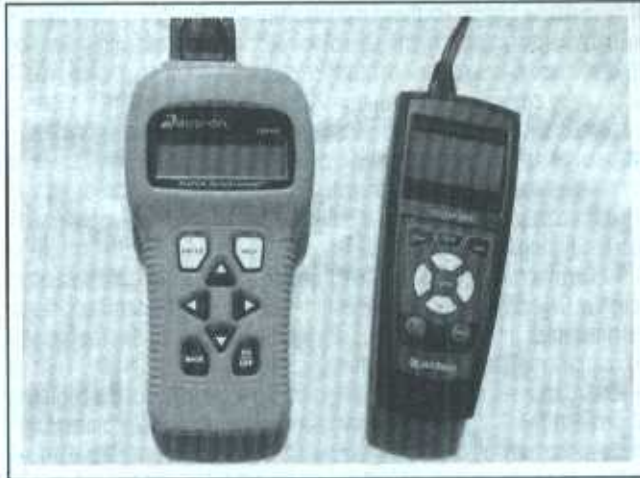
2.2 Scanners like these from Actron and AutoXray are powerful diagnostic aids - they can tell you just about anything that you want to know about your engine management system
