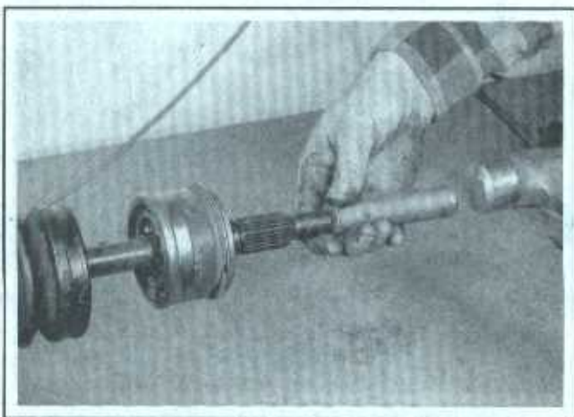
13.43i . . . then use a hammer and brass punch to carefully drive the joint onto the drive axle disassembly
