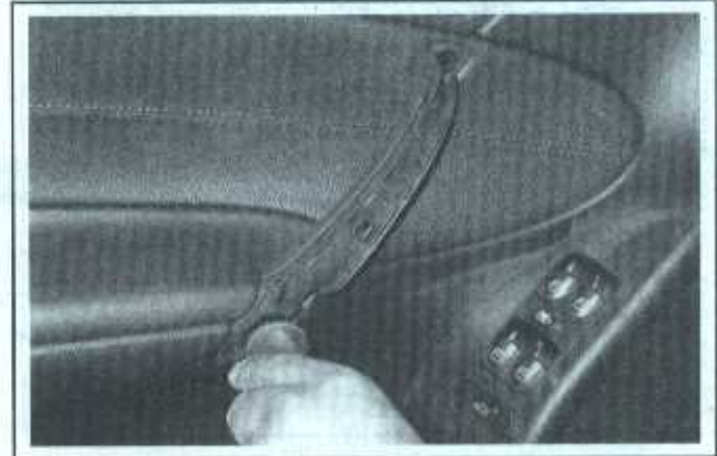
13.3 Remove the door panel screws from the armrest and from behind the SRS emblem
