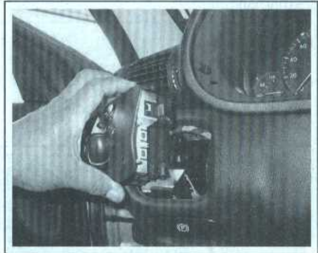
8.4 ... disengage the clips and pull the switch out of the dash ...
