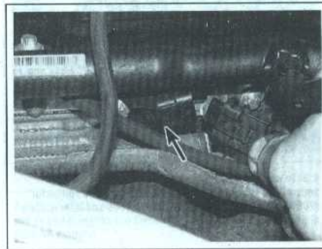
5.17b Exhaust CMP sensor, located on the right side of the cylinder head, just below the valve cover (2003 through 2005 four-cylinder engines)
