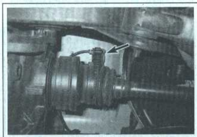
12.15 Location of the wheel speed sensor and brake pad wear sensor electrical connectors
