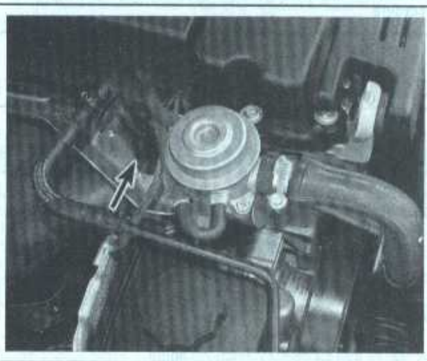
7.24 On 2003 through 2005 four-cylinder models, the ECT sensor is located on the right side of the cylinder head
