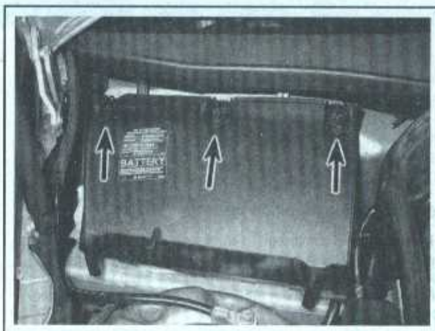
3.6 To remove the battery cover, flip open these three retainer clips, then carefully pull off the cover
