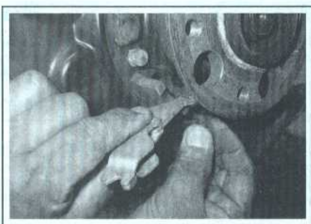
10.4j Move the expanding lock and remove the pin that connects it to the cable. Lubricate the moving parts of the lock and pin with high-temperature brake grease and place it back into position
