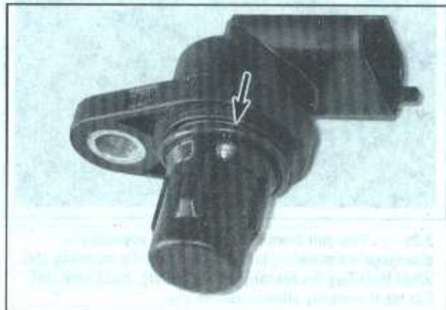
5.4 Even if you plan to reuse the old CMP sensor, be sure to remove and replace the O-ring
