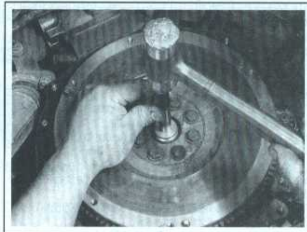
6.6 If available, use a bearing driver to install the pilot bearing
