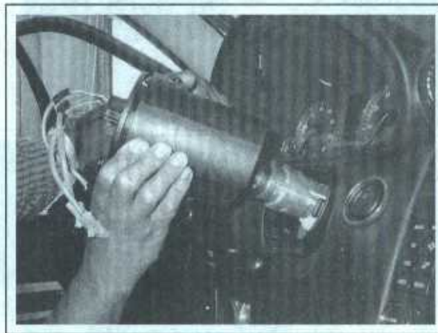
23.3b . . . then slide the cover and switches off the steering column
