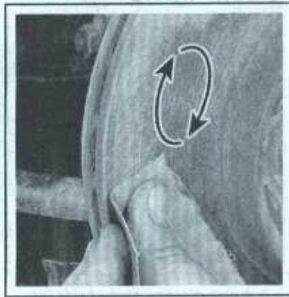
5.6b Using a swirling motion, remove the glaze from the disc surface with sandpaper or emery cloth
