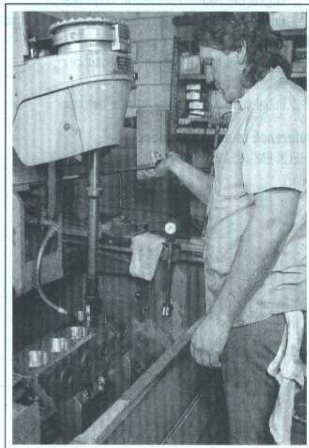
1.2 If the cylinders are bored, the machine shop will normally hone the engine on a machine like this
