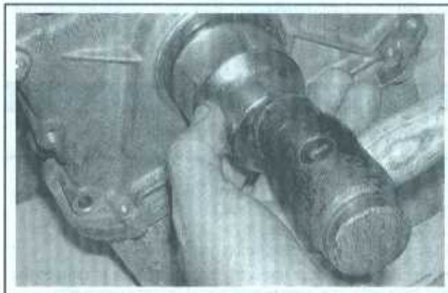
12.4 A seal driver or an appropriate-size socket can be used when tapping in the new seal
