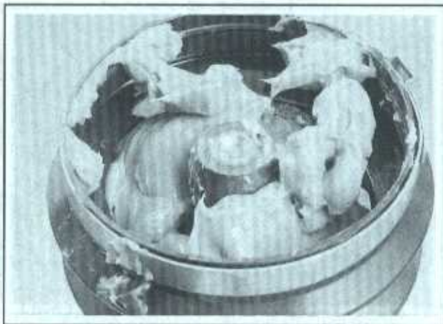
13.43g . . . the level is up to the end of axle
