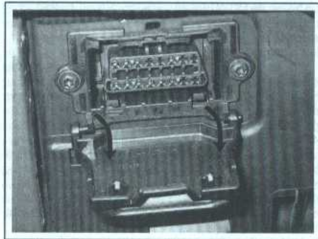
2.26b To access the diagnostic connector, flip open this small hinged door, then plug in the scan tool
