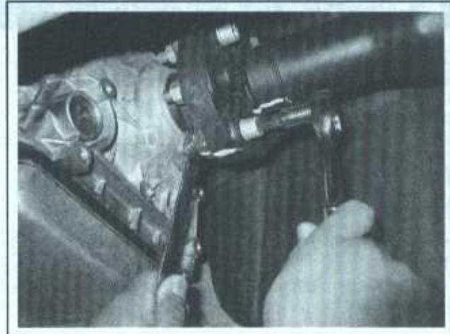
9.8 Remove the bolts securing the driveshaft flange to the transmission pinion flange
