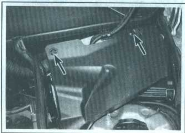
4.14 Release the clips by turning them 1/4-turn, then remove the cover to access the brake fluid reservoir
