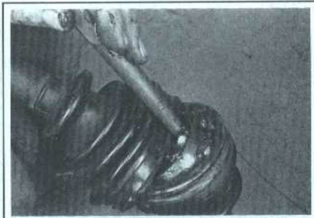
13.43b Clamp the driveaxle in a vise, pull back the boot, then strike the inner race of the CV joint with a hammer and drift to dislodge it from the axle
