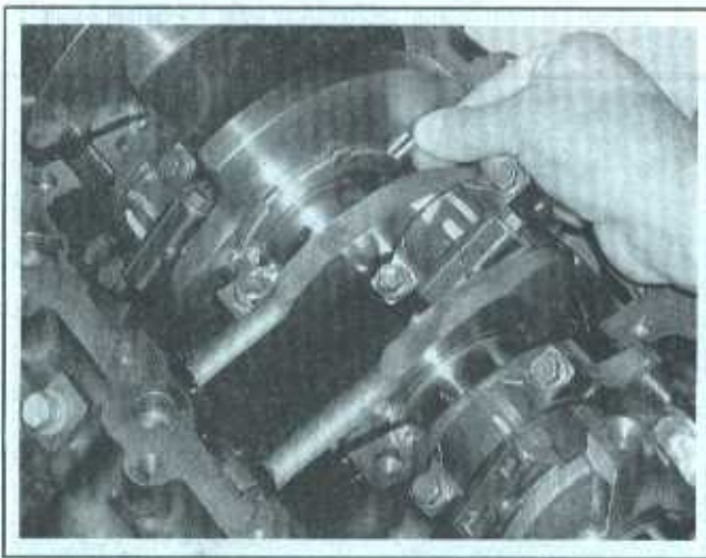
10.14 Insert the thrust washer into the machined surface between the crankshaft and the upper bearing saddle, then rotate it down into the block until it's flush with the parting line on the main bearing saddle - make sure the oil grooves on the thrust washer face the crankshaft
