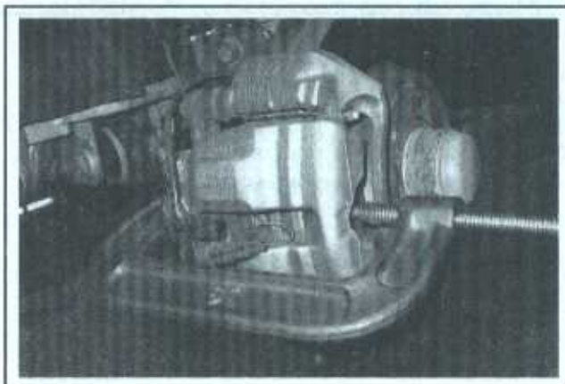
3.5 Before removing the caliper, slowly depress the piston into the caliper bore by using a large C-clamp between the outer brake pad and the back of the caliper
