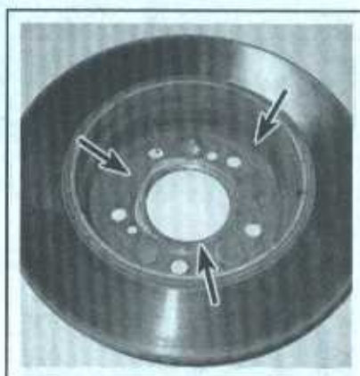
5.10b Clean any rust or corrosion from the area inside the disc that contacts the hub flange. Again, power tools are very useful for this job
