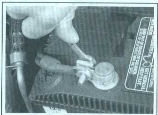
9.6b Removing a cable from the battery post with a wrench - sometimes a pair of special battery pliers are required for this procedure if corrosion has caused deterioration of the nut hex (always remove the ground (-) cable first and hook it up last!)
