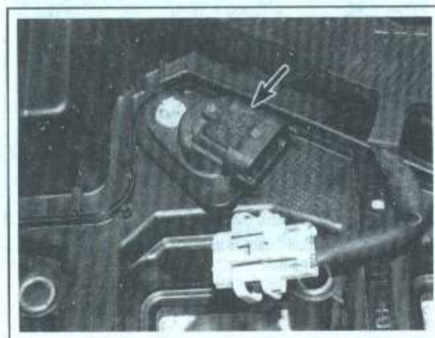
5.17a Intake CMP sensor, located on the top of the valve cover on the left side (2003 through 2005 four-cylinder engines)
