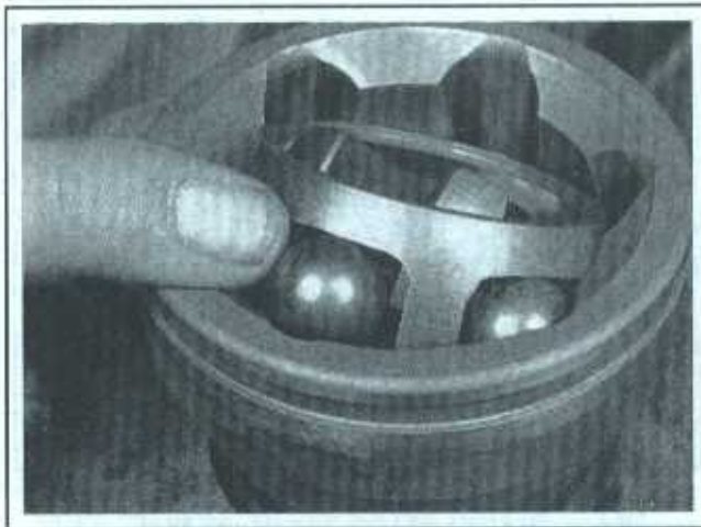
13.7 With the cage and inner race tilted, the balls can be removed one at a time (driveaxle shaft removed for clarity)
