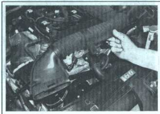
9.22 Remove the air intake duct
