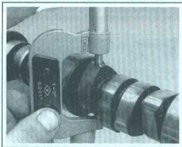
7.16 Measure the camshaft lobe height (greatest dimension) with a micrometer
