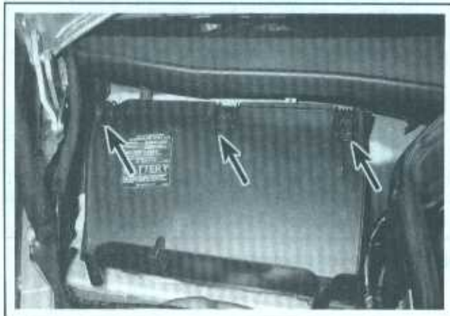
15.1a Release the clips to open the air inlet grille
