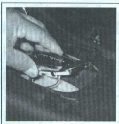
22.1b Release the clips and lift off the trim panel . . .
