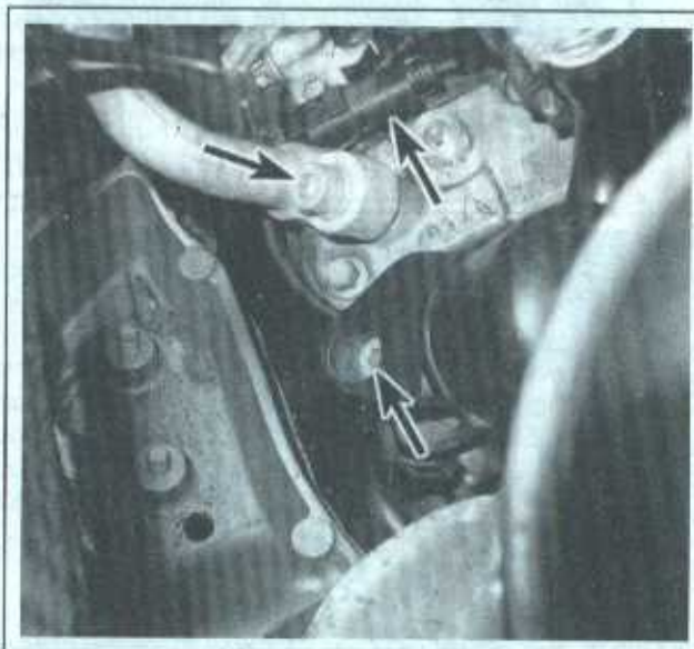
13.5 Disconnect the wiring and refrigerant lines from the compressor
