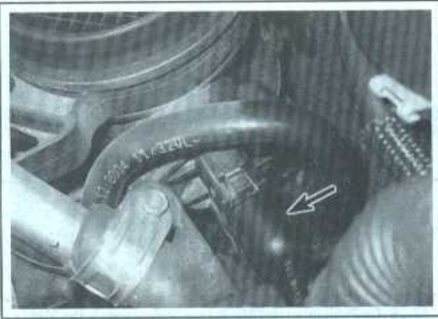
12.2a To disconnect the electrical connector from the MAF/IAT sensor . . .
