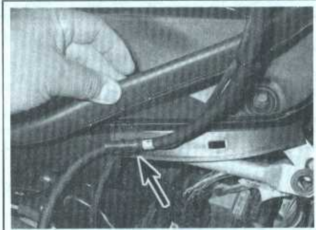
12.4a Pull the gasket off the water deflector and free the wiring harness from the retainer
