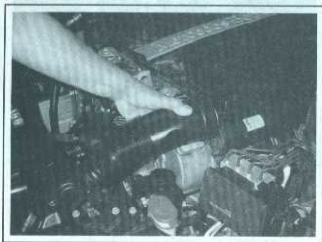
7.5 Pull off the fresh air intake ducts from the air filter housing
