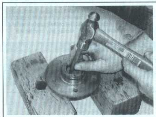
7.7 Set the hub between two blocks of wood. Use a drift to remove the inner bearing and grease seal from the hub
