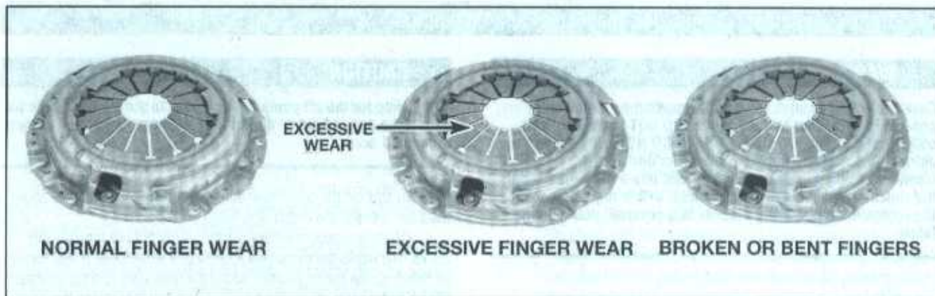
4.11a Replace the pressure plate if excessive wear is noted
