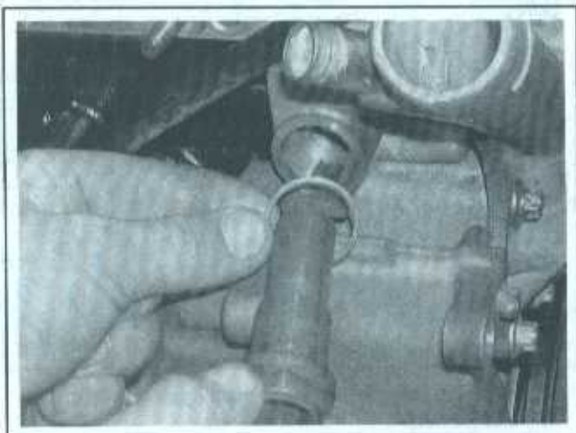
7.6 Timing chain tensioner removal - be sure to replace the sealing ring during installation
