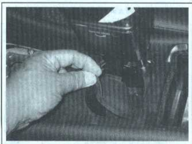
22.5a Open the cup holder and remove the liner from the bottom . . .
