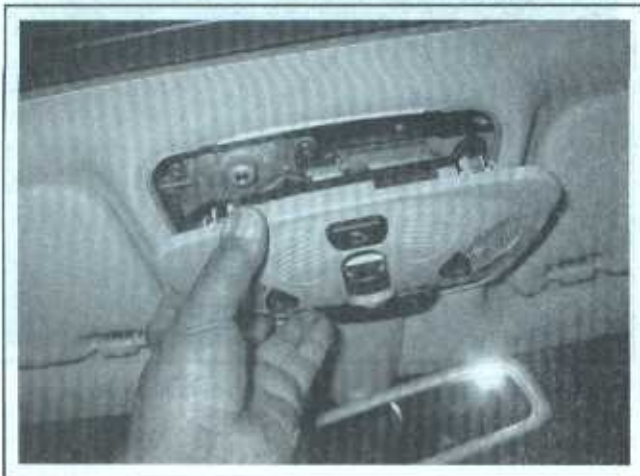
8.9b ... lower the switch unit out of the headliner ...
