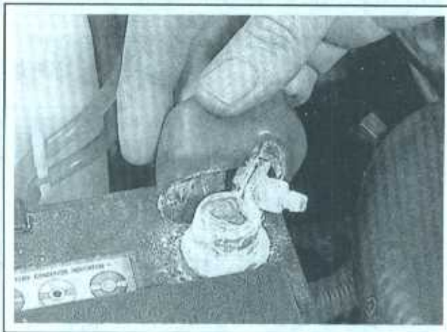
9.6a Battery terminal corrosion usually appears as light, fluffy powder
