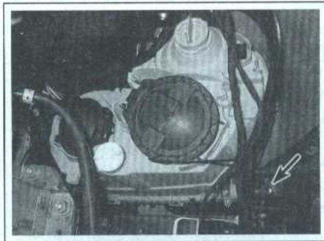
13.2b . . . and the lower mounting bolt and thumbwheel
