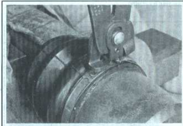
13.22 Depending on the type of clamps furnished with the replacement boot, you'll most likely need a special pair of clamp tightening pliers (most auto parts stores carry these)
