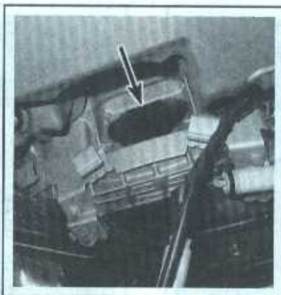
8.8 Remove the torque converter cover from the transmission
