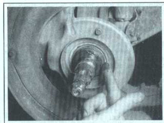
7.9 Coat the entire spindle with high-temperature brake grease
