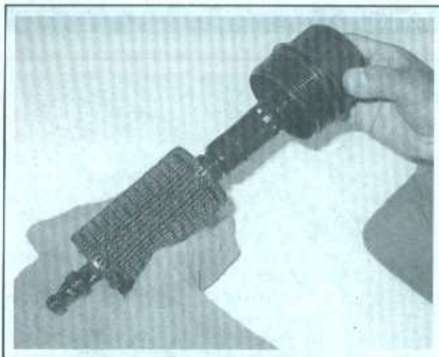
6.6c Pull the used element off of the filter cap stem
