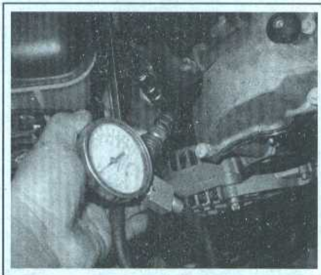
3.6 Use a compression gauge with a threaded fitting for the spark plug hole, not the type that requires hand pressure to maintain the seal
