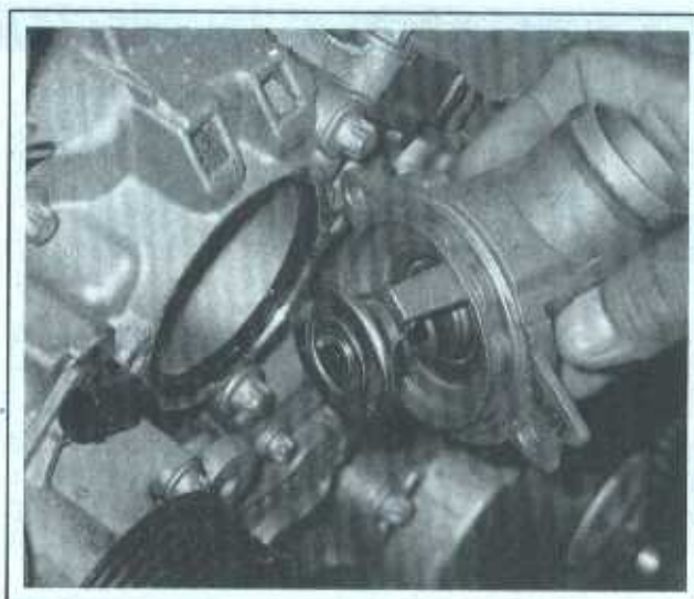
3.11b Unbolt and remove the thermostat housing cover from the timing case cover (2005 and earlier V6 engines)
