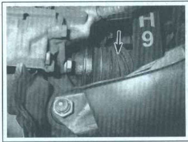
17.14 Inspect the inner and outer driveaxle boots for loose clamps, cracks or signs of leaking lubricant
