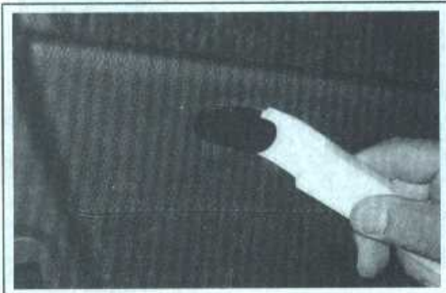
13.2 Pry the SRS emblem out of the door panel
