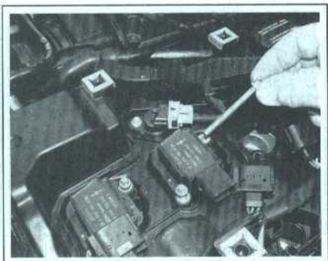
7.14a Remove the mounting bolts . . .
