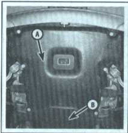
8.3 Front (A) and rear (B) engine splash shields
