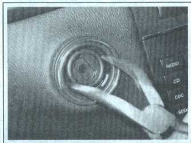
7.9 If you don't have a special socket, a pair of needle-nose pliers can be used to unscrew the ignition switch nut
