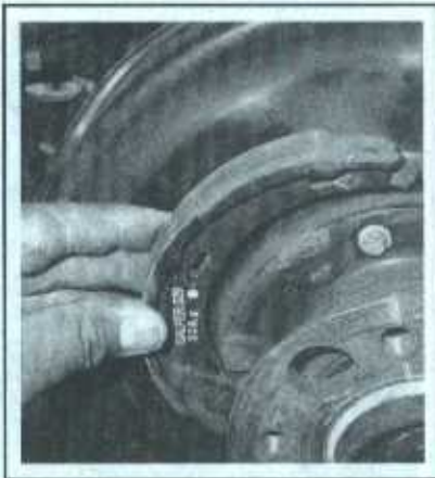
10.4n Place the upper shoe into position . . .
