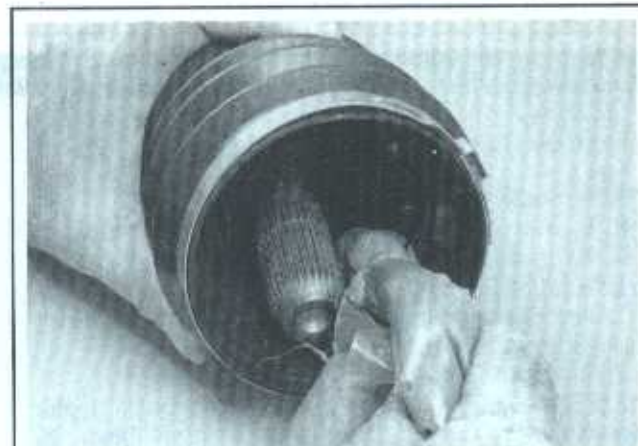
13.43f Install the small clamp and the boot on the driveaxle and apply grease to the inside of the axle boot until . . .
