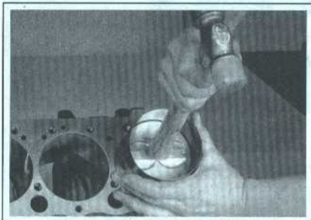
9.35 Use a plastic or wooden hammer handle to push the piston into the cylinder
