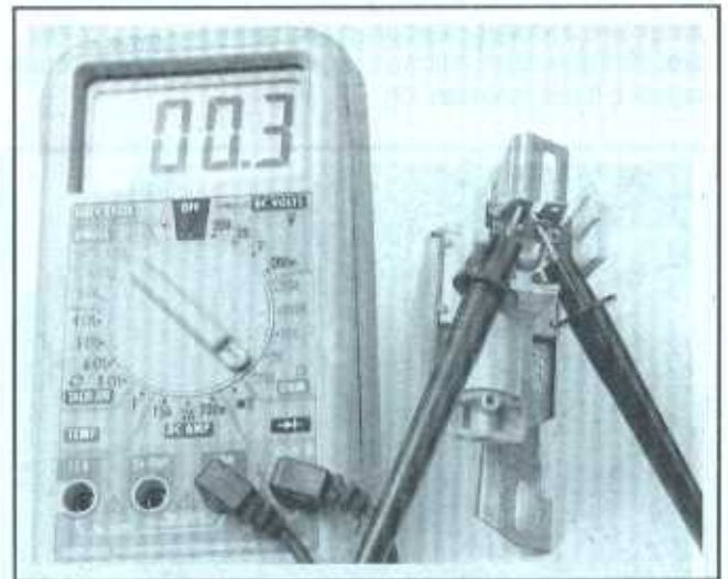
2.9 With a multimeter set to the ohm scale, resistance can be checked across two terminals - when checking for continuity, a low reading indicates continuity, a high reading or infinity indicates high resistance or lack of continuity
