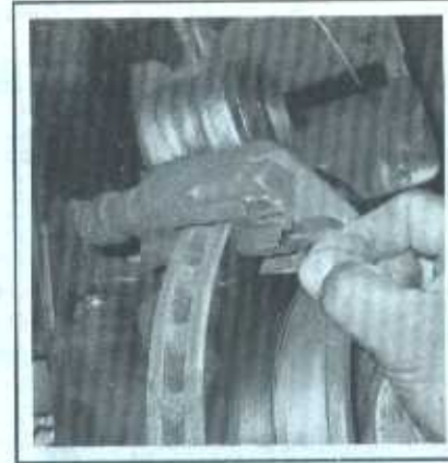
3.6h Remove the upper and lower anti-rattle clips; make sure they fit tightly and aren't worn. Replace them if necessary
