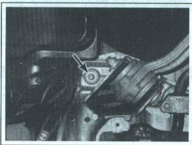
9.20a Location of the left-front mounting bolt (rear wheel drive model shown - 4MATIC models similar)
