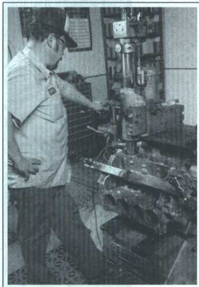
1.1 An engine block being bored. An engine rebuilder will use special machinery to recondition the cylinder bores
