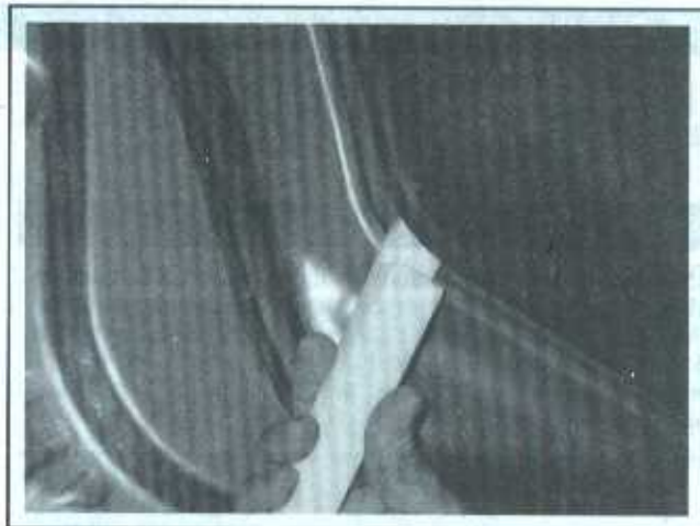
13.7a Start from the bottom of the trim panel and work around the perimeter until all the fasteners have been released from the door . . .
