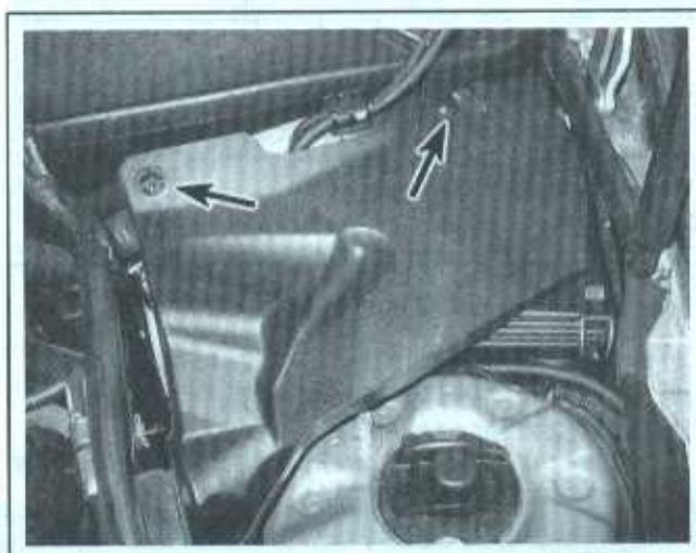
6.3 Turn the fasteners 1/4-turn and remove the cover
