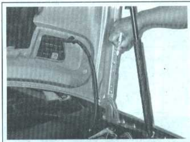
9.2 Before removing the hood, draw a mark around each hinge
