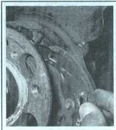
10.4q . . . and then into the lower shoe and place the shoe into position
