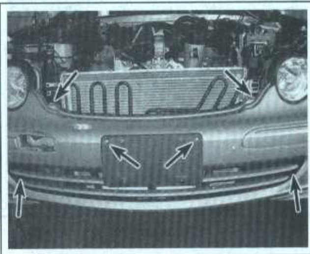
11.5 Remove the license plate holder and bumper cover bolts
