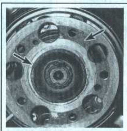
5.10a Clean any rust and corrosion from the areas of the hub flange that contact the disc. A wire brush or sanding tool, designed to be used with a power drill, can make the job a lot easier
