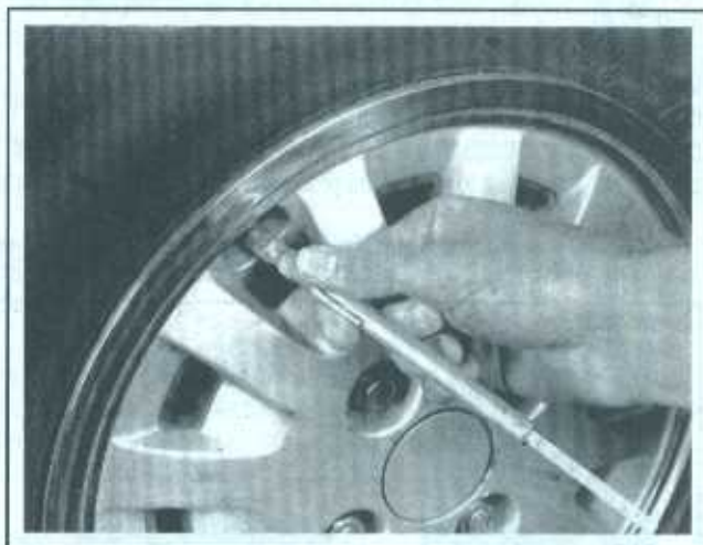
5.8 To extend the life of your tires, check the air pressure at least once a week with an accurate gauge (don't forget the spare!)
