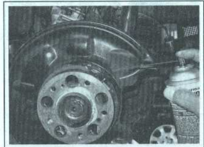
10.2 Wash the parking brake assembly with brake cleaner. Use a pan or rags underneath to catch the runoff. DO NOT USE COMPRESSED AIR TO BLOW BRAKE DUST OFF THE PARTS!
