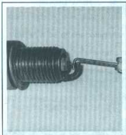
21.5 Spark plug manufacturers recommend using a wire-type gauge when checking the gap - the wire should slide between the electrodes with a slight drag
