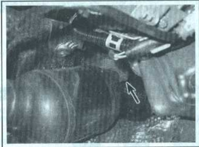
16.4a Use penetrating oil to loosen up bolts and nuts that secure the flanges between exhaust manifolds and exhaust pipes . . .
