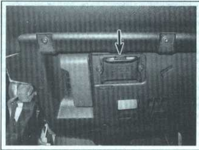
2.26a The Data Link Connector (DLC), or diagnostic connector, is located in the left underside of the instrument panel
