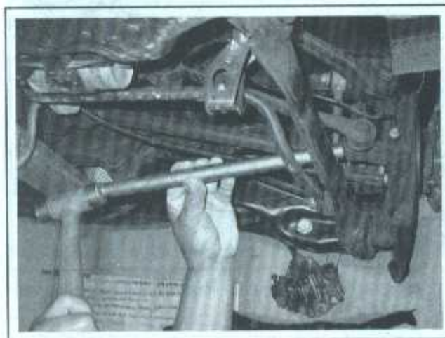
12.32 To separate the link-mounted balljoint from the rear knuckle, loosen the balljoint stud nut, then strike the knuckle using a large brass drift or equivalent to break the taper loose
