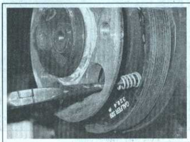
10.4r Install the lower shoe hold-down spring
