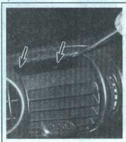
24.14b . . . then pivot the vent down and release the two retaining tangs by prying them downward
