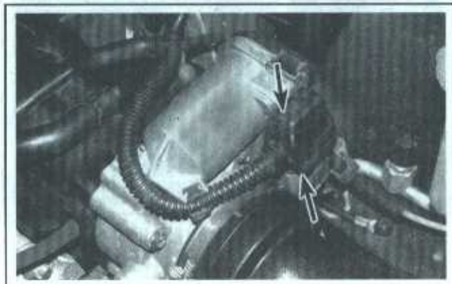
12.18 Depress the tabs and detach the electrical connector from the throttle body (2003 and later four-cylinder engines)
