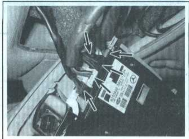
8.9c ... and disconnect its electrical connectors
