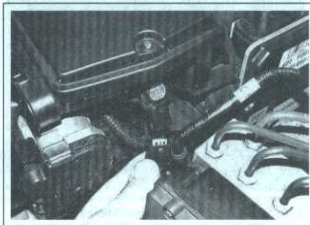
9.24c Disconnect the electrical connector from the altitude sensor
