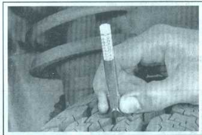
5.2 A tire tread depth indicator should be used to monitor tire wear - they are available at auto parts stores and service stations and cost very little
