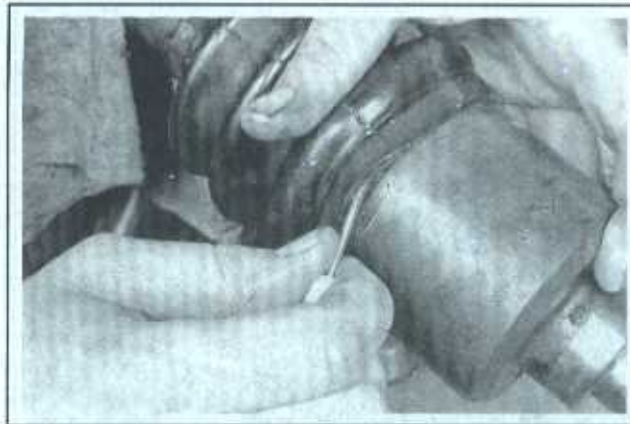
13.21 After positioning the joint mid-way through its travel, equalize the pressure inside the boot by inserting a small, dull screwdriver between the boot and the CV joint housing
