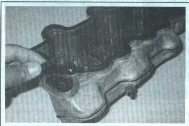
4.10a Clean and inspect the rubber valve cover gaskets - they can be reused if not cracked or damaged
