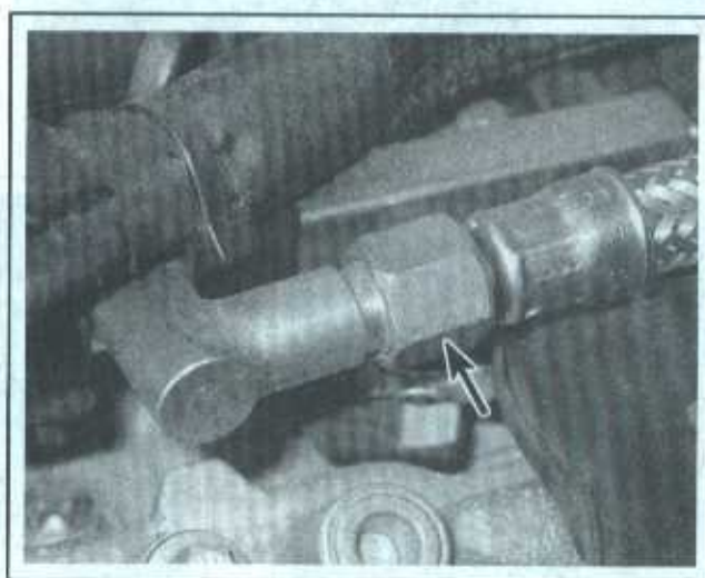
13.8 Fuel supply hose fitting at the fuel rail (2006 and later V6 models shown, earlier V6 models similar)
