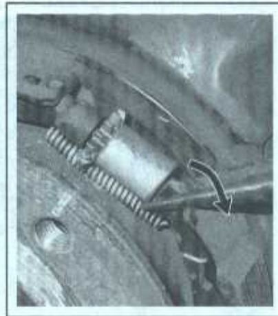
10.4b Pry the lower shoe and adjuster apart to remove the adjuster
