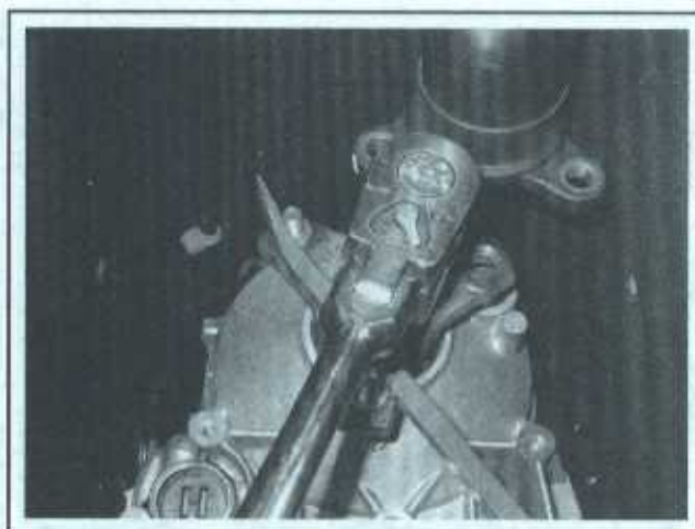
5.4b Use a long prybar for leverage when removing the retaining nut; it's on very tight
