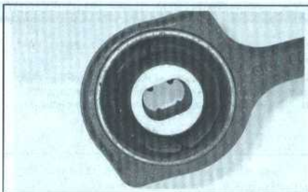
4.6 The torque strut and cross strut have lugs in the center of the bushing that engage grooved mounting bolts. Regular (non-grooved) mounting bolts are placed in between the lugs (directly in the center). Grooved bolts are placed on one side or the other (cross strut shown - torque strut is similar)
