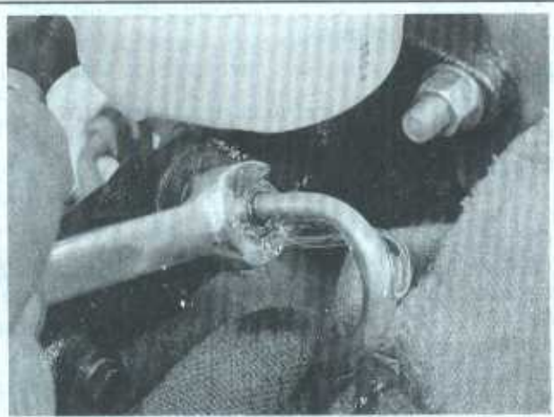
6.22 With the brake pedal depressed, loosen a fitting on the master cylinder to bleed it when it is installed on the vehicle. Bleed the lines one at a time (typical shown)
