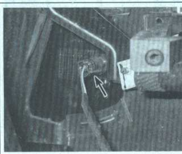
11.3 Disconnect the outside temperature sensor electrical connector, then unclip the sensor and remove it
