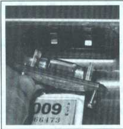
16.21 The license plate light bulb will come out with the lens
