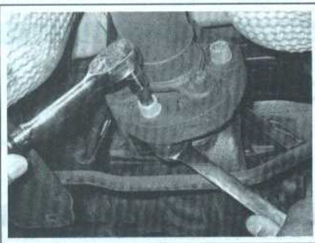
9.5 Remove the bolts securing the driveshaft flange to the differential pinion flange
