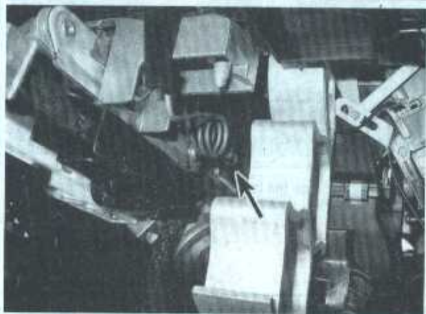
17.14 The location of the lower steering column mounting bolt
