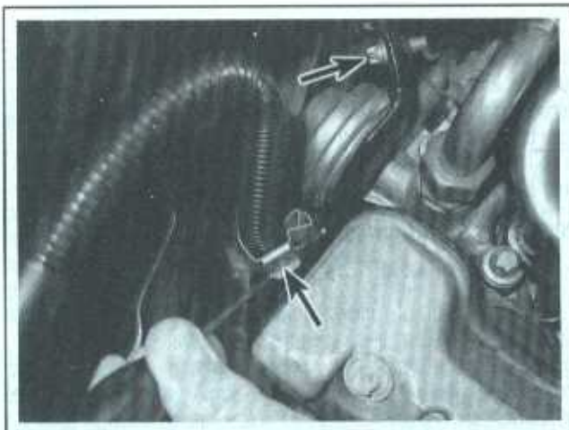
17.4 Use a small screwdriver to disengage the clip securing the battery cable. Also remove the bolt securing the dipstick tube to the bracket
