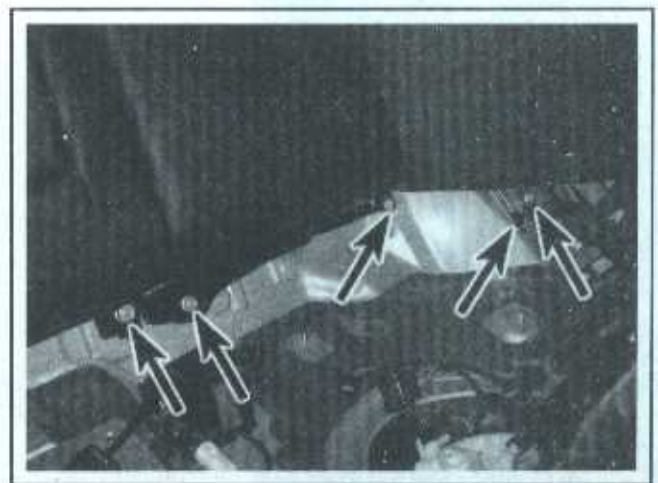
25.8 Detach the retaining bolts at the lower edge of the seat back
