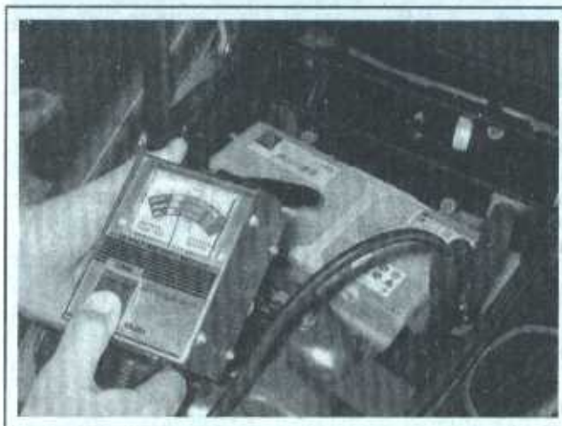
3.4 Some battery load testers are equipped with an ammeter, which enables the battery load to be precisely dialed in. Less expensive testers like this one only have a load switch and a voltmeter
