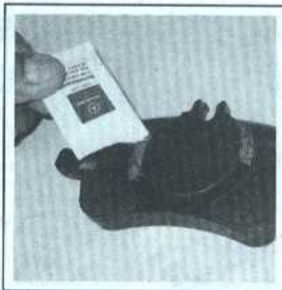
3.6m The inner pad has a shim attached that matches with the caliper piston (a circular pattern). Lubricate the contact areas with an anti-seize compound approved for disc brake use (Mercedes Benz brake pad paste shown)
