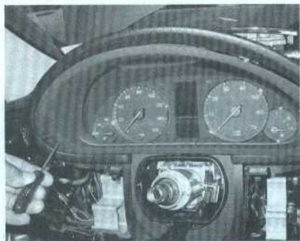
9.2a Insert hooked removal tools into the removal slots . . .
