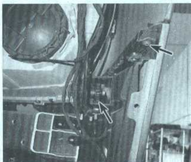
11.2a Unbolt the bumper bracket (upper arrow) and note how the bumper fits on the adjuster (lower arrow) . . .
