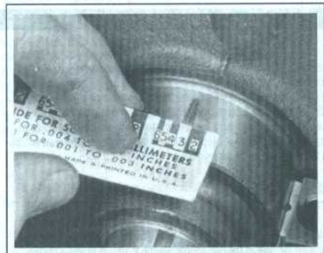
10.21 Use the scale on the Plastigage package to determine the bearing oil clearance - be sure to measure the widest part of the Plastigage and use the correct scale; it comes with both standard and metric scales
