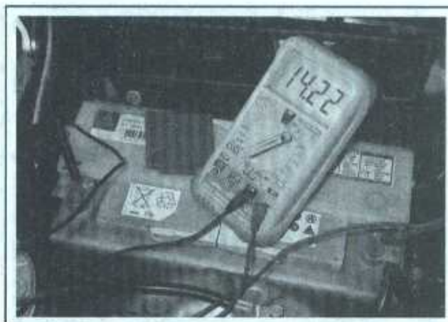
9.3 To test the charging voltage, connect a voltmeter to the battery terminals. A healthy charging system should put out at least 13 volts, but not more than 15 volts
