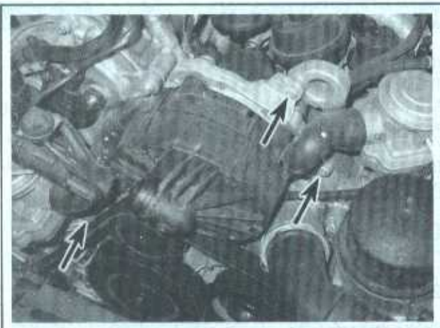
19.25 To detach the air injection pump and mounting bracket from the cylinder head, remove these two upper bolts; to detach it from the timing chain cover, remove this lower bolt (bolt not visible in this photo) (2006 and later V6 models)
