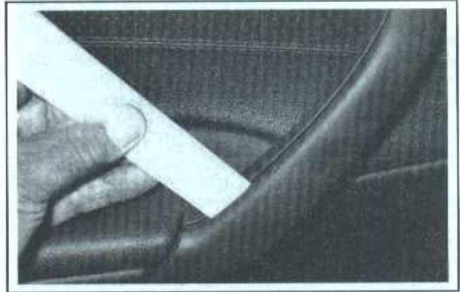
13.1 Pry the grab handle trim away from the door with a trim stick
