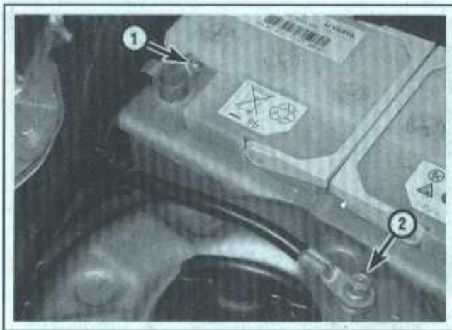
4.10 To remove the battery ground cable, disconnect it from the negative battery terminal (1), then disconnect it from the vehicle body (2)
