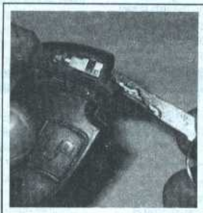
25.3b . . . then insert the mechanical key into the end of the fob and push the lock to release the battery holder
