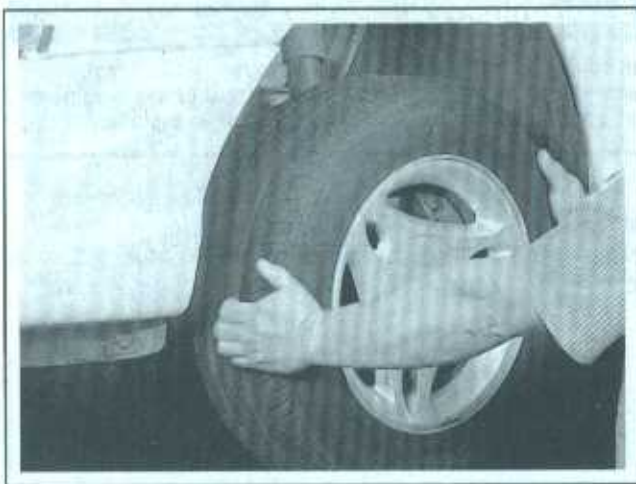
17.11 With the steering wheel in the locked position and the vehicle raised, grasp the front tire as shown and try to move it back-and-forth - if any play is noted, check the steering gear mounts and tie-rod ends for looseness
