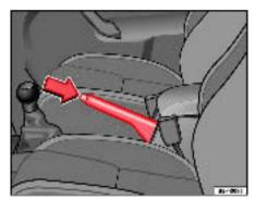
Fig. 144 Handbrake between the front seats
