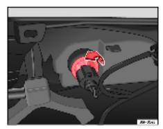
Fig. 194 Lamp on interior side of bumper
