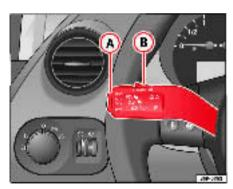
Fig. 148 Turn signal and main beam headlight lever switch and rocker switch for the cruise control
