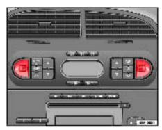
Fig. 95 Thumb wheel for the front seat heating
