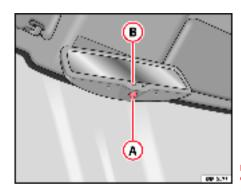
Fig. 89 Automatic antidazzle interior mirror.
