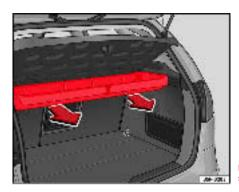
Fig. 125 Removing storage shelf
