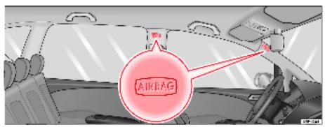
Fig. 24 Location of left curtain airbag
