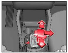
Fig. 142 Changing gear with Tiptronic
