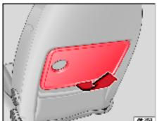
Fig. 103 Folding table of front left seat
