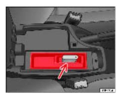
Fig. 120 iPod connection in central armrest compartment.
