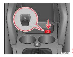
Fig. 118 Auxiliary audio connection
