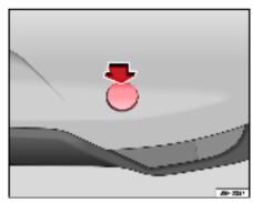
Fig. 207 Cover for towing eve at rear
