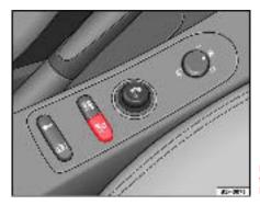
Fig. 48 Central console: tyre monitor system button
