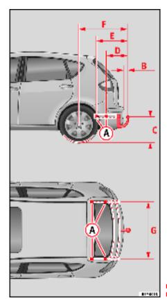
Fig. 158 Attachment points for towing bracket
