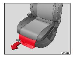
Fig. 102 Stowage area under the front seats
