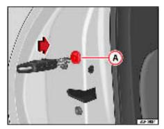
Fig. 59 Locking the doors manually
