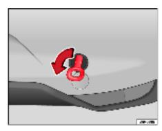
Fig. 208 Fitting the towing eye to the rear of the vehicle
