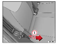
Fig. 97 Rear seat backrest angle adjustment
