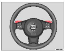
Fig. 143 Steering wheel with levers for automatic gearbox
