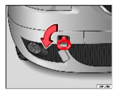
Fig. 203 The front right section of the vehicle: Fitting the front towing
