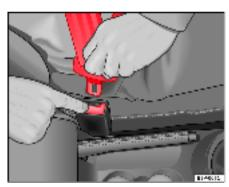
Fig. 16 Removing latch plate from buckle
