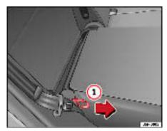
Fig. 99 Folding or opening the front seat
