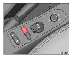
Fig. 134 Detail of the centre console: ESP button
