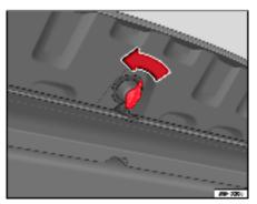
Fig. 123 Opening the storage compartment
