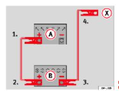
Fig. 202 How to connect the jump leads
