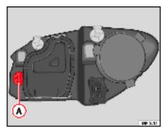
Fig. 183 Turn signal lamps
