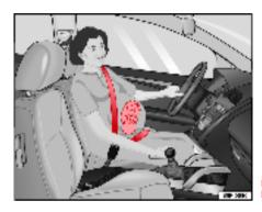
Fig. 15 Positioning seat belts during pregnancy
