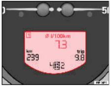
Fig. 40 Digital instrument panel display: average fuel consumption indicator
