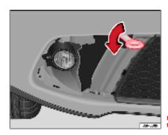
Fig. 206 Attachment for towing eye
