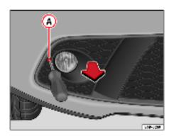
Fig. 205 Access to towing eye housing
