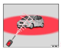
Fig. 65 Range of the remote control
