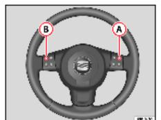
Fig. 58 Steering wheel audio version controls
