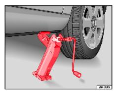
Fig. 177 Fitting the jack
