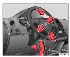
Fig. 132 Adjusting the steering wheel position
