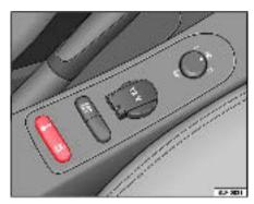
Fig. 60 Detail of the centre console: central locking system button
