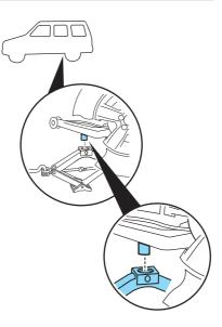
3. Position the jack according to the guides and turn the jack handle clockwise until the tire is a maximum of 1 inch (25 mm) off the ground.
