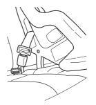
Airbags can kill or injure a child in a child seat. NEVER place a rear-facing child seat in front of an active airbag. If you must use a forward-facing child seat in the front seat, move the vehicle seat all the way back.
