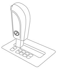
**WARNING:** Always set the parking brake fully and make sure the gearshift is latched in P (Park). Turn the ignition to the off position and remove the key whenever you leave your vehicle.
