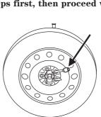
3. Lay the tire on the ground with the valve stem facing down. If your vehicle is equipped with aluminum wheels, remove the wheel ornament.
