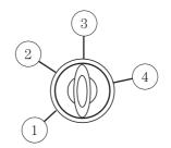
Do not crank the engine for more than 10 seconds at a time as starter damage may occur. If the engine fails to start, turn the key to off and wait 30 seconds before trying again.
