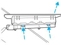
3. Pull the bulb straight out of the socket and push in the new bulb. Install the new bulbs in reverse order.
