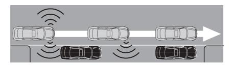
When the system has found a space, the message center will display SPACE FOUND PULL FORWARD followed by a chime. Drive forward until the message center displays SPACE FOUND STOP followed by a chime. When you stop the vehicle in position to begin parking, the message center displays REMOVE HANDS PUT IN REVERSE. The driver should always come to a complete stop before changing gears.
