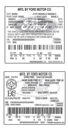
**WARNING:** Exceeding the Safety Compliance Certification Label vehicle weight rating limits could result in substandard vehicle handling or performance, engine, transmission and/or structural damage, serious damage to the vehicle, loss of control and personal injury.
