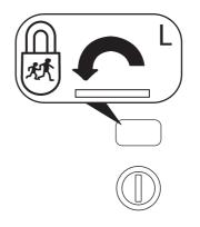
Insert the key and turn in the direction of arrow shown on the door to engage the child proof lock. Turn in the opposite direction to disengage childproof locks.
