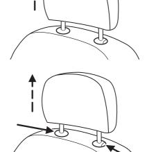
2. Simultaneously press and hold both the adjust/release button and the unlock/remove button, then pull up on the head restraint.
