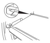
**WARNING:** Ensure that the posts are properly latched in mounting features. The cover may cause injury in a sudden stop or accident if it is not securely installed.
