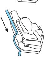
3. While holding the shoulder and lap belt portions together, route the tongue through the child seat according to the child seat manufacturer's instructions. Be sure the belt webbing is not twisted.
