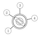
4. Start— cranks the engine. Release the key as soon as the engine starts.
