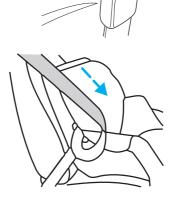
6. Allow the belt to retract to remove slack. The belt will click as it retracts to indicate it is in the automatic locking mode.7. Try to pull the belt out of the retractor to make sure the retractor is in the automatic locking mode (you should not be able to pull more belt out). If the retractor is not locked, repeat Steps 5 and 6.
