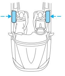
The airbag SRS is designed to activate when the vehicle sustains lateral deceleration sufficient to cause the sensors to close an electrical circuit that initiates airbag inflation.
