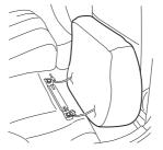
Attach the safety belt web snap button to the quarter trim panel snap button. This will ensure that safety belt does not get caught by staying out of the seat back folding path.
