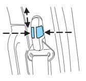
**WARNING:** Position the safety belt height adjusters so that the belt rests across the middle of your shoulder. Failure to adjust the safety belt properly could reduce the effectiveness of the safety belt and increase the risk of injury in a collision.
