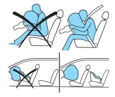
**WARNING:** All occupants of the vehicle, including the driver, /!\ should always properly wear their safety belts, even when an air bag supplemental restraint system (SRS) is provided.
