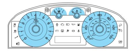
Speedometer: Indicates the current vehicle speed.
