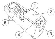
5. Small storage trays and (if equipped) an ambient light control switch.
