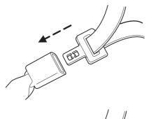
2. To unfasten, press the release button and remove the tongue from the buckle.
