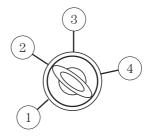
3. Turn the ignition to the 1 (off) position and remove the first  ${\bf coded}$   ${\bf key}$  from the ignition.
