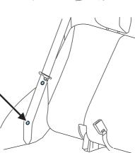
4. To release seatback, pull the seatback release lever (on top of seat) toward the front seat. This is common for both 60% and 40% seatbacks.
