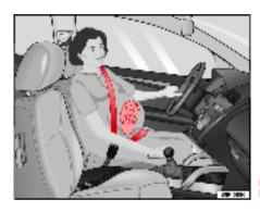
Fig. 14 Positioning seat belts during pregnancy
