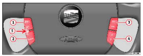
Fig. 53 Multi-function steering wheel with controls:
