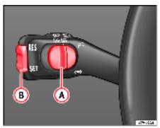
Fig. 132 Turn signal and main beam headlight lever control (A) and rocker switch (B) for cruise control
