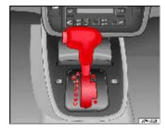
Fig. 129 Centre console: gearbox selector lever with locking button
