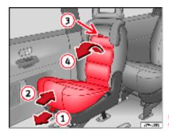
Fig. 35 Using the integrated child seat
