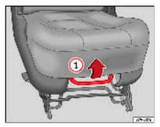
Fig. 89 Adjustment of the seat forwards and backwards
