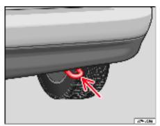
Fig. 173 Rear towline anchorage
