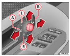
Fig. 82 Detail of driver door: wing mirror controls
