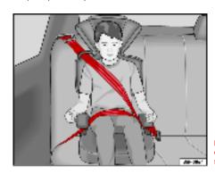
Fig. 32 Forward-facing child seat installed on rear
