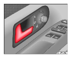
Fig. 58 Driver's door release lever in normal position
