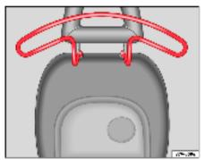
Fig. 107 Clothes hangers on the front seat
