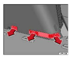
Fig. 120 Air outlets for heating the passenger compartment
