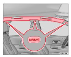
Fig. 26 Location of left curtain airbag
