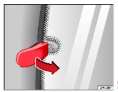
Fig. 65 Release lever for mechanical vent wing
