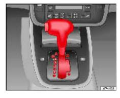
Fig. 127 Centre console: selector lever of the automatic gearbox with locking button
