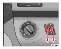
Fig. 71 Instrument panel: headlight range control (1) and illumination of instruments and switches
