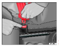
Fig. 16 Removing latch plate from buckle
