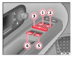
Fig. 64 Detail of driver door: buttons for front and rear electric windows
