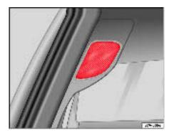
Fig. 62 Interior monitoring system sensor
