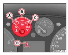
Fig. 45 Instrument panel: engine coolant temperature gauge
