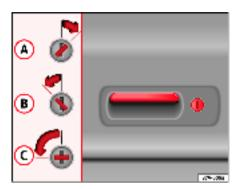
Fig. 63 Key slot positions of tailgate lock
