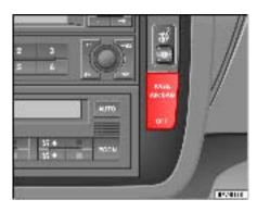
Fig. 29 Warning lamp for disabling airbag in dash panel
