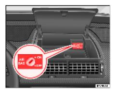
Fig. 28 Interior of centre compartment on instrument panel: Key switch for switching off the front passenger airbags
