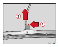
Fig. 146 Changing a rear wiper blade
