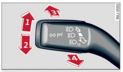
Fig. 58 Turn signal and high beam lever
