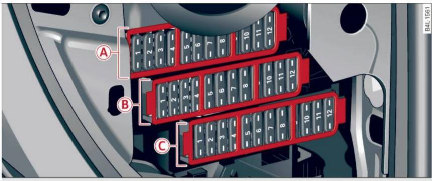
Fig. 258 Right cockpit: fuse panel with plastic clip
