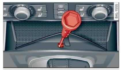
Fig. 163 Emergency release for selector lever
