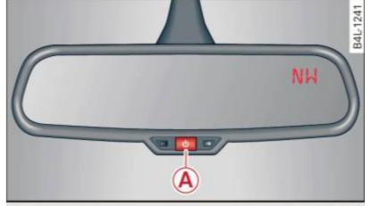
Fig. 72 Inside rear view mirror: digital compass activated
