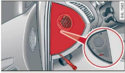
Fig. 255 Left cockpit: fuse panel cover
