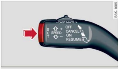
Fig. 129 Control lever: Storing speed
