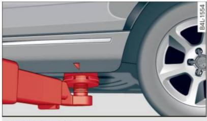
Fig. 268 Rear lifting point
