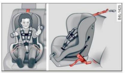
Fig. 205 Schematic overview: installation of the attachments applicable to a LATCH seat
