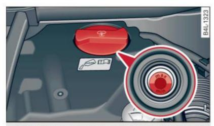
Fig. 233 Engine compartment: Coolant expansion tank
