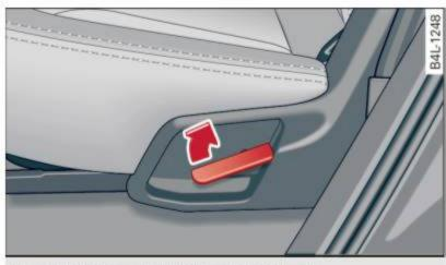
Fig. 86 Release lever for outer seatback
