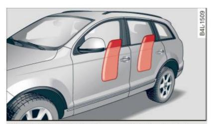
Fig. 201 Inflated side airbags on left side of vehicle, rear side airbag optional equipment
