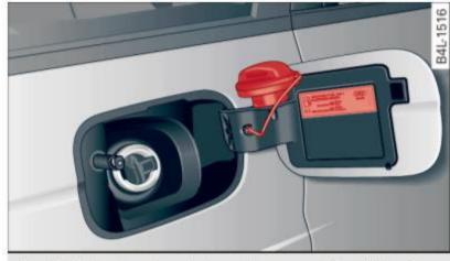
Fig. 221 Fuel cap hooked on the opened fuel filler flap
