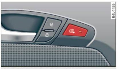
Fig. 149 Driver's door: Side assist button
