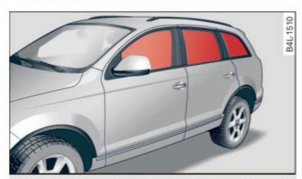
**Fig. 203** Illustration of principle: Inflated side curtain airbags on the left side
