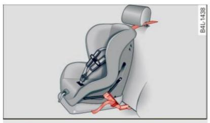
Fig. 216 Tether strap: proper routing and mounting
