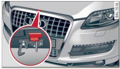
Fig. 228 Release lever under the engine hood
