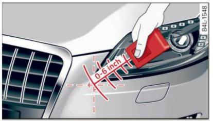
Fig. 180 Front bumper, driver side: location of transmitter unit
