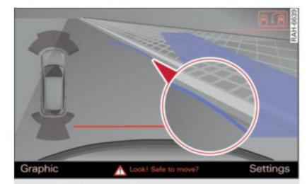
Fig. 173 MMI display: Blue curve on the curb
