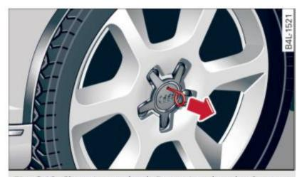
Fig. 249 Changing a wheel: Removing the wheel cover
