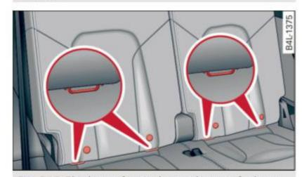
Fig. 210 Third row of seats: locator buttons for lower anchorages
