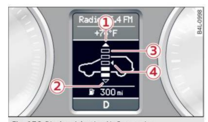
Fig. 176 Display: Adaptive Air Suspension
