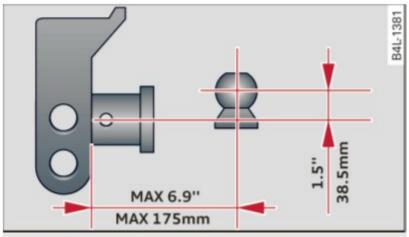
Fig. 219 Permitted ball position of the trailer hitch
