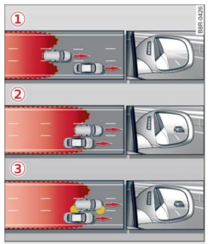
Fig. 154 Side assist: Vehicles dropping back quickly
