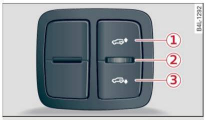
Fig. 178 Luggage compartment detail: Cargo mode switch
