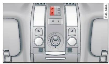
Fig. 51 Section of front headliner: Switch for sunshade
