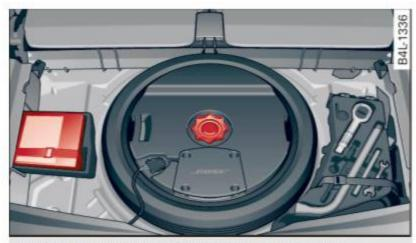
Fig. 248 Inflatable spare tire with compressor
