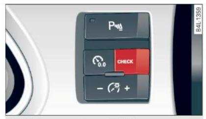
Fig. 24 Instrument cluster: CHECK button
