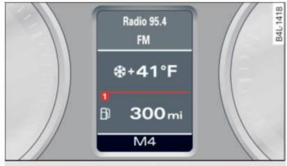
Fig. 161 Display: manual shift program, selected gear
