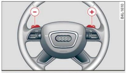
Fig. 162 Steering wheel: Shift buttons
