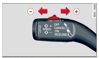
Fig. 133 Control lever: Setting distance
