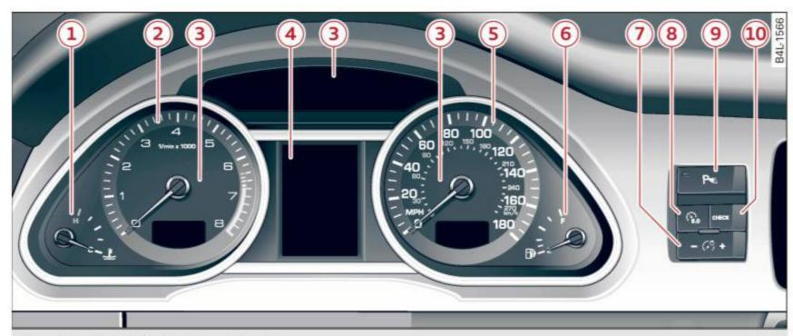
Fig. 3 Overview of the instrument cluster
