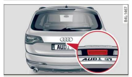
Fig. 38 Position of handle in the rear lid
