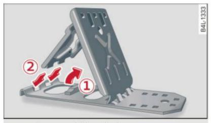
Fig. 246 Opening folding chocks
