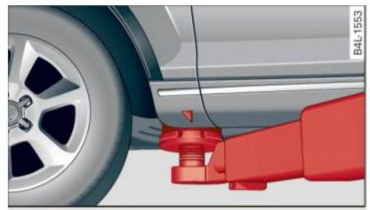
Fig. 267 Front lifting point
