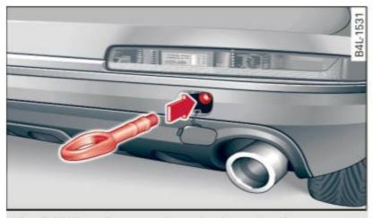
Fig. 265 Rear bumper: Screwing in towing loop
