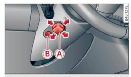
Fig. 118 Switch for steering wheel adjustment
