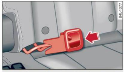
Fig. 212 Close-up: fitting the guidance fixture over the lower anchorage bracket
