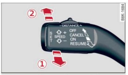
Fig. 128 Control lever: Switching on and off
