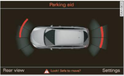
Fig. 169 MMI display: visual distance display
