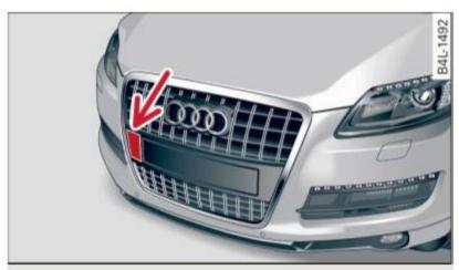
**Fig. 126** Front bumper: Position of radar sensor (not visible from outside)
