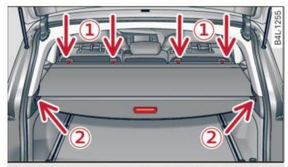
Fig. 90 Luggage compartment: compartment cover closed
