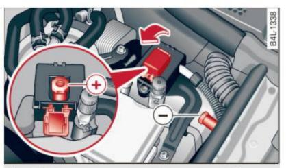
**Fig. 260** Engine compartment: Connectors for jumper cables and charger
