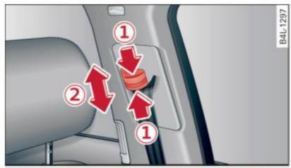
Fig. 195 Safety belt height adjustment – loop-around fittings
