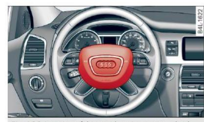
Fig. 196 Location of driver airbag: in steering wheel
