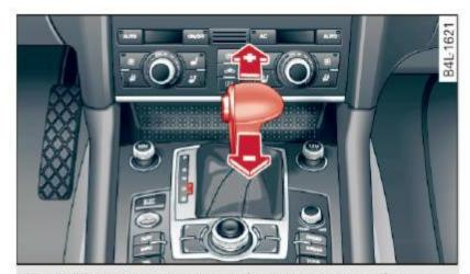
Fig. 160 Center console: shifting the tiptronic® manually
