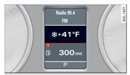
Fig. 11 Display: outside temperature
