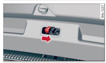
**Fig. 42** Section of the luggage compartment: Emergency release
