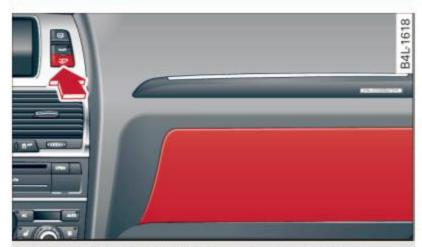
Fig. 102 Unlocking button for glove compartment
