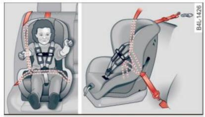
Fig. 206 Schematic overview: installation of the seat using the vehicle's safety belt system
