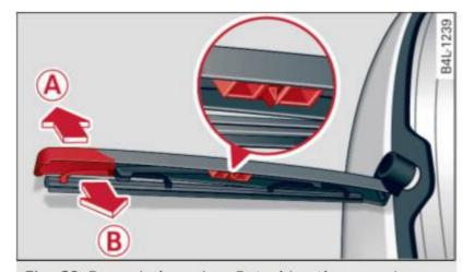
Fig. 69 Rear window wiper Detaching the rear wiper blade
