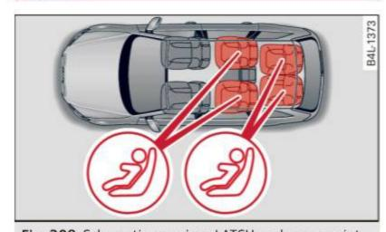
Fig. 208 Schematic overview: LATCH anchorage point locations
