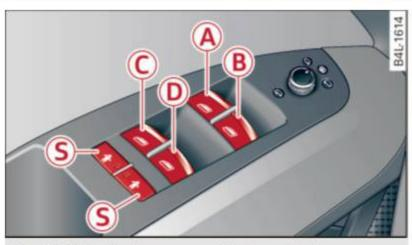
Fig. 46 Driver's door: power window switches
