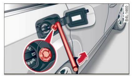
Fig. 225 Right rear vehicle side: removing the AdBlue cap
