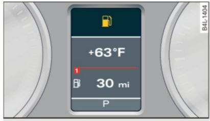
Fig. 26 Display: low fuel level warning (priority 2)
