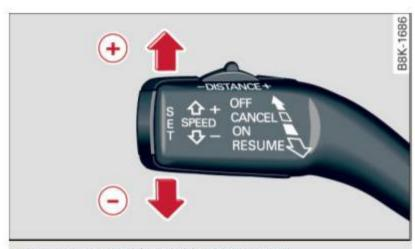
Fig. 130 Control lever: Changing speed
