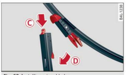
Fig. 68 Installing wiper blades
