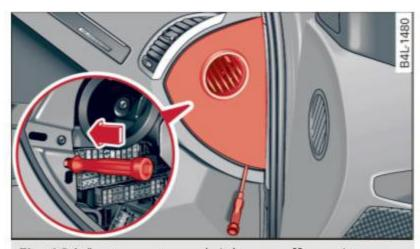
Fig. 104 Instrument panel right: pry off security cover
