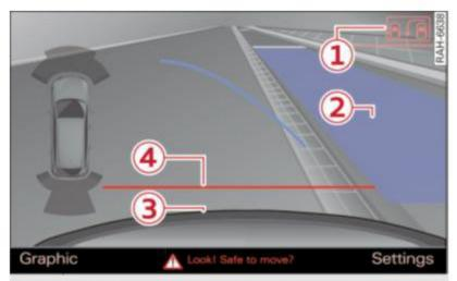
Fig. 172 MMI display: blue surface in the parking spot
