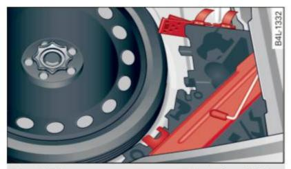
Fig. 245 Luggage compartment vehicle jack and folding chocks
