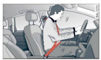
Fig. 190 Driver is correctly restrained in a sudden braking maneuver
