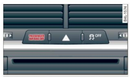
**Fig. 199** Section from the instrument panel: PASSENGER AIR BAG OFF light
