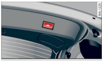
Fig. 40 Locking switch in the rear lid
