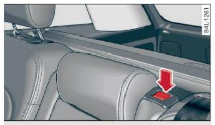
Fig. 87 Release lever for center seatback
