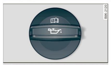
**Fig. 232** Engine compartment: cover on the engine oil filler neck
