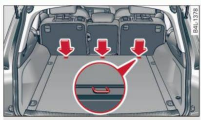
Fig. 214 Tether anchors for second row of seats: attachment hook locations
