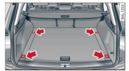
Fig. 88 Location of the tie-down rings in the luggage compartment
