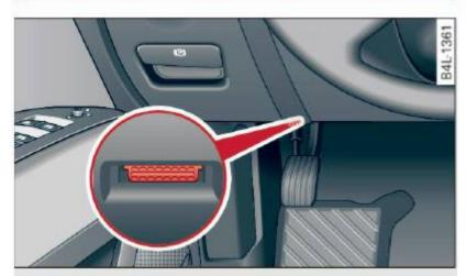
Fig. 22 Location of Data Link Connector (DLC)
