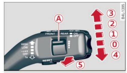
Fig. 65 Windshield wiper lever
