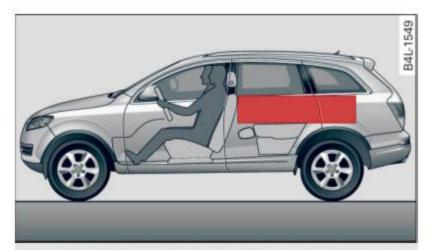
**Fig. 184** Safe load positioning: place heavy objects as low and as far forward as possible.
