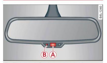
Fig. 71 Automatic dimming rearview mirror\*
