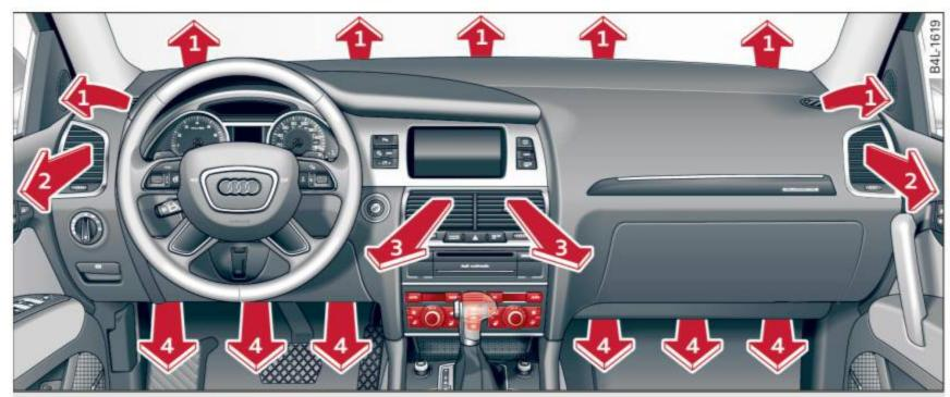
Fig. 112 Instrument panel: air outlet locations and airflow directions
