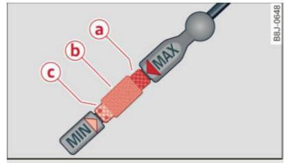
Fig. 231 Illustration of principle 2: Markers on oil dipstick
