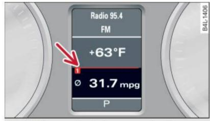
Fig. 17 Trip computer display: memory level 1
