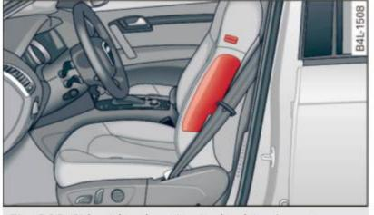
Fig. 200 Side airbag location in the driver's seat
