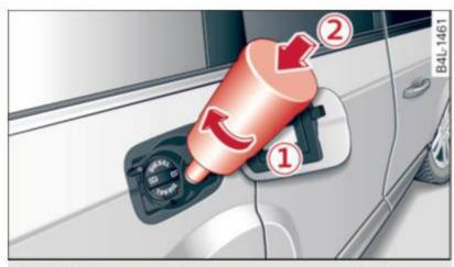
Fig. 226 AdBlue filler tube: inserting the refill bottle
