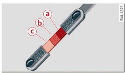
Fig. 230 Illustration of principle 1: Markers on oil dipstick
