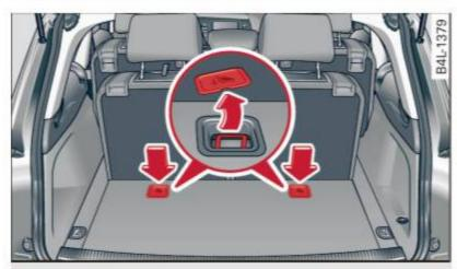
Fig. 215 Tether anchors for third row of seats: attachment hook locations
