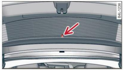
Fig. 64 Sun shade pulled up on the rear lid window
