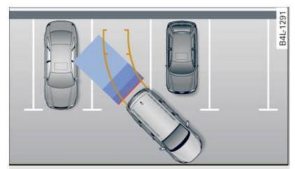
Fig. 164 Parking mode 1: Backing into a parking space
