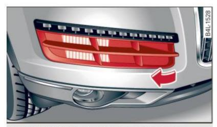
Fig. 262 Right front bumper: Removing the cover
