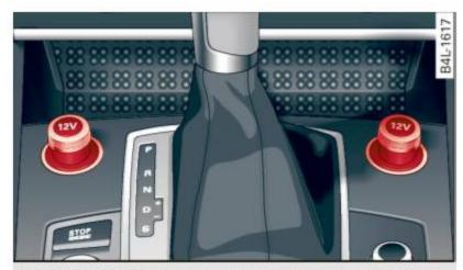
Fig. 100 Section from center console: 12-volt outlets
