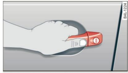
Fig. 44 Convenience key: unlocking vehicle door
