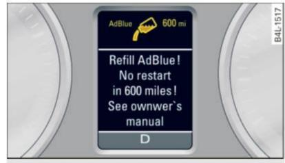
Fig. 224 Instrument cluster: indicator in the display
