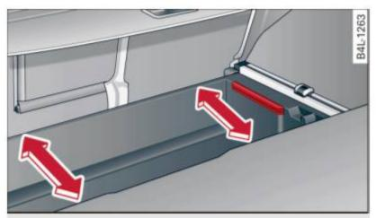
Fig. 93 Removing the cargo floor
