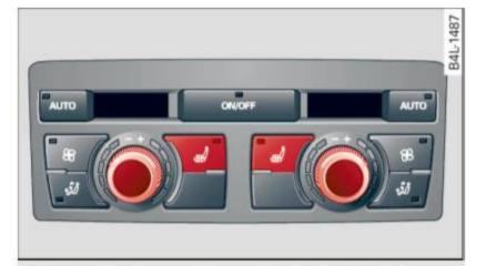
Fig. 115 Center console rear: Seat heating with fourzone automatic comfort air conditioning\*
