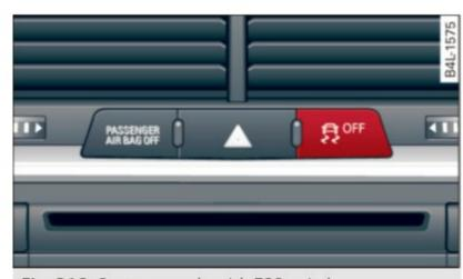
Fig. 218 Center console with ESC switch
