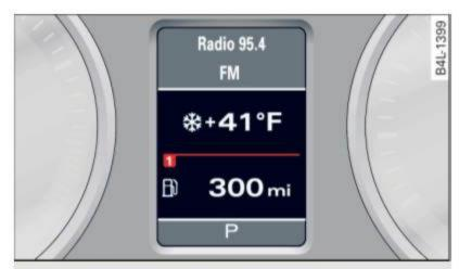
Fig. 9 Instrument cluster: center display
