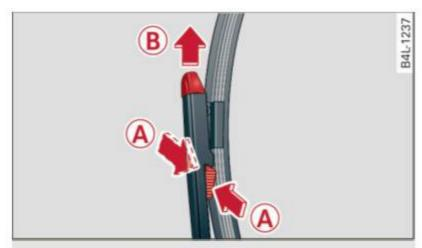
Fig. 67 Removing the wiper blades
