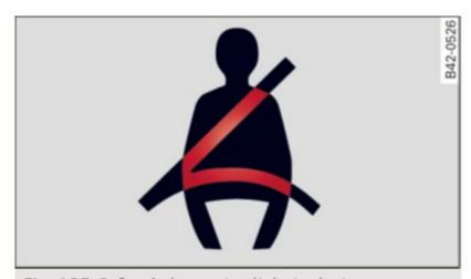
**Fig. 185** Safety belt warning light in the instrument cluster - enlarged
