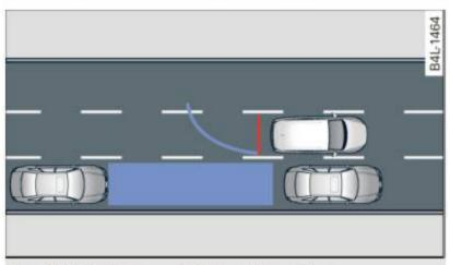
Fig. 165 Parking mode 2: parallel parking
