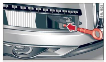
**Fig. 263** Right front bumper without cover: Screwing in towing loop
