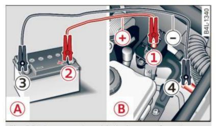
**Fig. 261** Jump starting with the battery of another vehicle: A – booster battery, B – discharged vehicle battery
