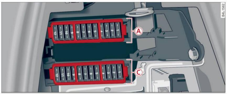
Fig. 259 Right luggage compartment: fuse panel with plastic clip
