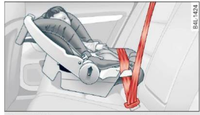
Fig. 204 Schematic overview: rearward-facing infant seat, properly installed on the rear seat
