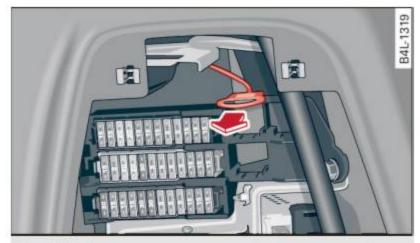
Fig. 223 Luggage compartment: Emergency opening of fuel filler flap
