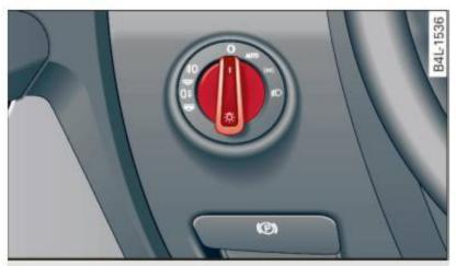
Fig. 53 Instrument panel: light switch
