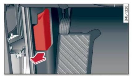
Fig. 227 Driver's side footwell: engine hood release lever
