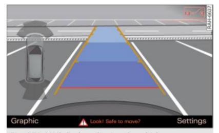
Fig. 171 MMI display: aligning the vehicle
