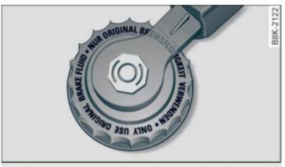
Fig. 234 Engine compartment: cover on the brake fluid reservoir
