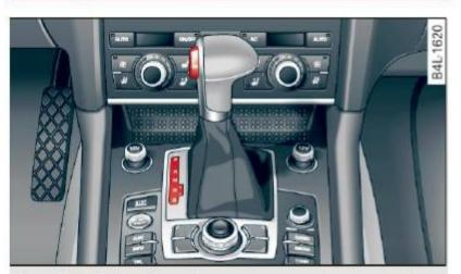
**Fig. 157** Shift gate on the center console: selector lever with release button
