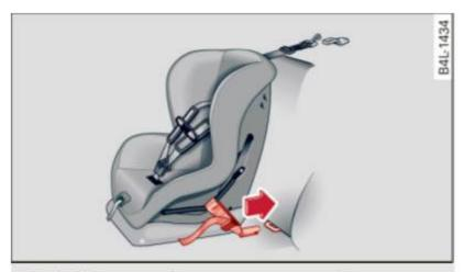
Fig. 213 Lower anchorages: proper mounting
