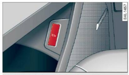
Fig. 39 Driver's door: Unlocking the rear lid
