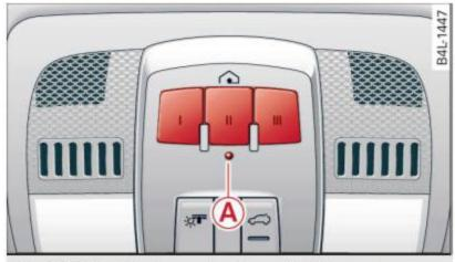
Fig. 181 Overhead console: HomeLink® keypad
