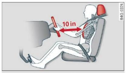
Fig. 182 Correct seating position
