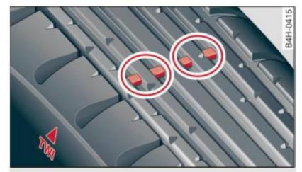
Fig. 239 Tire tread: tread wear indicators (TWI)
