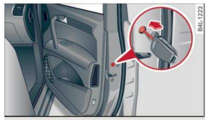
Fig. 36 Emergency locking of the front passenger's door
