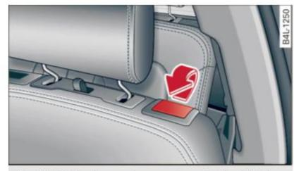
Fig. 78 Seatback second row seating: Seatback latch
