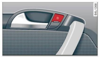
Fig. 35 Rear doors: power locking switch
