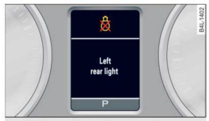
Fig. 14 Display: defective light bulb warning
