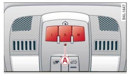
Fig. 179 Overhead console: HomeLink® keypad
