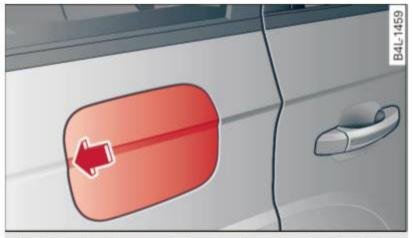
Fig. 220 Right rear vehicle side: Opening the fuel filler flap
