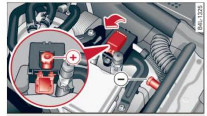
Fig. 235 Engine compartment: Connectors for charger and jumper cables
