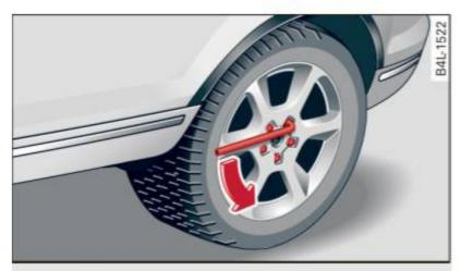
Fig. 251 Changing a wheel: loosening the wheel bolts
