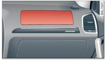
Fig. 197 Location of front passenger's airbag: in the instrument panel
