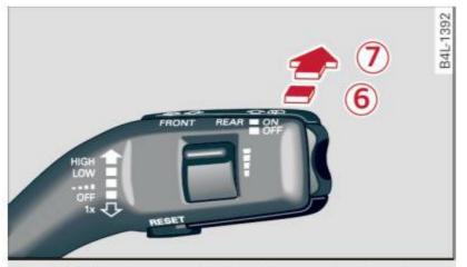
Fig. 66 Wiper lever: activating the rear window wiper and washer
