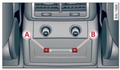
Fig. 114 Center console rear: Heated seats
