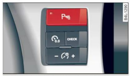
Fig. 168 Center console: Parking system switch
