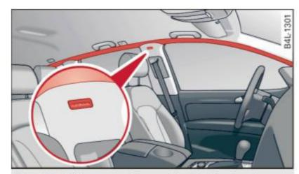
Fig. 202 Side curtain airbags, driver's side: location
