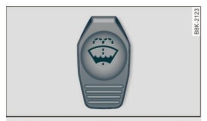
Fig. 236 Engine compartment: cover on the windshield and headlight\* washer fluid reservoir
