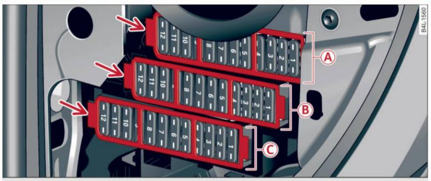
Fig. 257 Left cockpit: fuse panel with plastic clip
