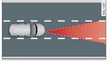
**Fig. 127** Basic principle diagram: Radar sensor measurement range
