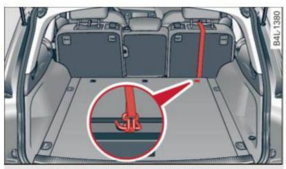
Fig. 217 Tether strap for second row seats: proper routing and mounting
