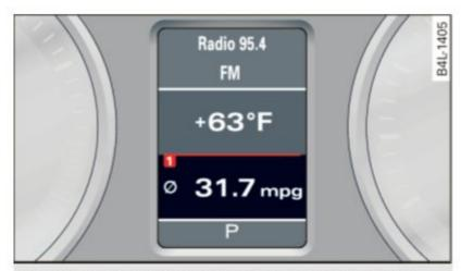
Fig. 16 Trip computer display: Average fuel mileage
