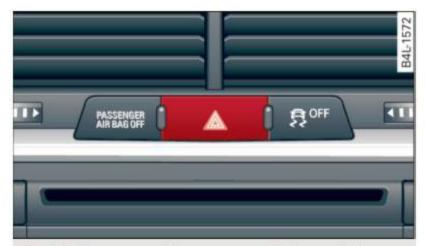
Fig. 57 Center console: emergency flasher switch
