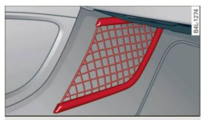
Fig. 108 Storage net in passenger's footwell
