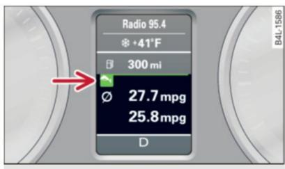
Fig. 19 Display: efficiency program
