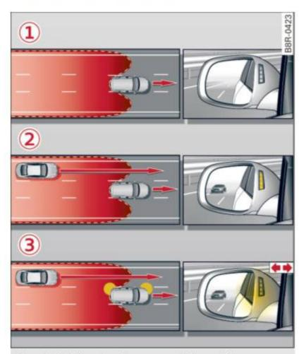
Fig. 151 Side assist: Fast approaching vehicles
