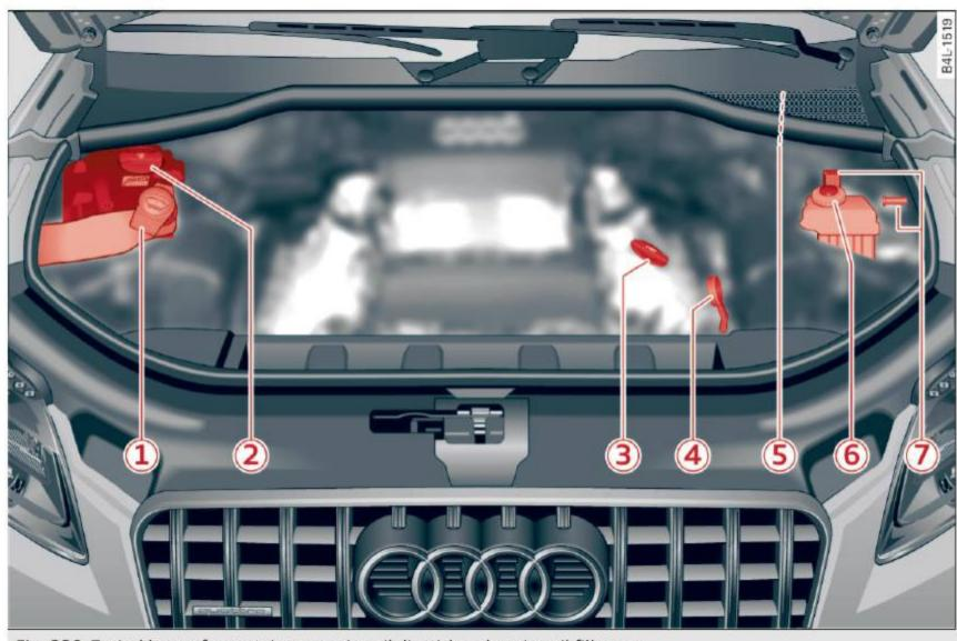
Fig. 229 Typical layout for containers, engine oil dipstick and engine oil filler cap
