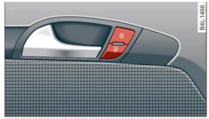
Fig. 34 Front doors: power locking switch
