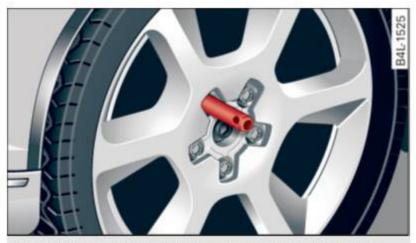
Fig. 254 Changing a wheel: alignment pin inside the top hole
