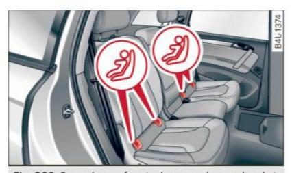
Fig. 209 Second row of seats: lower anchorage bracket locations
