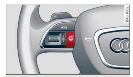
Fig. 116 Steering wheel: button for steering wheel heating
