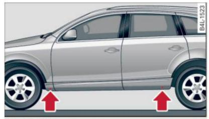
Fig. 252 Sill panels: markings
