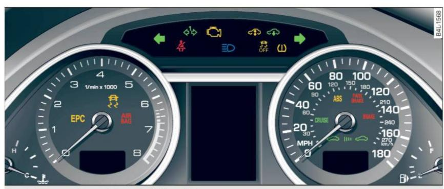
Fig. 8 Instrument cluster with warning/indicator lights
