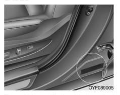
The vehicle certification label attached on the driver's side center pillar contains the vehicle identification number (VIN).
