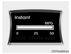
Instant fuel consumption (MPG or 1/100km) This mode calculates the instant fuel consumption every 2 seconds (supervision type: every 0.2 second) from the driving distance and quantity of fuel injection.
