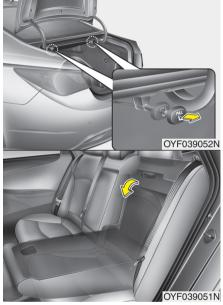
5. Pull on the seatback folding lever located in the trunk, then fold the seat toward the front of the vehicle.
