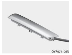
11. Remove the high mounted stop lamp after removing screws.
