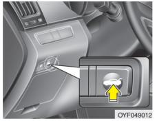
• To open the trunk from inside the vehicle, press the trunk lid release button. Once the trunk is opened and then closed, the trunk is locked automatically.
