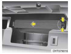
Remove the climate control air filter cover while pressing the lock on the right of the cover.
