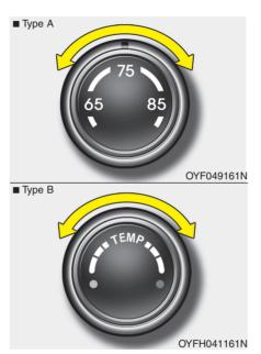
2. Turn the temperature control knob to set the desired temperature.
