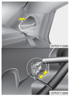
Take the C-pillar out carefully. If you pull the C-pillar strongly, it will be broken.
