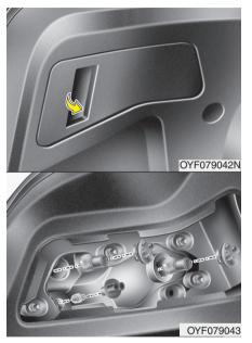
Rear turn signal, stop and tail light, side marker
