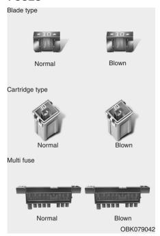
A vehicle's electrical system is protected from electrical overload damage by fuses.
