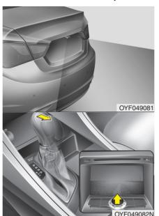
The rearview camera will activate when the back-up light is ON with the ignition switch ON and the shift lever in the R position.
