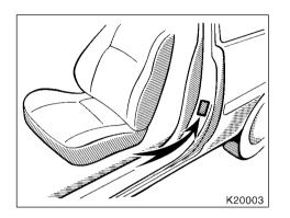
The vehicle identification number (VIN) is also on the Certification Label.
