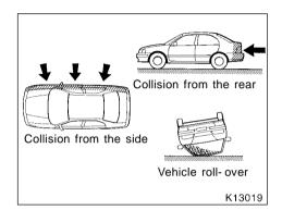
The SRS airbag is not designed to inflate if the vehicle is subjected to a side or rear impact, if it rolls over, or if it is involved in a low-speed frontal collision.
