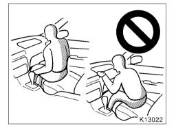
► Do not sit on the edge of the seat or lean over the dashboard when the vehicle is in use. The airbags inflate with considerable speed and force; you may be killed or seriously injured. Sit up straight and well back in the seat, and always use your seat belt.
