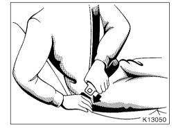
Adjust the seat as needed (front seats only) and sit up straight and well back in the seat. To fasten your belt, pull it out of the retractor and insert the tab into the buckle.
