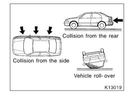
The SRS airbags are not designed to inflate if the vehicle is subjected to a side or rear impact, if it rolls over, or if it is involved in a low-speed frontal collision.
