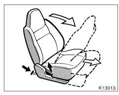
After putting back the seat, try pushing the seat forward and rearward to make sure it is secured in place.
