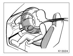
The SRS (Supplemental Restraint System) airbag is designed to provide further protection for the driver when added to the primary protection provided by the seat belt.
