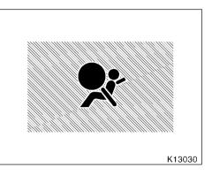
This indicator comes on when the ignition key is turned to the "ACC" or "ON" position. It goes off after about 6 seconds. This means the SRS airbag is operating properly.
