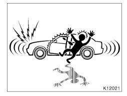
To deter the vehicle theft, the system is designed to give an alarm and keep the engine from being started if any of the doors, trunk or hood is forcibly unlocked or the battery terminal is disconnected and then reconnected when the vehicle is locked.
