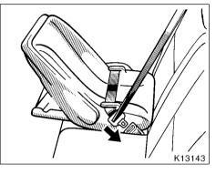
1. Run the lap and shoulder belt through or around the infant seat following the instructions provided by its manufacturer and insert the tab into the buckle taking care not to twist the belt. Keep the lap portion of the belt tight.
