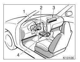
The SRS airbag system mainly consists of the following components and their locations are shown in the illustration.
