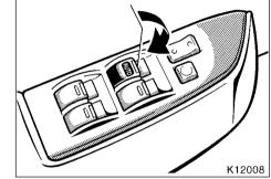
The windows can be operated with the switch on each door.
