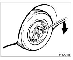
9. Lower the vehicle completely and tighten the wheel nuts.
