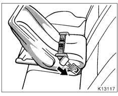
1. Run the center lap belt through or around the infant seat following the instructions provided by its manufacturer and insert the tab into the buckle taking care not to twist the lap belt.
