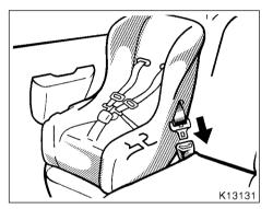
1. Run the lap and shoulder belt through or around the convertible seat following the instructions provided by its manufacturer and insert the tab into the buckle taking care not to twist the belt. Keep the lap portion of the belt tight.
