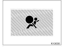
This SRS airbag system has a service reminder indicator to inform the driver of operating problems. If either of the following conditions occurs, this indicates a malfunction of the airbag. Contact your Toyota dealer as soon as possible to service the vehicle.
