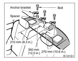
To comply with Canada Motor Vehicle Safety Standards, vehicles sold in Canada are provided with a bracket set in the glovebox, designed for use with any of the 3 anchor locations shown in the illustration.
