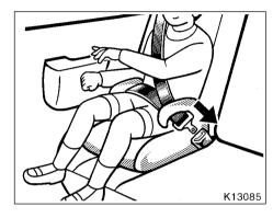
1. Sit the child on a booster seat. Run the lap and shoulder belt through or around the booster seat and child following the instructions provided by its manufacturer and insert the tab into the buckle taking care not to twist the belt.
