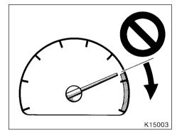
The tachometer indicates engine speed in thousands of rpm<sup>[2]</sup>(revolutions per minute). Use it while driving to select correct shift points and to prevent engine lugging and overrevving.
