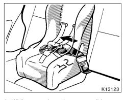
2. While pressing the convertible seat firmly against the seat cushion and seatback, tighten the lap belt by pulling its free end to hold the convertible seat securely.
