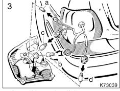
a: Rear side marker light b: Rear turn signal light c: Stop and tail light d: Back-up light
