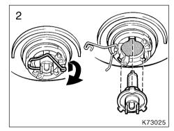
2. Release the bulb retaining spring and remove the bulb. Install a new bulb and the bulb retaining spring.
