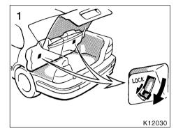
This system deactivates the lock release lever so that things locked in the trunk can be protected.
