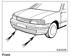
(c) Towing with sling type truck
