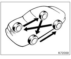
To equalize tire wear and help extend tire life, Toyota recommends that you rotate your tires approximately every 12000 km (7500 miles). However, the most appropriate timing for tire rotation may vary according to your driving habits and road surface conditions.
