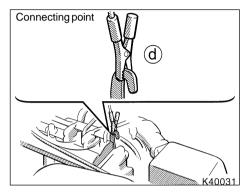
Do not connect it to or near any part that moves when the engine is cranked.
