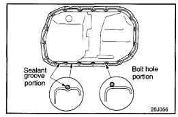
Note the difference in bolt lengths at the location shown.Install the oil pan and tighten the bolts to the specified torque.
