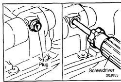
10. Remove the oil pump driven gear and left counter balance shaft retaining bolt.
