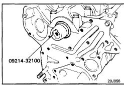
4. Install the front case assembly through a new front case gasket and temporarily tighten the flange bolts (other than those for tightening the filter bracket).
