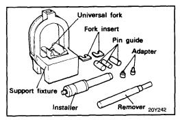
Insert the proper removal tool through the hole in the arch of the tool.
