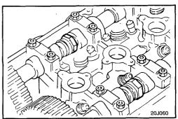
8. Install the rocker cover. Apply sealant as shown.
