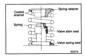
**4.** Using the special tool, Valve Spring Compressor (09222-28000, 09222-28100), remove the retainer lock. Next remove the spring retainer, valve spring, spring seat and valve.
