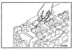
Check the cylinder head gasket surface for flatness by using a straight edge in the direction of A, B, ... as shown.
