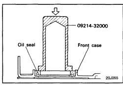
3. Set the special tool (09214-32100) on the front end of crankshaft and apply a thin coat of engine oil to outer circumference of the special tool to install the front case.
