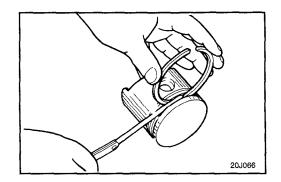
To measure the piston ring end gap, insert a piston ring into the cylinder bore. Position the ring at right angles to the cylinder wall by gently pressing it down with a piston. Measure the gap with a feeler gauge. If the gap exceeds the service limit, replace the piston ring.
