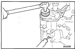
13. Install the camshaft sprocket and tighten the bolt to the specified torque.
