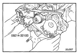
5. Install the front case assembly with a new gasket, and tighten the bolts to the specified torque.
