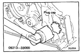
Remove the left side cylinder block plug and insert a screwdriver with an 8 mm (0.32 in.) diameter shaft into plug hole.
