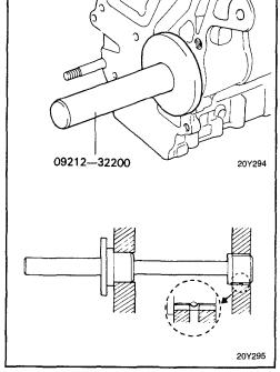
6. Using special tool, install the right counter balance shaft front bearing to the cylinder block.
