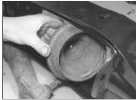
15.4 . . . and rubber cone spring
