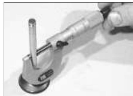
8.17 Measuring the valve stem diameter
