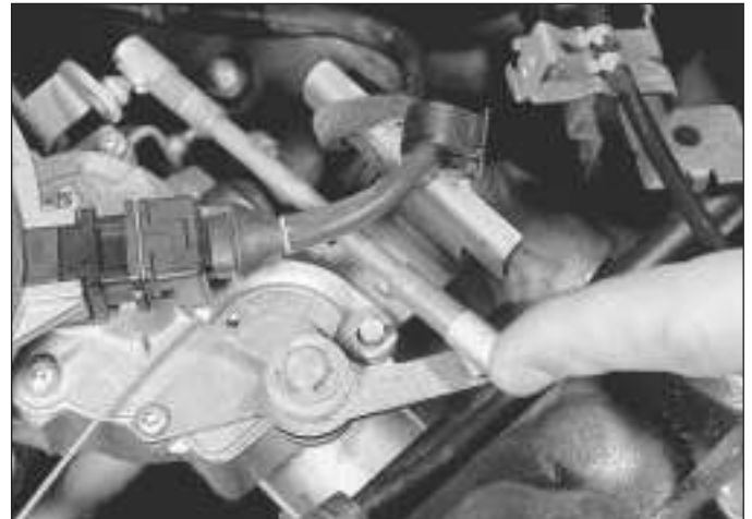
4.9 To adjust the accelerator cable, index the stepper motor . . .
