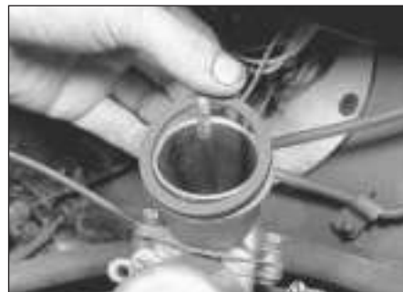
2.2b Recover the sealing ring
