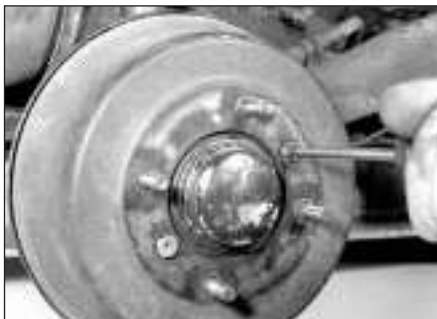
4.2c Remove the brake drum retaining screws . . .
