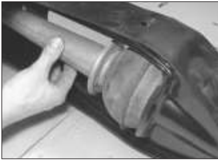
15.3 Remove the rear rubber cone spring strut . . .
