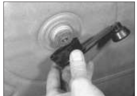
6.2b . . . and the window regulator handle
