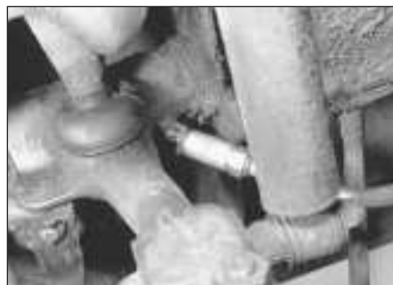
16.1b . . . the upper suspension arm inner pivot grease nipple . . .
