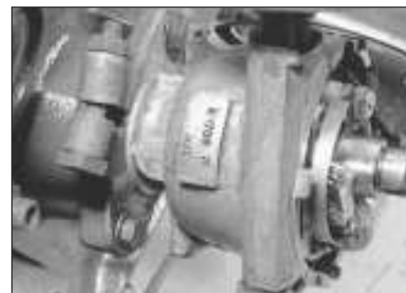
13.6 The distributor number is stamped on the body below the vacuum unit
