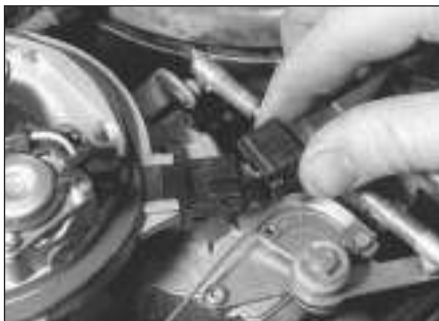
13.12 Disconnecting the injector housing wiring connector
