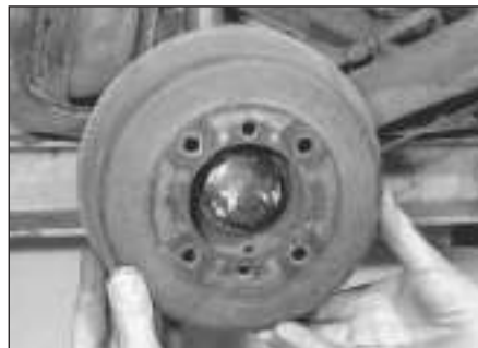
4.3 . . . and withdraw the drum
