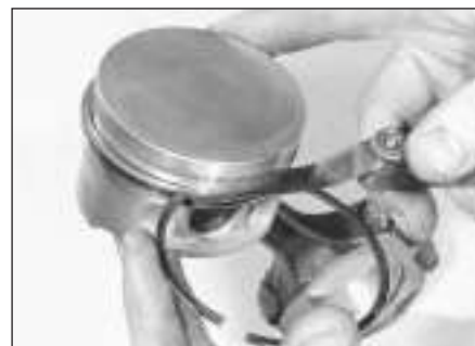
11.17 Measuring the piston ring-to-groove clearance
