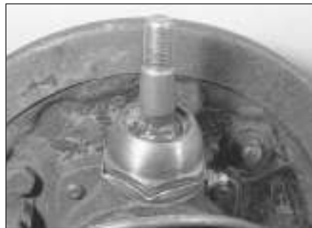
5.12d Bend up the lockwasher ...
