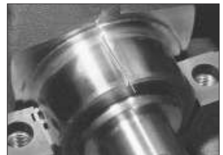
17.7 Plastigage in place on main bearing journal
