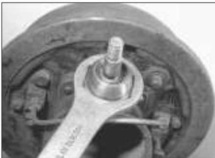
5.12c ... and fully tighten the nut
