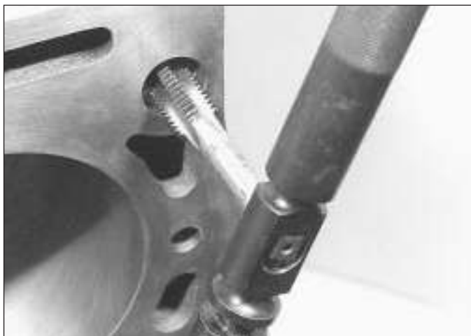
13.7 Using a tap to restore cylinder block threads
