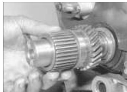
5.30 Slide on the primary gear ...
