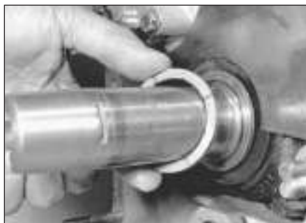
5.29 Position the primary gear thrustwasher on the crankshaft
