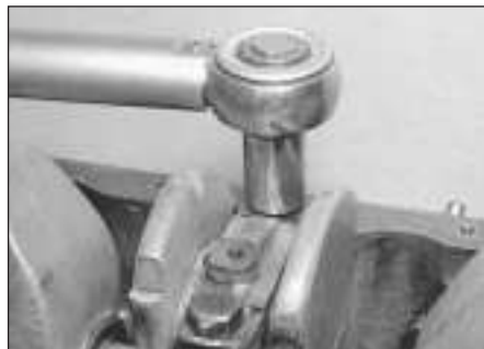
17.22 Tighten the main bearing cap bolts to the specified torque
