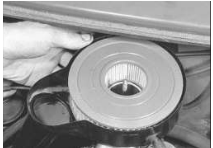
2.2a If the air cleaner is retained by a single wing nut, lift off the top cover and withdraw the air cleaner body from the carburettor
