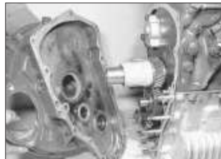
5.35 Refitting the flywheel housing
