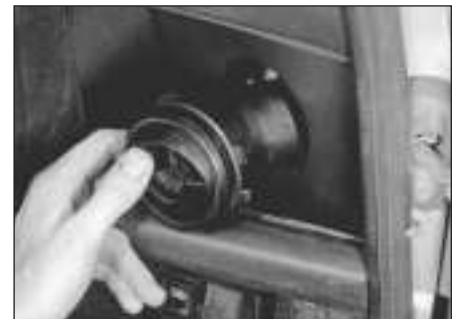
13.2 Turn the air vent anti-clockwise to remove
