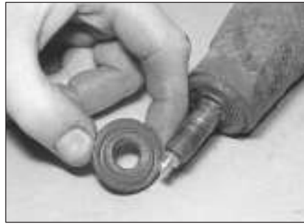
19.12b . . . and thrustwasher . . .
