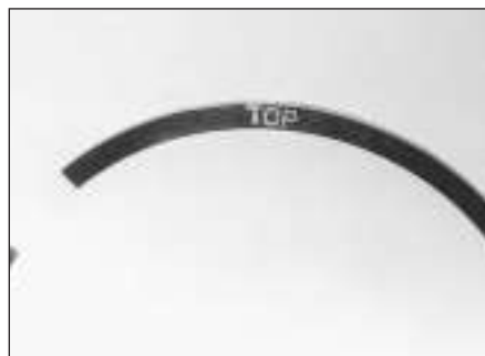
16.3 Piston ring identification markings
