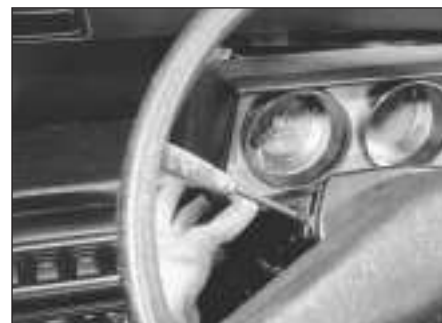
15.25 Remove the instrument cluster nacelle
