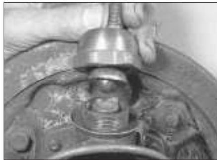
5.12a Refit the ball-pin and nut ...
