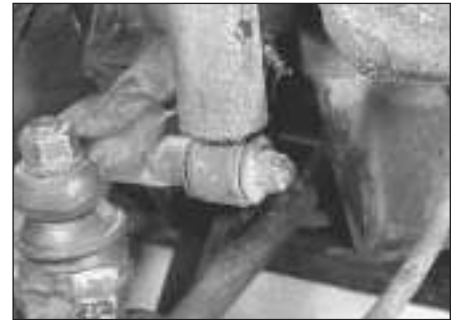
11.2b ... and lower mounting
