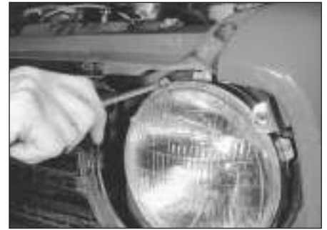
5.4a Unscrew the inner rim securing screws . . .
