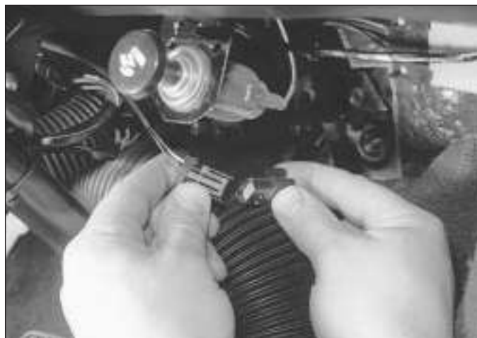
13.47 Disconnect the wiring connector . . .
