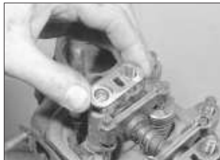
7.15a Recover the pedestal plate (where fitted) . . .
