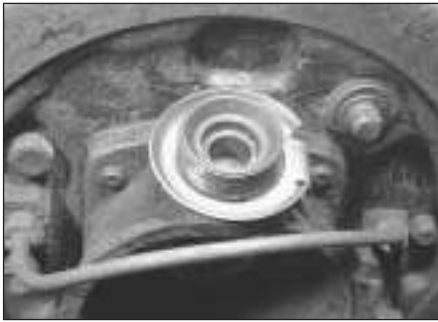
5.11a Fit the lockwasher ...
