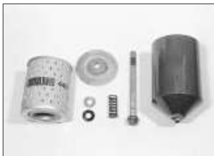
13.9 Components of the cartridge type oil filter
