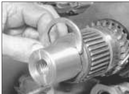
5.31b ... and the C-shaped washer
