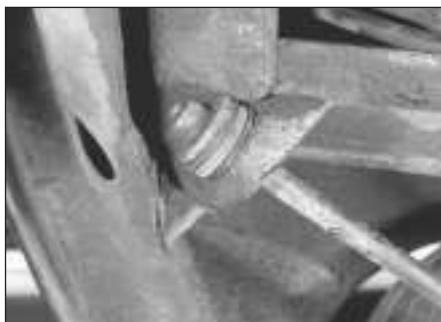
7.2 Tie-bar front mounting
