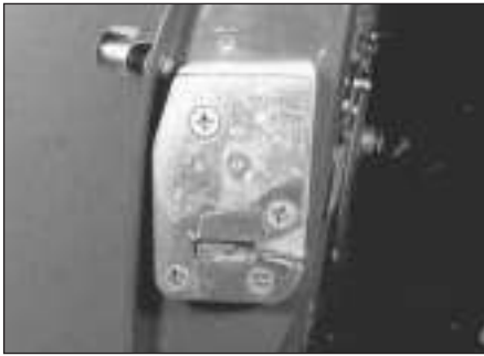
10.4 ... and the door lock retaining screws
