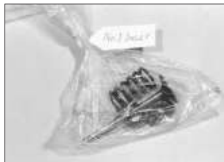
8.6 Keep all valve components together in a labelled plastic bag
