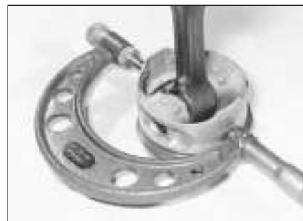
11.16 Measuring the piston diameter
