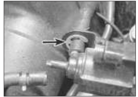
6.30 Prise off the C-clip (arrowed), and remove the inlet hose adapter from the purge valve
