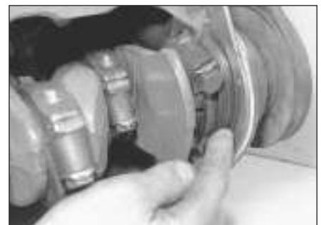
5.25 Fitting a new front oil seal . . .
