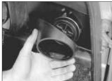
13.1b . . . and lift away the binnacle
