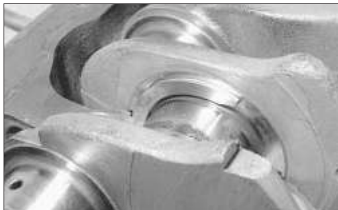
17.19 Refitting the crankshaft thrustwasher upper halves
