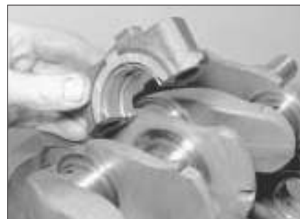
12.8 Main bearing cap with thrustwashers in position
