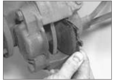
7.3b . . . then withdraw the two brake pads
