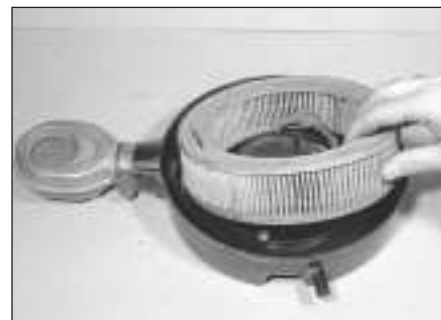
30.6b . . . and lift out the element
