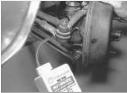
2.13 One-man brake bleeding kit connected to the front bleed screw
