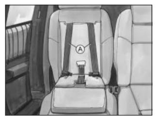
You will be using the child restraint's harness (A) to secure your child. Do not use the vehicle's safety belts.
