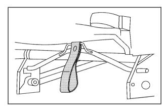
From behind the bench seat, pull the nylon strap at the center of the base of the seat to release the rear latches from the floor pins.
