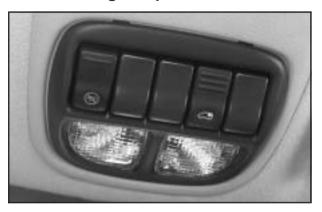
There are two reading lamps in the overhead console. To turn either reading lamp on or off, press the lens of the lamp. These lamps will come on each time you open a door, unless you turn on the interior lamps override feature. See "Interior Lamps Override" earlier in this section.
