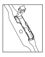
While holding the wiper arm away from the glass, push the release clip from under the blade.
