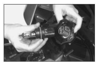
Install the new bulb through the black retainer ring and into the electrical connector. Tighten the black retainer ring in place. Push the bulb firmly enough so that the blue tabs hook over the tab on the bulb.
