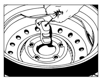
To remove the compact spare tire from the cable, tilt the retainer at the end of the cable so it can be pulled up through the wheel opening.  If your vehicle is an AWD vehicle, after removing the compact spare tire, turn the wrench clockwise to raise the cable back up.
