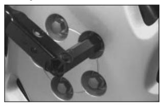
If your vehicle has the plastic bolt-on wheel covers, loosen the bolts completely using the folding wrench, and remove the wheel cover.
