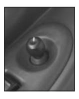
The control located on the driver's door operates both outside rearview mirrors.
