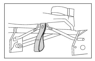
From behind the seat, pull the nylon strap, located at the base of the seat, to release the rear latches from the floor pins.
