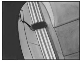
3. Be sure that the belt is not twisted and it lies flat. The guide must be on top of the belt.
