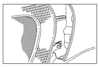
7. To reinstall the lamp assembly, line up and insert the tabs on the back of the assembly in the slots in the fender. Engage the lower clip on the back of the lamp assembly into the fender, keeping the upper tab on the front turn signal/parking lamp assembly inboard of the headlamp bracket tab.
