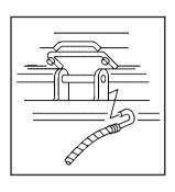
5. Hook the cable onto the outside portion of the liftgate hinges.
