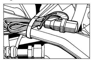
Your vehicle may have an engine coolant heater. In very cold weather, 0°F (–18°C) or colder, the engine coolant heater can help. You'll get easier starting and better fuel economy during engine warm-up. Usually, the coolant heater should be plugged in a minimum of four hours prior to starting your vehicle. At temperatures above 32°F (0°C), use of the coolant heater is not required.
