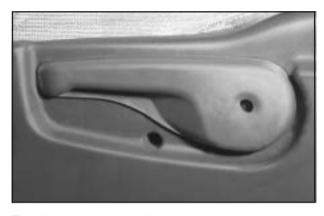
To adjust a seatback, pull up on the lever located on the outboard side of the driver's or front passenger's seats. Release the lever to lock the seatback where you want it. Push and pull on the seat to make sure it's locked into position. Pull up on the lever, and the seat will go to its original upright position.
