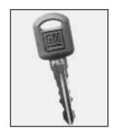
Your vehicle is equipped with the PASS-Key® III (Personalized Automotive Security System) theft-deterrent system. PASS-Key® III is a passive theft deterrent system. This means you do not have to do anything different to arm or disarm the system. It works when you insert or remove the key from the ignition.
