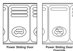
If you have the one power sliding door, these switches are located in the overhead console switchbank.
