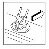
Make sure the metal tube is centered at the striker. Push the tube towards the front of the vehicle.
