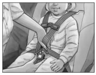
Pull up on the latch plates to make sure they are secure.
