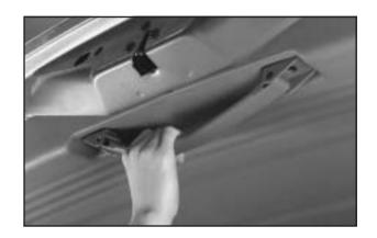
To close the liftgate, pull down on the handle, then firmly shut the liftgate. Don't drive with the liftgate open, even slightly. See *Engine Exhaust on page 2-43*.
