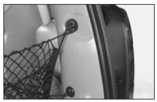
Attach the upper loops to the posts on both sides of the liftgate opening. The label on the net should be in the upper left corner.
