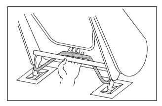
Squeeze the angled bar toward the solid crossbar while placing the front hooks of the bench seat onto the front two floor pins.
