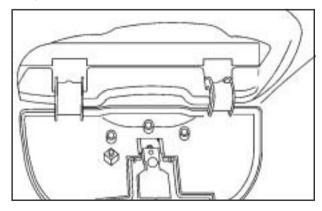
Add one peg at a time until your garage door opener operates with the compartment door closed when you press on it.
