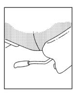
Use the lever located on the front of the seat to adjust the seat forward or rearward. Pull up the lever to unlock the seat. Slide the seat to where you want it and release the lever.
