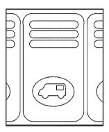
This switch, located in the overhead console switchbank, is used for opening and closing the power rear quarter windows.
