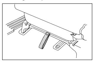
1. Pull the nylon strap behind the chair to release the rear hooks from the floor pins.
