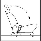
Fold the seatback flat on the seat, by either pulling on the nylon strap on the rear of the seat or lifting up on the lever located on the front of the seatback.
