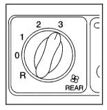
This knob is located below the main climate control system on the instrument panel switchbank. Use this knob to adjust the fan speed for the rear seat passengers.
