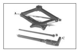
The tools you will be using include the jack (A), extension (B) and folding wrench (C).
