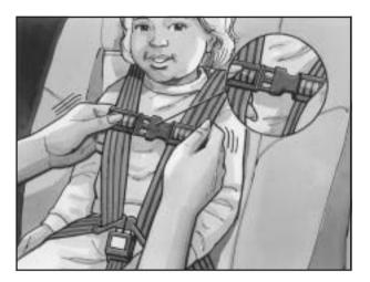
Now fasten the left and right halves of the shoulder harness clip together. The clip can be easily pulled apart and is designed to pull apart during a collision.
