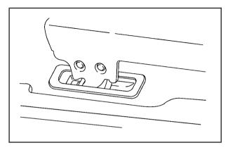
2. The seat can then be lifted off the front floor pins and removed from the vehicle.
