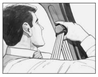
To move it down, push down on the button and move the height adjuster to the desired position. You can move the adjuster up just by pushing up on the shoulder belt guide. After you move the adjuster to where you want it, try to move it down without pushing the button down to make sure it has locked into position.
