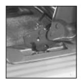
Make sure the bench seat is angled so that the front hooks clear the floor pins.
