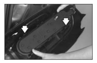
Remove the bulb holder by pressing the four retaining tabs and pulling the holder away from the assembly.
