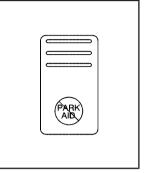
URPA can be turned off by pressing the rear park aid disable switch located in the overhead console switchbank. While the system is disabled, an indicator light will be lit on the switch. You will not see any lights on the rear display if the switch is in the off position.
