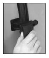
To open, pull the latch forward to release it, then swing the window outward. Press the center of the latch to secure the window in the open position.
