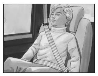
Buckle, position and release the safety belt as described in Rear Seat Passengers on page 1-46. Make sure that the shoulder belt crosses the shoulder.
