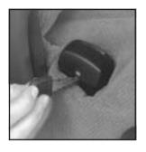
Push the red center of the buckle with a small pointed object to remove the seat belt, if needed
