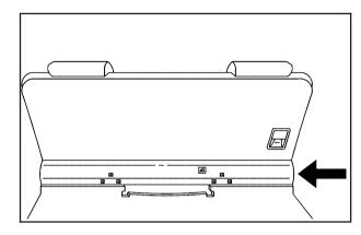
4. Put the tray sill, located on the back of the convenience center, in the upright position.
