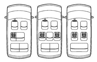
Your vehicle has the LATCH system. You will find anchors (A) in the second row outboard bucket seats, the 40 side of the 60/40 split bench seat, and both second row captain's chairs.
