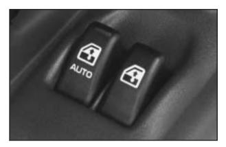
The switches on the driver's door armrest control the front windows when the ignition is in RUN, ACCESSORY or when Retained Accessory Power (RAP) is active. See "Retained Accessory Power (RAP)" under *Ignition Positions on page 2-32*.
