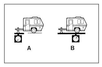
If you are using a weight-carrying or a weight-distributing hitch, the trailer tongue weight (A) should be 10 percent to 15 percent of the total loaded trailer weight (B). Do not exceed the maximum allowable tongue weight for your vehicle.
