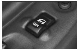
From the inside, press the front of the power door lock switch, located on either front door, to unlock all doors and the liftgate. With the content theft-deterrent system, the power door lock switch will not unlock the doors until the system is disarmed. See *Content Theft-Deterrent on page 2-27* for more details.
