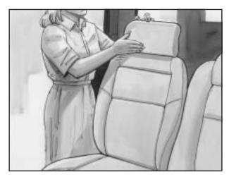
Rotate the head restraint rearward until it touches the top of the seatback. Make sure there is no gap between the lower edge of the head restraint and the top of the seatback.
