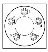
9. Tighten the wheel nuts firmly in a crisscross sequence, as shown.
