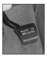
The parking brake is located under the instrument panel on the driver's side of the vehicle.
