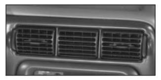
Use the knob located in the center of the outlet, to change the direction of the air flow.
