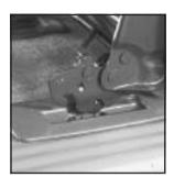
Make sure the bucket seat is angled so that the front hooks clear the floor pins.
