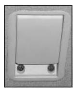
To fold down the seatback, pull up on the lever located on the back of the seat, and push the seatback down until it is locked into place.
