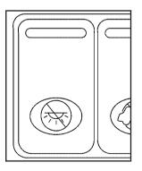
This switch is located in the overhead console switchbank. Press the bottom of the switch to keep the interior lamps off while any door is open, or the top of the switch to allow the interior lamps to come on while any door is open.
