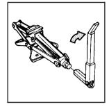
Attach the folding wrench to the jack, and turn the wrench clockwise to raise the jack head a few inches.
