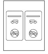
If you have the dual sliding doors, your vehicle has these switches. The left switch is for the driver's side power sliding door and the right switch is for the passenger's side sliding door. The power sliding door and the power sliding door override is one switch.
