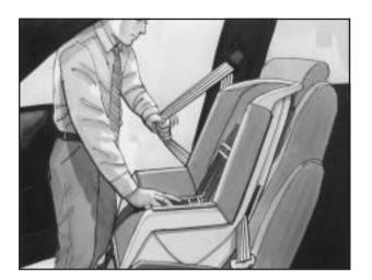
Pull the rest of the lap belt all the way out of the retractor to set the lock.
