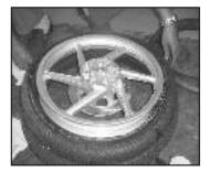
Place the wheel rim over the tyre and align it properly from all the sides with respect to inner diameter of the tyre beading portion.
