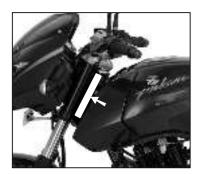
The Engine and Frame serial numbers are used to register the vehicles. They are the only means of identifying your particular vehicle from the other of the same model and type. These serial numbers may be needed by your dealer when ordering the parts. In the event of theft, the investigating authorities will require both these numbers in addition to the model, type and any special features of your vehicle that can help identifications.
