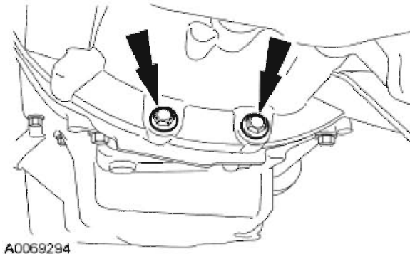
Fig. 167: Locating Transaxle-To-Engine Bolts Courtesy of FORD MOTOR CO.
