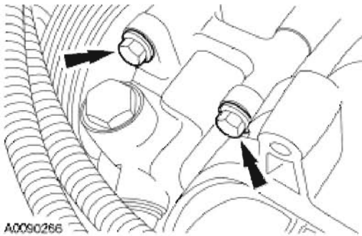
Fig. 423: Locating Power Steering Pump Bolts Courtesy of FORD MOTOR CO.
