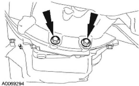
Fig. 467: Locating Transaxle-To-Engine Bolts Courtesy of FORD MOTOR CO.
