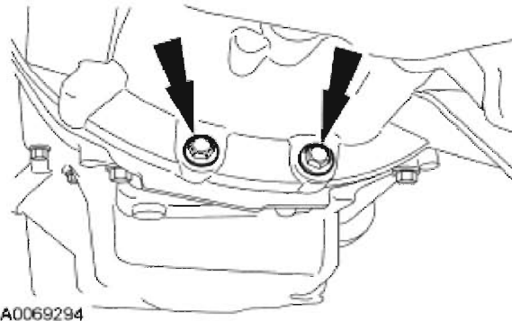
Fig. 217: Locating Transaxle-To-Engine Bolts Courtesy of FORD MOTOR CO.
