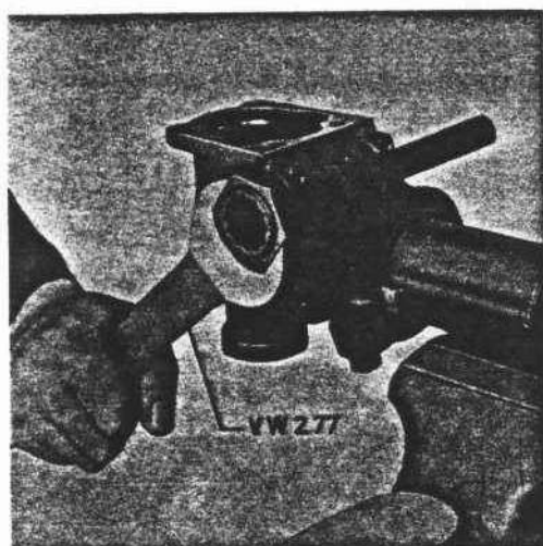
Fig. 3 Remove the lock-nut of the adjusting screw.
