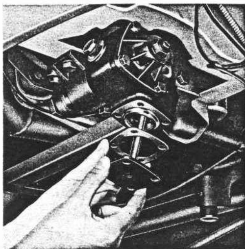
Fig. 10 Adjust the axial play of the worm spindle.
