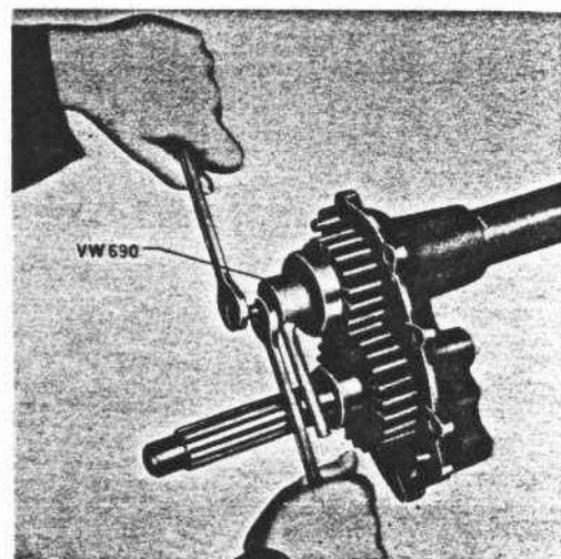
Fig. 9 Install the outer bearing of the axle shaft.
