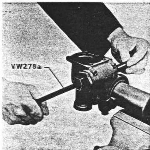
Fig. 6 Fit the adjusting screw of the shaft and tighten it slightly so that the bearings sit properly.
