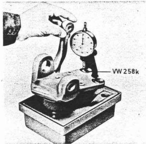
Fig. 20 Check securing surfaces (disc brake), steering knuckle removed.
