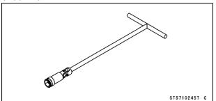
Rotor Puller, M16/M18/M20/M22 × 1.5: 57001-1216
