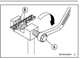
• Set the plate holder [A] and the cutting and rivetting pin [B] as shown.
