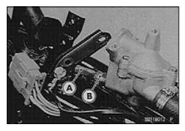
Radiator Fan Switch, Water Temperature Switch Installation
