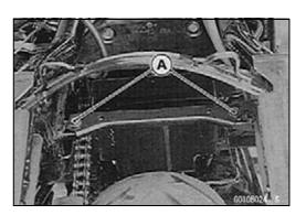
• Twist the battery case [A] to get clear of the bracket [B], and remove the case.
