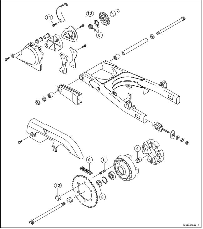
T1: 11 N·m (1.1 kgf·m, 95 in·lb) T2: 74 N·m (7.5 kgf·m, 54 ft·lb) 59 N·m (6.0 kgf·m, 43 ft·lb) (Self Locknut) T3: 127 N·m (13 kgf·m, 94 ft·lb)
