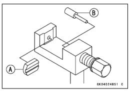
• Turn the pin holder until the rivetting pin touches link pin.
