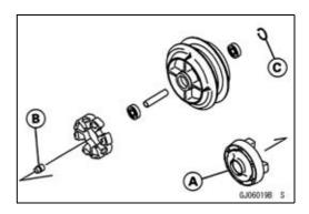
• Take the bearings [A] out of the hub, using the bearing remover.
