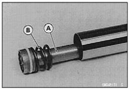
• Separate the inner tube from the outer tube as follows. ORemove the dust seal [A] from the outer tube. ORemove the retaining ring [B] from the outer tube.
