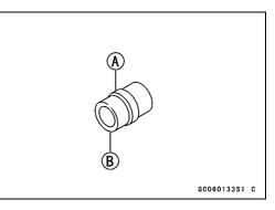
• Carefully screw in the needle jet holder. It will seat against the needle jet, pushing the end of the jet into the carburetor bore.
