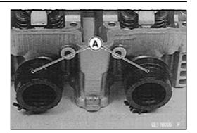
• Install the holder clamps [A] as shown being careful of the screw position and the screw head [B] direction.
