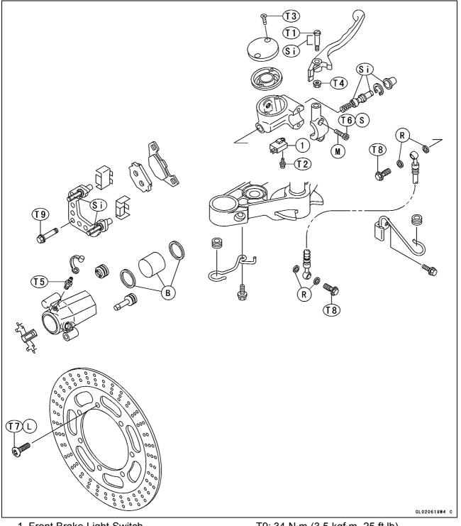
1. Front Brake Light Switch T1: 1.0 N·m (0.1 kgf·m, 9 in·lb) T2: 1.2 N·m (0.12 kgf·m, 10 in·lb) T3: 1.5 N·m (0.15 kgf·m, 13 in·lb) T4: 5.9 N·m (0.6 kgf·m, 52 in·lb) T5: 7.8 N·m (0.8 kgf·m, 69 in·lb) T6: 11 N·m (1.1 kgf·m, 95 in·lb) T7: 27 N·m (2.8 kgf·m, 20 ft·lb) T8: 34 N·m (3.5 kgf·m, 25 ft·lb)
