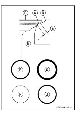
★If the width is too wide [G], too narrow [H] or uneven [J], repair the seat (see Valve Seat Repair).
