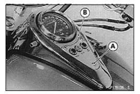
Remove: Connectors [A] Speedometer Cable [B]
