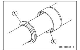
OGrasp the inner tube and stroke the outer tube up and down several times. The shock to the fork seal separates the inner tube from the outer tube.
