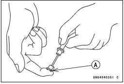
• Lubricate the throttle cable with a penetrating rust inhibiter.
