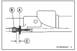
• Pull the clutch cable [A] tight and tighten the adjuster nuts against the bracket.
