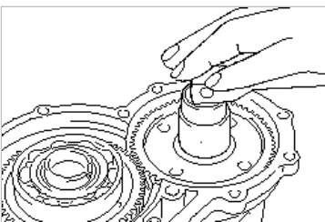
9. Using the special tool, remove the transfer driven gear.
