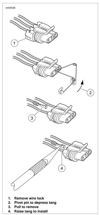
Figure A-40. 150 Metri-Pack Connector: Push-to-Seat
