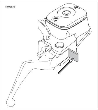
Figure 8-80. Install 5/32 in. (4 mm) Thickness Cardboard Insert
