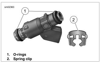
Figure 4-32. Fuel Injector
