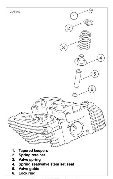
Figure 3-99. Valve Assembly
