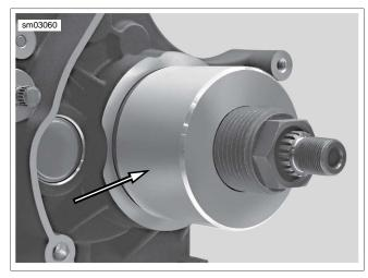
Figure 7-50. Place Installer (Part No. HD-47856-1) over Adapter
