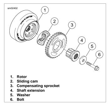
Figure 6-9. Compensating Sprocket
