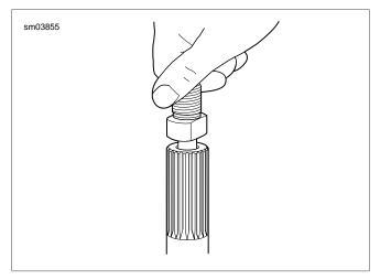
Figure 3-141. Thread Pilot Adapter into Sprocket Shaft
