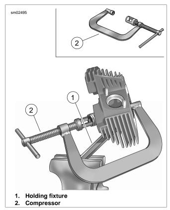
Figure 3-86. Valve Spring Compressor (Part No. HD-34736-B)
