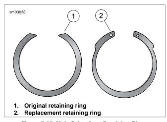
Figure 7-37. Main Drive Gear Retaining Rings
