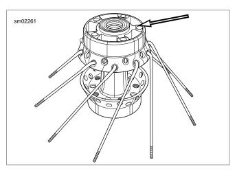
Figure 2-21. Hub: Brake Side (Narrow Flange) Up
