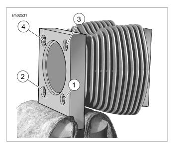
Figure 3-103. Cylinder Torque Plate Bolt Sequence
