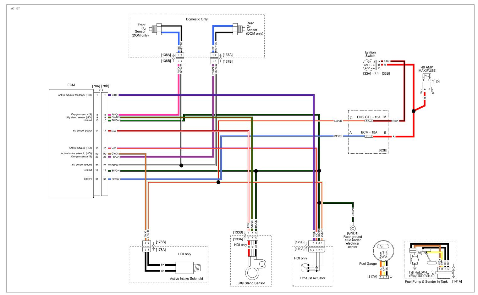
Figure B-14. 2008 ALL FXDWG, FXDC, FXDF DYNA DOM. and INT. MODELS, MAIN HARNESS, SHEET 2 OF 3
