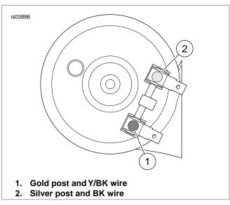
Figure 8-66. Horn Wiring
