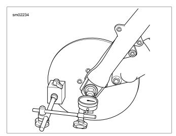
Figure 2-13. Wheel Bearing Inspection (Front Wheel Shown)
