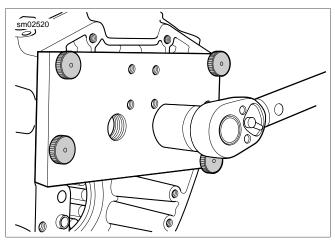
Figure 3-125. 1 Inch (25.4 mm) Bearing Installation
