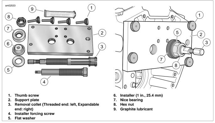
Figure 3-121. Camshaft Needle Bearing Remover/Installer (Part No. HD-42325-A)
