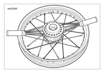
Figure 2-34. Completed Spokes: Bottom Flange Outer
