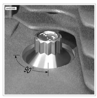
Figure 3-41. Final Tightening for Cylinder Head Bolts
