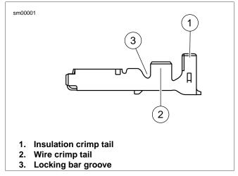
Figure A-7. AMP Multilock Connector: Socket Terminal
