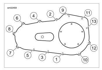
Figure 6-3. Primary Chaincase Cover Torque Sequence
