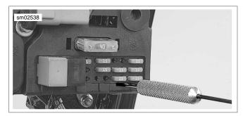
Figure 8-2. Removing Relay/Fuse Panels
