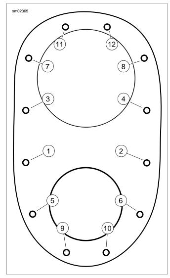
Figure 4-55. Top Plate Torque Sequence: FXD/FXDB/FXDL
