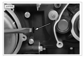
Figure 7-10. Transmission Case Pry Point
