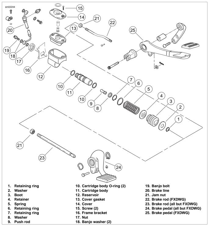
Figure 2-74. Rear Brake Master Cylinder
