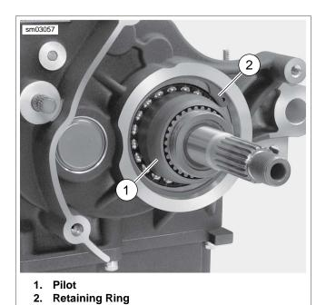
Figure 7-47. Install Pilot (Part No. HD-47856-2)
