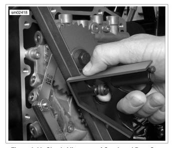
Figure 3-69. Check Alignment of Crank and Rear Cam Sprocket Faces
