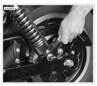
Figure 1-41. Rear Shock Absorber Spring Adjustment (Typical)
