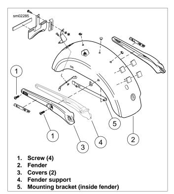
Figure 2-110. Rear Fender (FXD, FXDC, FXDB, and FXDL)
