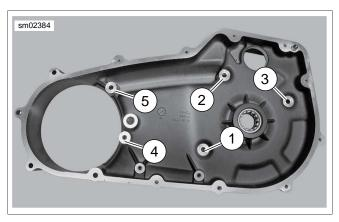
Figure 6-29. Sealing Fastener Torque Sequence
