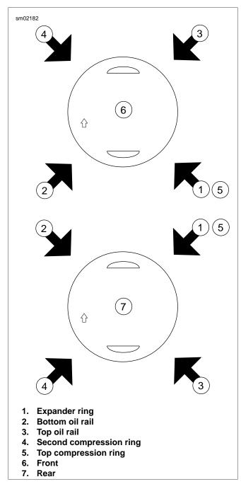
Figure 3-111. Piston Ring Gap Alignment
