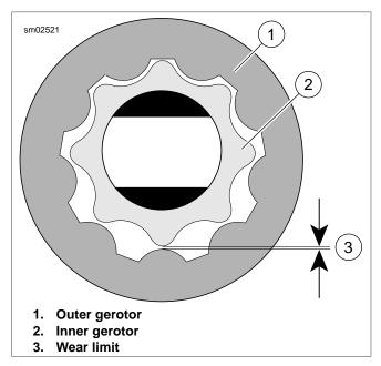
Figure 3-128. Measure Gerotor Sets for Wear
