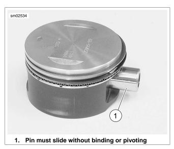
Figure 3-106. Piston Pin Clearance
