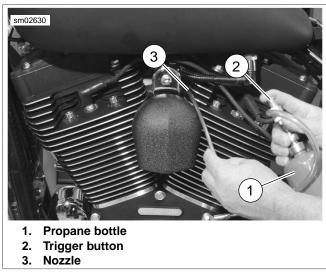
Figure 4-71. Checking for Leaks
