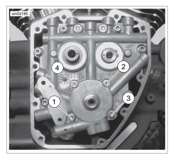
Figure 3-67. Oil Pump Torque Sequence
