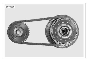
Figure 6-6. Remove Drive Components
