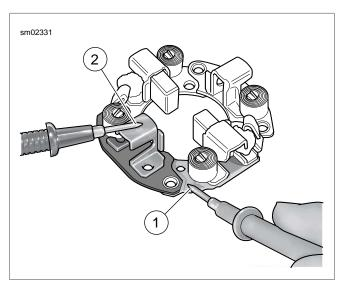
Figure 5-8. Brush Holder Insulation Test
