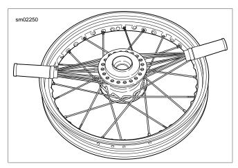
Figure 2-35. Beginning Spoke: Bottom Flange Inner
