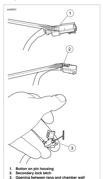
Figure A-43. 480 Metri-Pack Connector: Remove Socket Terminal
