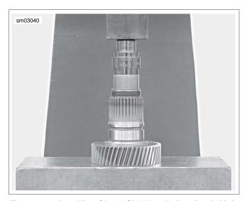
Figure 7-38. Installing Clutch Side Needle Bearing in Main Drive Gear
