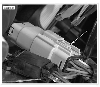
Figure A-27. Molex Connector: Latch
