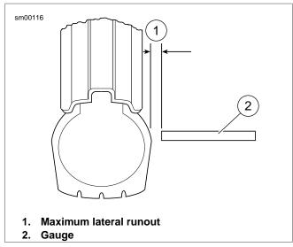
Figure 2-55. Checking Tire Lateral Runout
