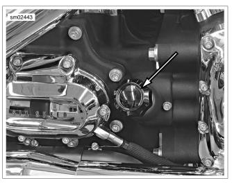
Figure 1-1. Checking Engine Oil Level
