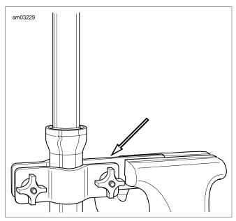
Figure 2-82. Fork Holding Tool (HD-41177) (mounted vertically to slider)
