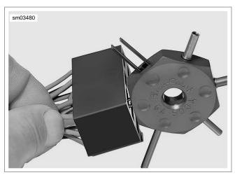
Figure A-11. Removing Autofuse Terminal from Fuse Block
