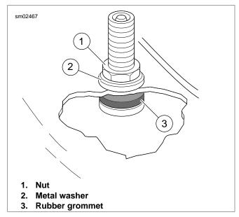
Figure 2-81. Tubeless Tire Valve Stem
