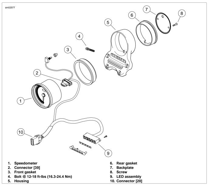
Figure 8-53. Instrumentation: FXD
