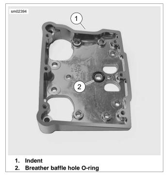
Figure 3-44. Rocker Housing Alignment
