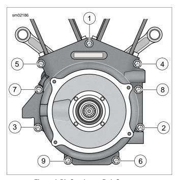
Figure 3-58. Crankcase Bolt Sequence
