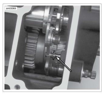
Figure 7-58. Shifter Shaft Lever Spring
