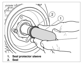
Figure 7-42. Seal Protector Sleeve
