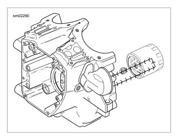
Figure 3-3. Oil Filter Flow
