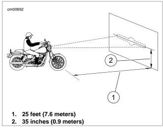
Figure 1-46. Checking Headlamp Alignment: Dyna Models
