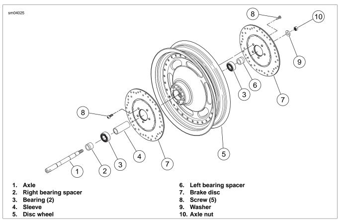
Figure 2-6. Cast Front Wheel Components (FXDF)
