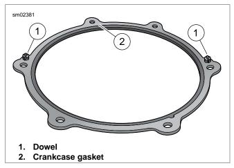
Figure 6-26. Crankcase Gasket
