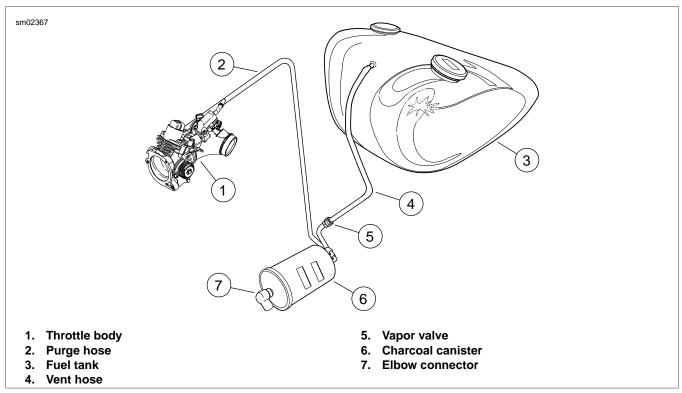
Figure 4-72. Schematic-CA Evaporative Emissions Control System
