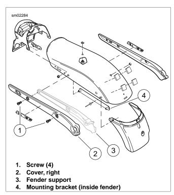
Figure 2-109. Rear Fender (FXDWG/FXDF)
