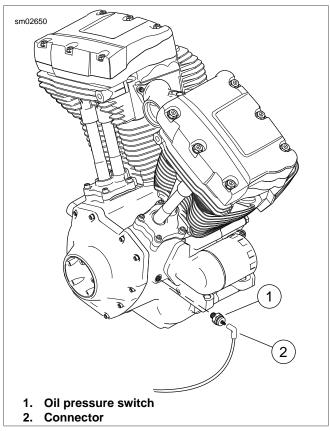
Figure 8-63. Oil Pressure Switch
