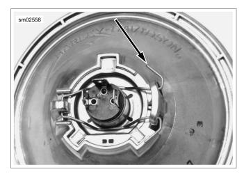
Figure 8-19. Wire Retaining Clip
