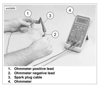
Figure 1-44. Testing Resistance
