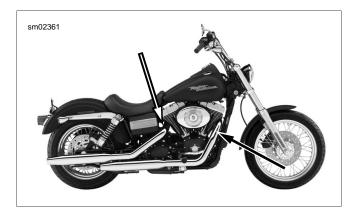
Figure 4-27. Oxygen Sensors (Inboard Side of Exhaust Pipes)
