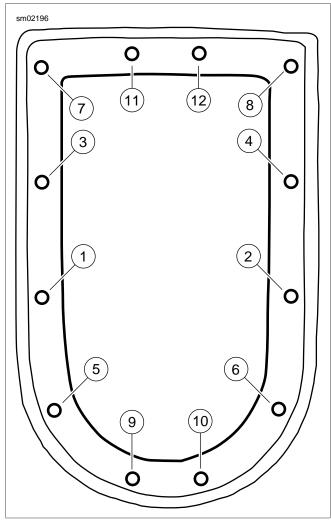
Figure 8-49. Top Plate Torque Sequence: FXDWG/FXDC/FXDF
