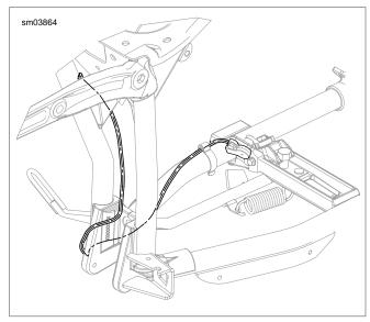
Figure 2-112. Jiffy Stand Sensor Harness Routing
