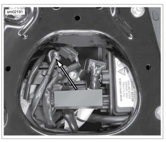
Figure 4-29. Rear O2 Connector and Harness
