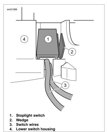
Figure 8-88. Install Stoplight Switch
