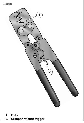
Figure A-26. Packard Terminal Crimper (HD-38125-7)
