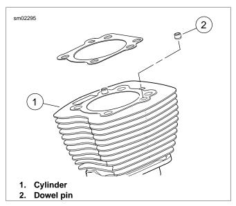
Figure 3-39. Cylinder Dowel Pins
