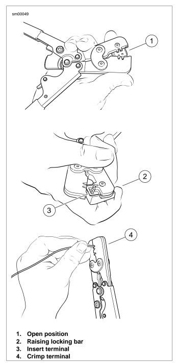
Figure A-53. Packard Micro 64 Connector: Terminal in Crimper
