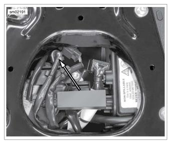
Figure 4-65. Rear O2 Connector and Harness
