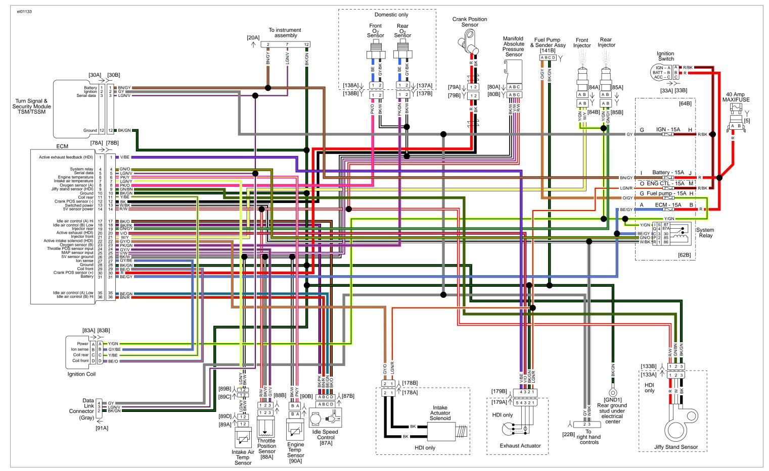
Figure B-7. 2008 ALL DYNA DOM. and INT. MODELS (Except FXDWG, FXDC, FXDF), IGNITION CIRCUIT
