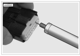
Figure A-30. Molex Connector: Terminal Remover (HD-48114)
