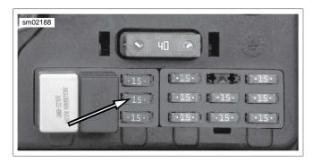
Figure 8-11. Fuel Pump Fuse
