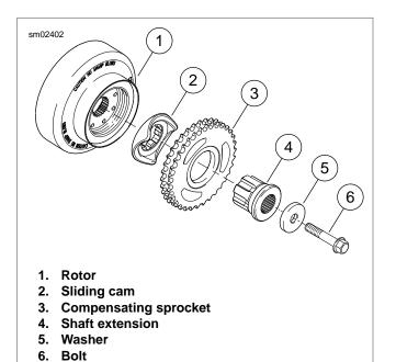
Figure 6-10. Compensating Sprocket
