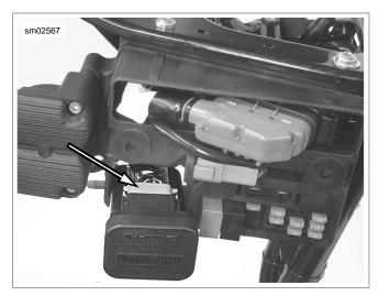
Figure 8-32. TSM/TSSM/HFSM Connector [30] (typical)
