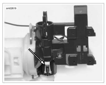
Figure 4-46. Fuel Pump Hose Retaining Clip (2)
