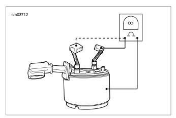
Figure 5-6. Grounded Field Test
