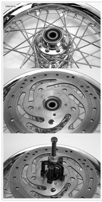
Figure 2-15. Brake Disk as Puller Aid
