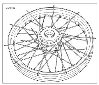
Figure 2-39. Beginning Spoke: Top Flange Inner
