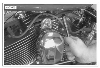
Figure 4-16. Engine Temperature Sensor Removal
