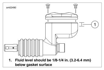
Figure 1-6. Rear Brake Master Cylinder Reservoir
