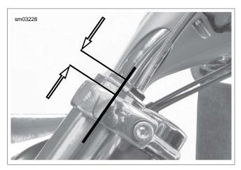
Figure 2-88. Fork Tube Protrusion: Typical
