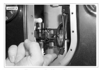
Figure 4-39. Fuel Pump Removal
