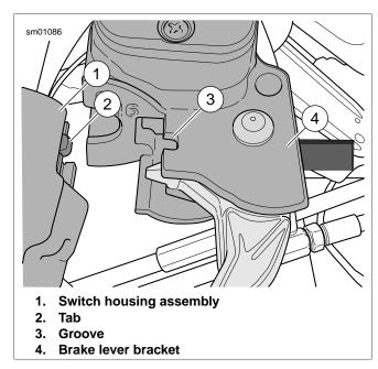
Figure 8-84. Switch Housing Alignment (typical)
