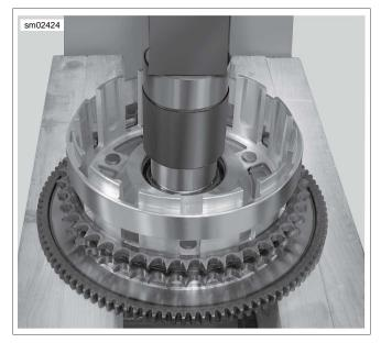
Figure 6-35. Pressing Bearing From Clutch Shell
