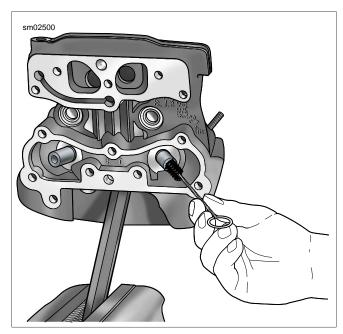
Figure 3-92. Scrubbing Valve Guide Bore
