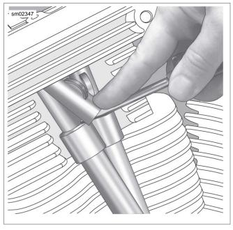
Figure 3-48. Install Spring Cap Retainers
