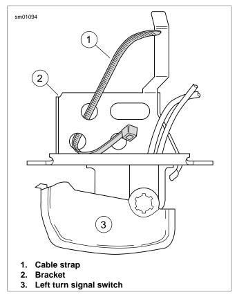
Figure 8-95. Insert Cable Strap in Switch Bracket
