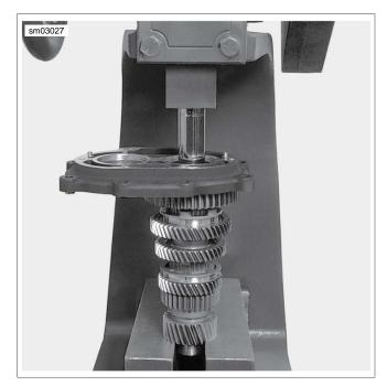
Figure 7-28. Installing Countershaft
