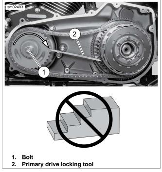
Figure 6-11. Installing Compensating Sprocket Bolt
