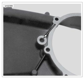
Figure 6-25. Shifter Shaft Bushing
