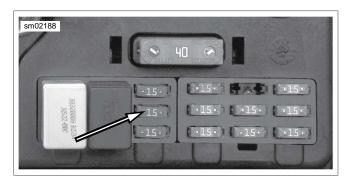
Figure 4-56. Fuel Pump Fuse
