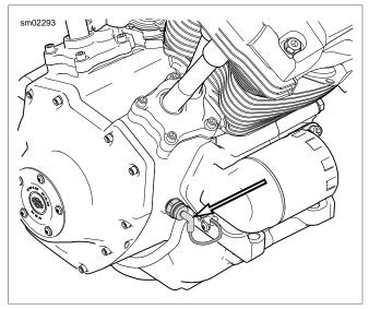
Figure 3-14. Oil Pressure Switch
