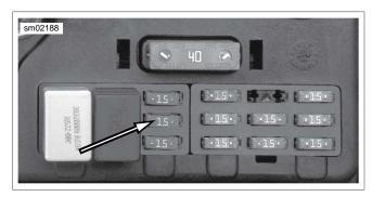
Figure 4-13. Fuel Pump Fuse
