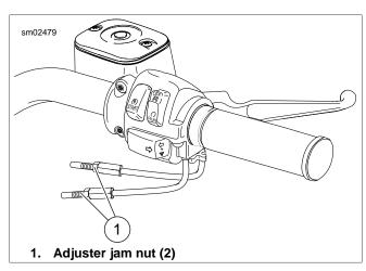
Figure 2-94. Handlebar Throttle Control
