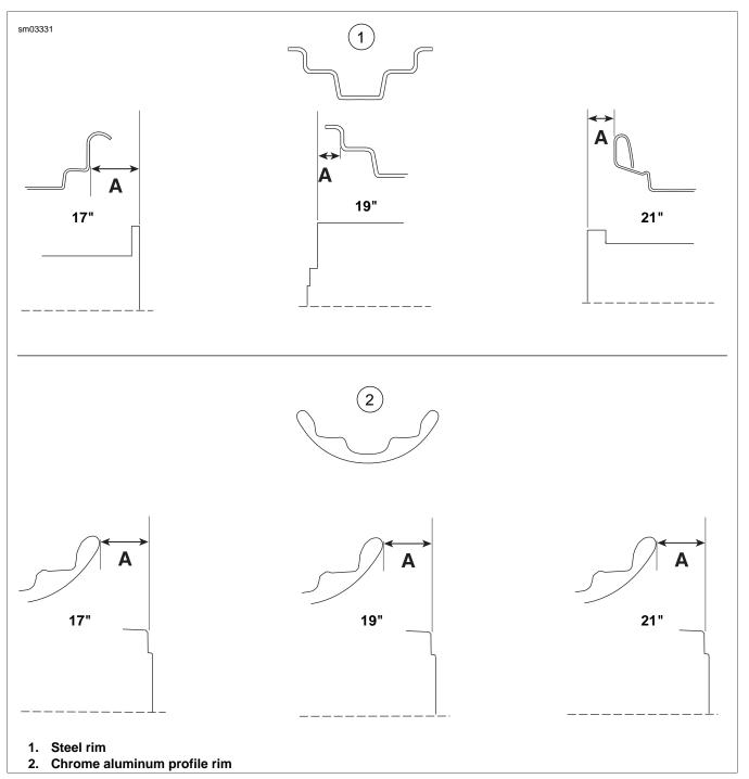
Figure 2-53. Laced Wheel Hub Offset Dimensions
