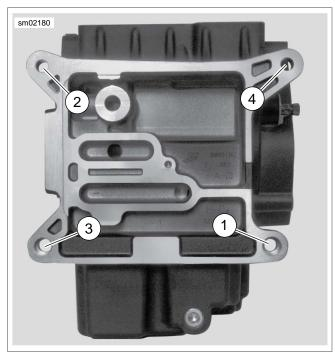
Figure 7-54. Transmission Housing to Crankcase Torque Sequence
