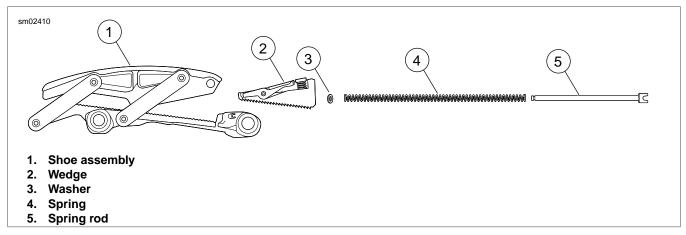
Figure 6-14. Primary Chain Tensioner Assembly
