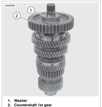
Figure 7-20. Countershaft 1st Gear
