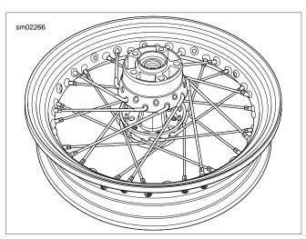
Figure 2-27. Sprocket Side Up: Bottom Row of Spokes Laced
