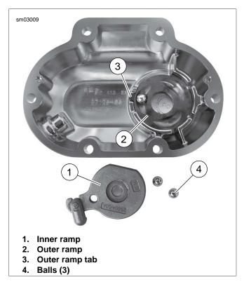
Figure 7-5. Coupling and Ramp Assembly
