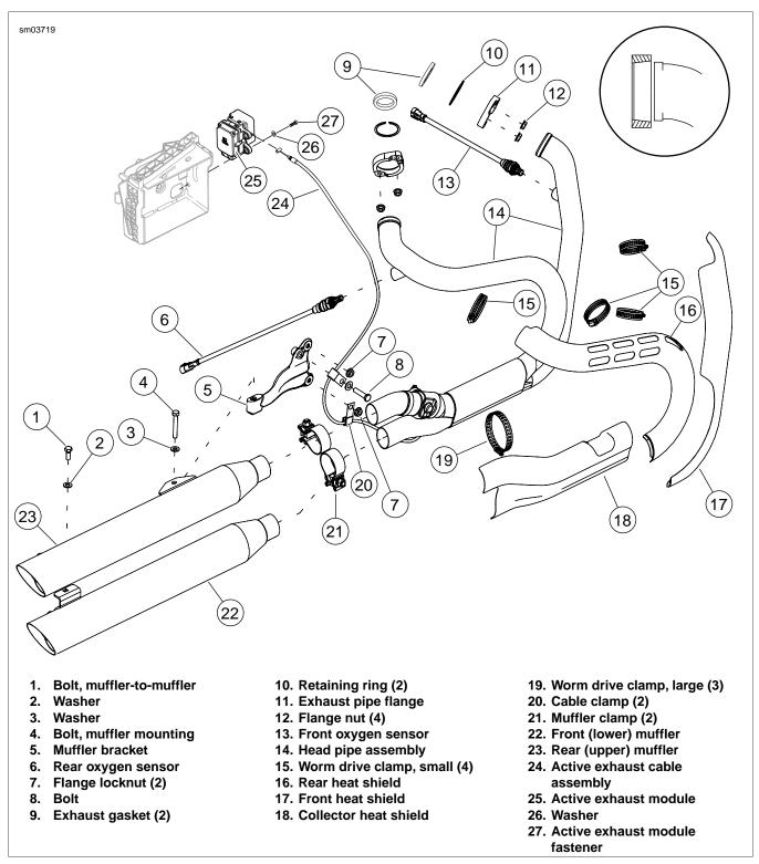
Figure 4-68. Exhaust System: FXDF
