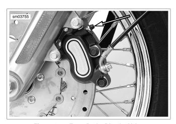
Figure 1-31. Front Brake Bleeder Valve
