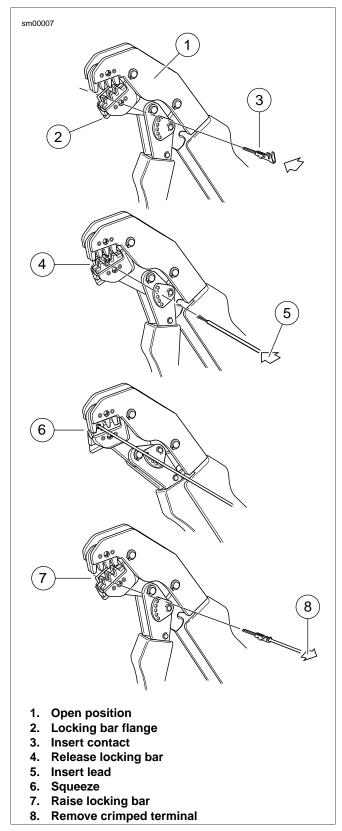
Figure A-8. AMP Multilock Connector: Terminal Crimping Procedure
