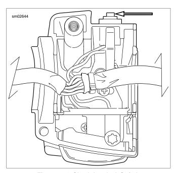
Figure 8-94. Clutch Interlock Switch
