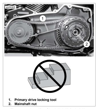
Figure 6-12. Installing Clutch Hub Mainshaft Nut
