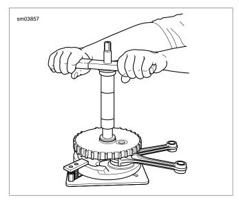
Figure 3-143. Press Inner Race onto Sprocket Shaft:
