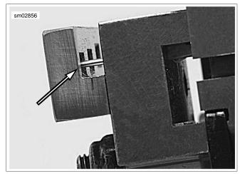
Figure A-35. Pin Terminal against Pin Locator Bar
