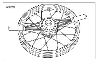
Figure 2-33. Beginning Spoke: Bottom Flange Outer
