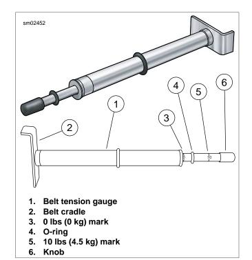
Figure 1-25. Belt Tension Gauge (Part No. HD-35381-A)
