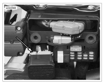
Figure 8-33. HFSM Antenna Connector [208]
