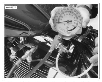
Figure 4-59. Fuel Pressure Gauge Installed (Typical)
