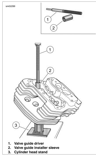
Figure 3-90. Install Valve Guide
