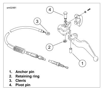
Figure 2-99. Clutch Cable Installation
