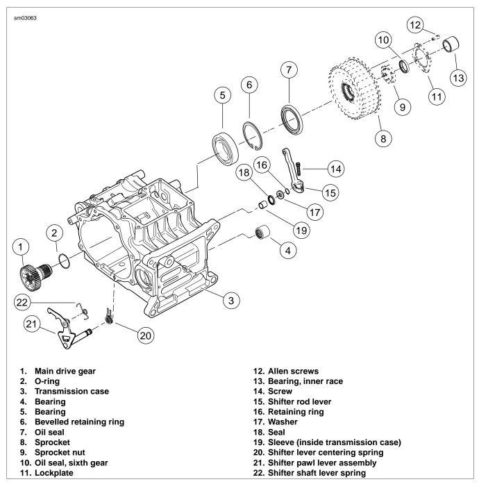
Figure 7-53. Transmission Case, Sprocket and Main Drive Gear
