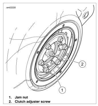
Figure 1-21. Clutch Adjuster Screw
