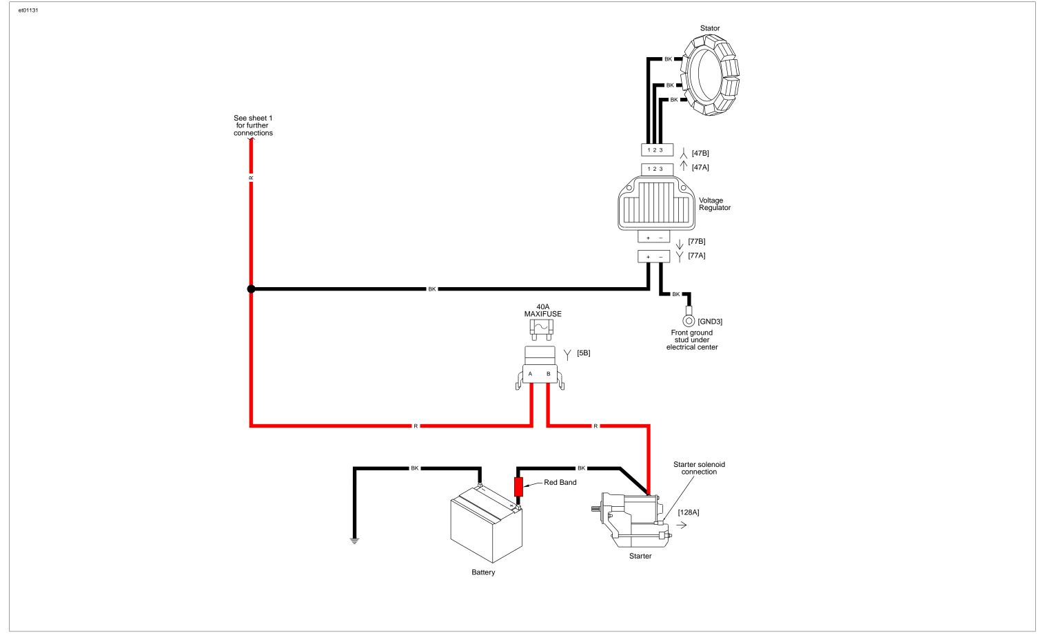
Figure B-5. 2008 ALL DYNA DOM. and INT. MODELS (Except FXDWG, FXDC, FXDF), CHARGING CIRCUIT
