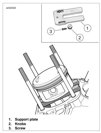
Figure 3-36. Piston Support Plate
