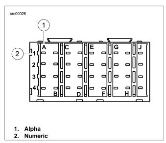
Figure A-42. Fuse Block: Coordinates (typical)
