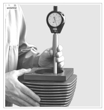
Figure 3-104. Measure for Out-of-Round and Taper
