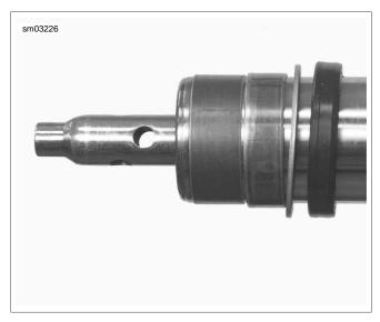
Figure 2-86. Seat Pipe Centered in Fork Tube
