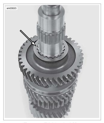
Figure 7-23. Third Gear Lock Ring
