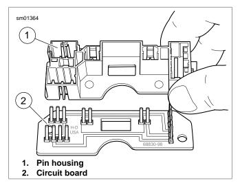
Figure 8-25. Pin Housing and Circuit Board
