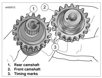
Figure 3-115. Camshaft Timing Marks
