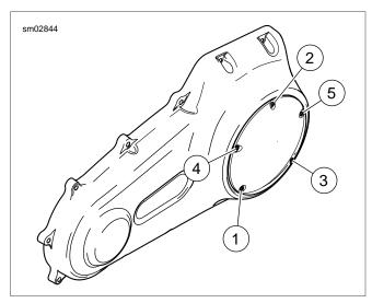
Figure 1-16. Clutch Cover Torque Sequence
