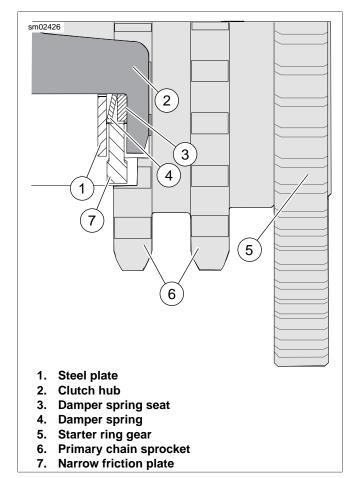
Figure 6-36. Clutch Stackup
