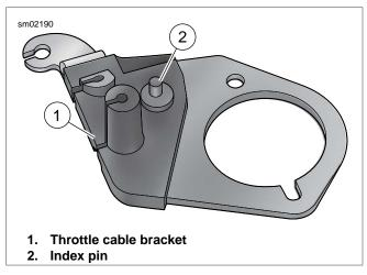
Figure 4-26. Throttle Cable Bracket
