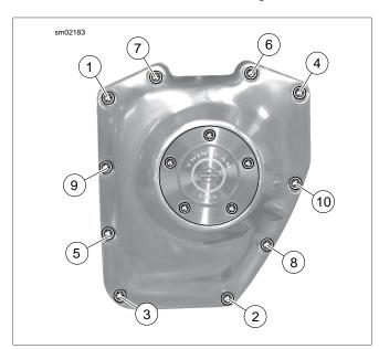
Figure 3-51. Cam Cover Screws
