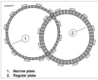
Figure 6-31. Friction Plates
