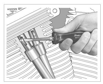
Figure 3-19. Removing Spring Cap Retainer
