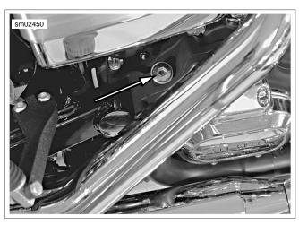
Figure 1-17. Transmission Filler Plug/Dipstick Location
