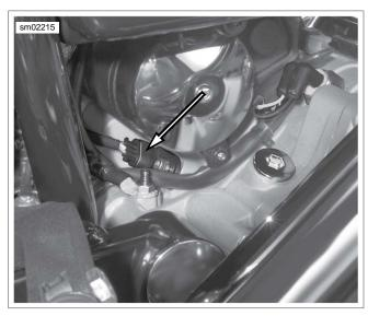
Figure 8-54. Vehicle Speed Sensor and Connector [65]
