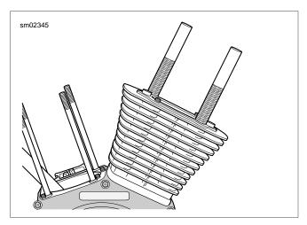
Figure 3-38. Install Threaded Cylinders to Studs
