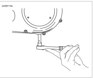
Figure 1-14. Removal/Installation of Chaincase Drain Plug
