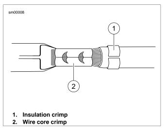
Figure A-9. AMP Multilock Connector: Terminal Crimp
