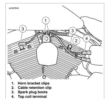
Figure 8-7. Spark Plug Cable Routing
