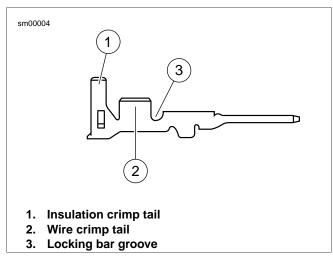
Figure A-6. AMP Multilock Connector: Pin Terminal
