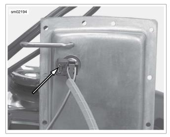
Figure 8-45. Connector Tab
