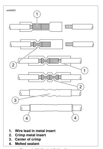
Figure A-55. Sealed Splice Connector
