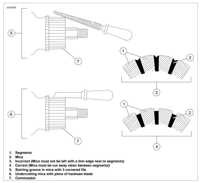
Figure 5-2. Undercutting Mica Separators
