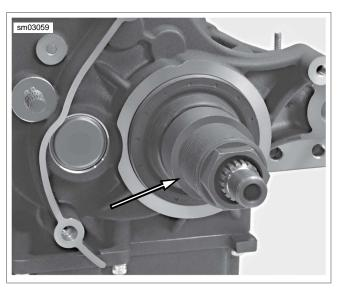
Figure 7-49. Install Adapter (Part No. HD-47856-3)
