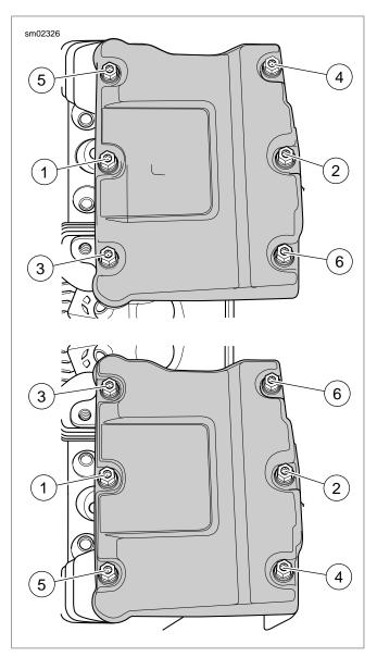
Figure 3-18. Rocker Cover Bolt Removal Sequence
