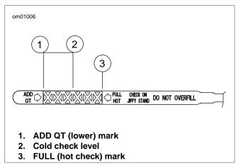
Figure 1-2. Engine Oil Dipstick
