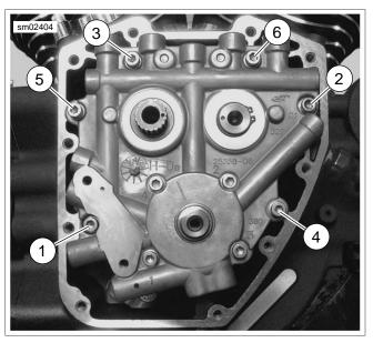
Figure 3-66. Cam Support Plate Torque Sequence
