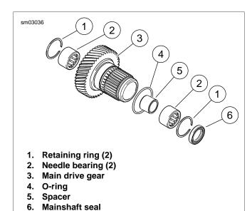
Figure 7-36. Main Drive Gear Assembly
