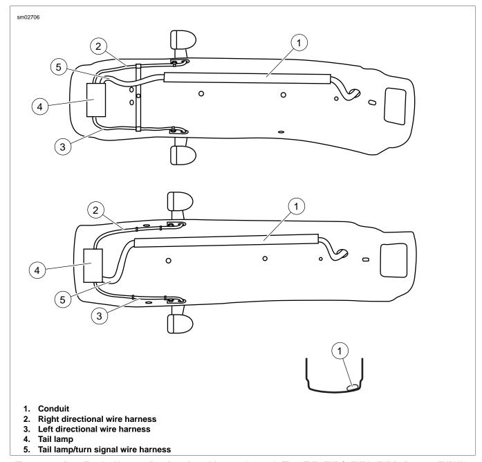
Figure 8-29. Rear Fender Harness Routing-viewed from underneath (Top: FXD, FXDC, FXDL, FXDB; Bottom: FXDWG, FXDF)
