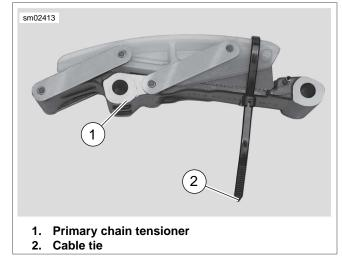
Figure 6-17. Securing Primary Chain Tensioner
