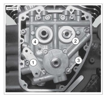
Figure 3-54. Oil Pump Torque Sequence
