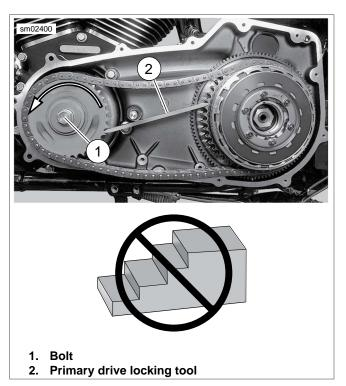
Figure 6-8. Removing Compensating Sprocket Bolt
