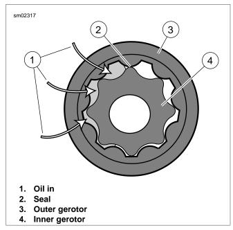
Figure 3-10. Inlet Side Oil Flow
