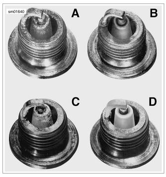
Figure 1-43. Typical Spark Plug Deposits
