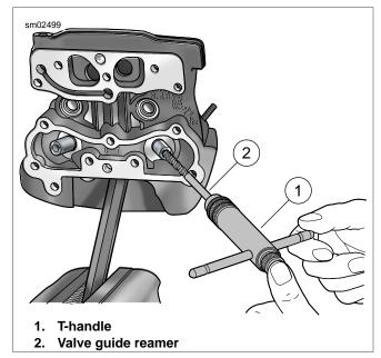
Figure 3-91. Reaming Valve Guide Bore
