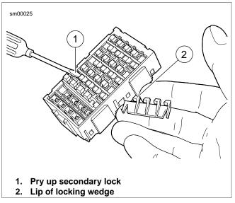
Figure A-41. Fuse Block: Remove Secondary Locks
