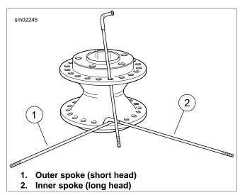
Figure 2-30. Lacing 19 Inch Wheel Hub
