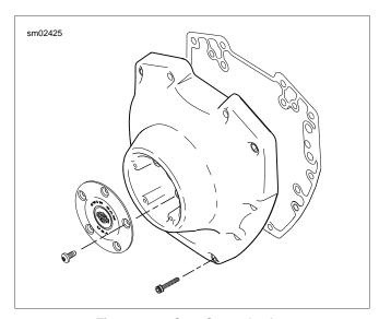
Figure 3-72. Cam Cover Gasket
