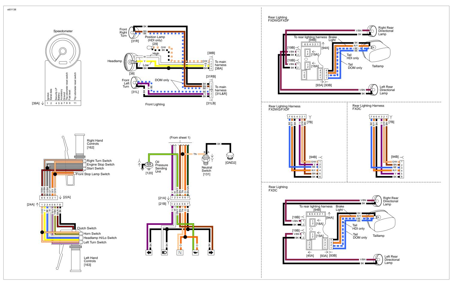
Figure B-15. 2008 ALL FXDWG, FXDC, FXDF DYNA DOM. and INT. MODELS, MAIN HARNESS, SHEET 3 OF 3
