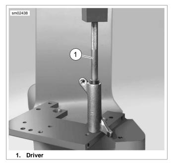
Figure 3-80. Install Bushings
