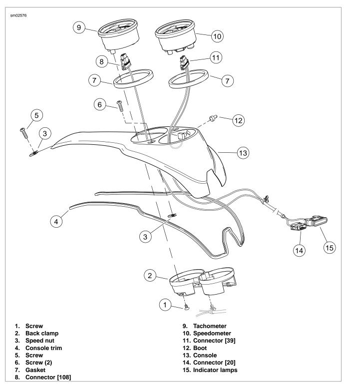
Figure 8-52. Instrumentation: FXDL, FXDB
