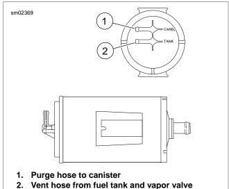
Figure 4-74. Charcoal Canister Connections
