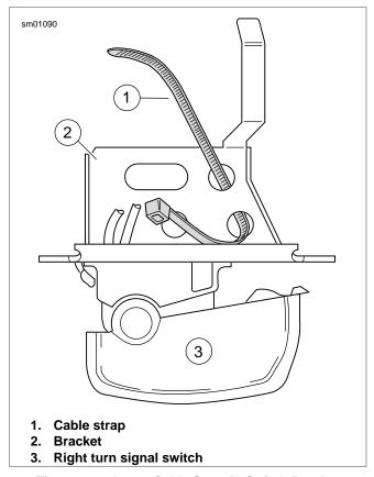
Figure 8-89. Insert Cable Strap in Switch Bracket
