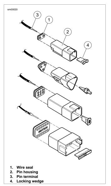
Figure A-22. Deutsch Connector: 2, 3, 4 and 12-Place Pin Housings
