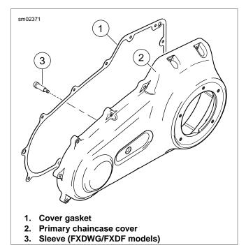
Figure 6-2. Primary Chaincase Cover Gasket
