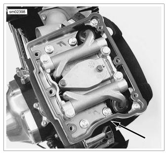
Figure 3-49. Rocker Cover Gasket Indent (Front Cylinder Shown)
