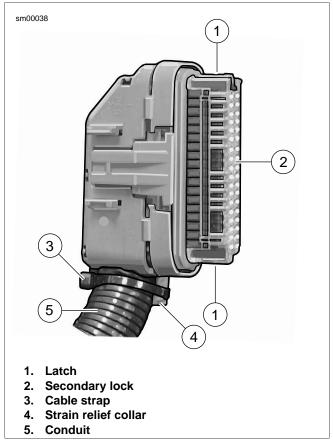
Figure A-47. Packard 100W Connector
