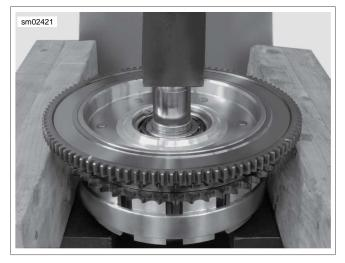
Figure 6-33. Pressing Clutch Hub From Bearing
