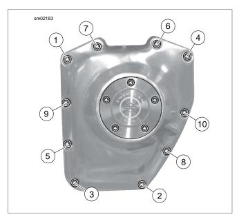
Figure 3-73. Cam Cover Screws
