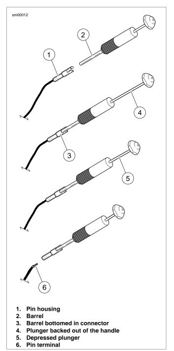
Figure A-2. AMP Pin Terminal Remover (HD-39621-28)
