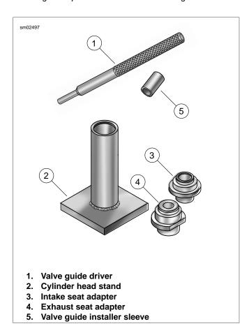
Figure 3-88. Valve Guide Replacement Tools
