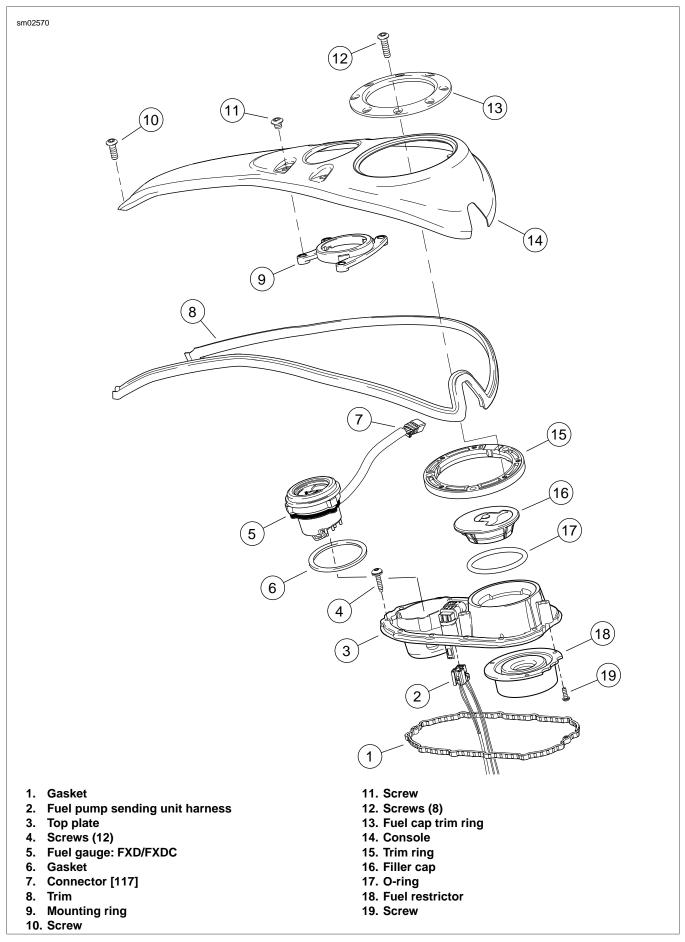
Figure 8-39. Fuel Gauge: FXD
