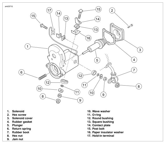
Figure 5-10. Solenoid Assembly
