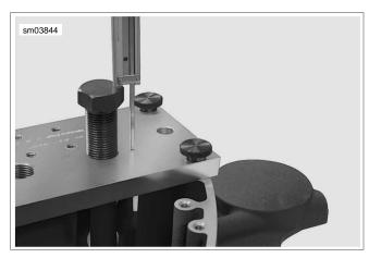
Figure 3-127. Measure from Top of Forcing Screw to Support Plate
