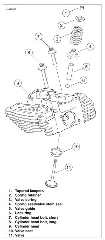
Figure 3-87. Cylinder Head Assembly
