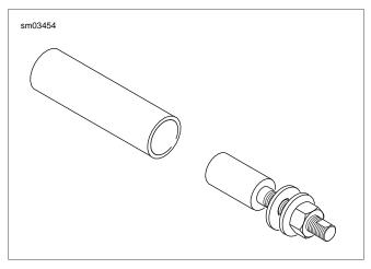
Figure 6-23. Mainshaft Bearing Inner Race Installer
