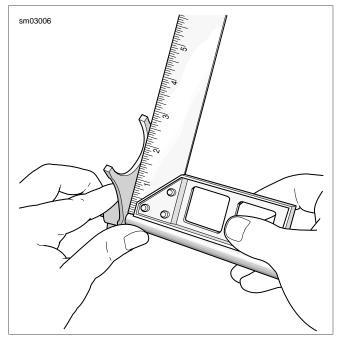
Figure 7-27. Checking Fork
