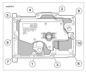
Figure 3-148. Oil Pan Torque Sequence
