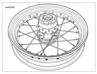
Figure 2-26. Sprocket Side Up: Start First Spoke of Bottom
