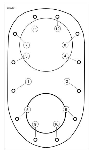
Figure 8-50. Top Plate Torque Sequence: FXD/FXDB/FXDL
