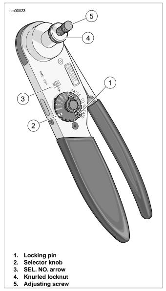
Figure A-24. Electrical Crimper Tool (HD-42879)
