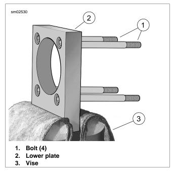
Figure 3-102. Attaching Cylinder Torque Plates
