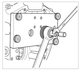
Figure 3-122. Bearing Removal
