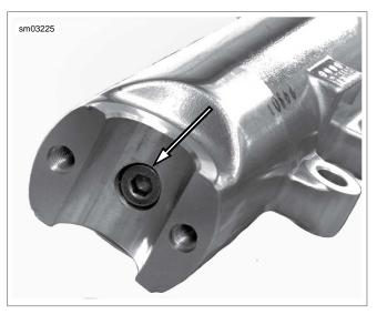
Figure 2-84. Seat Pipe Screw (right fork assembly)
