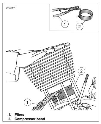
Figure 3-37. Piston Ring Compressor
