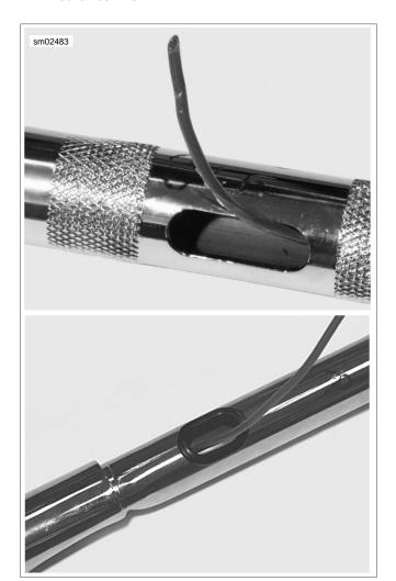
Figure 2-105. Wire Leader in Handlebars (Handlebars Removed from Motorcycle)
