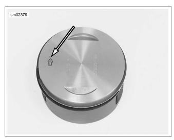
Figure 3-30. Piston Installation Arrow
