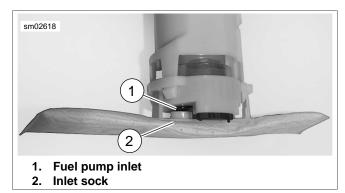
Figure 4-45. Fuel Sock Installation
