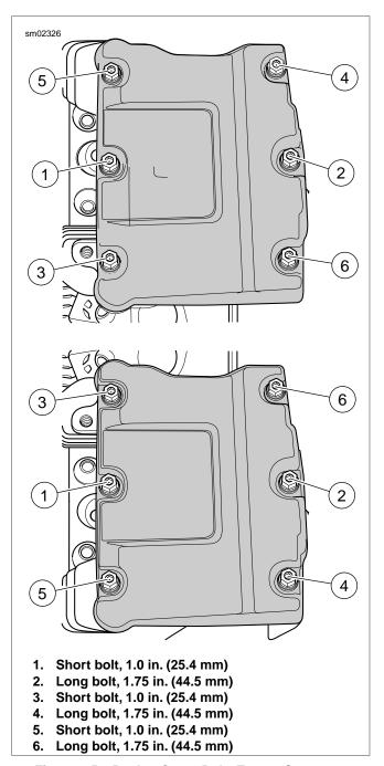
Figure 3-50. Rocker Cover Bolts Torque Sequence
