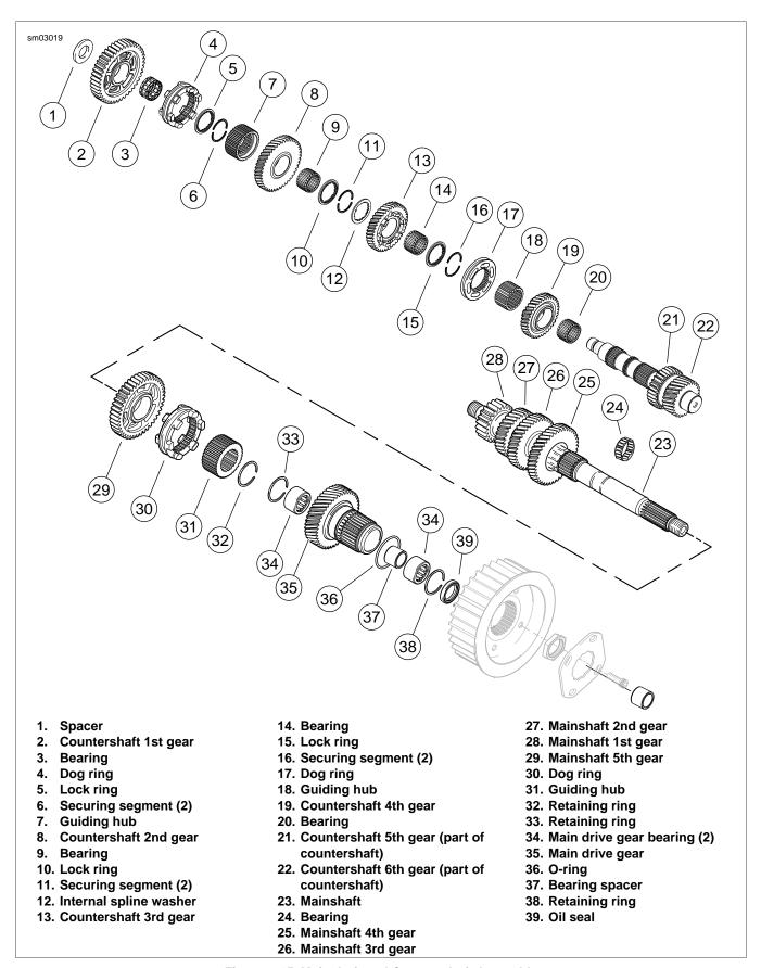
Figure 7-15. Mainshaft and Countershaft Assembly
