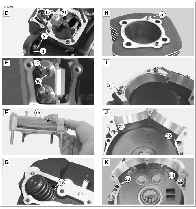
Figure 3-5. Engine Oil Flow - Top End
