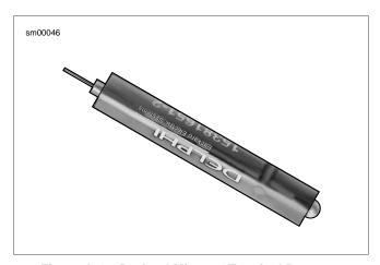
Figure A-49. Packard Micro 64 Terminal Remover (HD-45928)
