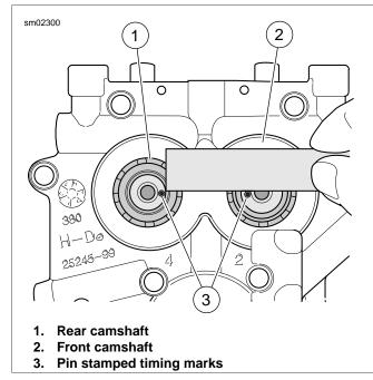
Figure 3-65. Verify Alignment of Punch Marks
