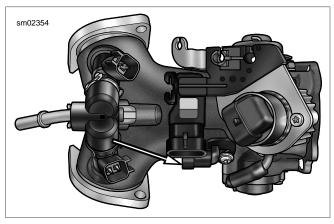
Figure 4-11. Intake Air Temperature Sensor Location
