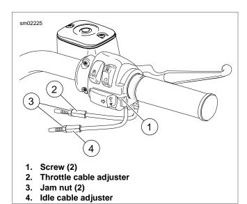
Figure 1-29. Throttle Cable Adjusters
