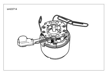
Figure 5-9. Install Paper Clips to Hold Brush Springs
