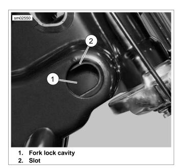
Figure 8-15. Fork Lock/Ignition Switch Cavity
