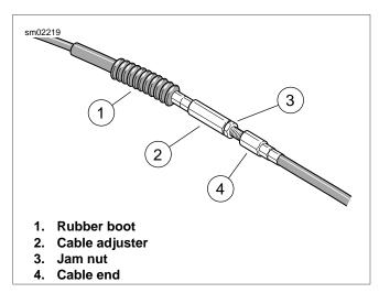
Figure 1-20. Clutch Cable Adjuster
