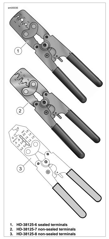
Figure A-44. Metri-Pack Terminal Crimp Tools
