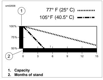
Figure 1-40. Battery Self-Discharge Rate
