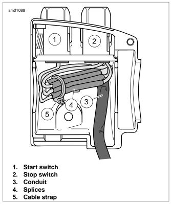
Figure 8-87. Upper Housing With Splices
