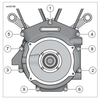
Figure 3-61. Tightening Crankcase Bolts
