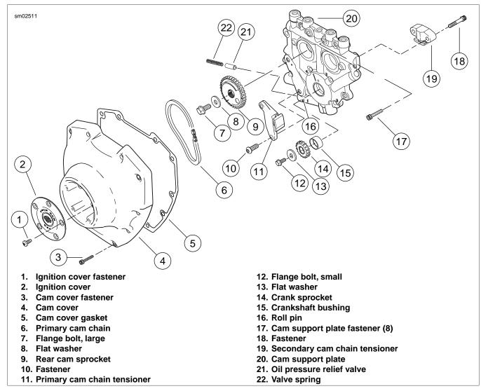
Figure 3-113. Cover and Cam Support Plate Assembly
