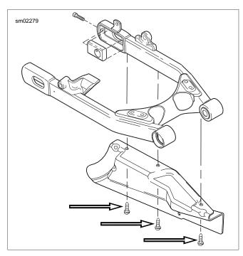
Figure 2-93. Debris Deflector Screws
