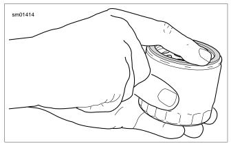
Figure 1-5. Lubricating New Oil Filter Gasket
