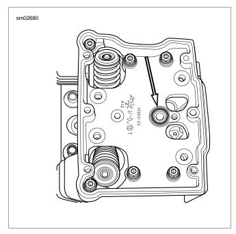
Figure 3-24. Breather Baffle Hole O-Ring
