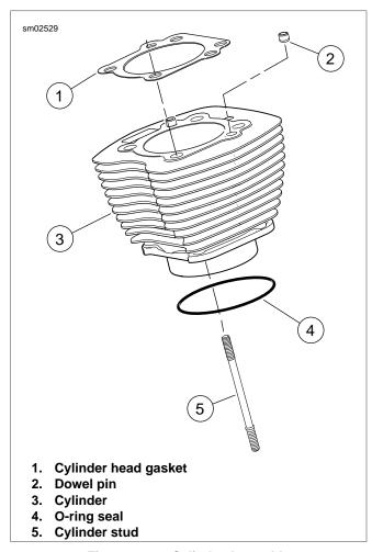
Figure 3-100. Cylinder Assembly
