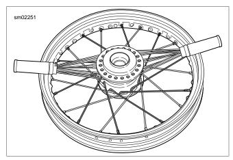
Figure 2-36. Completed Spokes: Bottom Flange Inner
