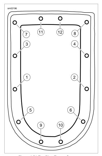
Figure 4-54. Top Plate Torque Sequence: FXDWG/FXDC/FXDF
