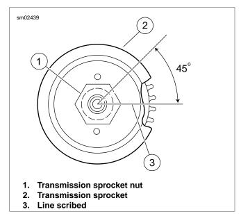
Figure 6-42. Transmission Sprocket Nut Final Tightening
