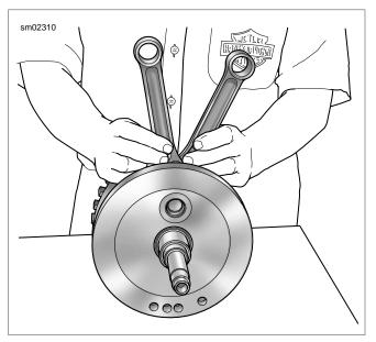
Figure 3-145. Connecting Rod Bearing Clearance
