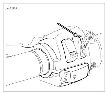
Figure 1-47. Headlamp Switch High Beam Setting
