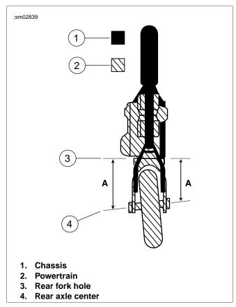
Figure 2-60. Adjust Axle Adjusters until A = A
