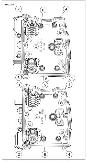
Figure 3-25. Rocker Housing Bolts Removal Sequence
