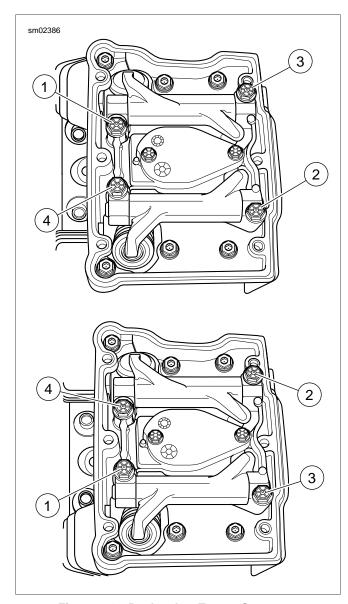
Figure 3-47. Rocker Arm Torque Sequence
