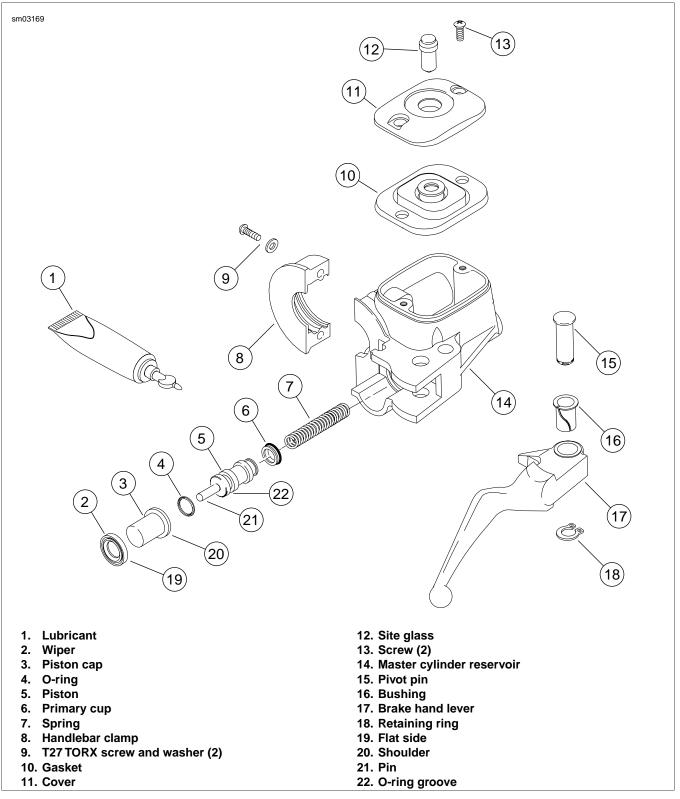
Figure 2-63. Front Brake Master Cylinder
