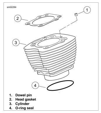
Figure 3-27. Cylinder Assembly
