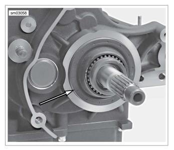
Figure 7-48. Place Main Drive Gear Seal Over Pilot
