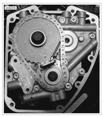
Figure 3-68. Camshaft Locking Tool
