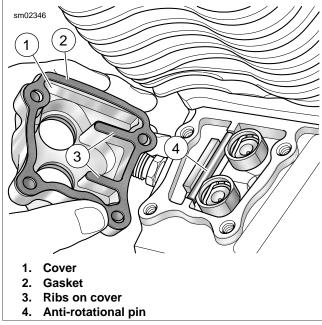
Figure 3-45. Installing Lifters
