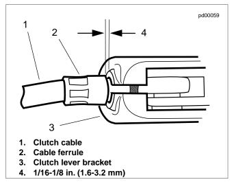
Figure 1-22. Clutch Hand Lever
