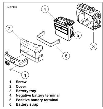
Figure 1-39. Battery Assembly
