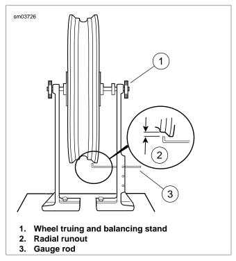
Figure 2-56. Checking Cast Rim Radial Runout
