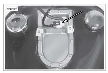
Figure 4-5. Fuel Pump Module Connector [141]
