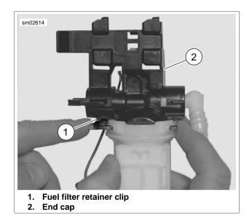
Figure 4-41. Filter Retainer Clip
