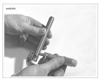
Figure 3-79. Checking Shaft to Bushing Fit
