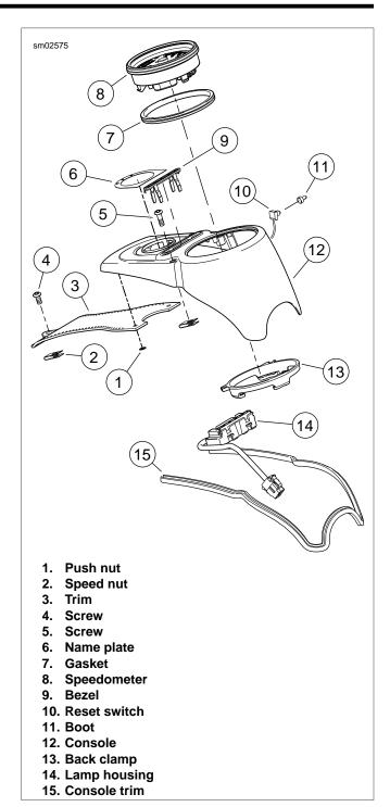
Figure 8-51. Speedometer: FXDWG/FXDC/FXDF
