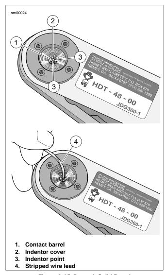
Figure A-25. Deutsch Solid Barrel
