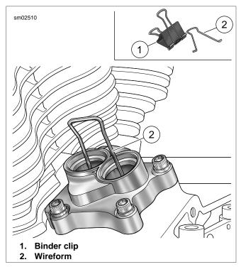
Figure 3-112. Hydraulic Lifter Holding Tool
