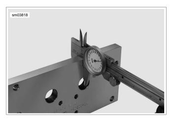
Figure 3-123. Measure Thickness of Support Plate
