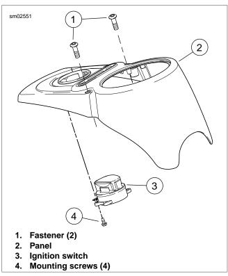
Figure 8-16. Ignition Switch: FXDWG, FXDC, FXDF
