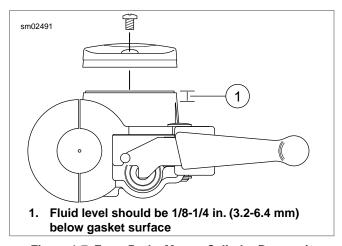
Figure 1-7. Front Brake Master Cylinder Reservoir
