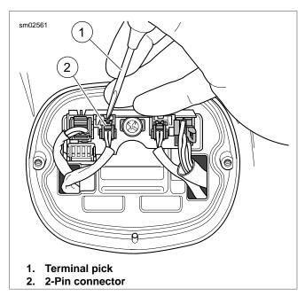
Figure 8-24. Removing 2-Pin Connectors
