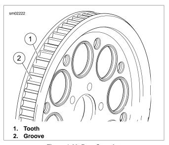
Figure 1-23. Rear Sprocket
