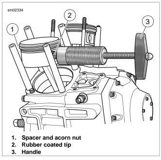
Figure 3-29. Piston Pin Remover (Part No. HD-42320-A)
