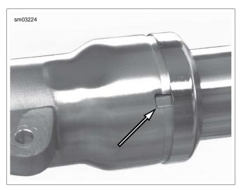
Figure 2-83. Notch in Slider
