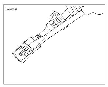
Figure A-16. Delphi Maxi-Fuse Housing: Bend Tang
