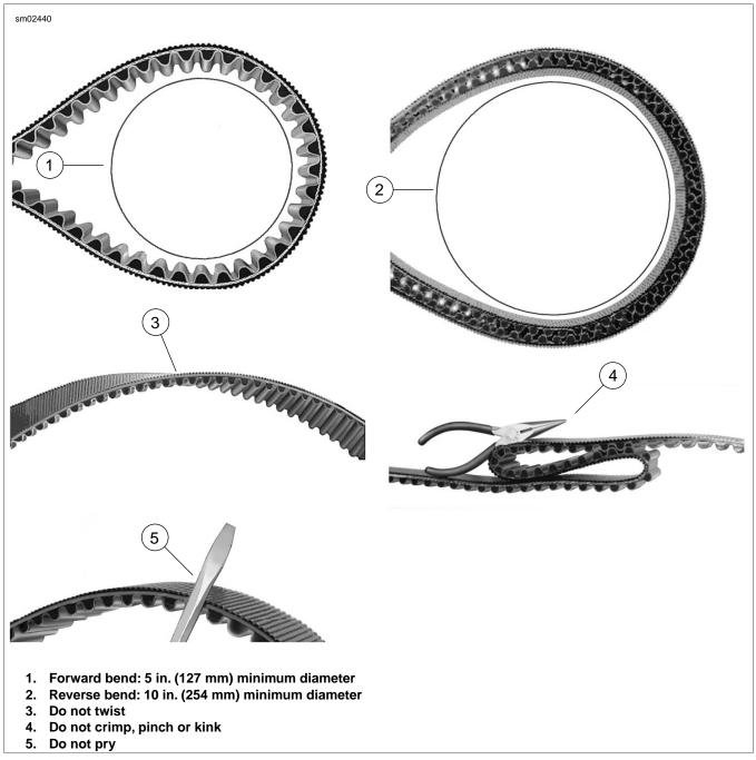
Figure 6-43. Proper Drive Belt Handling
