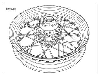
Figure 2-29. Wheel Completely Laced
