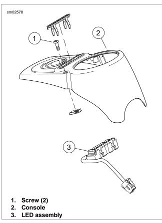
Figure 8-55. Indicator Lamp Assembly: FXDWG, FXDC, FXDF
