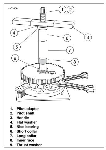
Figure 3-142. Press Inner Race onto Sprocket Shaft: Setup
