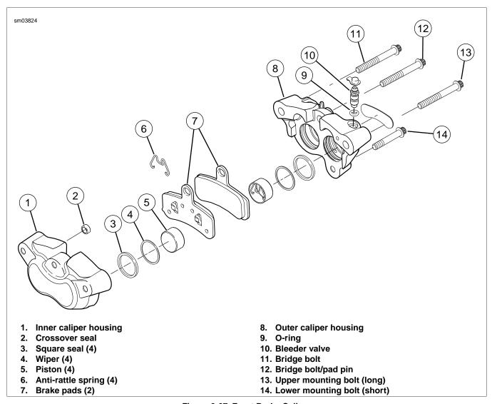
Figure 2-67. Front Brake Caliper
