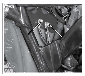
Figure 8-76. Vehicle Ground Studs
