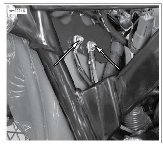
Figure 8-73. Vehicle Ground Studs
