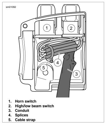
Figure 8-93. Upper Housing With Splices
