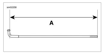
Figure 2-43. Measuring Spoke Length
