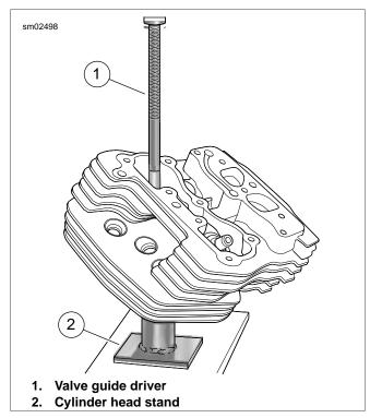
Figure 3-89. Remove Valve Guide
