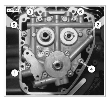
Figure 3-55. Cam Support Plate Torque Sequence
