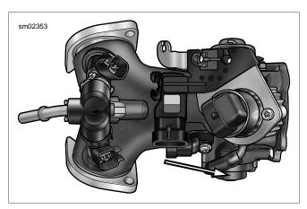
Figure 4-9. Throttle Position Sensor
