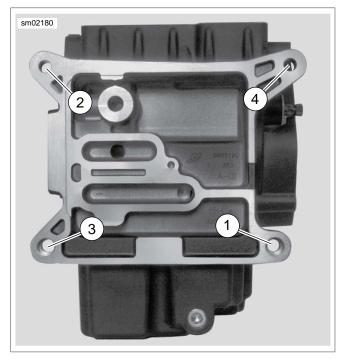
Figure 3-16. Transmission Housing to Crankcase Torque Sequence
