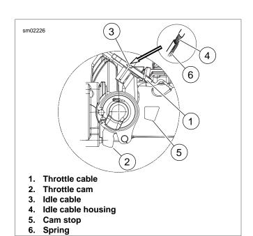
Figure 1-30. Induction Module Cable Connection
