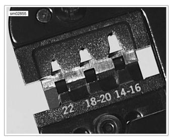
Figure A-34. Square Openings in Socket Locator Bar
