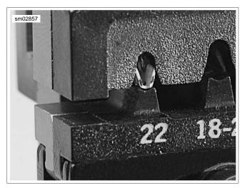
Figure A-36. Crimp Tails in Vertical Alignment between Punch and Die
