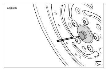
Figure 2-17. Installation Tool Support Plate
