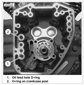
Figure 3-57. Oil Pump O-rings
