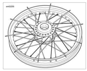
Figure 2-40. Completed Spokes: Top Flange Inner
