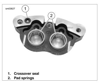
Figure 2-71. Front Caliper Pad Springs
