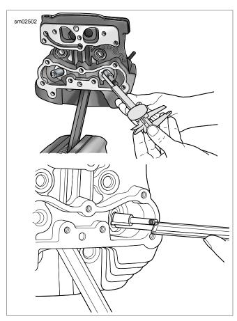
Figure 3-94. Checking Valve Stem Protrusion
