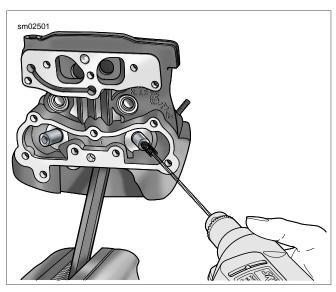
Figure 3-93. Honing Valve Guide Bore
