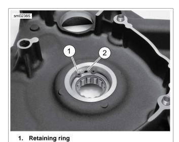
Figure 6-20. Retaining Ring Orientation
