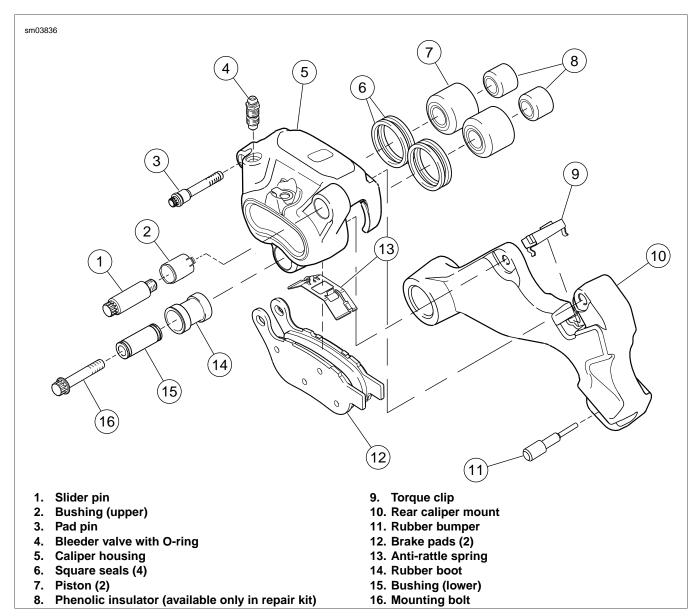
Figure 2-76. Rear Brake Caliper
