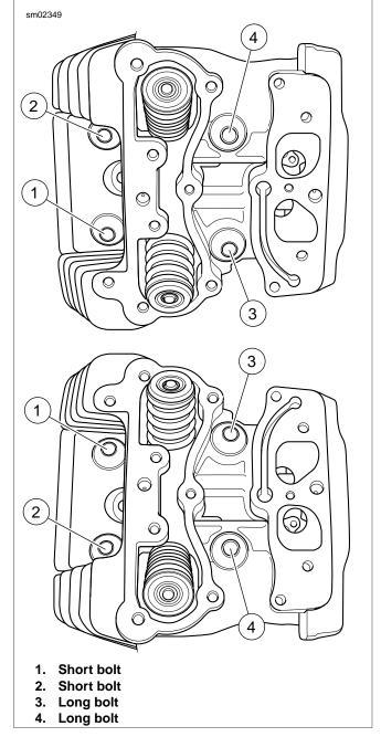
Figure 3-40. Cylinder Head Bolt Torque Sequence
