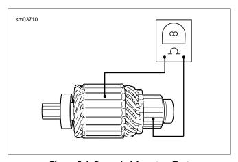
Figure 5-4. Grounded Armature Test
