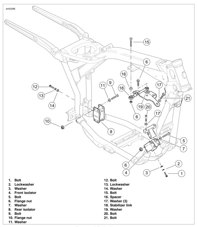
Figure 2-115. Engine Mounts
