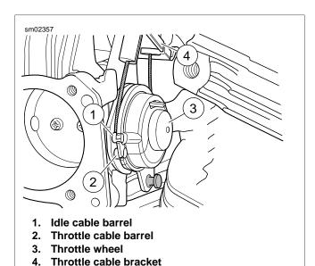
Figure 4-18. Throttle/Idle Cables
