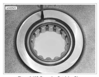
Figure 3-135. Removing Retaining Ring
