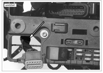
Figure 8-5. TSM/TSSM/HSFM Wiring
