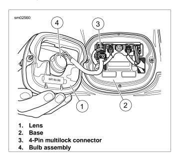
Figure 8-23. Tail Lamp: FXD, FXDC, FXDL
