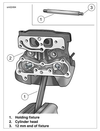
Figure 3-85. Cylinder Head Holding Fixture
