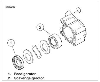
Figure 3-9. Oil Pump Gerotors
