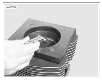
Figure 3-109. Measuring Ring Gap
