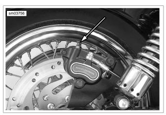
Figure 1-32. Rear Brake Bleeder Valve
