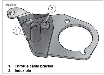
Figure 4-23. Throttle Cable Bracket
