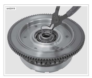
Figure 6-32. Clutch Hub Retaining Ring
