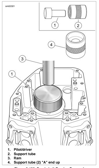
Figure 3-130. Crankshaft Bearing Removal
