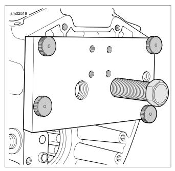
Figure 3-124. Installer Forcing Screw Installation
