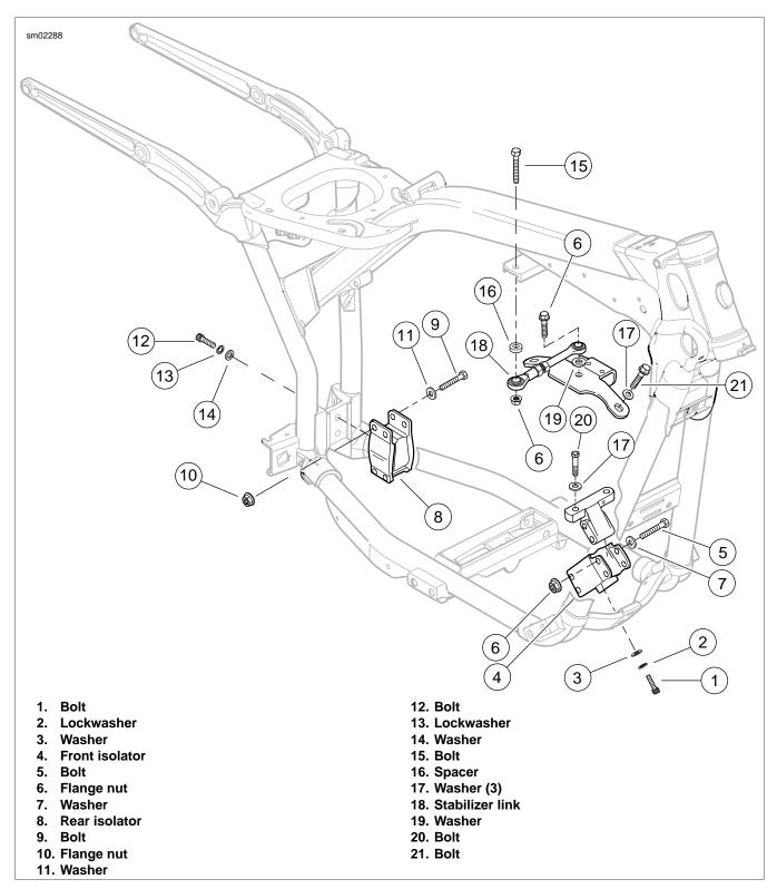
Figure 1-50. Engine Mounts
