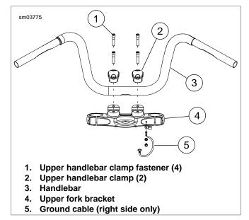
Figure 2-102. Handlebars: FXDB
