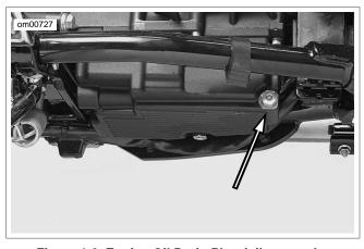
Figure 1-3. Engine Oil Drain Plug (oil pan under transmission, view from left side of vehicle)
