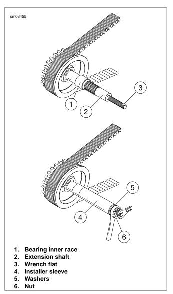
Figure 6-24. Installing Bearing Race
