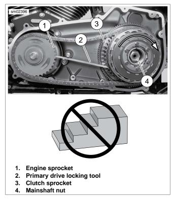
Figure 6-7. Removing Clutch Hub Mainshaft Nut
