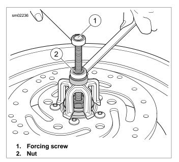
Figure 2-16. Remove Bearing
