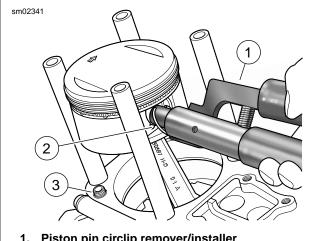
Piston pin circlip remover/installer
