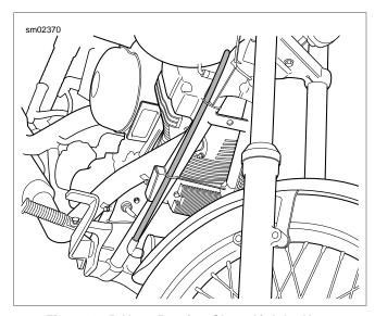
Figure 4-75. Hose Routing-Clean Air Inlet Hose
