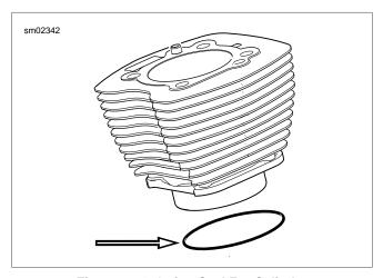
Figure 3-34. O-ring Seal For Cylinder
