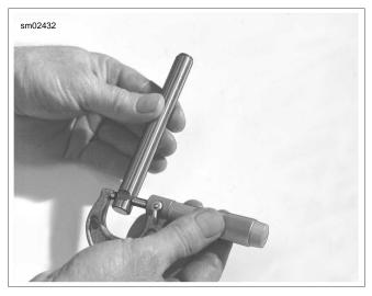
Figure 3-77. Checking Shaft to Support Plate Fit
