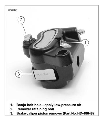
Figure 2-77. Removing Pistons
