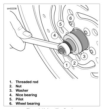
Figure 2-18. Installing Bearing
