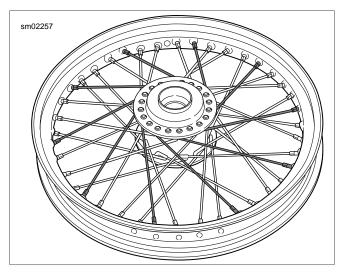
Figure 2-42. Completed Spokes: Top Flange Outer
