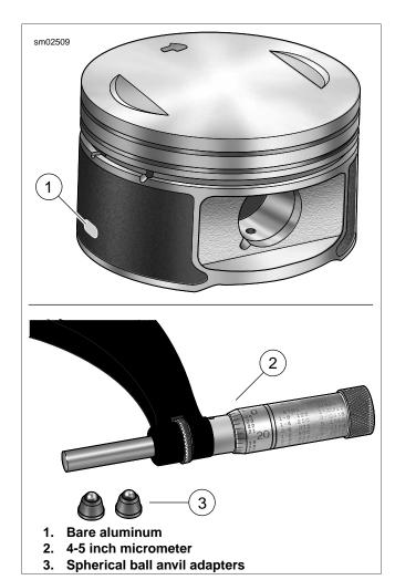
Figure 3-108. Measuring Running Clearance of Piston
