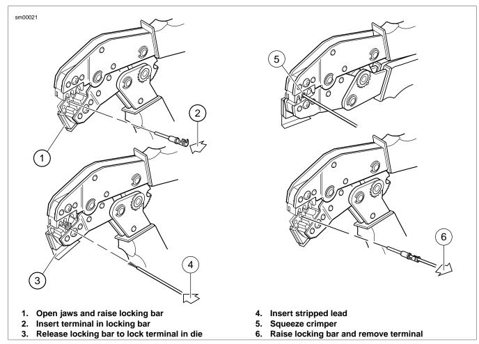
Figure A-23. Crimping a Deutsch Standard Terminal
