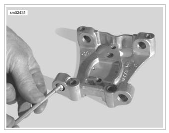
Figure 3-76. Checking Support Plate Bore
