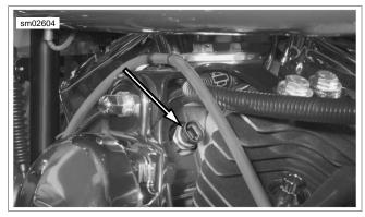
Figure 4-15. Engine Temperature Sensor
