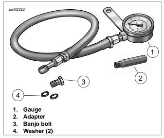
Figure 3-15. Oil Pressure Gauge Set
