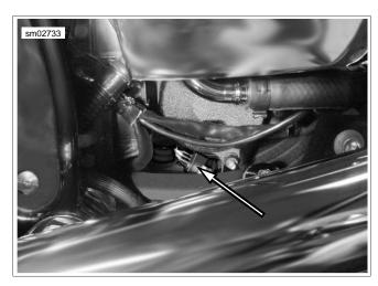
Figure 8-75. Vehicle Speed Sensor
