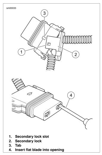
Figure A-15. Delphi Maxi-Fuse Housing: Remove Socket Terminals
