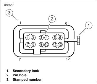
Figure A-51. Packard Micro 64 Connector: Housing
