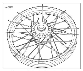
Figure 2-38. Setting Top Flange Inner Spokes
