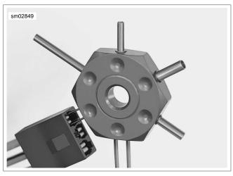
Figure A-10. Removing Autofuse Terminal from Ignition Switch
