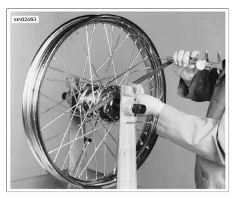
Figure 2-52. Front Wheel Hub Offset Dimension
