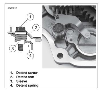
Figure 7-14. Detent Assembly
