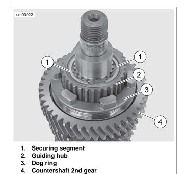
Figure 7-22. Securing Segment
