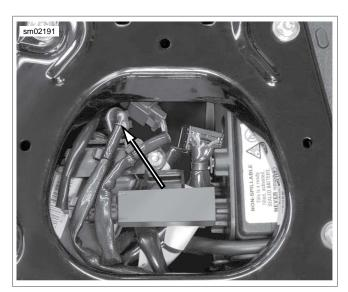
Figure 4-60. Rear O2 Connector and Harness
