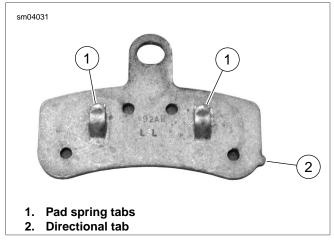
Figure 2-72. Front Brake Pad
