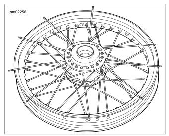
Figure 2-41. Beginning Spoke: Top Flange Outer
