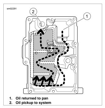
Figure 3-7. Oil Pan Baffles
