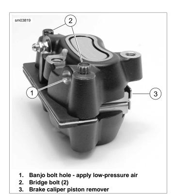
Figure 2-69. Removing Pistons
