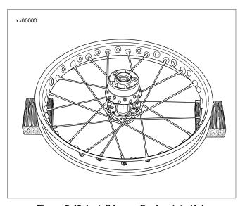
Figure 2-49. Install Lower Spokes into Hub
