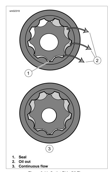
Figure 3-11. Outlet Side Oil Flow
