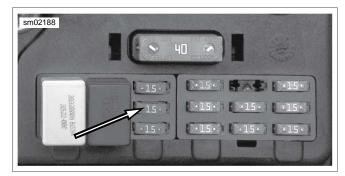
Figure 4-33. Fuel Pump Fuse
