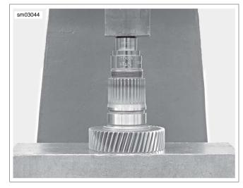
Figure 7-39. Pressing in Seal
