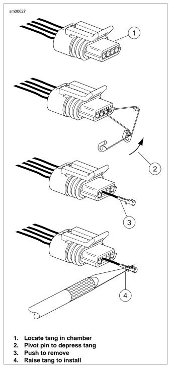
Figure A-39. 150 Metri-Pack Connector: Pull-to-Seat
