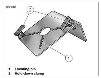
Figure 3-138. Flywheel Fixture (Part No. HD-44358)
