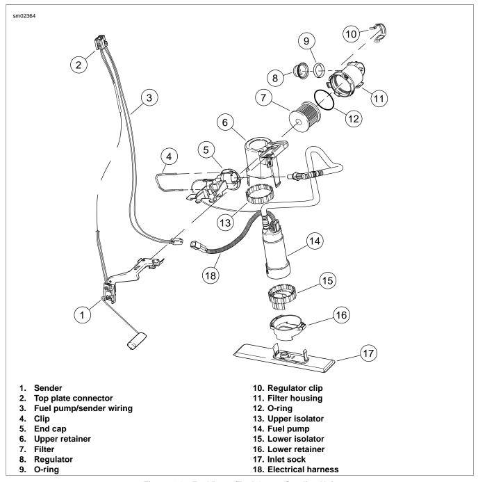
Figure 4-40. Fuel Pump/Fuel Gauge Sending Unit
