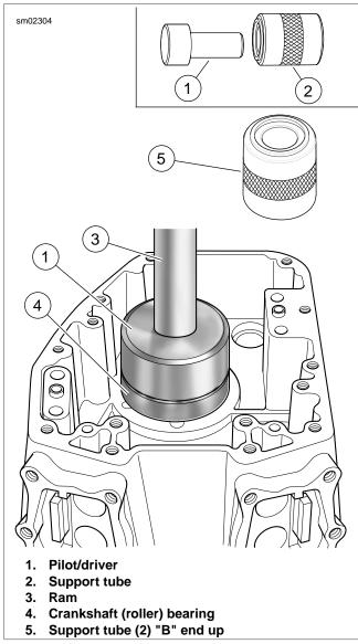
Figure 3-131. Crankshaft (Roller) Bearing Installation
