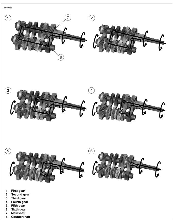
Figure 7-1. Transmission Power Flow
