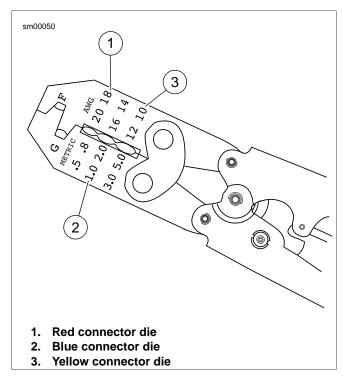
Figure A-54. Packard Crimping Tool (HD-38125-8)
