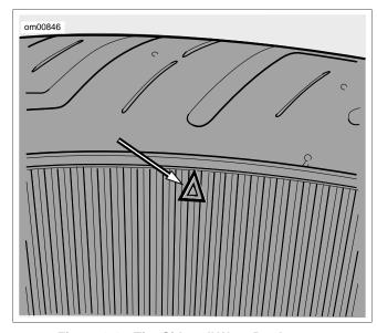
Figure 1-12. Tire Sidewall Wear Bar Locator
