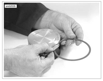
Figure 3-107. Measure Piston Ring Side Clearance
