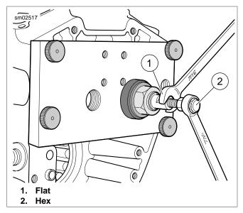
Figure 3-120. Expanding Collet by Turning Hex Clockwise
