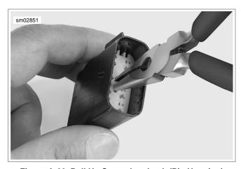
Figure A-29. Pull Up Secondary Lock (Pin Housing)
