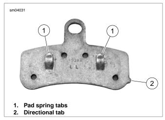
Figure 1-36. Front Brake Pad
