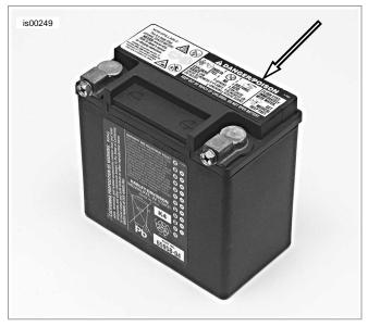
Figure 1-37. AGM Battery with Warning Label
