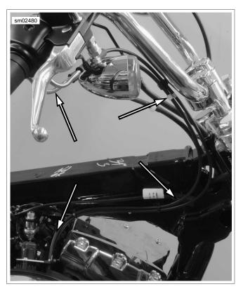
Figure 2-96. Throttle Cable Routing: FXDWG, FXDF (Typical)
