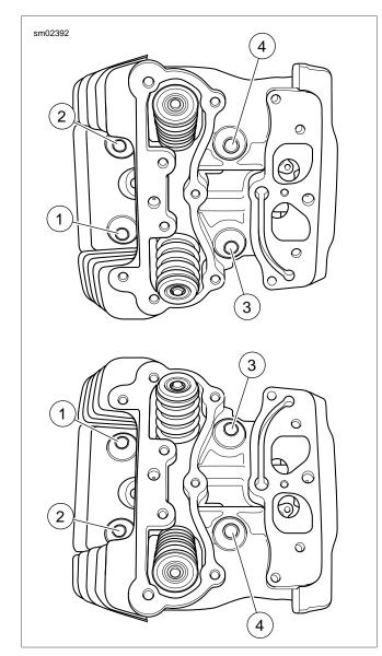
Figure 3-26. 1/4 Turn Head Bolts in Sequence
