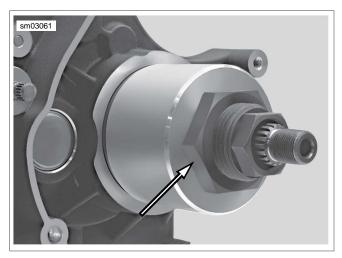
Figure 7-51. Install Nut (Part No. HD-47856-6)
