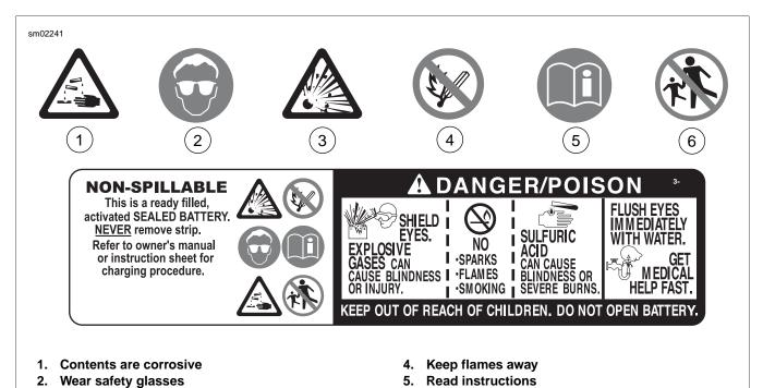
Figure 1-38. Battery Warning label
