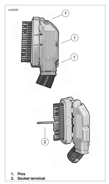
Figure A-48. Packard 100W Connector: Separate Halves of Socket Housing
