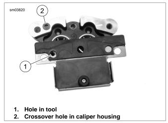
Figure 2-68. Installing Tool
