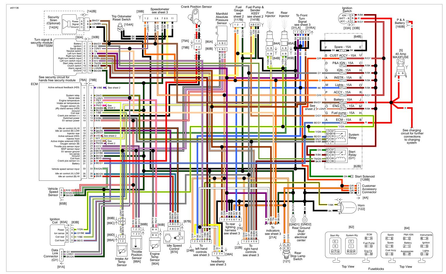
Figure B-13. 2008 ALL FXDWG, FXDC, FXDF DYNA DOM. and INT. MODELS, MAIN HARNESS, SHEET 1 OF 3
