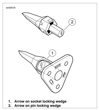
Figure A-19. Deutsch Connector: 3-Place Locking Wedges
