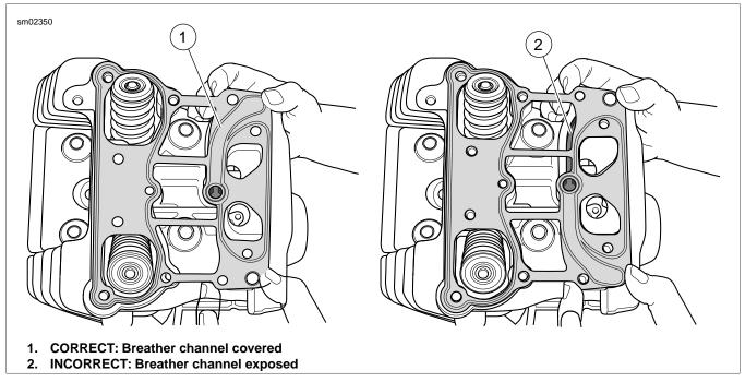
Figure 3-42. Install Rocker Housing Gasket (Rear Cylinder Shown)
