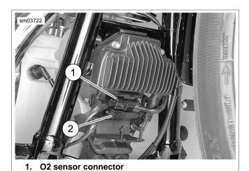
Figure 8-34. Front Electrical Caddy and Connectors
