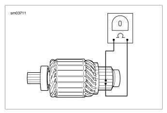
Figure 5-5. Armature Open Test
