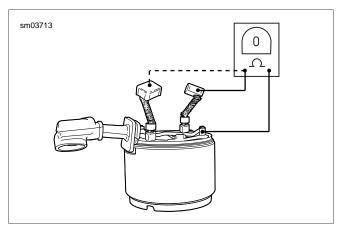
Figure 5-7. Open Field Test
