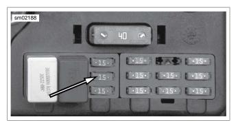
Figure 4-3. Fuel Pump Fuse
