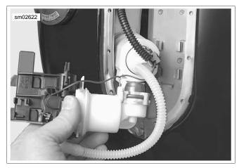
Figure 4-49. Fuel Pump Installation
