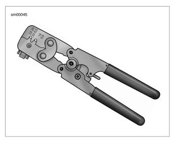
Figure A-52. Packard Micro 64 Terminal Crimper (HD-45929)
