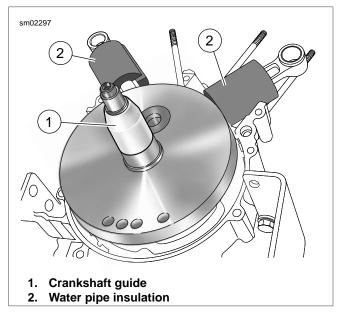
Figure 3-60. Crankshaft Guide (Part No. HD-42326-A)
