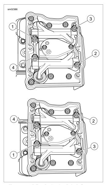
Figure 3-20. 1/4 Turn Rocker Arm Bolts in Sequence
