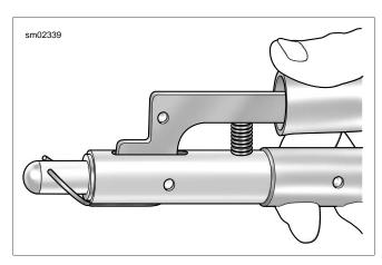
Figure 3-32. Aligning Circlip
