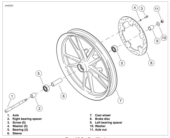
Figure 2-5. Cast Front Wheel
