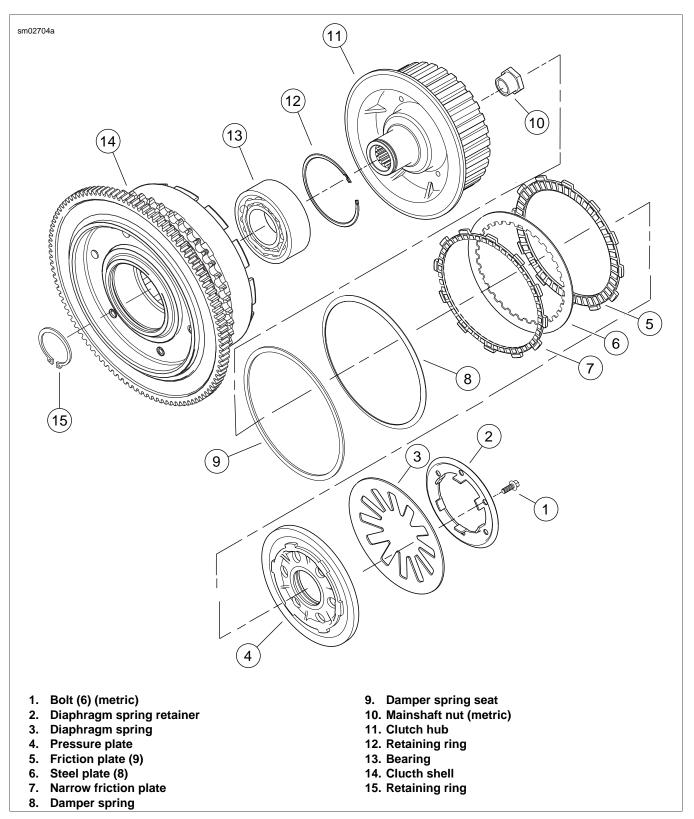
Figure 6-30. Clutch Shell Assembly
