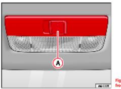
Fig. 62 Interior roof trim: front interior lights
