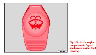
The **windscreen washer** and the **headlight washing system** are supplied with fluid from the windscreen washer fluid container in the engine compartment. The container holds approx. 2 litres; in vehicles with headlamp washers\* it holds approx. 4.5 litres.
