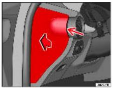
Fig. 146 Fuses in the dash panel
