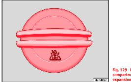
Fig. 129 In the engine compartment: Coolant expansion tank cap
