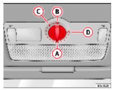
Fig. 55 Roof lining description: rotary sun roof control
