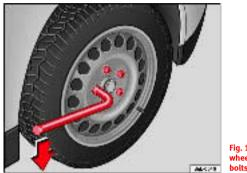
Fig. 141 Changing the wheel: loosen the wheel bolts
