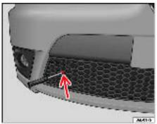
Fig. 172 Eye cover in the lower front grille.
