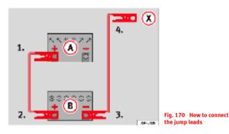
In  $\Rightarrow$  fig. 170, the flat battery is (A) and the charged battery (B).
