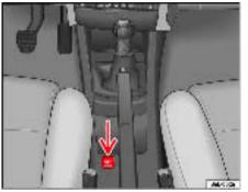
Fig. 99 Detail of the centre console: ESP button
