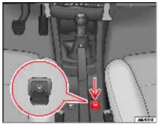
Fig. 87 Auxiliary audio connection
