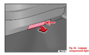
The light is activated when the tailgate is open, even when the ignition and lights are turned off. For this reason ensure that the tailgate is always closed.  $\blacksquare$
