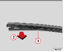
Fig. 132 Changing the rear window wiper blade
