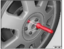
Fig. 144 Changing the wheel: hexagonal socket in screwdriver handle to turn the wheel bolts after they have been loosened
