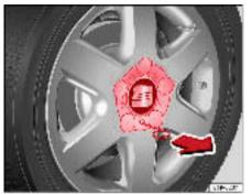
Fig. 139 Changing the wheel: Removing a hub cap
