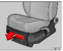
Fig. 81 Stowage compartment under the front passenger seat
