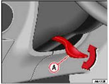
Fig. 97 Adjusting the steering wheel position
