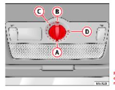
Fig. 54 Roof lining description: rotary sun roof control
