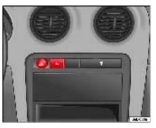
Fig. 60 Instrument panel: switch for hazard warning lights
