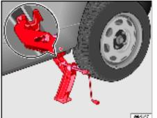
Fig. 143 Fitting the jack
