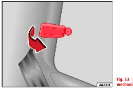
Fig. 53 Release lever for mechanical vent wing
