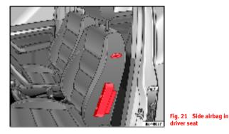
The side airbags are located in the driver seat and front passenger seat backrests  $\Rightarrow$  fig. 21. The locations are identified by the text "AIRBAG" in the upper region of the backrests.
