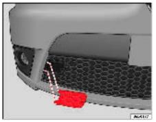
Fig. 173 Eye cover in the lower front grille.
