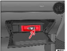
Fig. 89 USB connection\* in glove box on passenger side.
