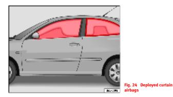
During some **side collisions** the curtain airbag is triggered on the impact side of the vehicle  $\Rightarrow$  fig. 24.
