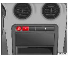
Fig. 59 Instrument panel: heated rear window switch The rear window heating only works when the engine is running. When it is switched on, a lamp lights up on the switch.
