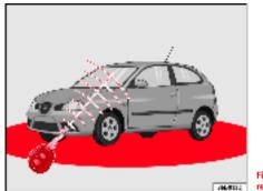
Fig. 49 Range of the remote control
