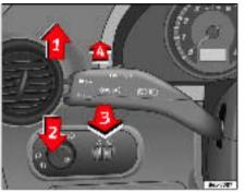
Fig. 61 Turn signal and main beam headlight lever
