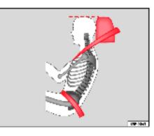
Fig. 13 Correct belt web and head restraint positions, viewed from side
