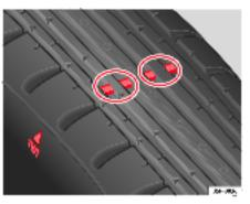
Fig. 134 Tyre tread wear indicators
