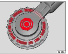
Fig. 133 In the engine compartment: Brake fluid reservoir cover
