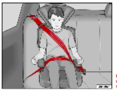
Fig. 29 Forward-facing child seat installed on rear seat.
