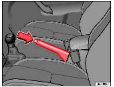
Fig. 105 Handbrake between the front seats
