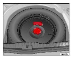
Fig. 138 Securing the defective wheel in the spare wheel well
