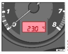
Fig. 38 Digital instrument panel display: outside temperature display.
