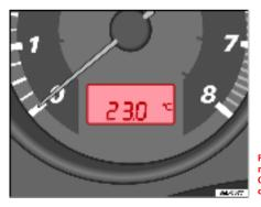
Fig. 36 Digital instrument panel display: Outside temperature display
