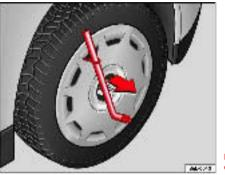
Fig. 140 Remove the complete hub cap
