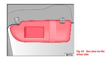
The sun visors for the driver and the front passenger can be pulled out of their mountings in the centre of the vehicle and turned towards the doors  $\Rightarrow$  fig. 65.
