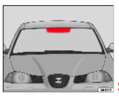
Fig. 69 Location of the electronic pricing device
