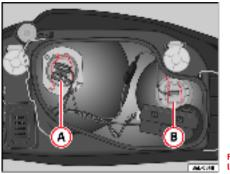
Fig. 151 Dipped headlight lamp
