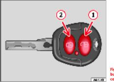
Fig. 48 Assignment of buttons on the remote control key
