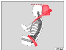
Fig. 4 Properly adjusted head restraint viewed from the side Adjust the head restraint properly to achieve maximum protection.
