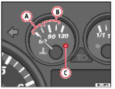
Fig. 33 Engine coolant temperature
