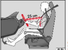
Fig. 1 The proper distance between driver and steering wheel
