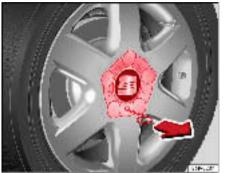
Fig. 131 Changing the wheel: Removing a hub cap
