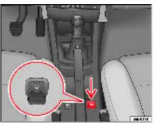
Fig. 84 Auxiliary audio connection
