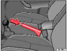
Fig. 101 Handbrake between the front seats
