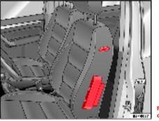
Fig. 21 Side airbag in driver seat
