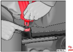
Fig. 15 Removing latch plate from buckle
