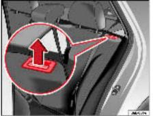
Fig. 75 Button for unlocking the rear backrest
