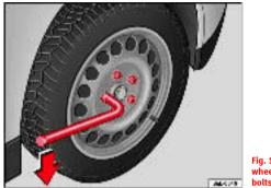
Fig. 133 Changing the wheel: loosen the wheel bolts
