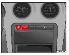
Fig. 59 Instrument panel: switch for hazard warning lights
