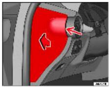
Fig. 138 Fuses in the dash panel
