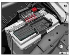
Fig. 139 Fuse box above battery
