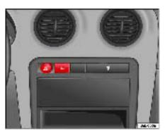
Fig. 58 Instrument panel: heated rear window switch The rear window heating only works when the engine is running. When it is switched on, a lamp lights up on the switch.
