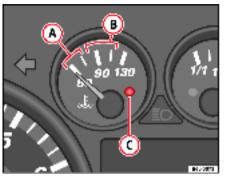
Fig. 33 Engine coolant temperature
