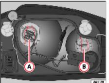
Fig. 144 Main beam lamp
