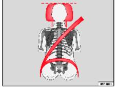
Fig. 69 Front view: head restraints and seat belts correctly adjusted
