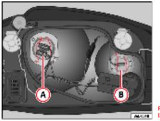
Fig. 143 Dipped headlight lamp
