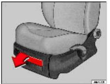
Fig. 78 Stowage compartment under the front passenger seat
