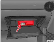
Fig. 85 iPod connection in glove box on passenger side.
