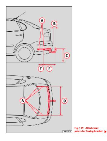
If a towing bracket is to be fitted after the vehicle is purchased, this must be completed according to the instructions of the towing bracket manufacturer.
