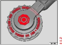
Fig. 128 In the engine compartment: Brake fluid reservoir cover
