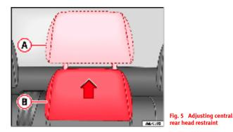
The central rear head restraint has 2 positions:
