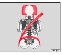
Fig. 12 Correct belt web and head restraint positions, viewed from front
