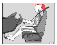
Fig. 2 Proper head restraint position for driver
