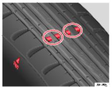
Fig. 129 Tyre tread wear indicators
