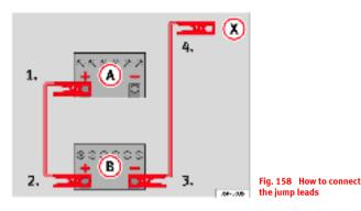
In  $\Rightarrow$  fig. 158, the flat battery is (A) and the charged battery (B).
