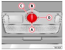
Fig. 54 Roof lining description: rotary sun roof control The sliding/tilting roof has a *roll-back function* which prevents larger objects getting trapped when the roof is closed. The roll-back function does not prevent fingers getting pinched against the roof opening. The sliding/tilting sunroof stops and opens again immediately if it is obstructed when closing.
