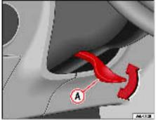
Fig. 93 Adjusting the steering wheel position
