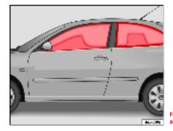
Fig. 24 Deployed curtain airbags
