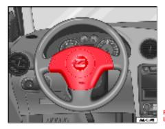
Fig. 17 Driver airbag located in steering wheel
