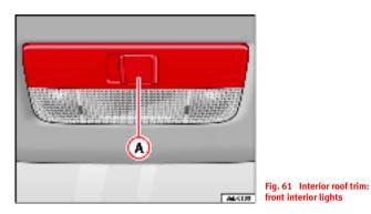
The switch  $\Rightarrow$  fig. 61 (A) is used to select the following positions:
