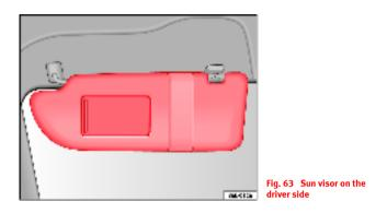
The sun visors for the driver and the front passenger can be pulled out of their mountings in the centre of the vehicle and turned towards the doors  $\Rightarrow$  fig. 63.
