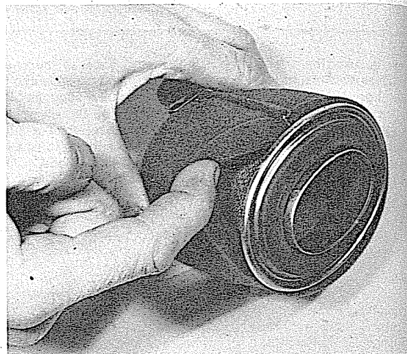
10.3 Peel element off frame for cleaning
