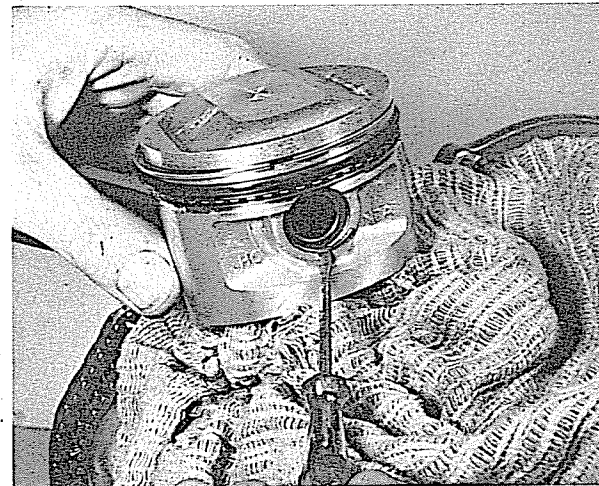
7.4 Pack crankcase mouth with rag, then displace circlips
