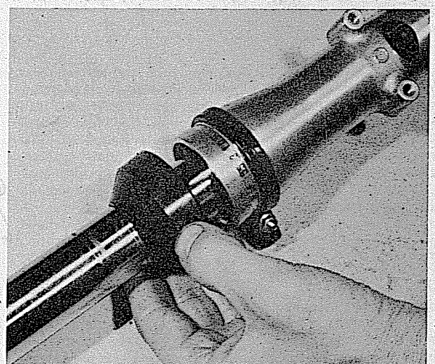
7.4a Displace dust seal from lower leg...
