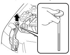
To inspect the washer fluid level in the front reservoir, pull off the cap. Then, holding your thumb over the hole in the center of the cap, lift it straight up. The fluid level can be seen from the fluid column in the pipe. Add fluid if necessary.
