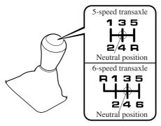
The vehicle is equipped with either a 5-speed or 6-speed manual transaxle. The shift pattern for each is shown above.
