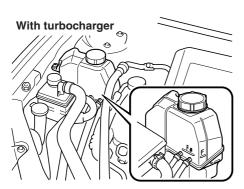
If it's at or near MIN or L, add enough coolant to the coolant reservoir to provide freezing and corrosion protection and to bring the level to MAX or F.
