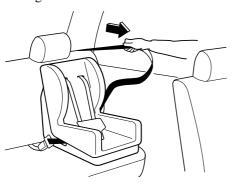
4. Push the child-restraint system firmly into the vehicle seat. Be sure the belt retracts as snugly as possible. Clicking from the retractor will be heard during retraction if the system is in the automatic locking mode. If the belt does not lock the seat down tight, repeat this step.
