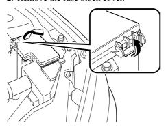
3. If any fuse but the MAIN fuse is blown, replace it with a new one of the same amperage rating.
