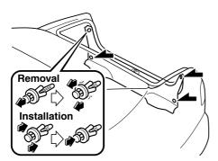
Pull the center of each plastic retainer and remove the retainers and partially open the trunk side trim.
