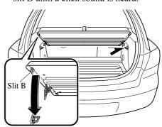
4. Rock the trunk board to make sure the board is installed securely.
