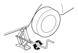
6. Remove the lug nuts by turning them counterclockwise; then remove the wheel and center cap.
