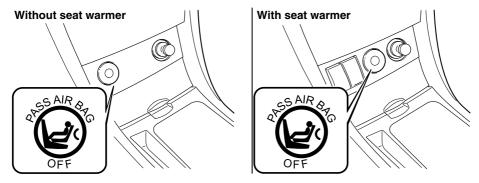
If the front passenger weight sensors are working properly, the indicator light illuminates when the ignition switch is turned to the ON position. After about 6 seconds it goes out.
