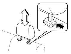
Adjust the head restraint so that the top is even with the top of the passenger's ears, never the passenger's neck.
