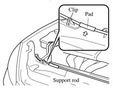
4. Secure the support rod in the stay hole indicated by the arrow to hold the hood open.
