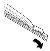
3. Remove the metal stiffener from each blade rubber and install them in the new blade.
