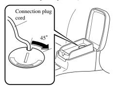
7. Pass the connection plug cord through the slit in the tray mat and then set the tray mat in place.
