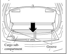
3. Rock the trunk board to make sure the board is installed securely.
