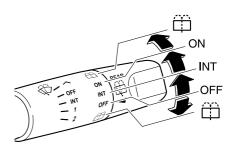
Turn the wiper on by turning the rear wiper/washer switch.
