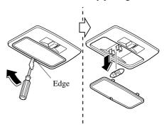
3. Install the new bulb in the reverse order of removal.
