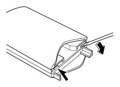
4. Press the portion of the battery indicated by A and remove the battery.
