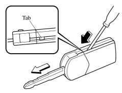
3. Insert a small screwdriver into the slot and gently pry open the transmitter.
