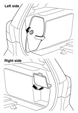
2. Turn the socket and bulb assembly counterclockwise and remove it.
