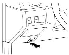
2. Slide the hood latch and lift the hood.
