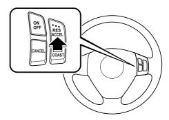
Your vehicle has a tap-up feature that allows you to increase your current speed in increments of 1.6 km/h (1 mph) by a momentary tap of the RES/ACCEL button. Multiple taps will increase your vehicle speed 1.6 km/h (1 mph) for each tap.
