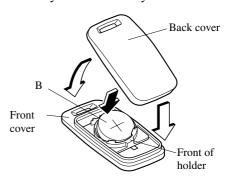
4. Align the front and back covers and snap the transmitter shut.
