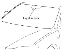
• The light sensor also works as a rain sensor for the auto-wiper control. Keep hands and scrapers clear of the windshield when the ignition switch is in the ON position as fingers pinched or the wipers and wiper blades damaged when they activate automatically. If you are going to clean the windshield, be sure the wipers are turned off completely this is particularly important when clearing ice and snow - when it is particularly tempting to leave the engine running.
