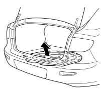
2. Turn the tire hold-down bolt counterclockwise with the lug wrench.
