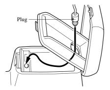
6. Make sure the connection plug cord is running through the cap slot; reinstall the cap and turn it clockwise (about 45° to the opened position).
