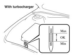
5. Pull it out again and examine the level. It's OK between Low or MIN and Full or MAX.
