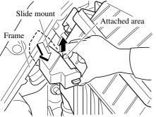
4. Remove the strap and raise the air filter.
