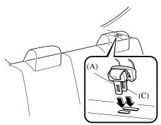
To pull out the seat belt, slide tongues with your finger, and slowly pull out the seat belt from the recess.
