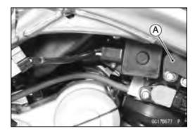
Subthrottle Sensor Input Voltage Inspection
