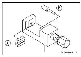
• Turn the pin holder until riveting pin touches link pin.
