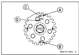
OMeasure the valve clearance of the valves for which the cam are turned away from each other.
