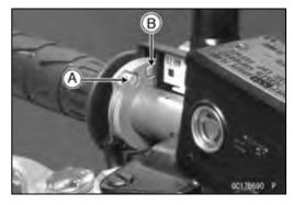
• Remove the throttle cable lower ends [A] from the throttle pulley.
