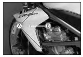
• Disconnect the turn signal lead connector [A].
