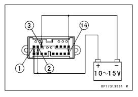
If each lights (LED) does not go on, replace the meter assembly.
