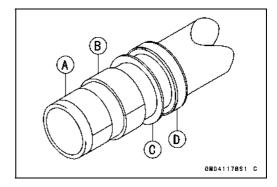
Remove the cylinder base [A] from the bottom of the outer tube
