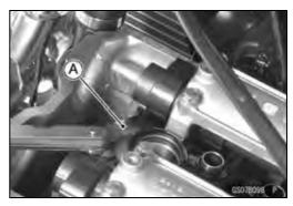
OEach piston has two inlet and two exhaust valves. Measure these two inlet or exhaust valves at the same crankshaft position.
