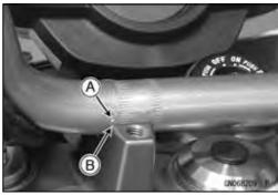
Tighten the front holder bolts first, and then the rear holder bolts. There will be a gap [A] at the rear part of the handlebar holder after tightening.
