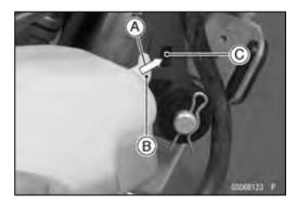
Place a container under the water pump drain bolt [A], then remove the drain bolt.
