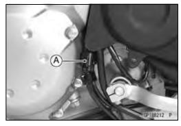
• Remove the oxygen sensor [A].
