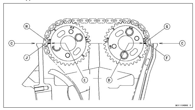
• Install the camshaft cap, while pushing the camshaft chain, tighten all camshaft bolts and chain guide bolts.
