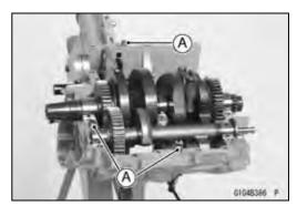
• Set the bearing groove [A] on the positioning ring [B] as shown.
