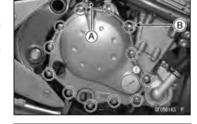
Turn the release lever [A] toward the rear as shown, and remove the clutch cover [B].
