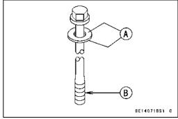
Apply molybdenum disulfide oil solution to flange [A] and the threads [B] of the M8 bolts which is tightening order is [7 ~ 10] only (see the next figure).
