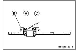
Press the mechanical seal [A] out of the housing with a bearing driver [B].
