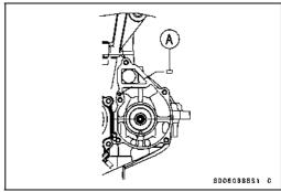
Replace the O-ring [A] on the water pump cover with a new one and grease it.
