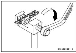
Set the plate holder (b) [A] and cutting and riveting pin [B] as shown.
