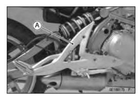
Remove the muffler body mounting bolts [A] and nut, and pull the muffler body [B] backward.
