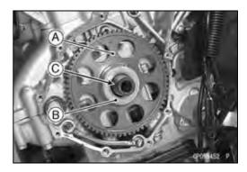
Install the alternator rotor [A] while turning [B] it counterclockwise.
