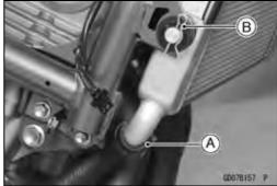
Pull [A] the radiator [B] toward the left, noting the baffle plate [C] on the cylinder head cover.
