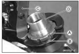
• To remove the bearing outer races [A] pressed into the head pipe [B], insert a bar [C] into the recesses of head pipe, and applying it to both recess alternately hammer it to drive the race out.
