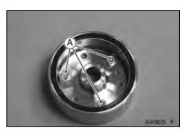
Remove: Starter Motor Clutch [A]
