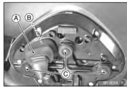
Meter, Gauge Disassembly
