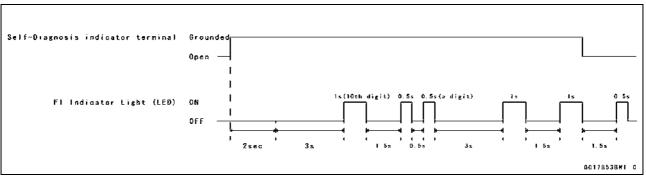
Olf the problem is with the following parts, the ECU cannot memorize these problems, the FI indicator light (LED) doesn't go on, and no service codes can be displayed.
