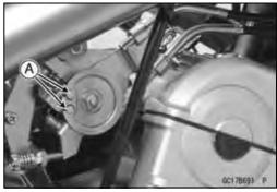
After removing the throttle body assy, stuff pieces of lint -free, clean cloth into the throttle body holders.
