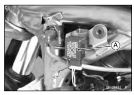
Connect one 12 V battery and turn signal lights as indicated in the figure, and count how may times the lights flash for one minute.
