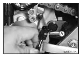
Set the hand tester [A] to the x 1 Ω range and connect it to the terminals in the oxygen sensor lead connector [B].
