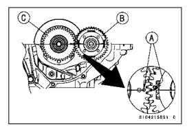
• Be sure to hang the camshaft chain [A] on the crankshaft.
