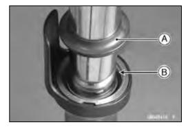
• Separate the inner tube [A] from the outer tube [B].
