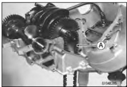
• Be sure that the dowel pins [A] are in position.
