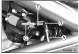
Push and pull [A] the fuel hose joint [B] back and forth more than two times and make sure it is locked and doesn't come off.
