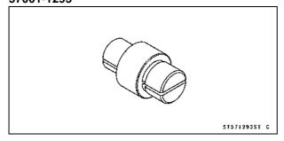
Bearing Remover Shaft,  $\phi$ 13: 57001-1377
