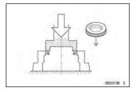
Apply specified grease to the lip of seal before installing the seal.
