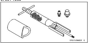
Piston Pin Puller Adapter C: 57001-1657
