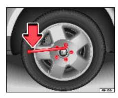
Fig. 177 Changing the wheel: loosen the wheel bolts
