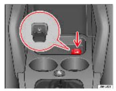
Fig. 120 Auxiliary audio connection
