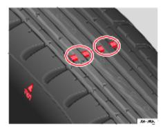
Fig. 173 Tyre tread wear indicators
