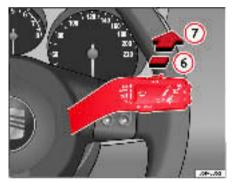
Fig. 89 Windscreen wiper and windscreen wash lever: rear window wiper
