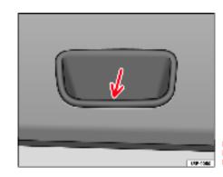
Fig. 67 Detail of the inside of the tailgate: hand grip
