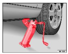
Fig. 179 Fitting the jack
