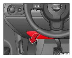
Fig. 183 Left side of dash panel: Fuse box cover
