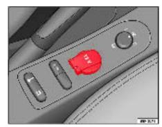
Fig. 118 Socket, centre console, front
