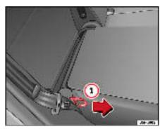
Fig. 99 Folding or opening the rear seat
