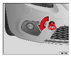
Fig. 207 Front towing eye for vehicles with fourwheel drive
