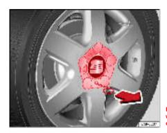
Fig. 176 Changing the wheel: Removing a hub
