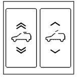
There are two switches in the overhead console that operate the sunroof.
