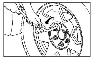
Use the wheel wrench to loosen all the wheel nuts. Turn the wheel wrench counterclockwise to loosen the wheel nuts. Do not remove the wheel nuts yet.
