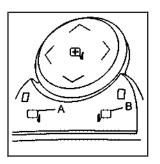
If your vehicle is equipped with outside power mirrors, the controls are located on the driver's door armrest.
