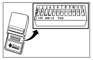
If you do not know if your garage door opener is a fixed code or rolling code device, open your garage door opener's remote control battery cover. Your garage door opener is a fixed code device if a panel of DIP switches is present. If not, your garage door opener is a rolling code device.
