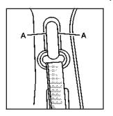
To move it down, squeeze the buttons (A) on the sides of the height adjuster and move the height adjuster to the desired position.
