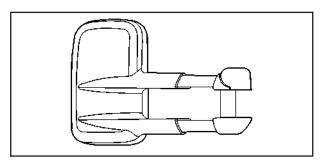
If your vehicle is equipped with this trailer towing type mirror, they can be adjusted so you can have a clear view of the objects behind you. Manually pull out the mirror head to extend it for better visibility when towing a trailer.
