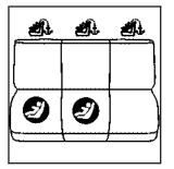
② (Lower Anchor): Seating positions with two lower anchors.
