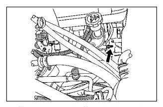
The remote negative (-) terminal is a stud located on the right front of the engine, where the negative battery cable attaches.
