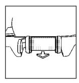
3. Unlatch the seat from the floor by pulling the carrying handle, located at the rear of the seat, rearward.
