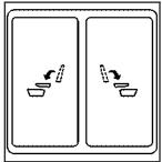
Overhead Console Buttons shown, Panel Button similar  From the front seats, press one of the automatic seat release buttons located on the overhead console.
