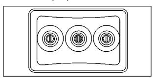
The A/V jacks are located on the rear of the floor console. The A/V jacks allow audio or video signals to be connected from an auxiliary device such as a camcorder or a video game unit to the RSE system. Adapter connectors or cables may be required to connect the auxiliary device to the A/V jacks. Refer to the manufacturer's instructions for proper usage.
