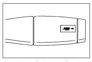
Your vehicle has a Tow/Haul mode. The selector button is located on the end of the column shift lever. You can use this feature to assist when towing or hauling a heavy load or if there is a need to charge a battery installed in a trailer. See *Towing a Trailer on page 416* for more information.
