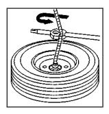
6. Use the wheel wrench hook that allows you to pull the hoist cable towards you, to assist in reaching the spare tire.
