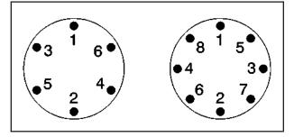
Tighten the nuts firmly in a crisscross sequence as shown by turning the wheel wrench clockwise.
