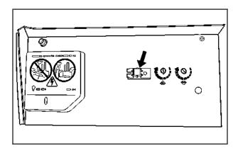
Go to the garage. Locate the garage door motor head and press and release the "learn" button.
