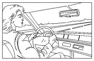
An emergency like this requires close attention and a quick decision. If you are holding the steering wheel at the recommended 9 and 3 o'clock positions, you can turn it a full 180 degrees very quickly without removing either hand. But you have to act fast, steer quickly, and just as quickly straighten the wheel once you have avoided the object.
