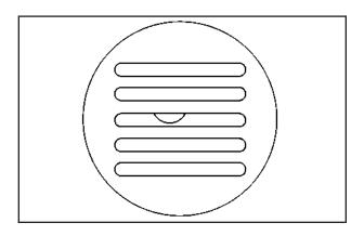
The interior temperature sensors located in the headliner above the driver side seat and in the headliner above the second row seats measure the temperature of the air inside your vehicle.
