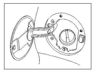
The tethered fuel cap is located behind a hinged fuel door on the driver's side of the vehicle. For vehicles with E85 fuel capability, a yellow cap with the words "E85 or gasoline" will appear.
