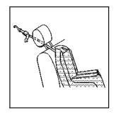
If the position you are using has an adjustable head rest/restraint and you are using a single tether, raise the head rest/restraint and route the tether under the head rest/restraint and in between the head rest/restraint posts.
