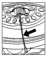
Check under the vehicle to see if the cable end is visible. If the cable is not visible, proceed to Step 6.
