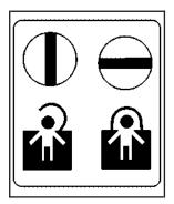
The rear door security locks are located on the inside edge of each rear door. You must open the rear doors to access them. The label depicting lock and unlock positions is located near the lock.
