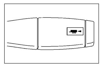
Press this button at the end of the shift lever to enable/disable the tow/haul mode.
