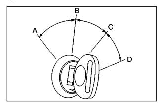
Use the key to turn the ignition switch to four different positions.
