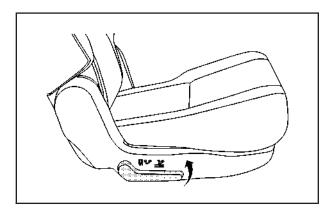
2. Lift the lever, located on the outboard side of the seat, to release the seatback.
