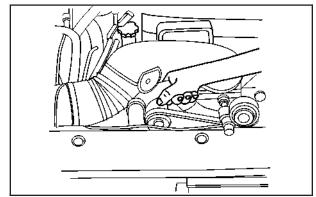
4. With the coolant surge tank pressure cap off, start the engine and let it run until you can feel the upper radiator hose getting hot. Watch out for the engine cooling fan.
