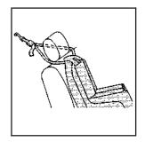
If the position you are using has an adjustable head rest/restraint and you are using a dual tether, route the tether around the head rest/restraint.
