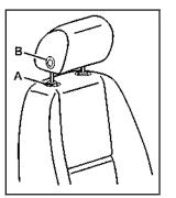
Pull the head restraint up to raise it. To lower the head restraint, press the release button (A), located on the top of the seatback, while you push the head restraint down.
