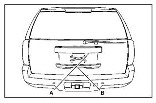
To open the liftglass, press the button on the underside of the license pocket applique (A). The liftglass can also be opened by pressing the liftglass release button on the RKE.
