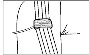
3. Be sure that the belt is not twisted and it lies flat. The elastic cord must be under the belt and the guide on top.
