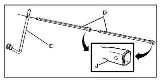
3. Assemble the two jack handle extensions (D) and wheel wrench (E) as shown.
