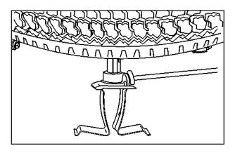
8. Attach the jack handle, extension, and wheel wrench to the jack and place it (with the wheel blocks) under the vehicle toward the front of the rear bumper.
