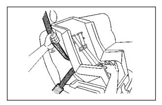
To tighten the belt, push down on the child restraint, pull the shoulder portion of the belt to tighten the lap portion of the belt and feed the shoulder belt back into the retractor. If you are using a forward-facing child restraint, you may find it helpful to use your knee to push down on the child restraint as you tighten the belt. You should not be able to pull more of the belt from the retractor once the lock has been set.
