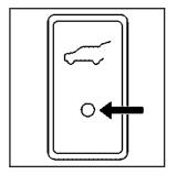
To change the liftgate to manual operation, toggle the switch on the overhead console to the "Disable" position indicated by a circle.
