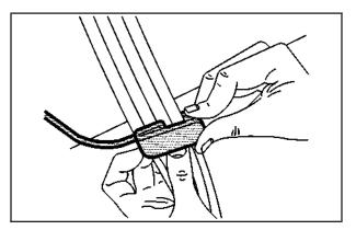
Slide the guide under and past the belt. The elastic cord must be under the belt. Then, place the guide over the belt, and insert the two edges of the belt into the slots of the guide.
