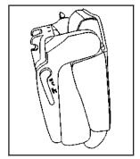
Lift the same lever again to release the rear of the seat from the floor. The seat will tumble forward.
