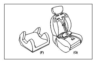
A booster seat (F-G) is a child restraint designed to improve the fit of the vehicle's safety belt system. Some booster seats have a shoulder belt positioner, and some high-back booster seats have a five-point harness. A booster seat can also help a child to see out the window.
