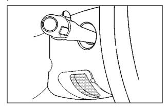
The tilt steering wheel lever is located on the lower left side of the column.
