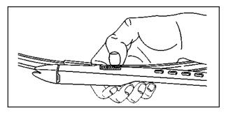
Squeeze the grooved areas on each side of the blade, and rotate the blade assembly away from the arm connector.
