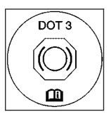
Your brake master cylinder reservoir is filled with DOT-3 brake fluid. See *Engine*Compartment Overview on page 450 for the location of the reservoir.
