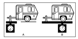
The trailer tongue weight (A) should be 10 percent to 15 percent of the total loaded trailer weight, up to a maximum of 600 lbs (272 kg) with a weight carrying hitch. The trailer tongue weight (A) should be 10 percent to 15 percent of the total loaded trailer weight, up to a maximum of 1,000 lbs (453 kg) for the 1500 series and up to a maximum of 1,500 lbs (680 kg) for the 2500 series with a weight distributing hitch.
