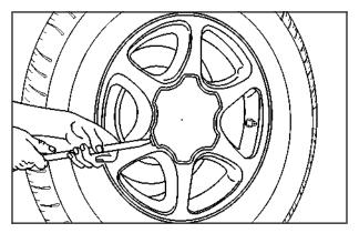
Remove the center cap, if your vehicle has one, by placing the chisel end of the wheel wrench in the slot on the wheel and gently pry the cap out. If the wheel has bolt-on wheel covers, loosen the plastic nut caps by turning the wheel wrench counterclockwise. If needed, finish loosening them by hand. The nut caps will not come off. Using the flat end of the wheel wrench, pry along the edge of the cover until it comes off.
