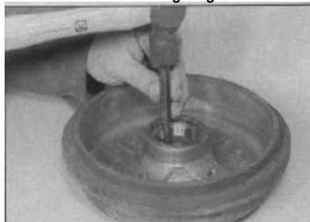
10.7 Drive the outer races out of position using a hammer and punch
