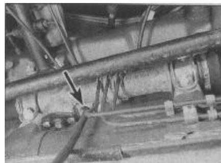
17.5 Clutch cable hole (arrowed) in the steering gear housing
