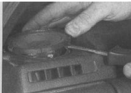
**17.2a Depress the tabs to release the loudspeaker from the fascia**
