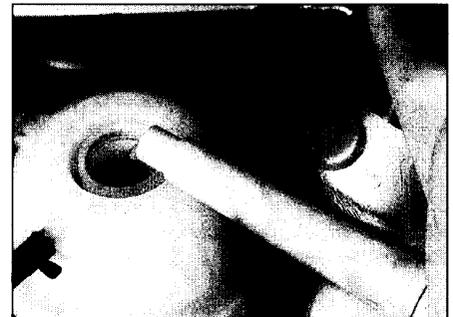
3 Add a mixture of water and antifreeze to the expansion tank until the coolant level is halfway between the level marks. Refit the cap and tighten it securely.
