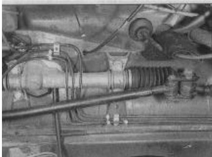
**17.10a Steering gear location (engine removed from car)**
