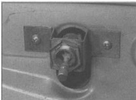
20.6 Exterior mirror control locknut and control knob on the inside of the door
