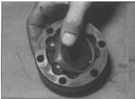
**3.12 The retaining circlip on the driveshaft inner joint**
