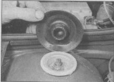
2.10a Removing the front suspension strut top cap
