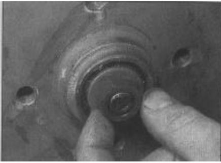
7.4a . . . then unscrew the retaining nut. . .
