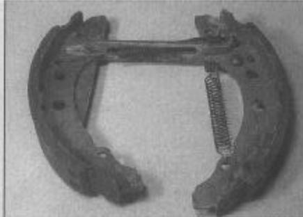
**5.10a Prior to dismantling, note the correct fitted location of the shoe components**
