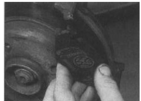
4.5 Removing the front brake pads
