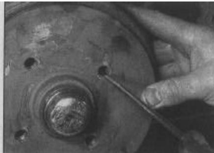
7.7 Release the brake shoes by inserting a screwdriver through the drum hole
