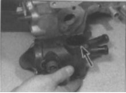
**4.2 Remove the thermostat housing together with its O-ring (arrowed)**
