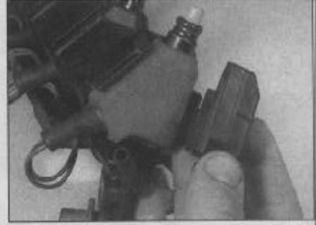
5.37a Unclip both halves of the plastic shielding from the injector body
