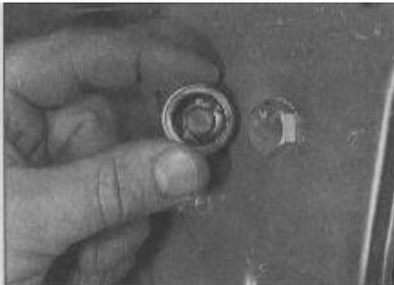
**25.14a Remove the cap for access to the rear seat belt inertia reel mounting bolt**
