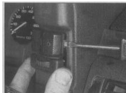
**4.7a Using a screwdriver to prise out the lighting switch**
