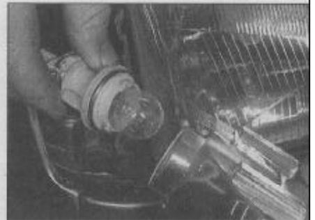
**5.14b** . . . then remove the bulbholder. . .
