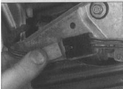
13.3a Disconnect the wiring plug . . .
