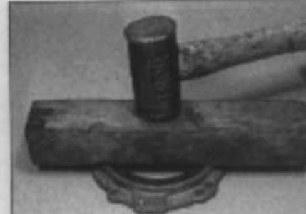
6.16 Driving the new oil seal into its housing
