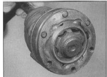
2.5 The driveshaft inner joint
