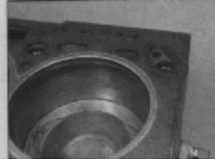
**9.30b** The gasket part number should face upwards
