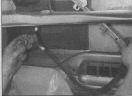
15.4 Removing the window regulator through the door aperture
