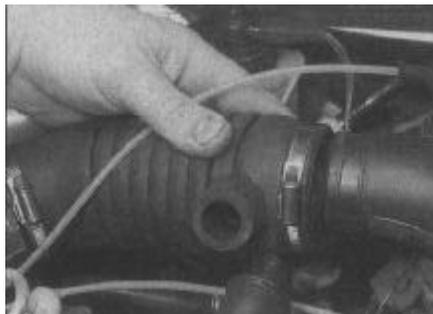
5.24a Slacken the clips and detach the inlet air ducting from the top of the throttle body inlet
