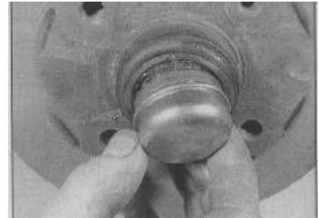
10.3a Removing the rear wheel hub cap
