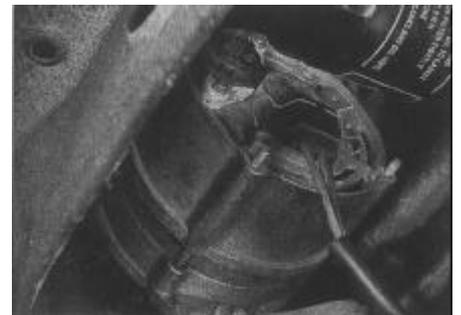
6.2 Release the clip and pull the multi-plug from the rear of the alternator
