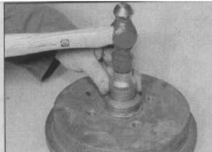
10.9 Drive the outer races securely into position using a socket on the outer edge
