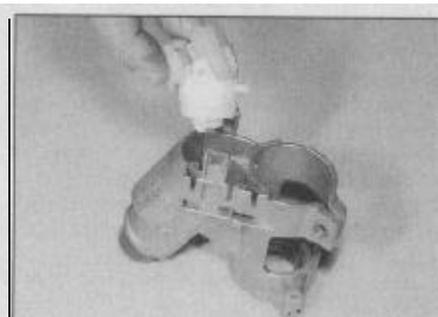
16.8b . . . and remove the ignition switch from the steering column lock assembly
