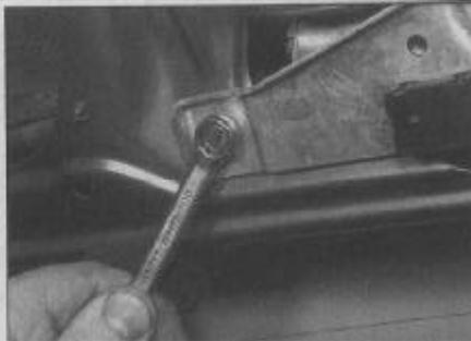
13.3b . . . unscrew the mounting bracket bolts . . .
