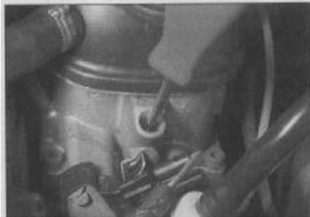
10.3a Idle speed adjustment screw location
