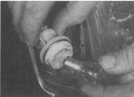
**5.14c** . . . and remove the front direction indicator bulb
