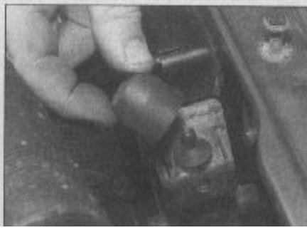
3.5b Removing the radiator upper mounting rubbers
