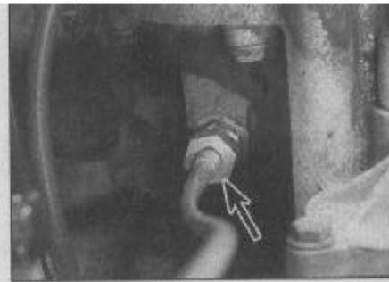
6.2 Speedometer drive cable locknut (arrowed) at the differential casing
