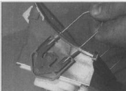
8.3b The special tools are used to hold in the side clips
