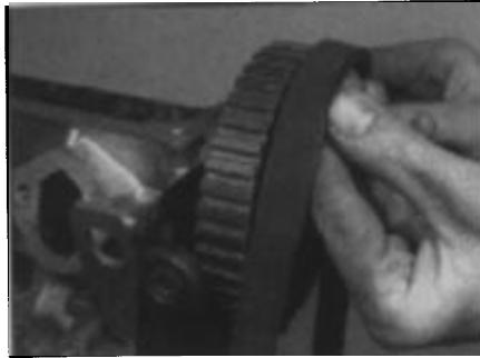
4.6 Releasing the timing belt from the camshaft sprocket
