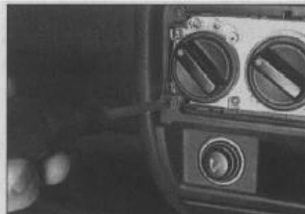
4.11a Removing the ashtray insert mounting screws
