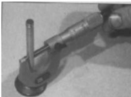
**4.40 Measure the diameters of the valve stems at several points along their lengths using a micrometer**
