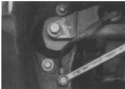
2.18 Unbolting the engine earthing strap
