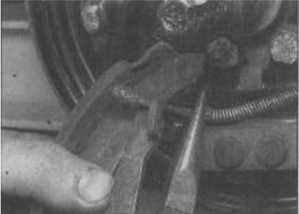
**5.9b Disconnecting the handbrake cable from the trailing shoe**
