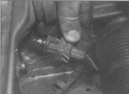
**5.10** Removing the front sidelight bulbholder
