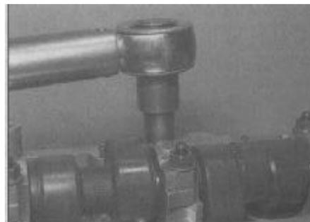
4.65 Tightening the camshaft bearing cap nuts
