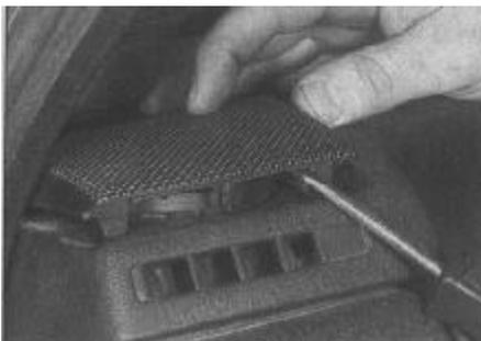
**17.1 Use a screwdriver to carefully prise the loudspeaker grille from the fascia panel**
