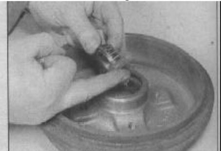
10.10 Work grease into the taper roller bearings prior to fitting them to the hub
