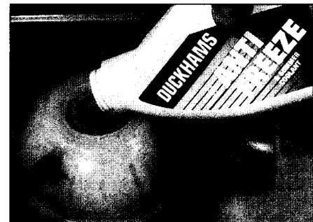
23.24 Topping up the cooling system with antifreeze
