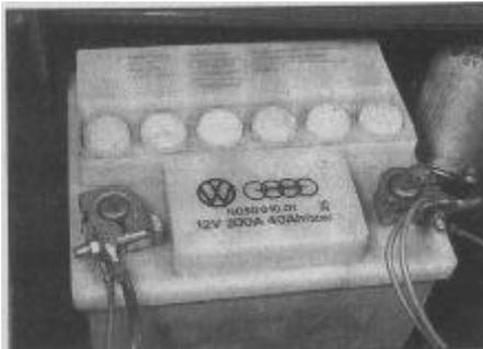
2.1 The battery is located under the bonnet, on the right-hand side of the bulkhead
