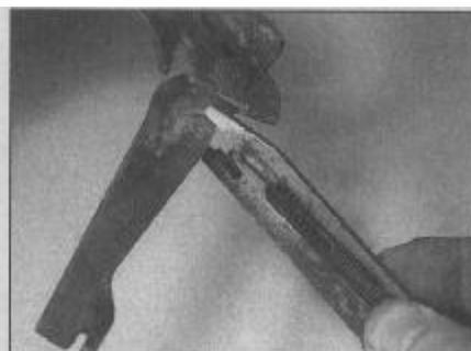
**5.11b . . . and remove the pushrod from the trailing shoe**
