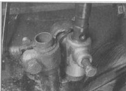
2.16a Disconnecting the shift rod coupling
