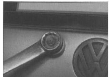
13.2a Unscrew the tailgate wiper motor outer nut . . .
