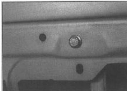
15.6 Bolt securing the front window channel
