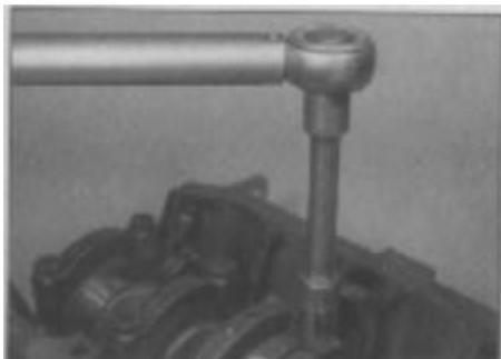
10.18 Tightening the main bearing bolts
