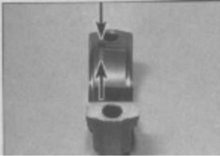
**12.17 Big end bearing shell lug and locating recess (arrowed)**
