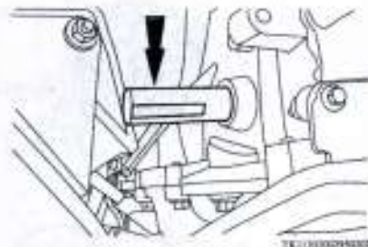
Fig. 136 Mazda 2.3L 4 Cyl. (Part 2 of 2). 2001-04 B2300 (crankshaft timing peg installation)
