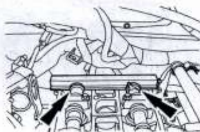
Fig. 19 Ford 2.3L (Part 1 of 2). 2001-04 Ranger (position camshaft alignment tool in slots on back of camshafts)
