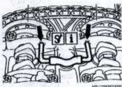
Fig. 158 Mercedes-Benz 119. Camshaft With Holding Tool
