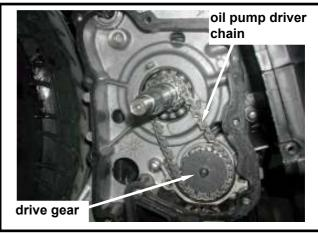
Install oil pump outer cover (2 bolts).
