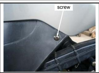
Remove the 4 screws between the rear center cover and the left/right body cover.
