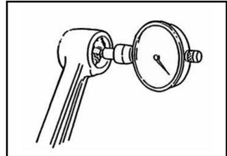
Measure the inner diameter of piston pin hole.
