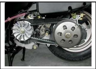
Install the clutch with universal fixture, and then tighten nut to specified torque value.
