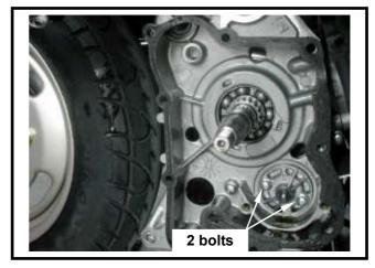
Install oil pump driver chain and drive gear.
