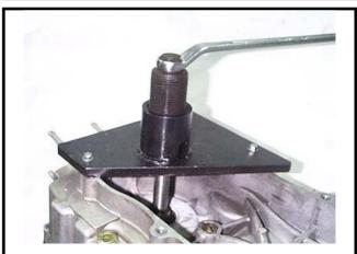
Remove the crankshaft from the right crankcase.
