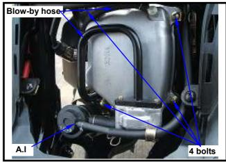
Remove the 2 cylinder head mounting bolts from cylinder head left side cover.
