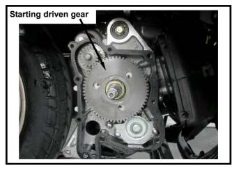
Hold the starting driven gear with the universal fixture.
