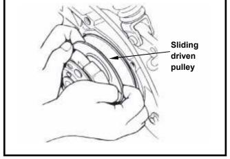
Install the clutch set with driving belt onto the driving shaft.
