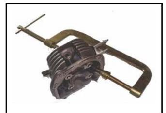
Tap valve stem to make valve retainer and valve stem sealing properly.
