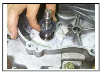
Press-fit the oil seal to specified position with the oil seal installer (25x37x6).
