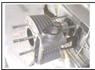
Remove cylinder gasket and lock pins
