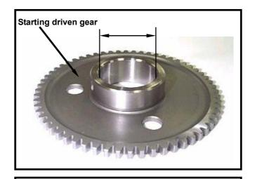
Check the starting reduction gear and shaft for wear or damage.
