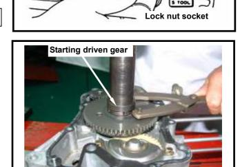
Remove starting clutch, starting reduction gear, and shaft.
