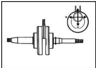
Place the crankshaft onto a V-block and measure run-out of the crankshaft with dial gauge.
