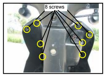
Remove the screw on the front inner box.
