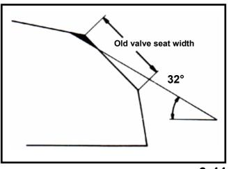
Use 60° cutter to cut a quarter lower part out. Remove the cutter and check new valve seat.
