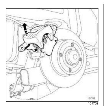
☐ Turn the brake callipers upwards.
