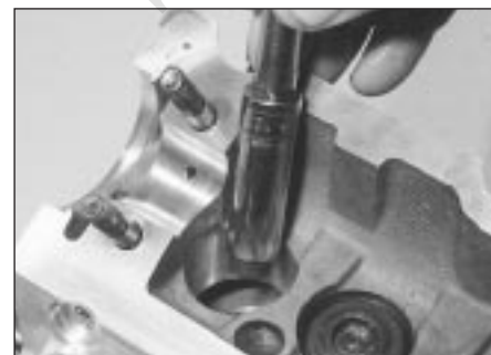
9.2 Fitting a valve stem oil seal using a socket
