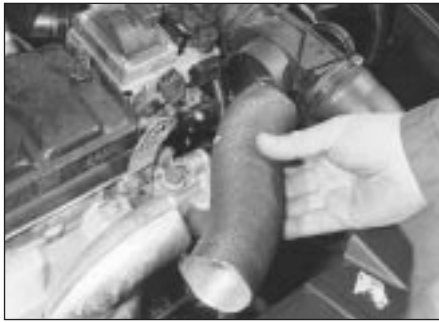
15.1 Remove the hot-air intake hose . . .
