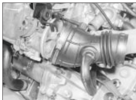
12.6 Detach the plastic duct
