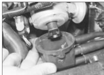
4.2c ... and remove the cap from the end of the distributor
