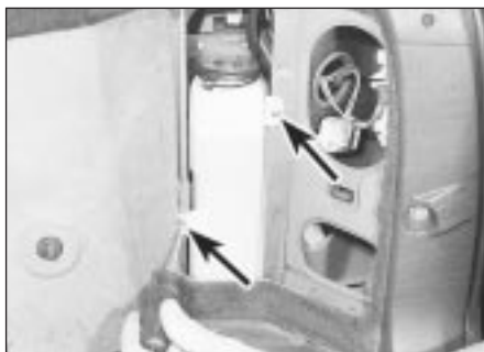
19.8a Remove the two securing screws (arrowed) . . .
