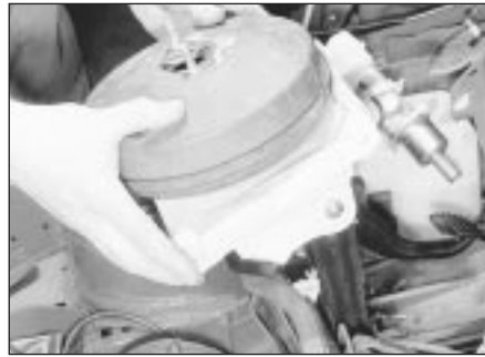
15.15 Removing the vacuum servo/pedal bracket assembly
