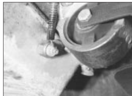
15.1 The oil temperature sensor is screwed into the sump
