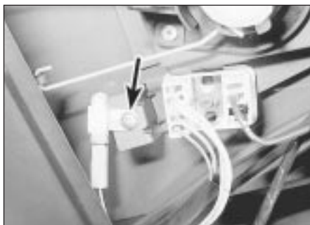
4.42 Luggage compartment courtesy light switch screw (arrowed) - Estate model
