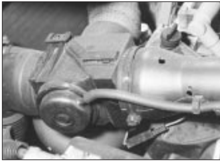
3.17 Air temperature control valve assembly (TU engine)
