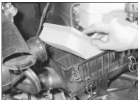
21.9 Removing the air filter element
