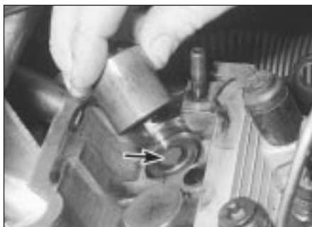
11.16a Lift out the follower and remove the shim (arrowed)
