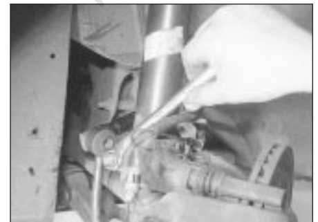
4.5 Unscrewing the hub carrier-to-suspension strut clamp bolt
