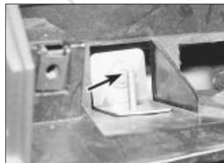
30.23 Upper facia securing bolt (arrowed)
