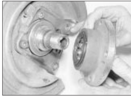
10.11a Fit the hub assembly ...
