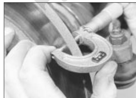
7.3 Using a micrometer to measure disc thickness
