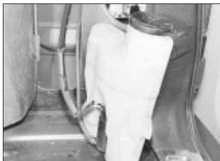
19.8b . . . and lift out the tailgate washer fluid reservoir
