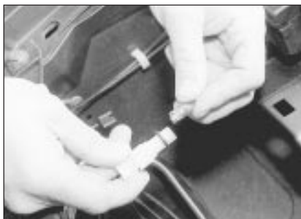
5.11 ... and withdraw the bulb
