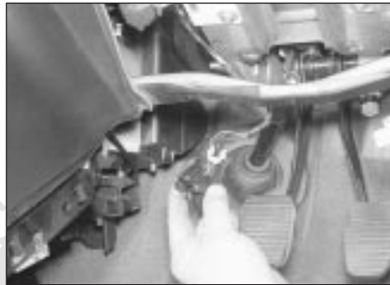
30.62b . . . then pull the connector from the steering column bracket
