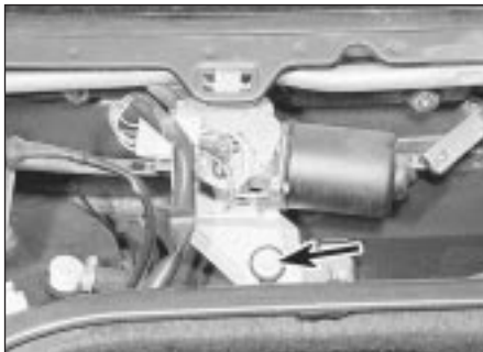
17.8a Windscreen wiper motor securing nut (arrowed)
