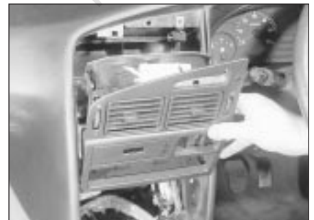
11.15 . . . then withdraw the housing
