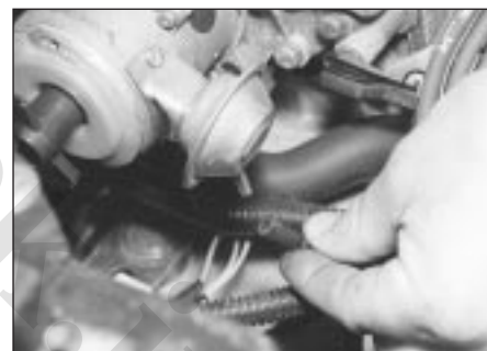
4.3b ... and the vacuum diaphragm hose
