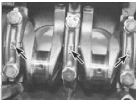
11.17 Main bearing cap identification markings (arrowed)
