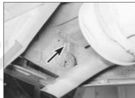
7.11 Rear underbody shield securing clip (arrowed) - Estate model
