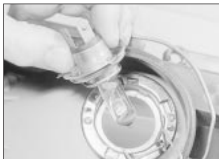
5.4b . . . then withdraw the headlight bulb
