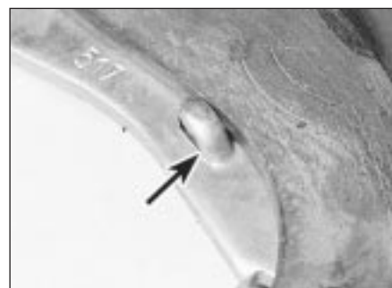
9.9 Check that the handbrake lever stop-peg (arrowed) is against the shoe edge
