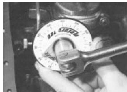
19.22b . . . then through the angle specified for stage 3
