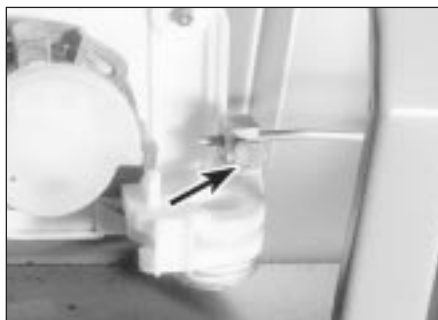
17.4 Unscrew the lock operating rod pinch-bolt (arrowed)
