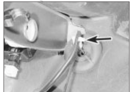
7.4 Accelerator cable connection to accelerator pedal (arrowed)
