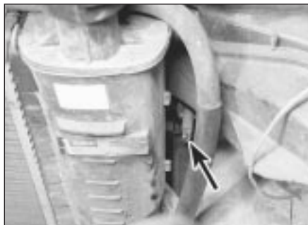
8.2b Headlight beam horizontal fine adjuster (arrowed)
