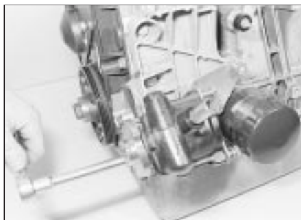
22.9a Unscrew the securing bolts ...
