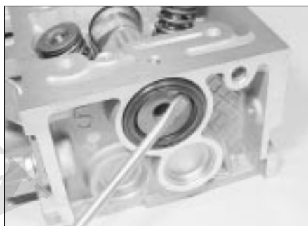
10.9a . . . prise out the oil seal . . .
