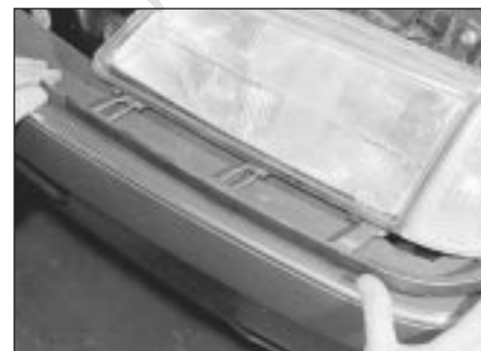
7.7 Removing the trim plate from the bottom of the headlight
