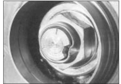
10.12c ... stake the hub nut firmly into the stub axle groove
