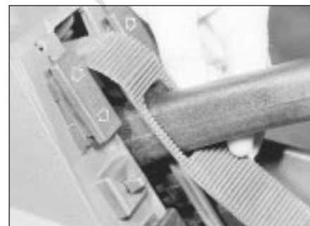
29.9 Removing the handbrake lever dust cover - models up to 1992
