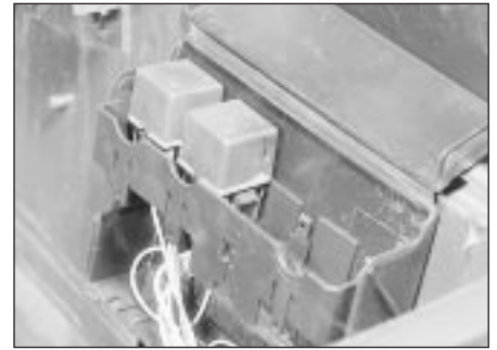
3.14d Relays in engine compartment relay box - models up to 1992
