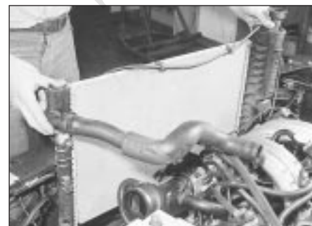
3.11 Lifting out the radiator
