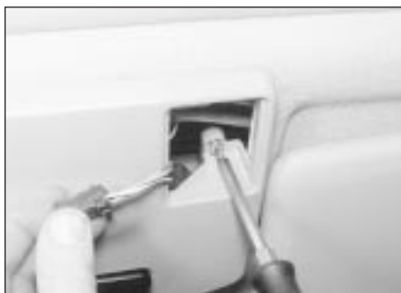
20.31 Removing a roof console securing screw
