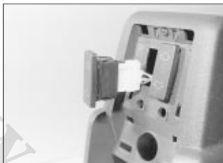
4.25 ... for access to the switches
