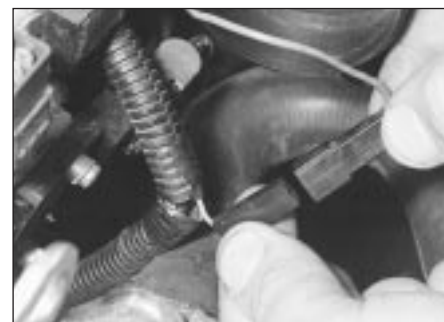
3.3 On breakerless ignition models, disconnect the capacitor wiring connector, and release the TDC sensor connector . . .
