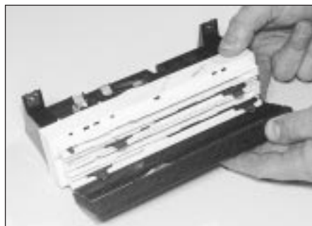
6.19 Unclip the front panel from the heater control unit
