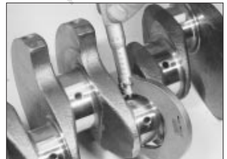
14.10 Measuring a crankshaft big-end journal diameter
