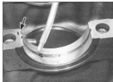
18.41 Ensure each bearing shell tab (arrowed) is correctly located, and apply clean engine oil
