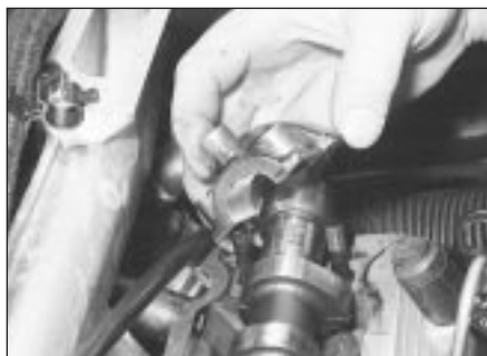
10.32 . . . and remove the camshaft bearing caps . . .
