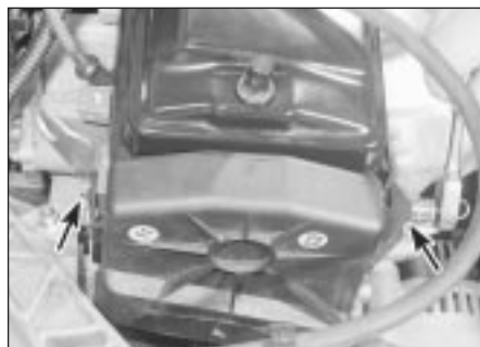
5.1a Undo the two retaining bolts (arrowed) . . .
