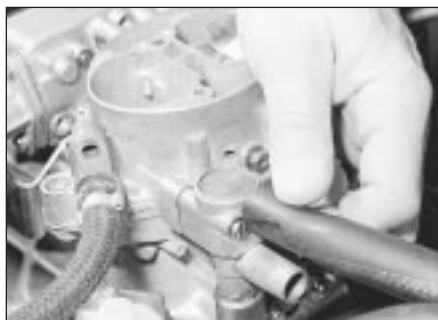
12.5 Disconnecting the float chamber breather pipe
