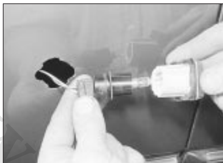
5.20 Removing the bulbholder from the front direction indicator side repeater light
