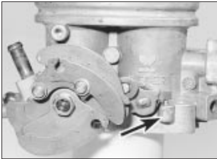
14.6a Secondary throttle adjusting screw (arrowed) . . .
