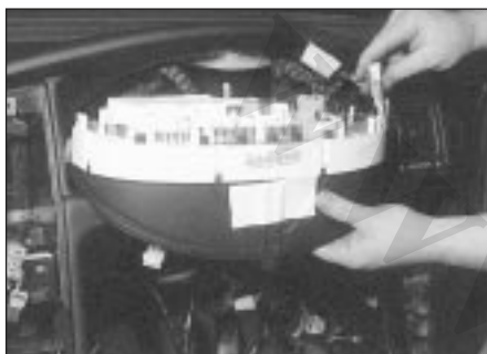
9.23 . . . until the instrument panel can be withdrawn
