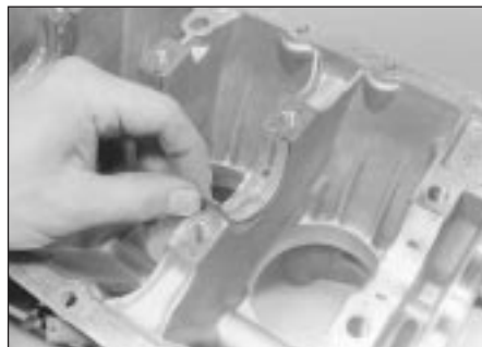
18.20 On TU series engines, note that the grooved bearing shells are fitted to Nos 2 and 4 main bearing journals
