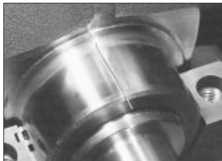
18.24 Plastigauge in place on a crankshaft main bearing journal
