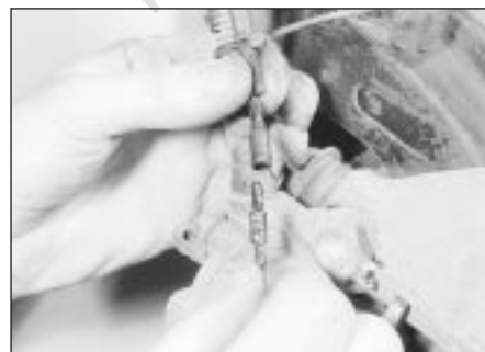
4.2 Disconnecting the pad wear sensor wiring connector
