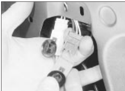
22.3 Disconnecting the door mirror wiring connectors
