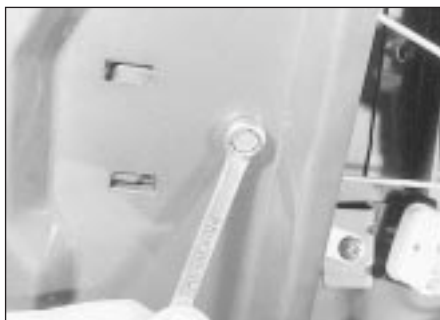
20.8 Unscrewing the tailgate lock motor securing bolt
