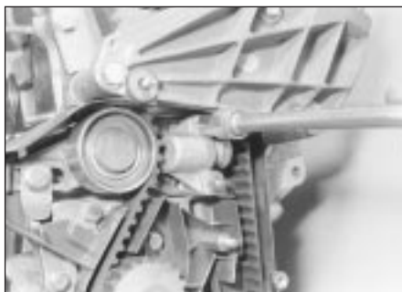
7.7 On early 1580 cc and 1905 cc models, slacken the tensioner assembly retaining nuts . . .
