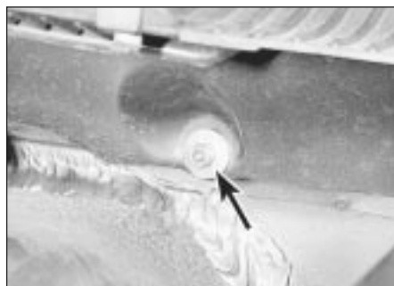
30.20 Facia securing nut (arrowed) in scuttle
