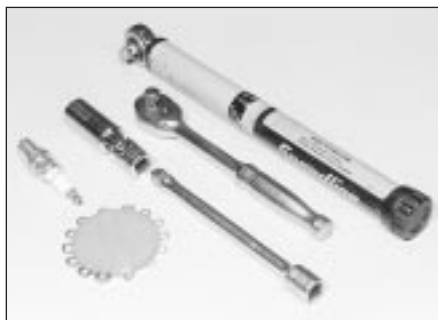
11.7 Tools required for spark plug removal, gap adjustment and refitting
