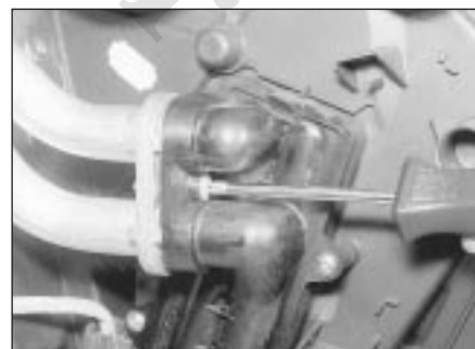
9.35 Remove the screw securing the heater pipes to the matrix connector
