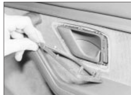
13.2 Removing the door interior handle surround
