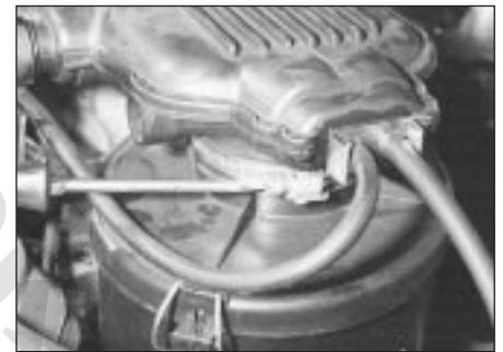
2.2a ... slacken the retaining clips ...
