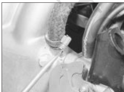
18.3 Disconnecting the brake servo vacuum hose
