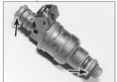
14.30 Injector O-ring seals (arrowed)
