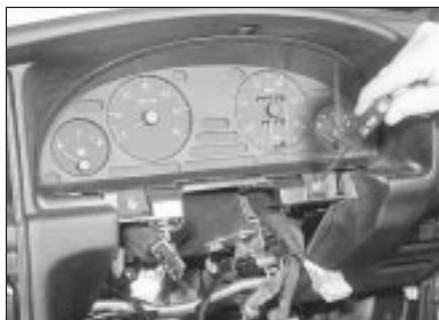
9.21 Unscrew the lower instrument panel securing screws
