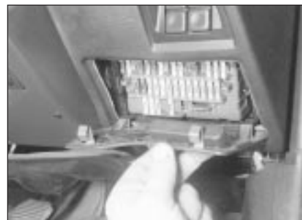
3.3c Removing the fusebox cover - later models
