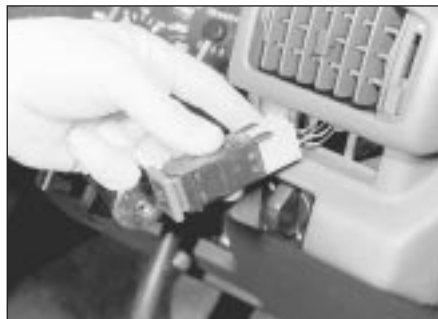
4.11 Removing a driver's side facia-mounted switch - models up to 1992
