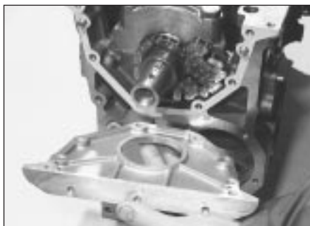
11.15 Removing the oil seal carrier from the front of the cylinder block - XU engine
