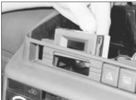
11.5 Removing the clock - models up to 1992
