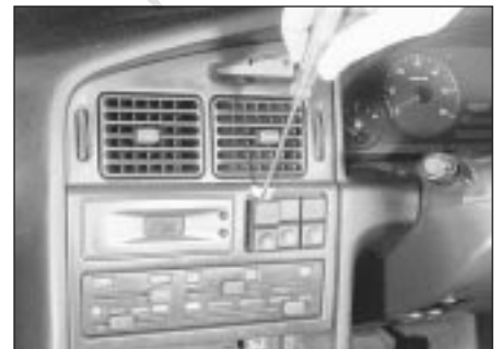
4.14 Prising out a facia-mounted switch - models from 1993
