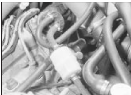
8.1 Fuel filter location on carburettor models
