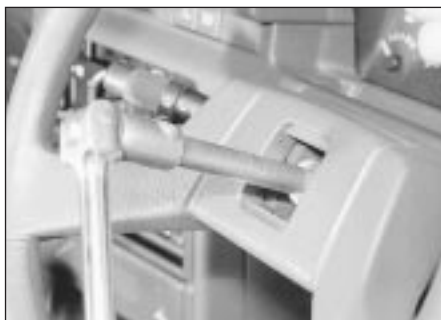
16.4 Unscrewing the steering wheel nut
