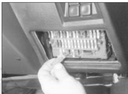
3.7 Removing a fuse using the plastic tool
