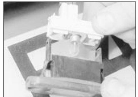
5.43 . . . and unclip the bulbholder from the lens - Estate model
