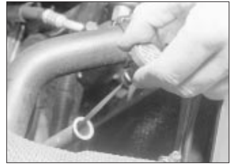
4.2a Withdrawing the automatic transmission dipstick
