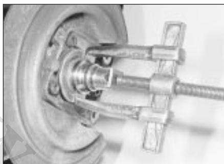
10.6b Removing the inner bearing race . . .
