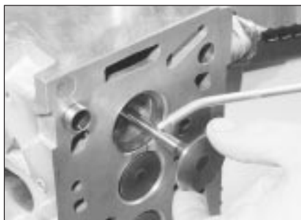
9.1 Lubricate the valve stems prior to refitting
