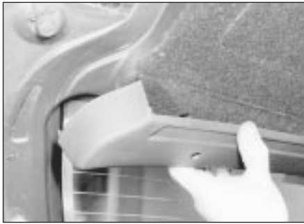
19.2 Withdraw the plastic trim panel from the tailgate . . .
