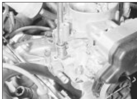
12.10a Remove the remaining nuts . . .
