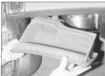
28.14 . . . and withdraw the glovebox - models from 1993
