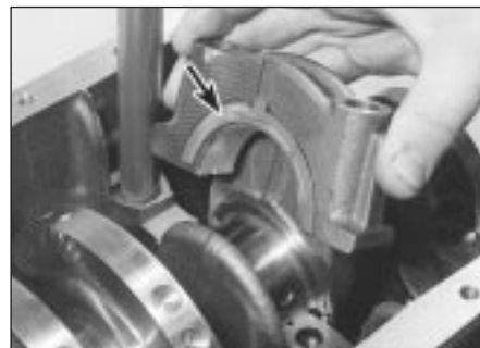
11.19 Removing No 2 main bearing cap. Note the thrustwasher (arrowed)
