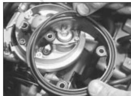
15.15b . . . then lift off the plastic ring and recover the sealing ring
