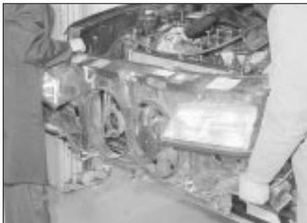
11.16 Withdrawing the body front panel assembly
