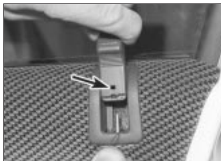
13.14b Push the button onto the rod until retaining tab appears in upper hole (arrowed)
