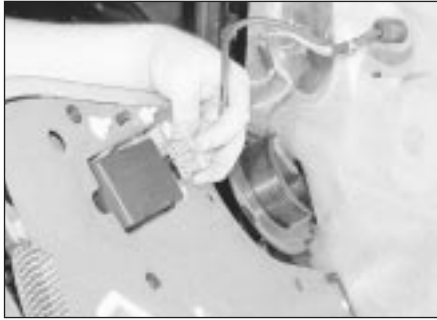
21.2 Disconnecting wiring plug from the electric windows electronic control unit
