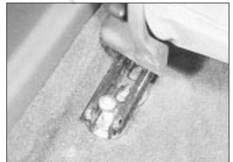
26.3 Front seat rear securing bolt partially removed
