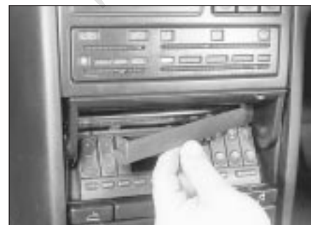
20.12 Prise the trim panel from the top of the radio/cassette player
