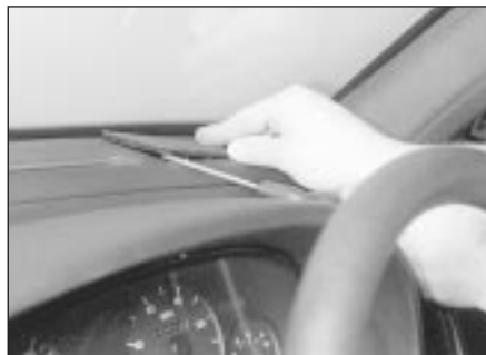
21.9a Prise the loudspeaker from the fascia . . .
