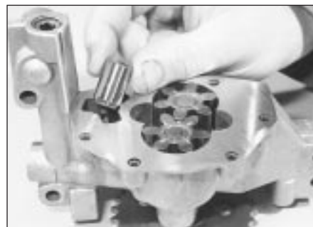
14.5c ... and relief valve piston, noting which way round it is fitted
