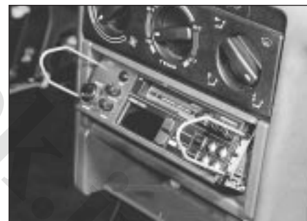
20.3 . . . then insert the removal tools . . .
