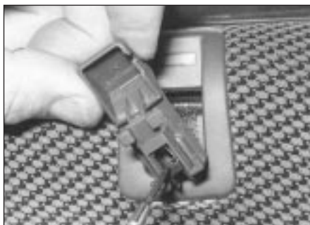
13.14a Position the lock button locating tab in the lower position
