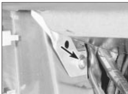
30.21 Lower facia mounting bracket-to-footwell bolt (arrowed)
