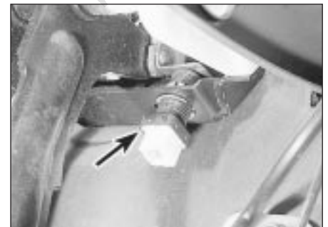
22.1 Stop-light switch (arrowed) on brake pedal bracket
