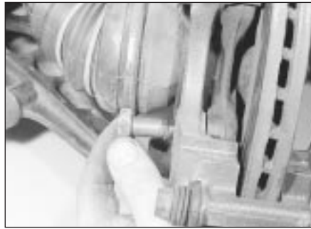
7.7 Removing a Girling caliper mounting bracket bolt
