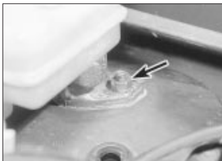
13.5 Master cylinder securing nut (arrowed)
