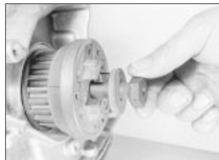
7.11a Remove the crankshaft sprocket retaining bolt ...
