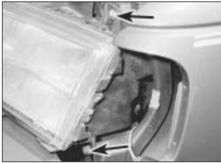
7.8 Outer headlight securing bolts (arrowed)
