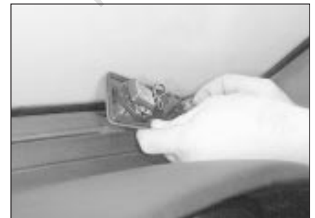
21.9b . . . and disconnect the wiring plug - models from 1993
