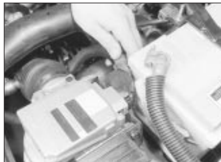
2.1 Disconnecting the airflow meter multi-plug (Bosch L3.1-Jetronic)
