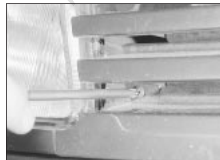
25.2 Remove the grille front securing screws . . .
