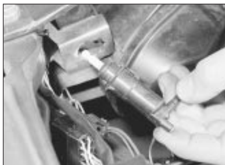
7.4 Removing a cable-operated headlight adjuster
