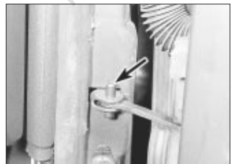
12.3 Drive the roll-pin (arrowed) from the door check strap
