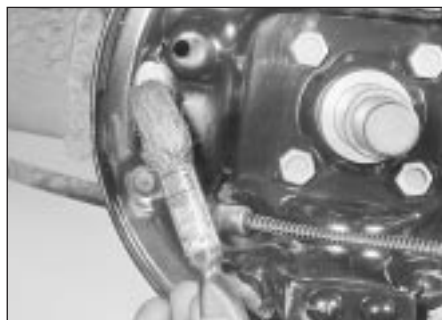
6.17 Apply high-melting-point grease to the shoe contact points on the backplate
