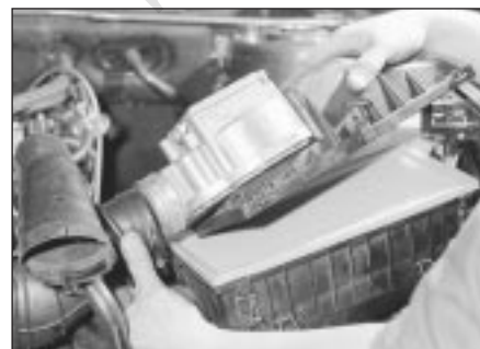
21.8 Lifting off the top cover
