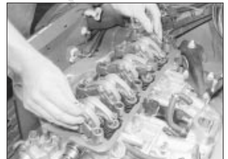
11.34 . . . and refit the rocker arm assembly
