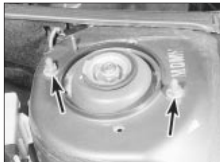
4.2 Suspension strut top mounting nuts (arrowed)
