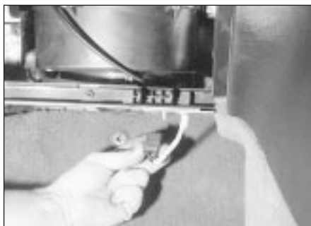
9.59 Disconnect the blower motor wiring plug
