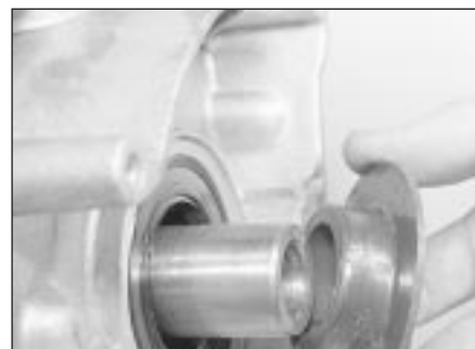
7.12 Remove the flanged spacer if necessary
