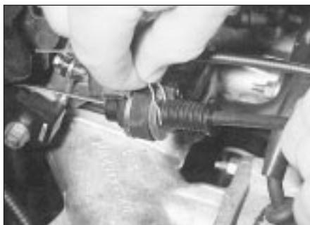
7.9 Adjusting the accelerator cable
