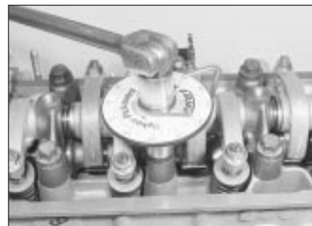
11.38 . . . then through the angle specified for stage 2
