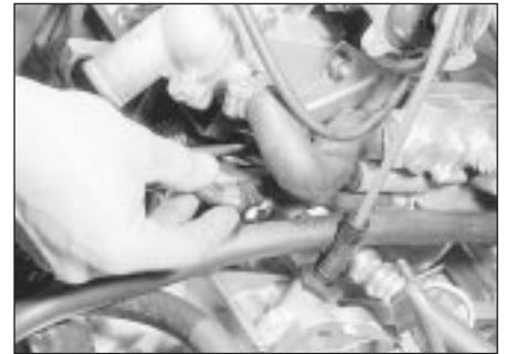
14.45 Disconnecting the supplementary air device plug
