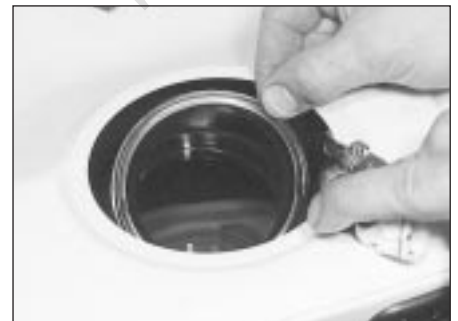
9.12b . . . and recover the rubber sealing ring
