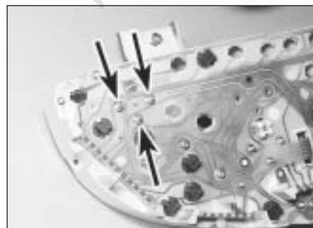
10.9 Fuel gauge securing nuts (arrowed)
