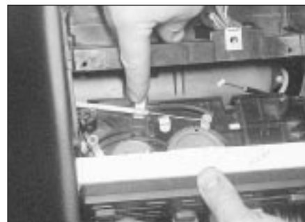
9.24 Disconnect the control cables from the heater control unit - models from 1993
