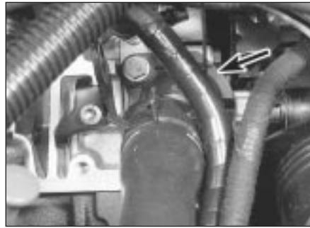
4.4b Thermostat housing cover (arrowed) - 2.0 litre engine
