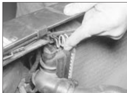
3.10 Releasing a radiator upper securing clip
