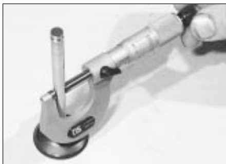
8.11 Measuring a valve stem diameter
