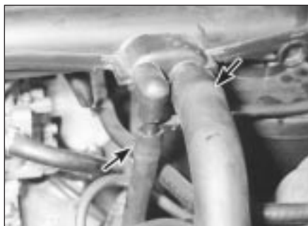
21.1 On TU models disconnect the hoses from the front of the duct . . .
