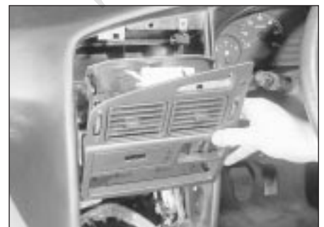
30.40 Withdrawing the ventilation nozzle housing
