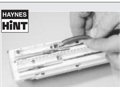
A length of rubber tubing can be used to remove and refit the bulbs
