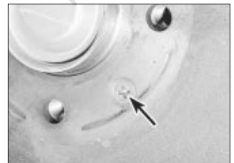
9.2 Rear brake drum retaining screw (arrowed)
