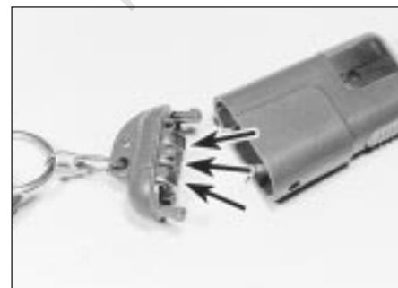
20.35 Rear cover removed from remote transmitter to expose batteries (arrowed)
