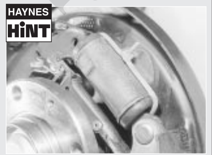
Restrain the wheel cylinder piston with a cable-tie or a strong elastic band
