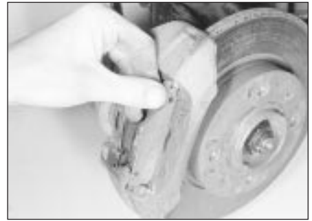
4.6 Withdrawing the outer brake pad - Bendix caliper
