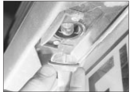
5.39 Prise the lens from the bumper . . .
