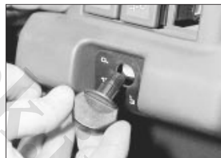
9.5 Prise off the headlight adjuster switch knob
