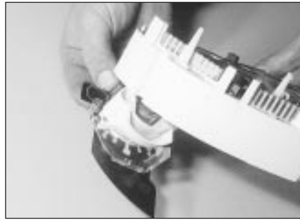
10.11a . . . then withdraw the gauge . . .
