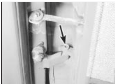
12.6 Door pivot pin (arrowed)
