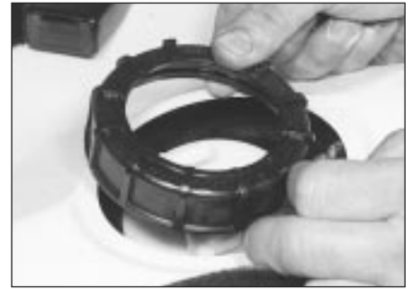
9.11 Unscrew the locking ring . . .
