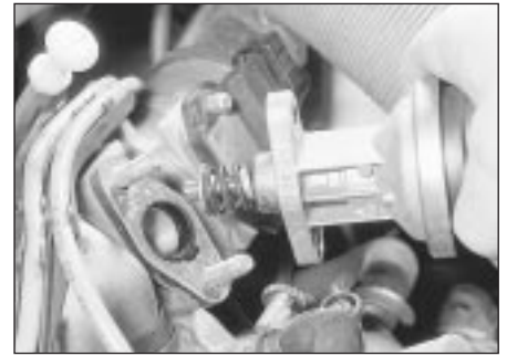
4.5 Removing the fuel pump (XU engine)
