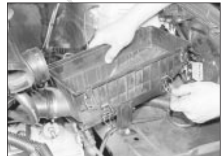
2.4 Removing the air cleaner housing
