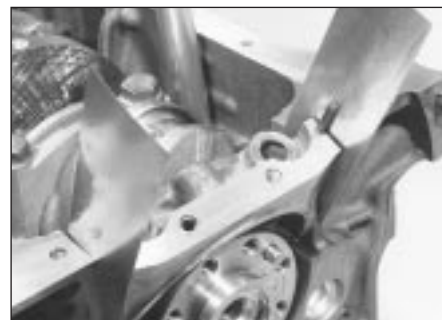
18.73a Fitting No 1 main bearing cap, using metal strips to retain the side seals
