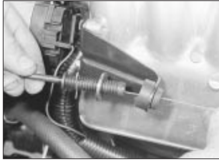
3.1b Disconnecting the accelerator cable end fitting (Bosch L3.1 system)
