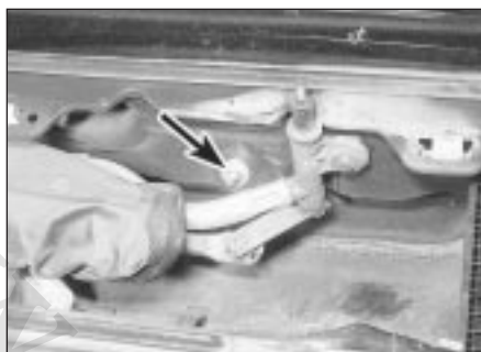
30.70 Facia securing nut (arrowed) in scuttle
