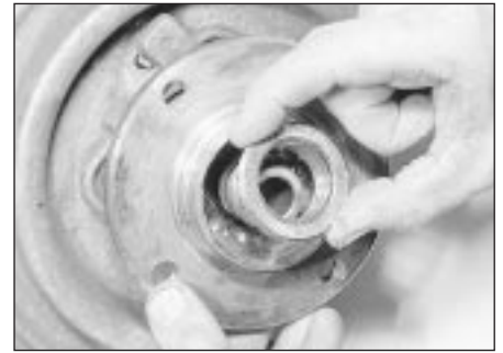
10.11b ... followed by the outer bearing race ...
