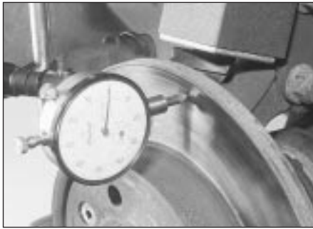
7.4 Checking disc run-out using a dial gauge
