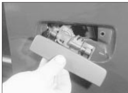
14.8 Withdrawing the exterior door handle
