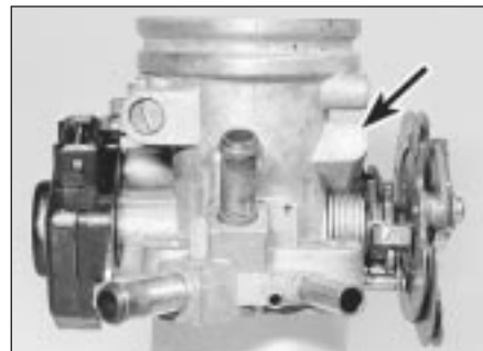
14.3 Tamperproof cap covering primary throttle stop screw (arrowed)
