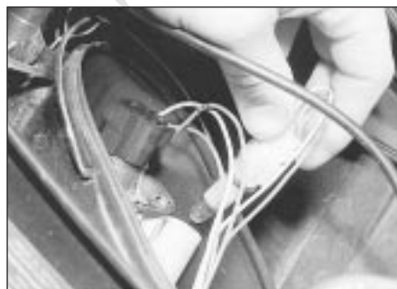
5.10 Pull out the sidelight bulbholder . . .
