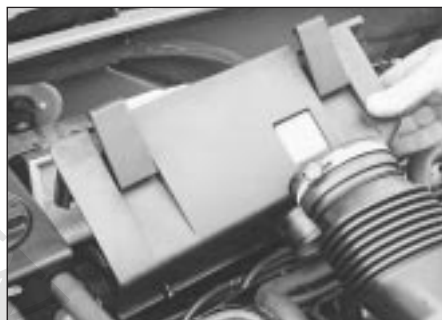
21.14c Lift off the filter cover ...
