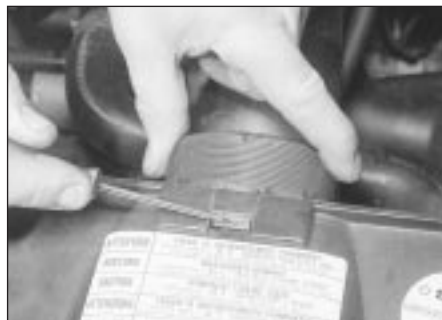
3.5a Depress the securing clip . . .
