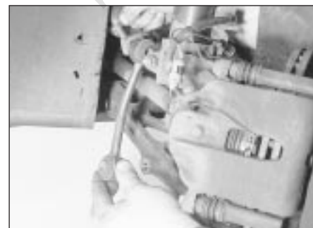
8.3 Removing an anti-roll bar drop link
