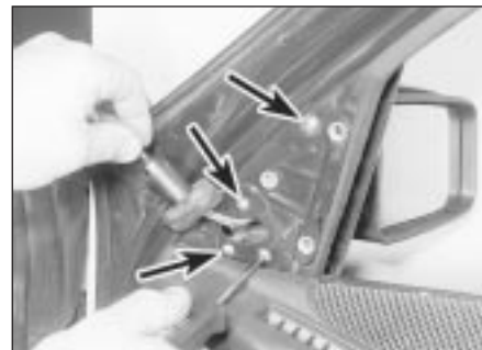
22.6a Remove the four securing screws . . .
