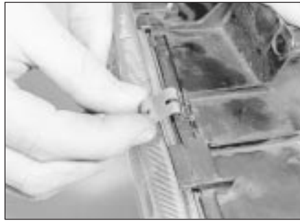
7.9 Removing a headlight lens securing clip
