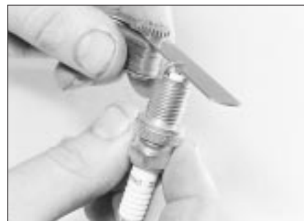
11.12 Measuring the spark plug gap with a feeler blade
