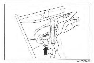
3. Remove the rubber by pulling it out.
