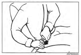
Insert the tongue plate into the open end of the buckle until an audible "click" is heard, indicating the belt is locked in the buckle.
