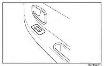
To open a window, press down on the front raised portion of the corresponding switch. To close a window, press down on the rear indented (▼) portion of the corresponding switch.
