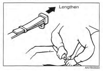
3. Grasp the free portion of the belt webbing and pull until the belt is snug over the hips and lower abdomen. If it becomes necessary to lengthen or shorten the belt, hold the latch plate tongue at right angles to the webbing and pull.
