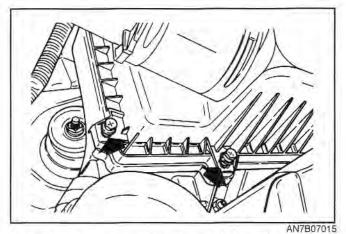
5. Install the cover. Install and tighten the (6) cover bolts.
