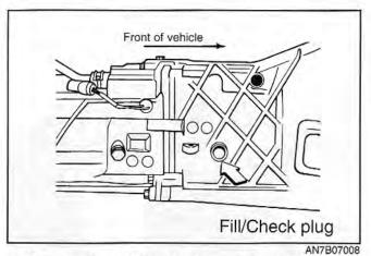
2. Remove the fill/check plug on the side of the transmission.
