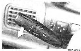
To flash the headlights, pull the lever toward you. It will return to the normal position when released. The headlight switch does not need to be on to use this flashing feature.
