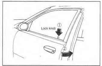
Depressing the door lock knob and then closing the door enables the door to lock without a key.
