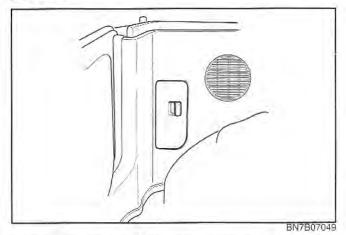
Pull out on the finger slots to remove the rear light cover.
