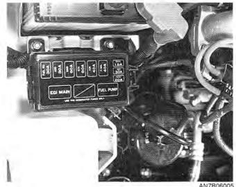
If the 80A "MAIN" fuse is blown, it must be removed as follows:
