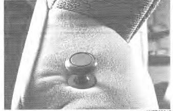
Pull up on one release knob (located on the outside top of each seatback) and, with your other hand, grasp the inside top of the same seatback and pull forward. Repeat this for the other seatback.
