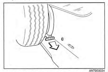
1. Reach behind the tire and pull the release lever on the carrier and swing the carrier out.
