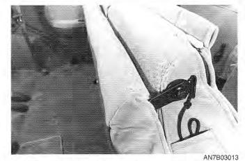
5. Grasp the rear of the seat, below the "fold," and pull up and forward. The seat will rotate to a near-vertical position.
