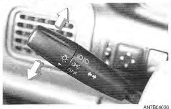
The ignition switch must be on for the turn signals to function. To turn on the turn signals, move the lever up or down. Green arrow indicators on the instrument panel indicate which turn signal is operating. They will self-cancel after a turn is completed. If the indicator continues to flash after a turn, manually return the lever to the OFF
