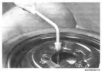
Open the tool compartment door, loosen the jack wing nut and remove the jack handle.
