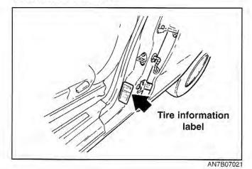
All tire pressures (including the spare) should be checked monthly when the tires are cold. "Cold Tires" means the vehicle has not been driven for at least three hours or driven less than 1.2 km (one mile). Recommended pressures must be maintained for the best ride, top vehicle handling, and minimum tire wear.
