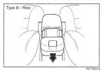
To access the rear console compartment, pull the latch rearward. To return to its original position, push it forward.
