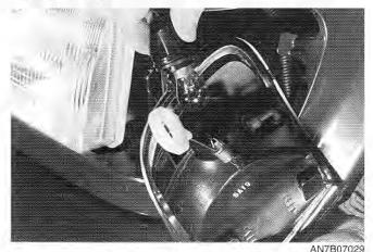
5. Remove the socket from the housing by turning the socket counterclockwise until the tabs on the socket align with the slots on the
