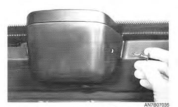
2. Pull out the retaining clips and remove the cover.
