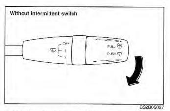
In the OFF position, pull the lever gently toward you, then push the lever forward to operate the wipers.
