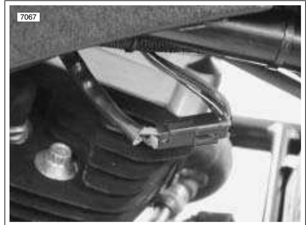
Figure 4-32. Fuel Pump Connector [86]
