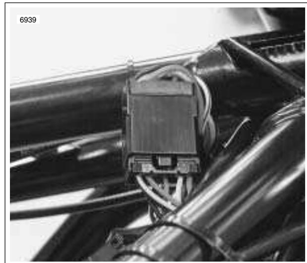
Figure 4-61. Speedometer/Tachometer Connector [39]
