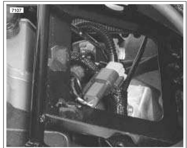
Figure 7-65. Speedometer Sensor Connector (Battery Removed For Illustration Purposes Only)
