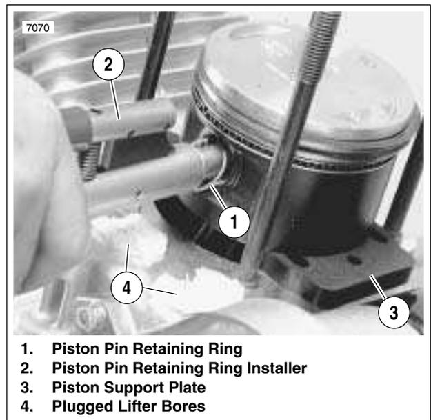
Figure 3-42. Installing Piston Retaining Rings
