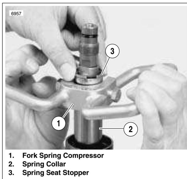
Figure 2-56. Front Fork Spring Compressor
