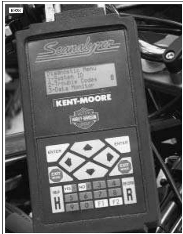
Figure 4-9. Scanalyzer Diagnostic Menu
