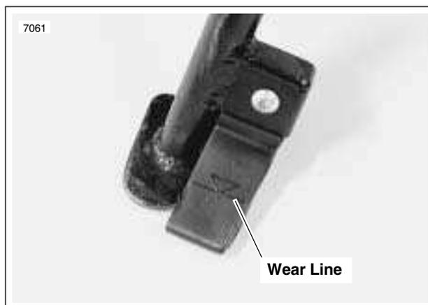
Figure 2-139. Side Stand Dragger Wear Limit
