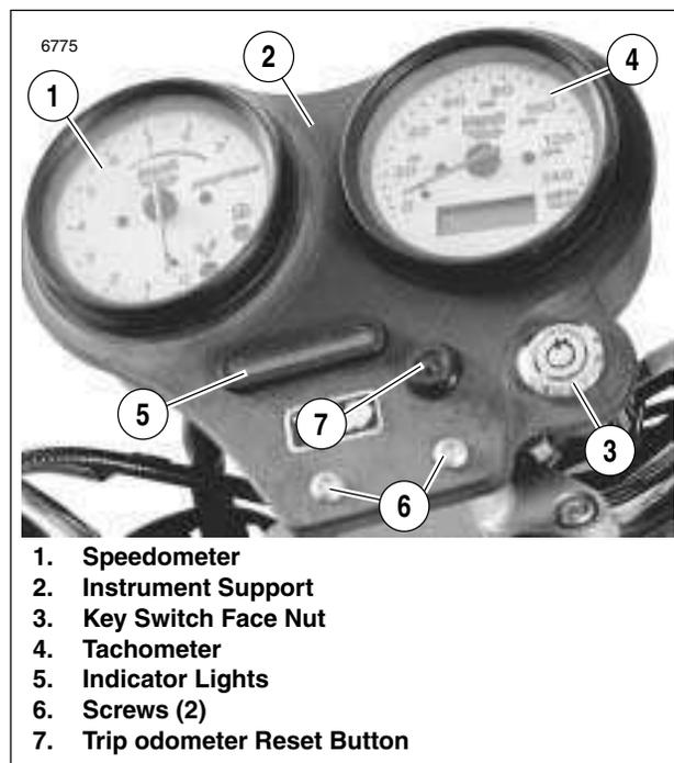
Figure 2-100. Instrument Support
