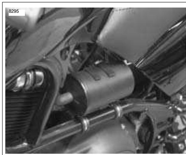
Figure 4-110. Carbon Canister Installation (Typical).
