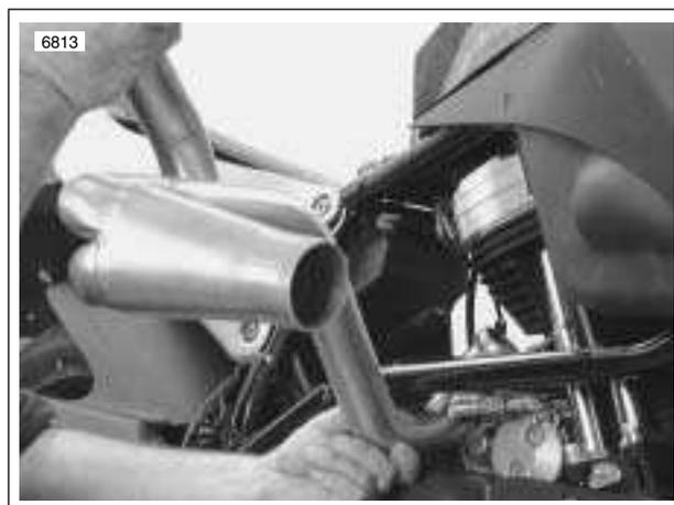
Figure 2-108. Exhaust Header Positioning
