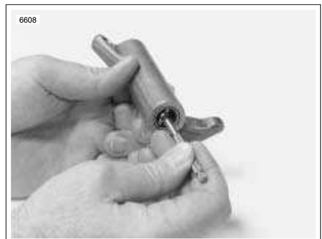
**Figure 3-15. Measuring Rocker Arm Bushing Inner Diameter**
