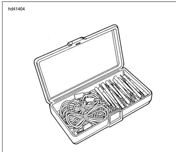
**Figure 4-35. Harness Connector Kit**
