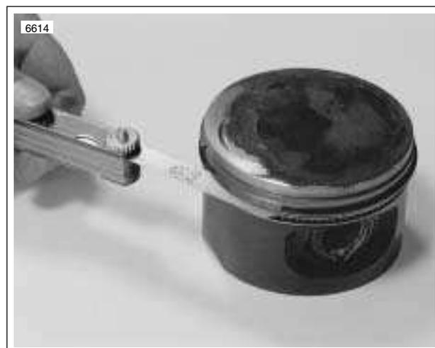
**Figure 3-39. Measuring Ring Clearance in Groove**
