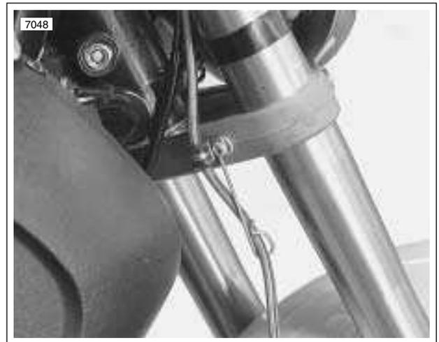
**Figure 2-37. Lower Triple Clamp**
