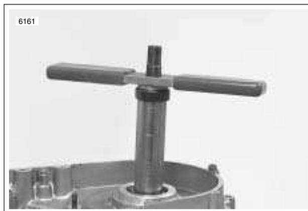
**Figure 3-94. Installing Flywheel Spacer and Outer Bearing**
