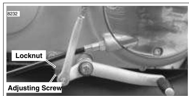
Figure 1-28. Measuring Primary Chain Adjustment
